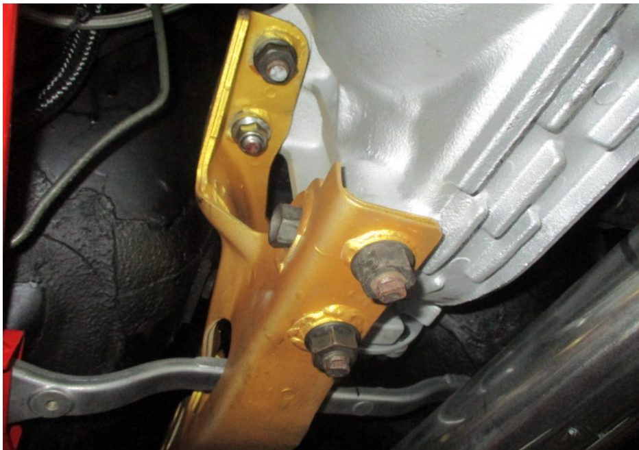
Photo 11 shows a closer view of the bracket that reinforces the support of the Motor Car's transmission. This was at the end that bolts onto the Motor Car's rear differential.
