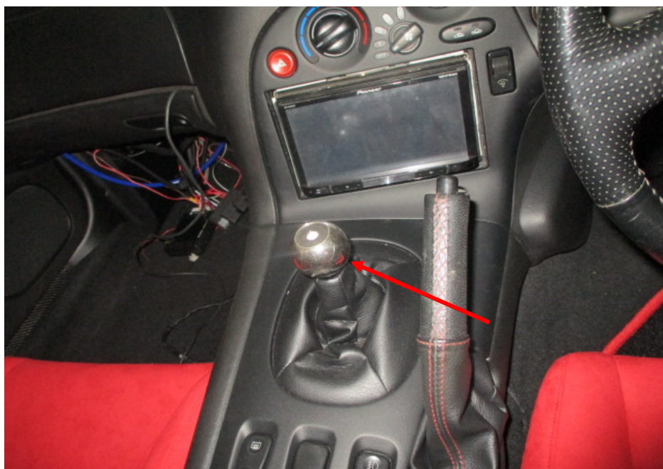
Photo 13 shows the gear shifter (arrowed) that was fitted on the Motor Car, for manually selecting the transmission gear to be engaged. The gear selector fork from the transmission of the Motor Car connects to this gear shifter through the floorboard of the Motor Car.
