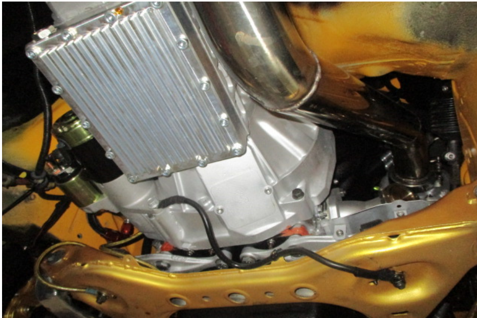
Photo 4 shows the front (input) side of the Motor Car's transmission, which was observed to be bolted to the crankshaft side (torque converter) of the engine block. The transmission is supported by its direct bolt on onto the crankshaft side of the engine block, and connection of the propeller shaft to the rear differential (refer to photograph 6, 7 & 9 below).
