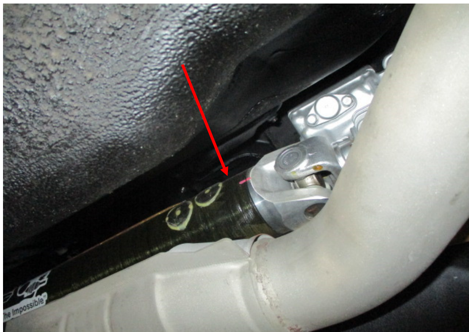
Photo 7 shows the propeller shaft (arrowed) of the Motor Car. The rear (output) side of the Motor Car's transmission (refer to photograph 6 above) connects to this propeller shaft, linking to the rear differential of the Motor Car, providing the drive to the rear wheels.
