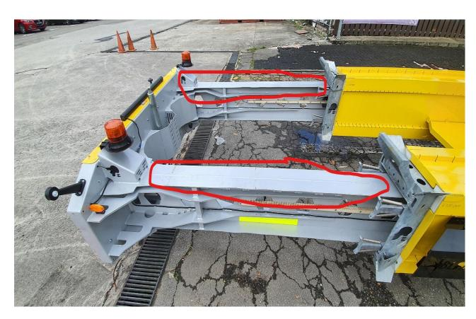
The H Beam Both Left and Right Side are bend and twisted
