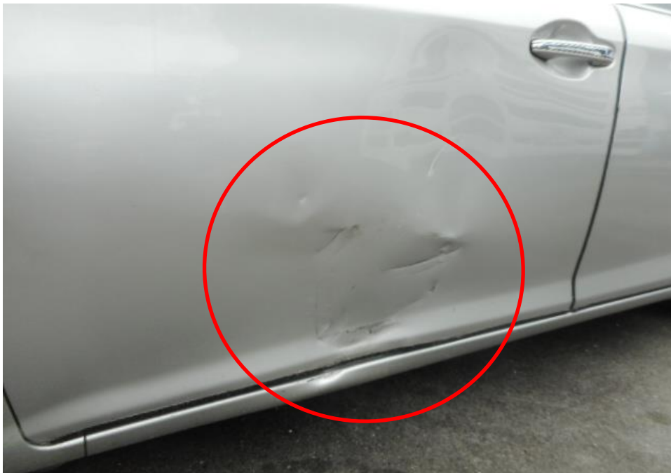
Photo 7 shows a close up view of the Motor Car's left body at the time of my inspection. The left portion of the Motor Car was observed to have sustained damage. Its left door panel was the body parts that were damaged as a result of the accident.
