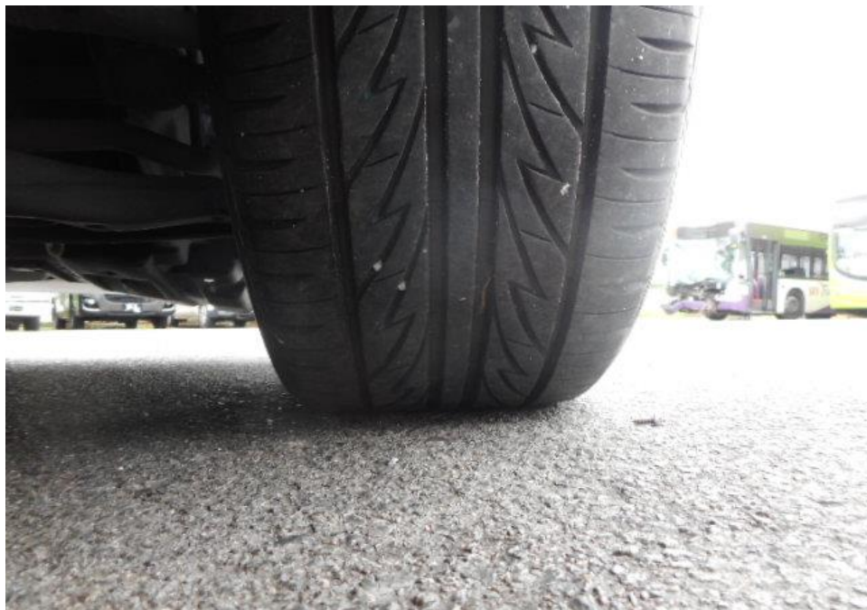
Photo 9 shows the condition of the front right tyre of the Motor Car, which was observed to be in serviceable condition with remaining tread depth of approximately 5.2mm. The tyre was sufficiently inflated for vehicular operation with no tear, cut or burst mark(s) on the outer and the inner sidewalls as well as across the tread. The 4 tyres of the Motor Car were wrapped around standard steel wheel rims without any damage.
