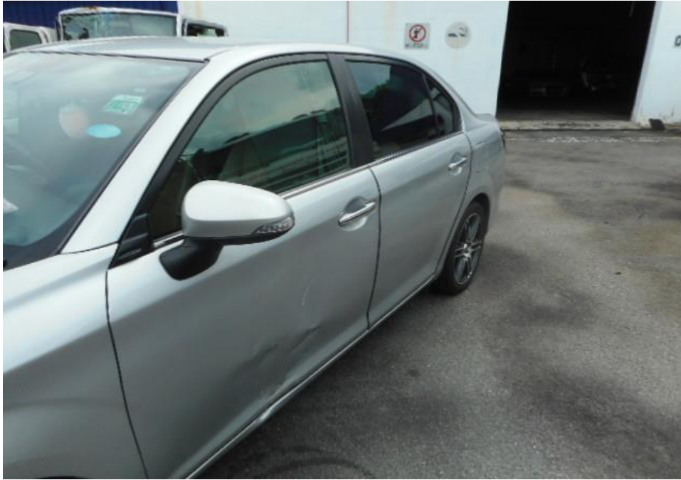
Photo 6 shows a general view of the Motor Car's left body at the time of my inspection. The left portion of the Motor Car was observed to have sustained damage. Its left door panel was the body parts that were damaged as a result of the accident.
