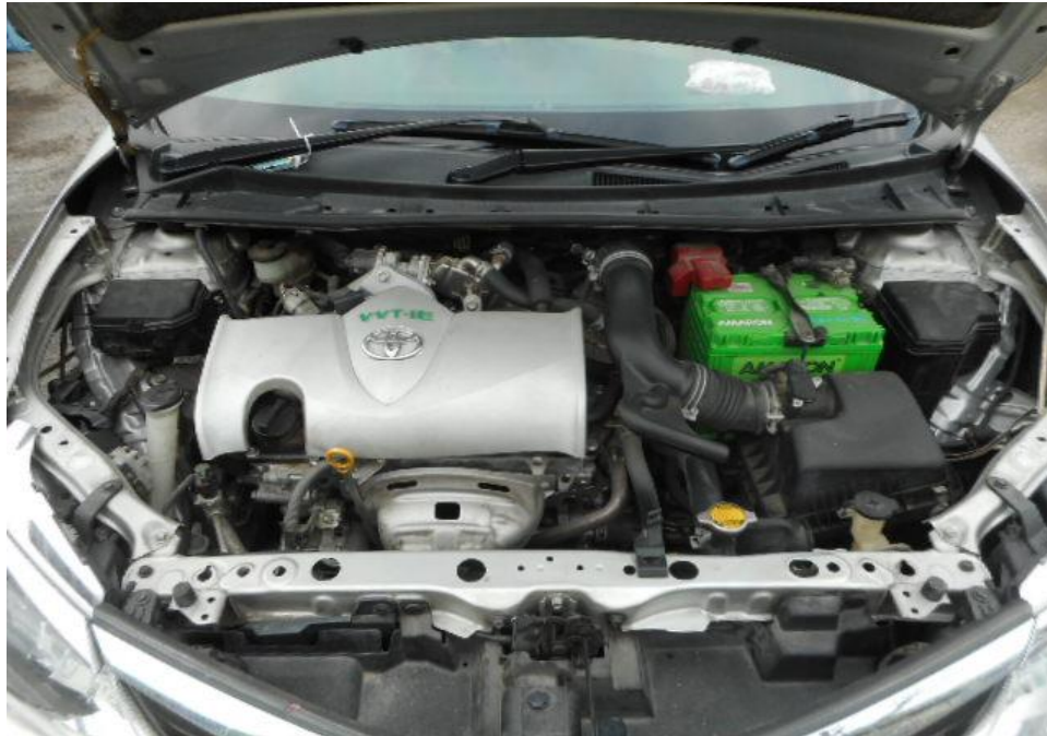
Photo 13 shows a general view of the Motor Car's engine compartment. The various parts and components inside the engine compartment were unaffected by the accident. There was also no sign(s) or indication(s) of fluid leakage and/or fluid stain within the engine compartment.
