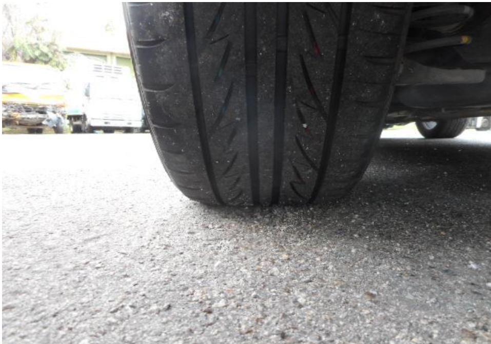
Photo 11 shows the condition of the rear left tyre of the Motor Car, which was observed to be in serviceable condition with remaining tread depth of approximately 3.4mm. The tyre, which was wrapped around steel wheel rim, was also observed to be sufficiently inflated for vehicular operation. The 4 tyres of the Motor Car were wrapped around standard steel wheel rims.
