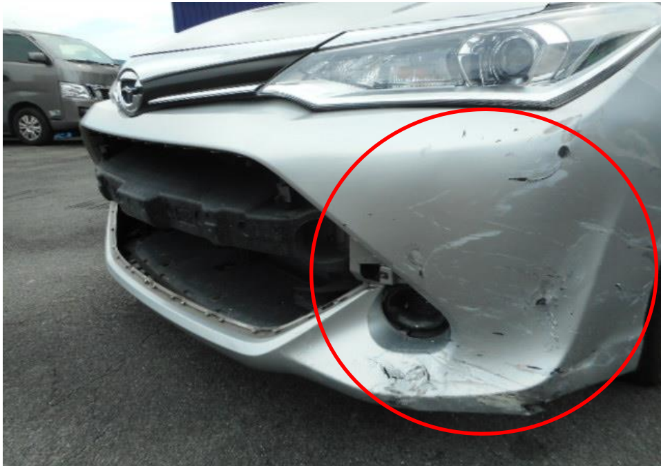
Photo 4 shows a close up view of the Motor Car's front body at the time of my inspection. The front portion of the Motor Car was observed to have sustained damage. Its front bumper (circled) was the body parts that were damaged as a result of the accident.
