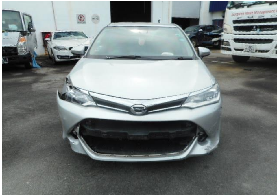
Photo 3 shows a general view of the Motor Car's front body at the time of my inspection. The Motor Car was observed to have sustained damage at its front and left portion. Its front bumper, front right headlamp and its front right fender as well as its left door panel were amongst the body parts that were damaged as a result of the accident.
