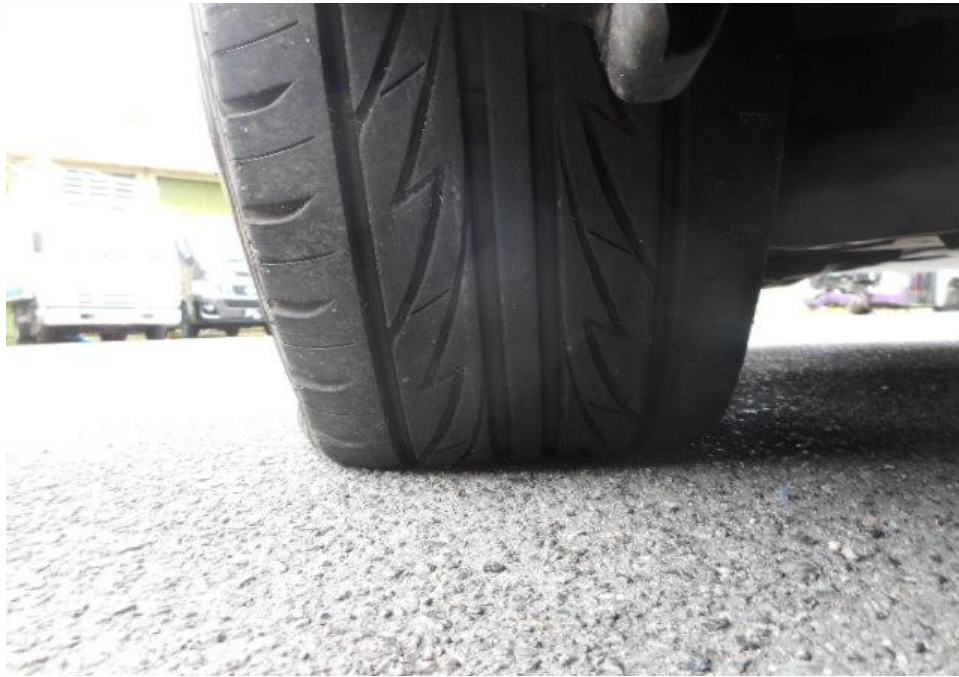
Photo 12 shows the condition of the front left tyre of the Motor Car, which was observed to be in serviceable condition with remaining tread depth of approximately 4.6mm. There was also no tear, cut or burst mark(s) on the outer and the inner sidewalls as well as across the tread of the Motor Car's 4 tyres.
