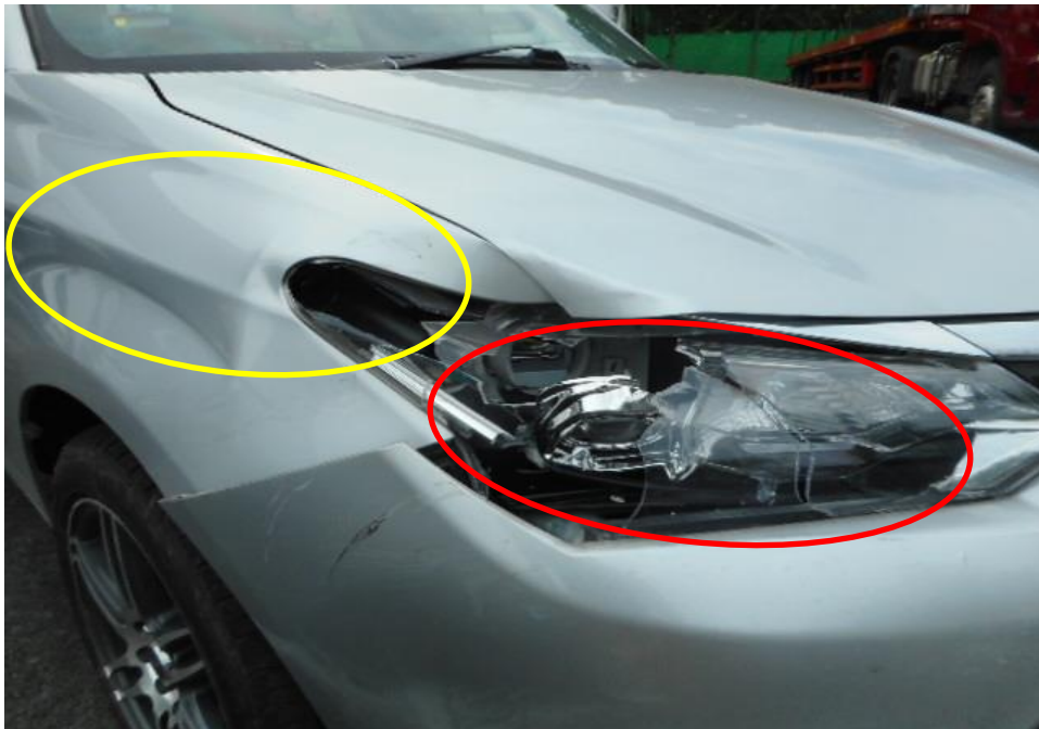
Photo 5 shows a close up view of the Motor Car's front body at the time of my inspection. The front portion of the Motor Car was observed to have sustained damage. Its front right fender (yellow circle) and front right headlamp (red circle) was the body parts that were damaged as a result of the accident.
