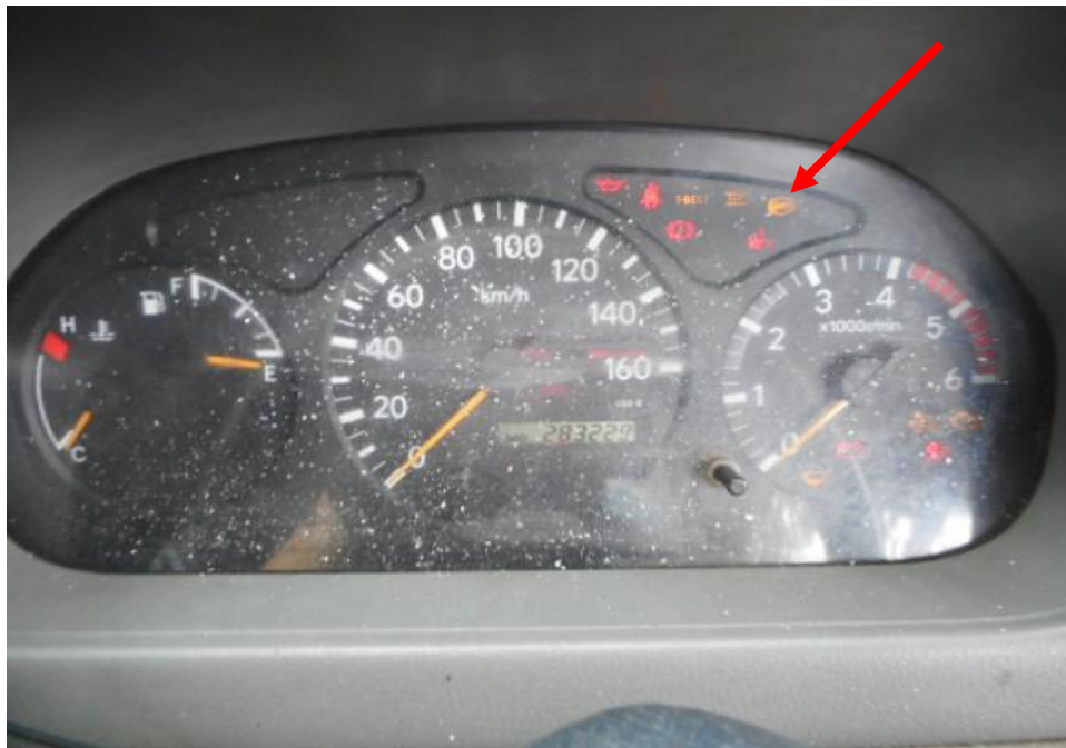
Photo 22 shows the warning light for Supplemental Restraint System (SRS) (arrowed) appearing on the instrument panel of the Motor Car during the self-test of its various electronic operating systems when its engine was cranked.
