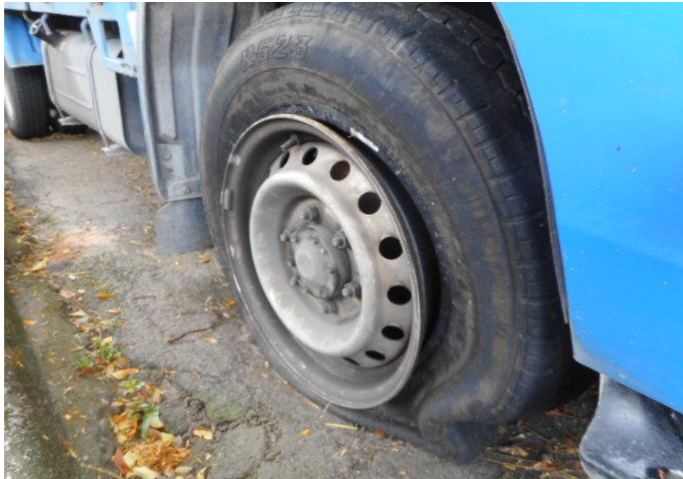
Photo 5 shows the condition of the front right tyre of the Motor Car, which was observed to be in unserviceable condition with remaining tread depth of approximately 3.8mm. The tyre was observed to be deflated and slip off as a result of the accident.
