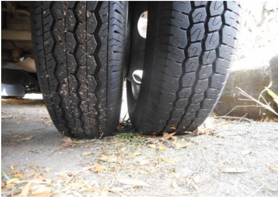
Photo 6 shows the condition of the rear right tyre of the Motor Lorry, which was observed to be in serviceable condition with remaining tread depth of approximately 5.9mm. The tyre, which was wrapped around standard steel wheel rim, it was observed to be sufficiently inflated for vehicular operation.
