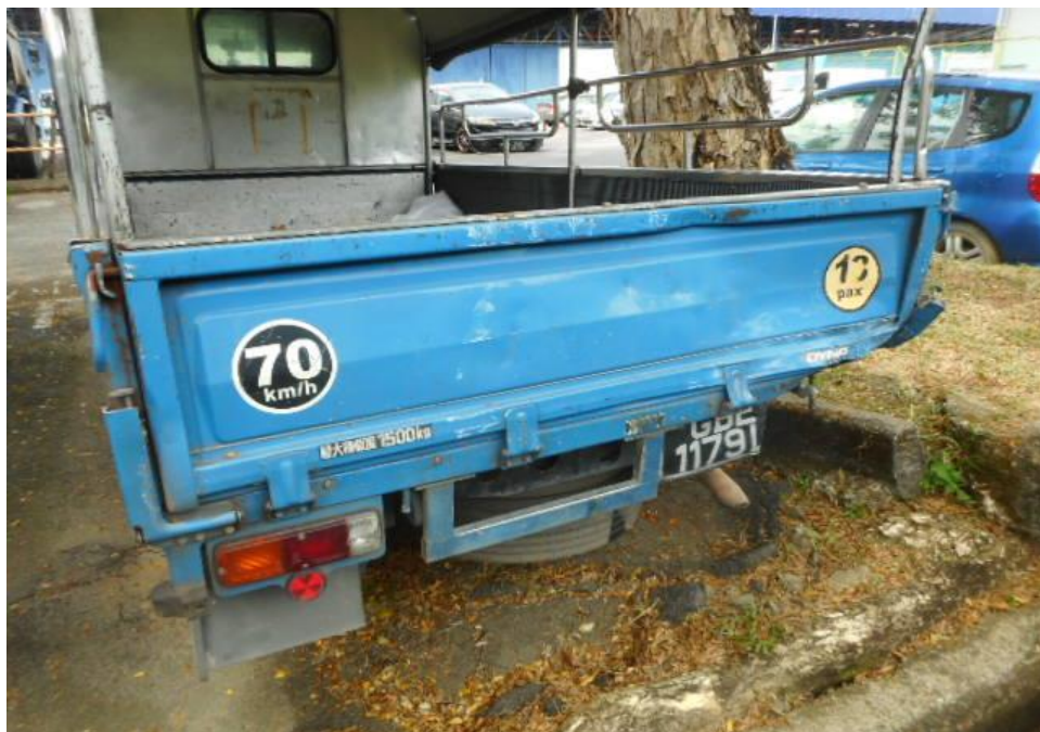
Photo 3 shows a general view of the rear body of the Motor Lorry at the time of my inspection. The Motor Lorry was observed to sustained damage at its rear portion. Its rear body panel and rear right brake lamp were damage at the time of my inspection as a result of the accident.
