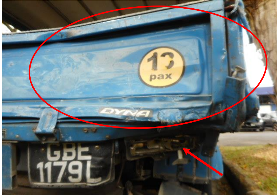
Photo 4 shows a close up view of the Motor Lorry's rear portion at the time of my inspection. Its rear body panel (circled) and rear right brake lamp (arrowed) was damage at the time of my inspection as a result of the accident.
