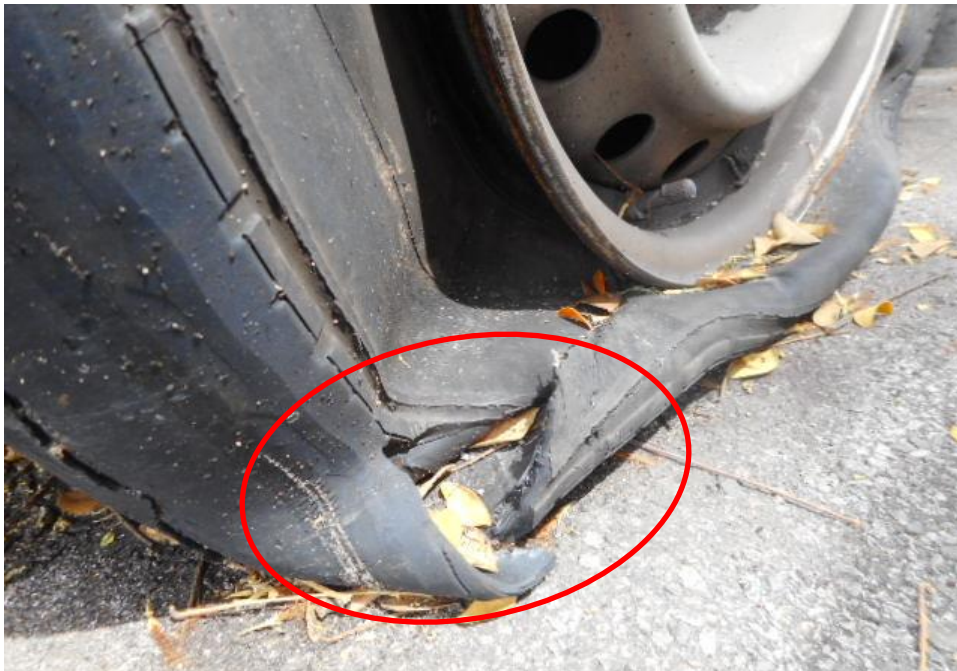
Photo 9 shows the close up condition of the front right tyre of the Motor Car, the tyre was observed to be deflated as a result of the cut sustained on the outer sidewall of the tyre (circled) as a result of the accident.
