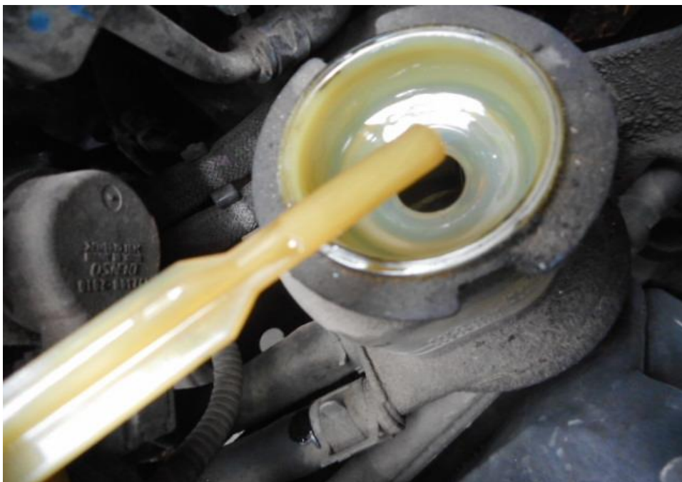
Photo 14 shows the power steering fluid reservoir of the Motor Lorry at the time of my inspection. The power steering fluid was observed to be of sufficient level and without any visible contamination.
