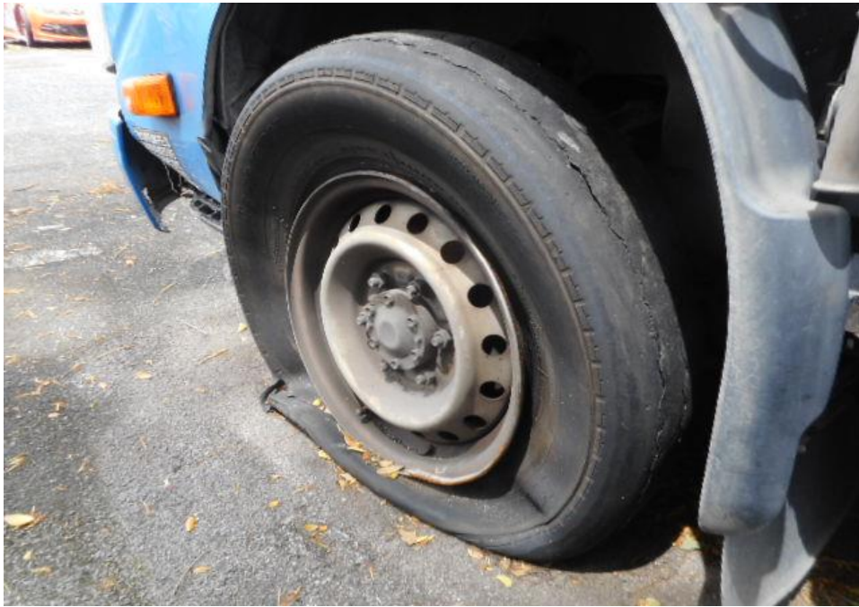
Photo 8 shows the condition of the front right tyre of the Motor Car, which was observed to be in unserviceable condition with remaining tread depth of approximately 3.8mm. The tyre was observed to be deflated as there was cut mark on the outer sidewall tyre as a result of the accident.
