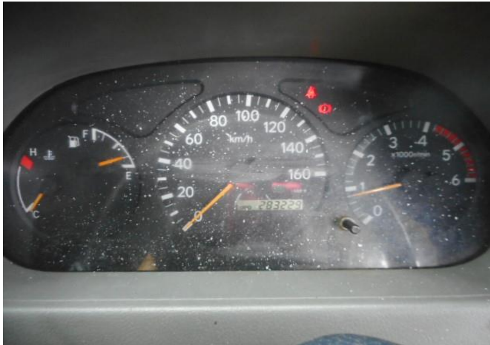
Photo 23 shows no warning lights illuminated on the instrument panel of the Motor Car after the engine was cranked. This would suggest that there was no abnormality to the electronic operating system of the Motor Car, like the SRS and etc.
