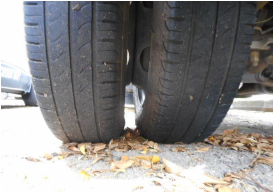
Photo 7 shows the condition of the rear left tyres of the Motor Lorry, which was observed to be in serviceable condition with remaining tread depth of approximately 2.3mm. The tyres, which were wrapped around standard steel wheel rim, were also observed to be sufficiently inflated for vehicular operation.
