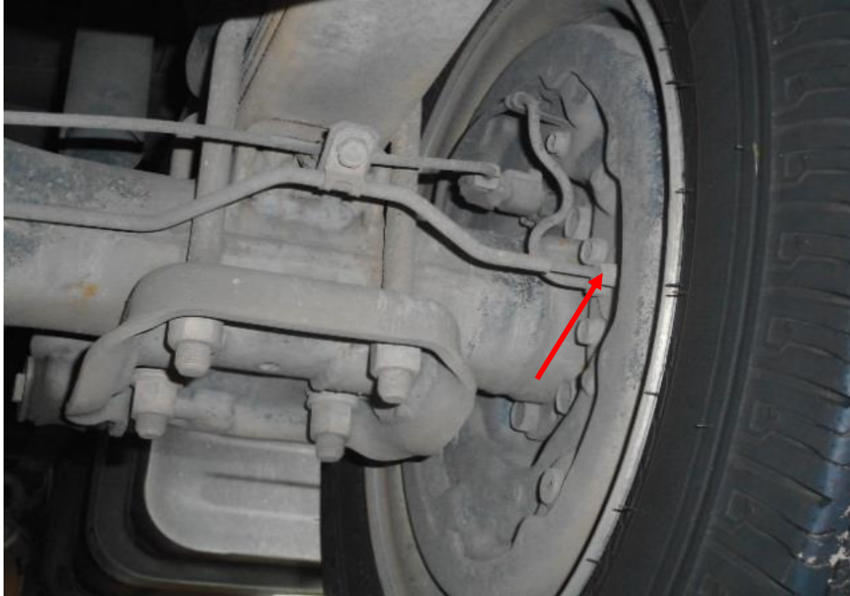
Photo 18 shows the brake pipe (arrowed) at the rear right wheel of the Motor Lorry. I did not observe any leakage of brake fluid at the time of my inspection of the Motor Lorry. My static tests of the Motor Lorry's braking system, along with my visual examination of the various mechanical components in the braking system, had indicated that there was no internal leakage of pressure/vacuum. Hence the braking system of the Motor Lorry was likely to be in serviceable condition at the material time of accident.
