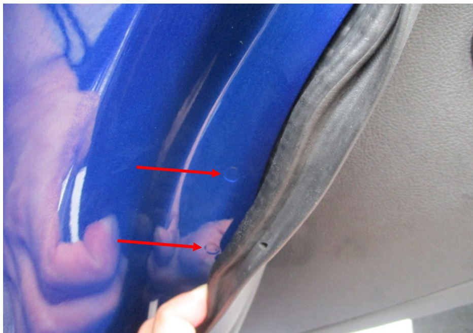
Photo 30 shows the left side "A" pillar of the Motor Car. I did not find any weld marks other than original spot weld marks (arrowed) on the left side "A" pillar of the Motor Car which, indicates that there was no re-welding works carried out. In general, I had found all the non-detachable body panels of the Motor Car to be originally fitted at the time of my inspection.
