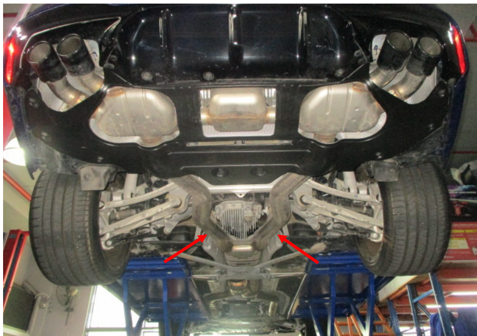
Photo 24 shows the rear section of the Motor Car's exhaust system. My examination of the Motor Car's exhaust system revealed no sign(s) or indication(s) of any cut or weld marks along its exhaust pipes (arrowed), on its rear mufflers, on its centre resonator boxes and on its catalytic converters.
