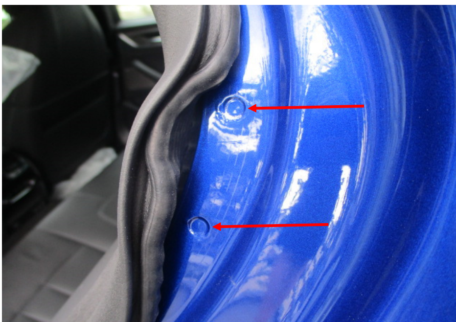
Photo 31 shows the left side "C" pillar of the Motor Car. I did not find any weld marks other than original spot weld marks (arrowed) on the left side "C" pillar of the Motor Car which, indicates that there was no re-welding works carried out. In general, I had found all the non-detachable body panels of the Motor Car to be originally fitted at the time of my inspection.
