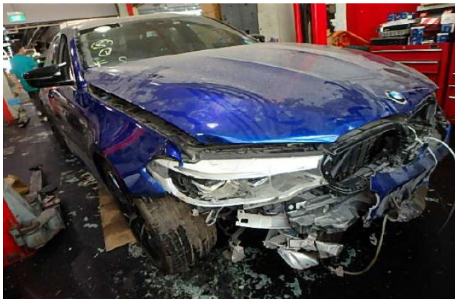
Photo 1 shows the front right body of the Motor Car (photograph provided to me). The photographs provided to me had showed damage to the frontal portion of the Motor Car. The front bumper, front bumper reinforcement, front bumper right lower grille, front bumper centre grille, radiator grilles, front bonnet, front right headlamp, front right fender, front right fender inner shield and front right radiator were amongst the body parts that were observed to have been damaged.
