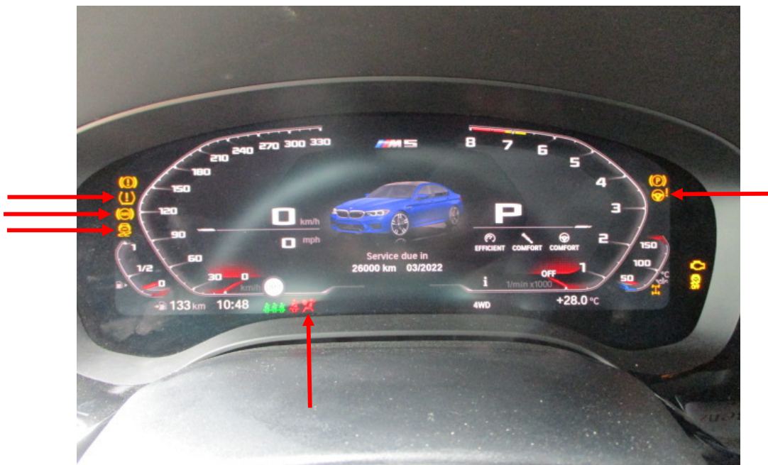
Photo 17 shows the warning lights for the various electronic safety features appearing on the instrument panel of the Motor Car during its self-test when the engine is cranked, in particular the ABS, SRS, IAS, TPM and DSC lights (arrowed).
