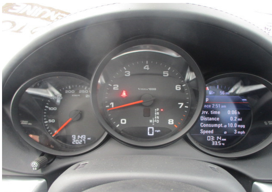
Photo 24 shows the respective warning lights no longer illuminated, indicating that there is no fault detected to ABS, SRS, TPM and TCS systems of the Motor Car during the self-test. These electronic systems were hence in working condition at the time of my inspection.
