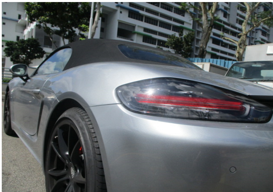
Photo 17 shows a closer view of the Motor Car's rear bumper, rear left taillamp and rear left fender at the time of my inspection. The body parts along the left side body of the Motor Car were visually examined and it was observed that the repair/restoration works carried out to the damaged area of the Motor Car (refer to photograph 5 – 7 above) were reasonably adequate and in order.
