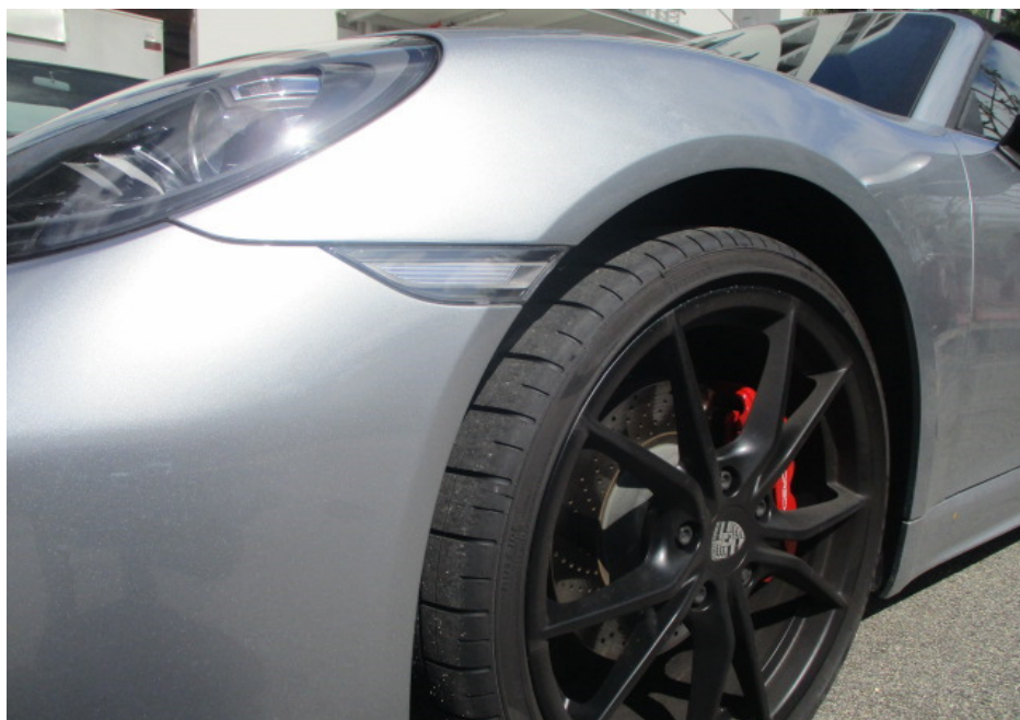
Photo 14 shows a closer view of the Motor Car's front bumper, front left signal lamp, front left fender and front left wheel rim at the time of my inspection. The body parts along the left side body of the Motor Car were visually examined and it was observed that the repair/restoration works carried out to the damaged area of the Motor Car (refer to photograph 5 – 7 above) were reasonably adequate and in order.
