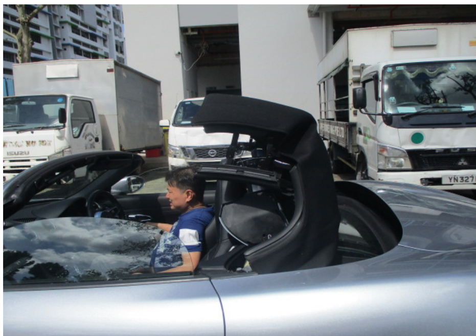
Photo 21 shows the Motor Car's soft top roof being tested. It was observed that as a safety feature, the soft top roof could only open and close when the Motor Car was in a stationary position. When opened, the soft top roof is completely folded into the rear compartment with no parts protruding out of the Motor Car's body. The soft top roof was also found adequately secured to the "A" pillar after closing.
