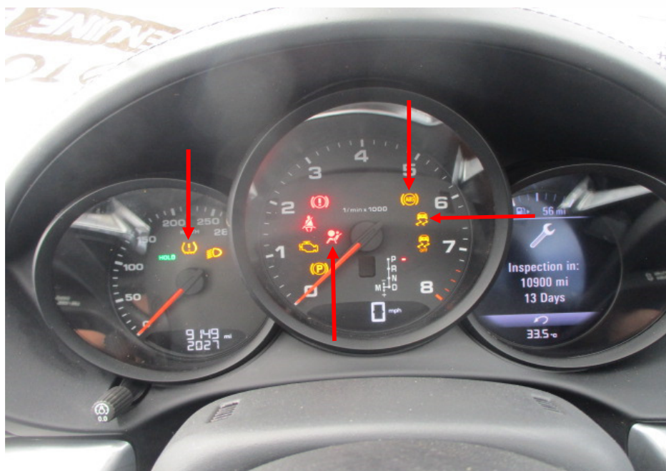
Photo 23 shows the warning lights for the various electronic safety features appearing on the instrument panel of the Motor Car during its self-test when the engine is cranked, in particular ABS, SRS, TPM and TCS lights (arrowed).
