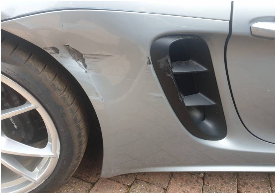
Photo 3 shows a closer view of the damaged right side rocker panel garnish and right side air vent of the Motor Car (photograph provided to me).
