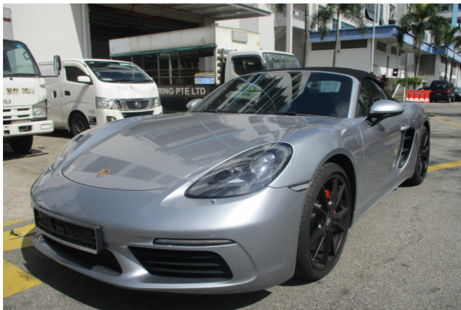
Photo 13 shows a general view of the front left body of the Motor Car at the time of my inspection. The Motor Car was observed to be in a relatively good general condition with no loose exterior fittings observed. The body parts along the left side body of the Motor Car were visually examined and it was observed that the repair/restoration works carried out to the damaged area of the Motor Car (refer to photograph 5 – 7 above) were reasonably adequate and in order.
