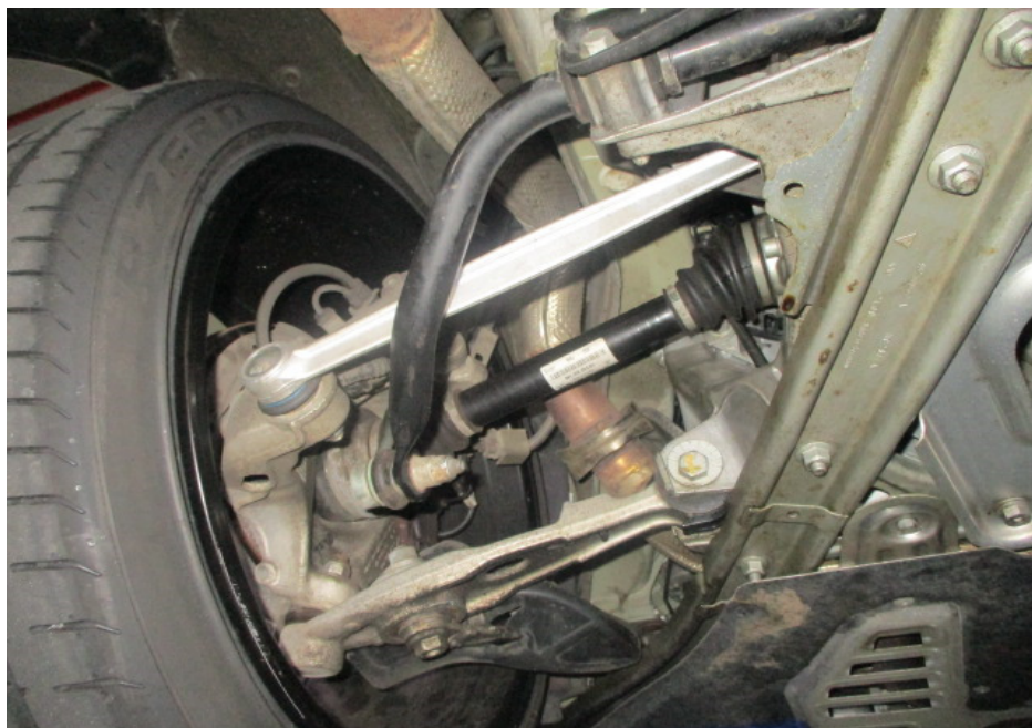
Photo 27 shows a general view of the control arms and linkages at the rear left wheel of the Motor Car. I did not observe any fluid leak and/or fluid stain on the underside of the Motor Car. All of the Motor Car's undercarriage components were observed to be intact and secured in an appropriate manner.
