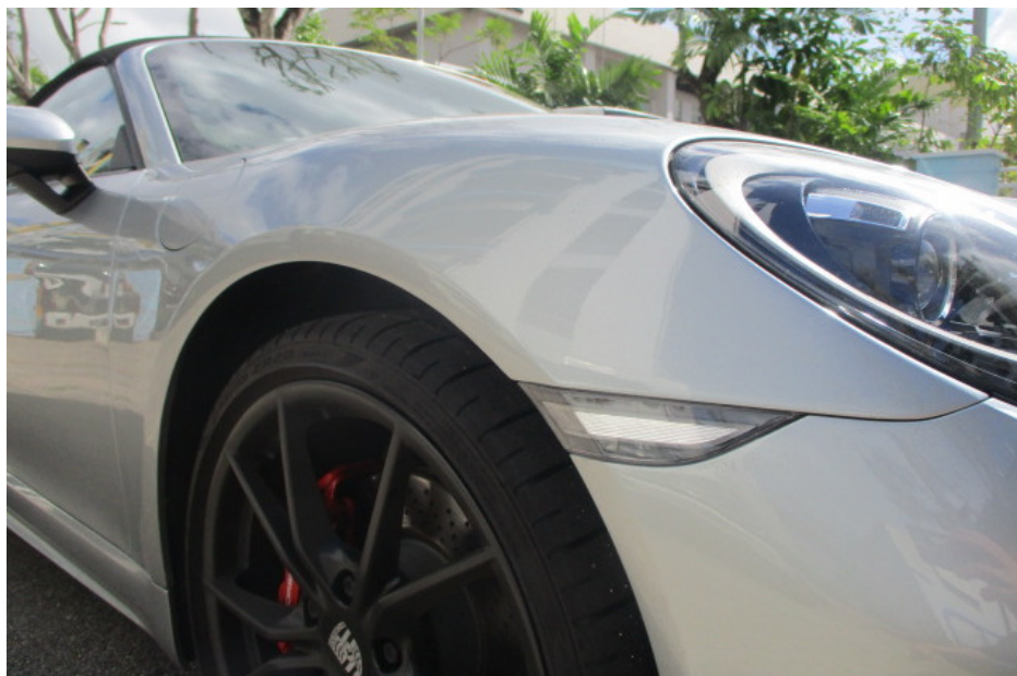
Photo 9 shows a closer view of the Motor Car's front bumper, front right signal lamp, front right fender and front right wheel rim at the time of my inspection. The body parts along the right side body of the Motor Car were visually examined and it was observed that the repair/restoration works carried out to the damaged area of the Motor Car (refer to photograph 1 – 4 above) were reasonably adequate and in order.
