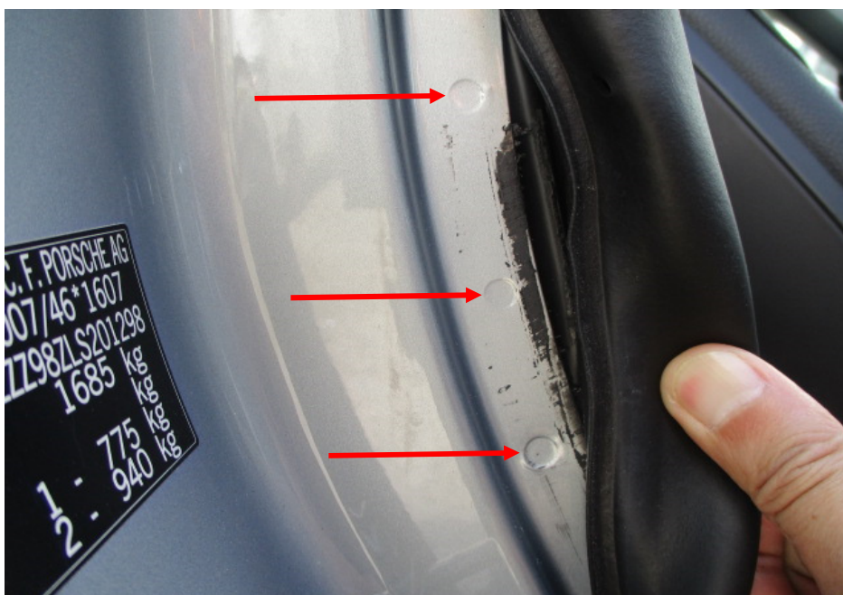
Photo 40 shows the rear right body panel of the Motor Car. I did not find any weld marks other than original spot weld marks (arrowed) on the rear right body panel of the Motor Car, which indicates that there was no re-welding works carried out. In general, I had found all the non-detachable body panels of the Motor Car to be originally fitted at the time of my inspection.
