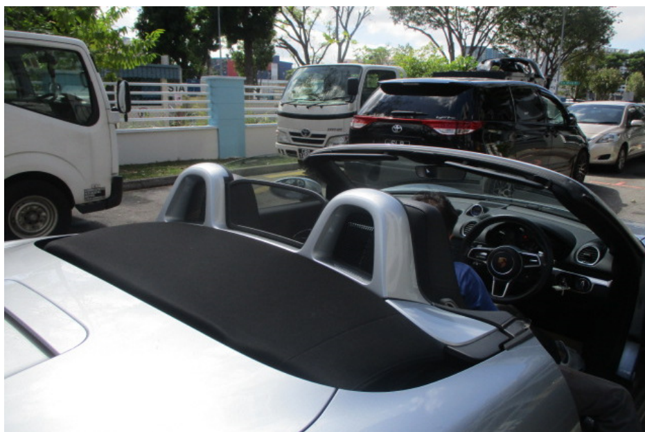
Photo 22 shows the Motor Car with its soft top roof completely folded. It was observed that as a safety feature, the soft top roof could only open and close when the Motor Car was in a stationary position. When opened, the soft top roof is completely folded into the rear compartment with no parts protruding out of the Motor Car's body. The soft top roof was also found adequately secured to the "A" pillar after closing.
