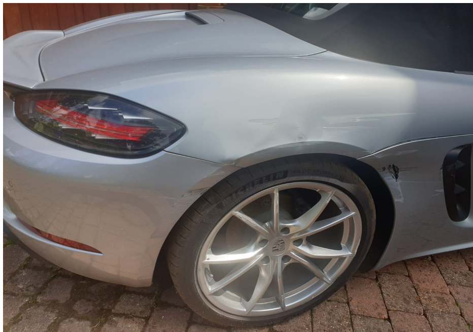
Photo 4 shows a closer view of the damaged right side rocker panel garnish, right side air vent, rear right fender, rear right wheel rim and rear bumper of the Motor Car (photograph provided to me).
