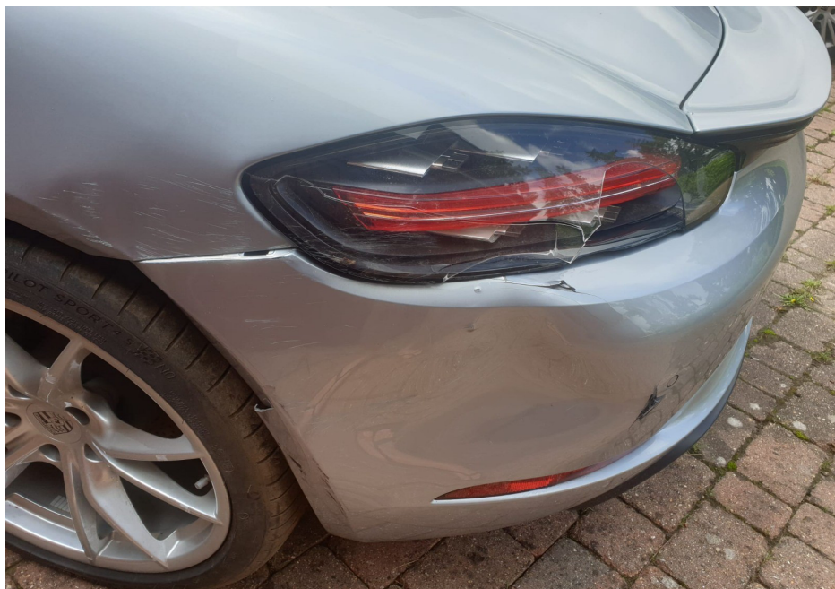
Photo 5 shows a closer view of the damaged rear bumper, rear left taillamp and rear left fender of the Motor Car (photograph provided to me). Apart for the right side body, the photographs provided had also showed relatively minor damage along the left side body of the Motor Car.
