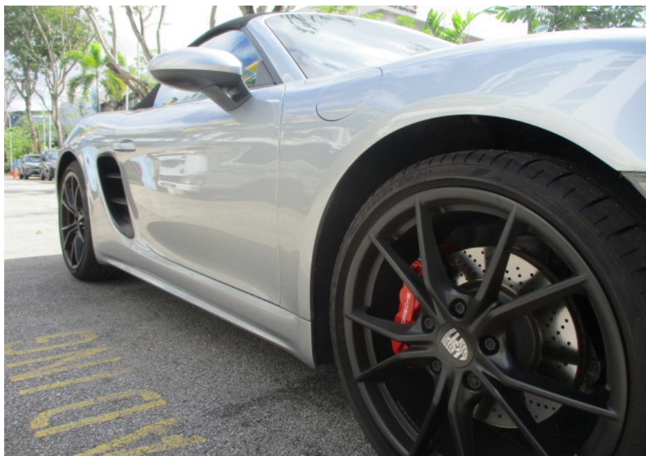
Photo 10 shows a closer view of the Motor Car's front right wheel rim, front right fender, front right door and right side rocker panel garnish at the time of my inspection. The body parts along the right side body of the Motor Car were visually examined and it was observed that the repair/restoration works carried out to the damaged area of the Motor Car (refer to photograph 1 – 4 above) were reasonably adequate and in order.
