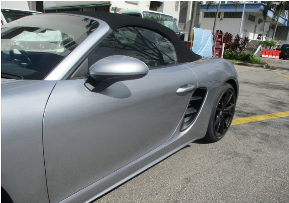
Photo 15 shows a closer view of the Motor Car's front left door and left side rocker panel garnish at the time of my inspection. The body parts along the left side body of the Motor Car were visually examined and it was observed that the repair/restoration works carried out to the damaged area of the Motor Car (refer to photograph 5 – 7 above) were reasonably adequate and in order.
