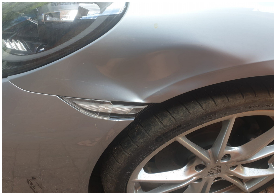
Photo 7 shows a closer view of the damaged front left fender, front left signal lamp and front bumper of the Motor Car (photograph provided to me). Apart for the right side body, the photographs provided had also showed relatively minor damage along the left side body of the Motor Car.
