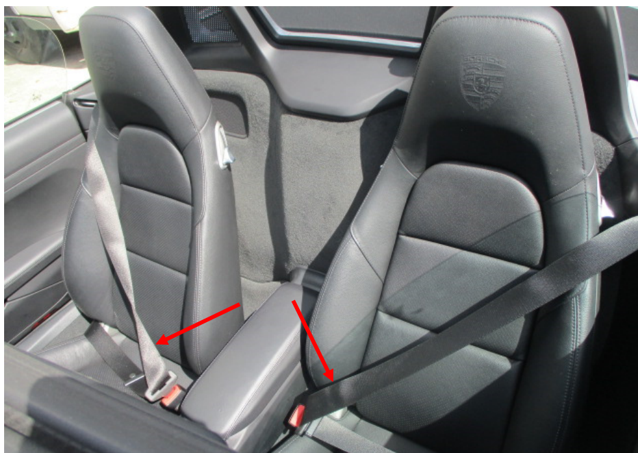
Photo 20 shows the seats of the Motor Car. All the seats of the Motor Car were secured via seat rails to the floorboard. They were also fitted with a retractable seat belt reel and a pre-tensioner. The seat belts (arrowed) were tested and were able to be fastened into the respective pre-tensions that were fitted on the side of each individual seat.
