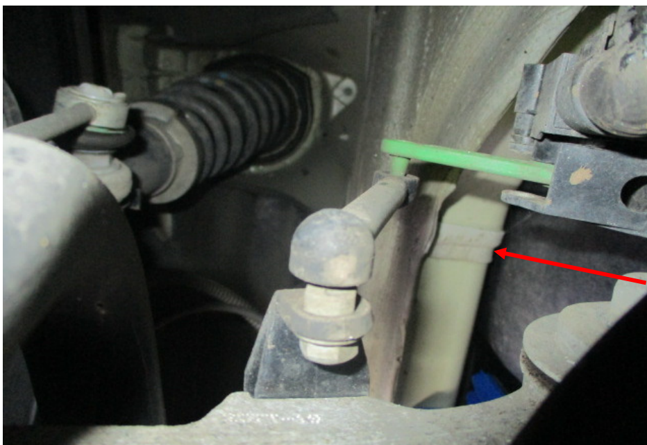
Photo 36 shows the chassis/structural body at the underside front left of the Motor Car. I did not find any weld marks other than original spot weld marks on the chassis/structural body of the Motor Car. The original factory sealant (arrowed) at the joints along the chassis/structural body was untouched, indicating no work was done on the chassis/structural body of the Motor Car and that the chassis/structural body was originally fitted.
