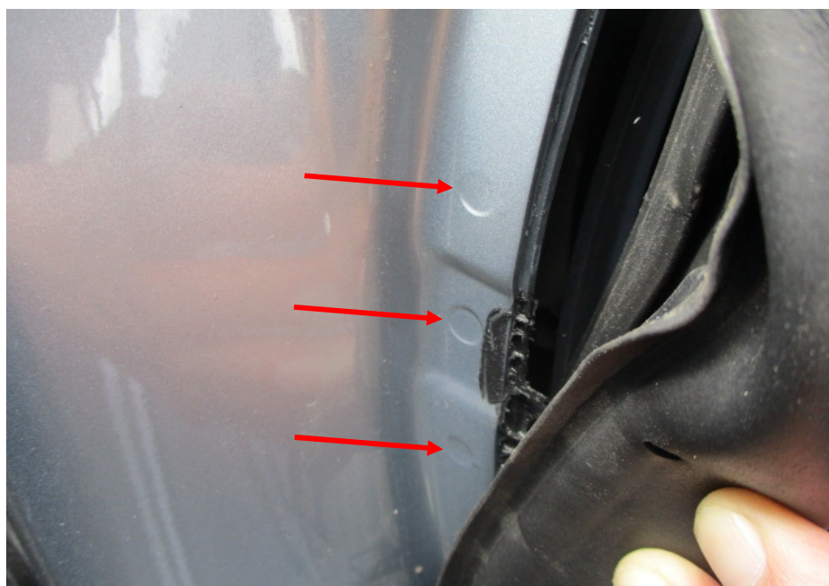
Photo 38 shows the left side "A" pillar of the Motor Car. I did not find any weld marks other than original spot weld marks (arrowed) on the left side "A" pillar of the Motor Car which, indicates that there was no re-welding works carried out. In general, I had found all the non-detachable body panels of the Motor Car to be originally fitted at the time of my inspection.
