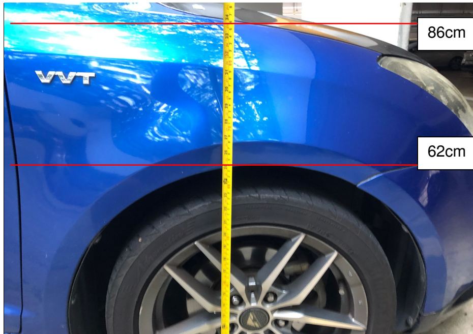
Photo 12 shows the height measurement being conducted on the right frontal portion of the Suzuki (using a similar make and model). The height range above ground level of the right front fender of the Suzuki, at the area where the damages were found, was measured to be approximately between 62cm to 86cm.
