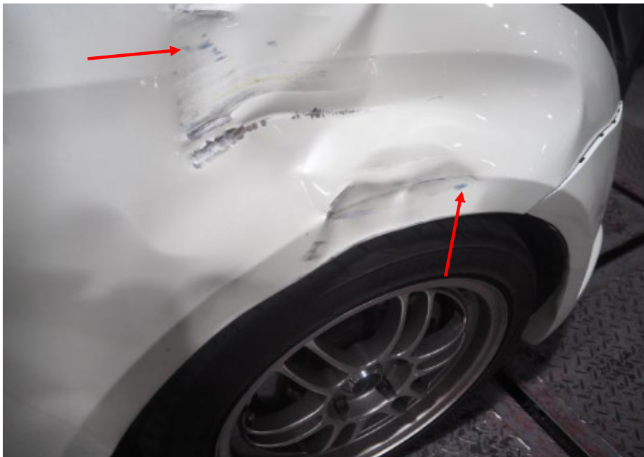
Photo 4 shows a closer view of the blue paint transfer marks found on the right front fender of the Suzuki (arrowed).
