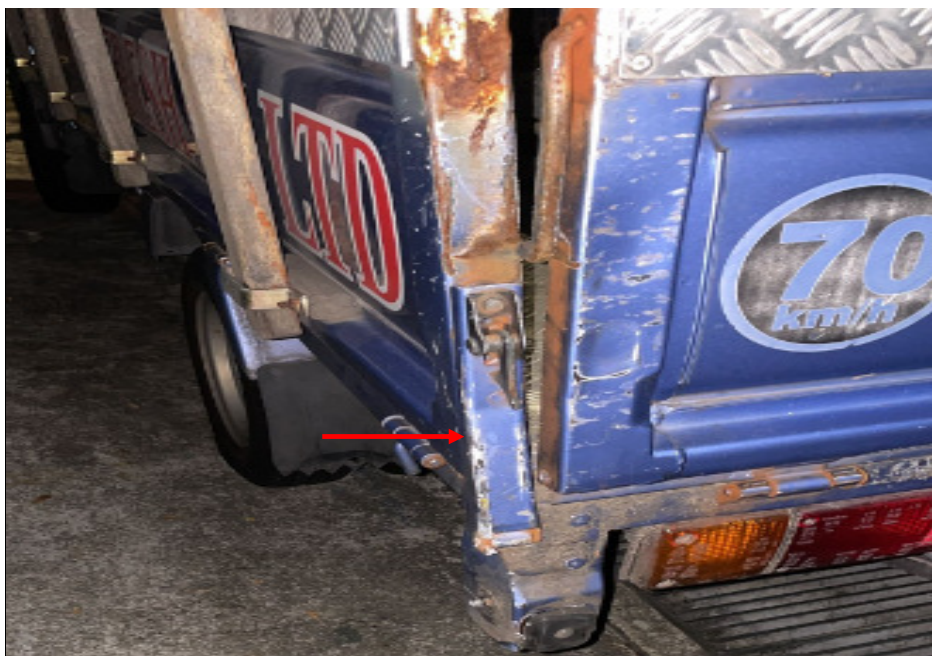
Photo 11 shows a close up view of the left rear portion of the Nissan at the accident location provided by Mr Tan. White paint transfer marks can be seen on the rear portion of the left side gate of the Nissan post- accident (arrowed).
