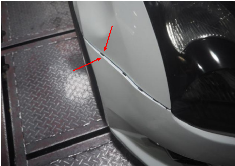
Photo 5 shows a closer view of the right corner edge of the front bumper of the Suzuki. We observed that the front bumper was misaligned at its corner edges (arrowed).
