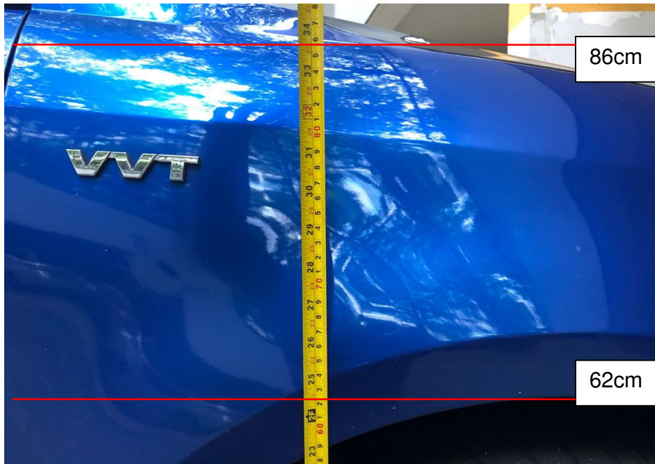
Photo 13 shows a closer view of the height measurement being conducted on the right frontal portion of the Suzuki (using a similar make and model). The height range above ground level of the right front fender of the Suzuki, at the area where the damages were found, was measured to be approximately between 62cm to 86cm.
