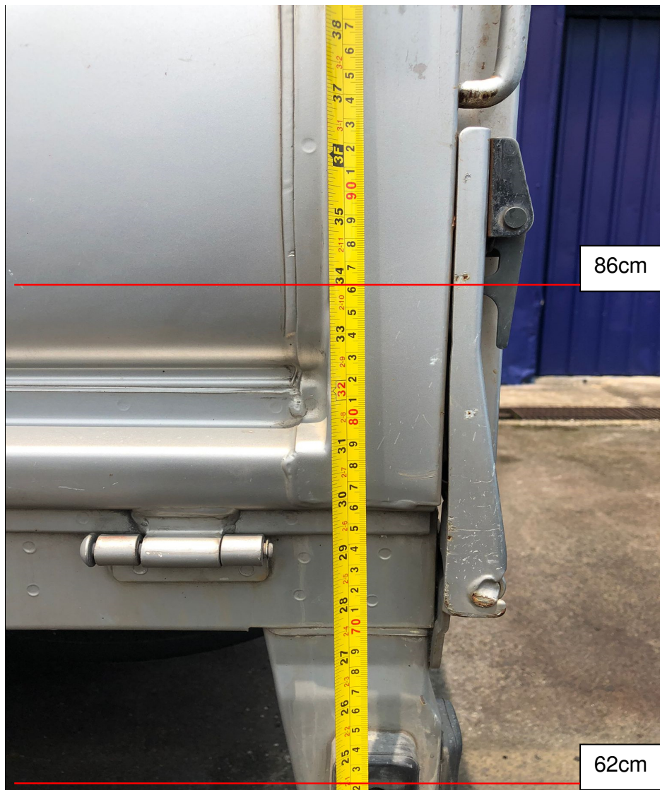
Photo 15 shows a closer view of the height measurement being conducted on the left rear portion of the Nissan (using a similar make and model). The body part at the height range of between 62cm to 86cm above ground level was the rear portion of the left side gate of the Nissan where the white paint transfer marks were observed.
