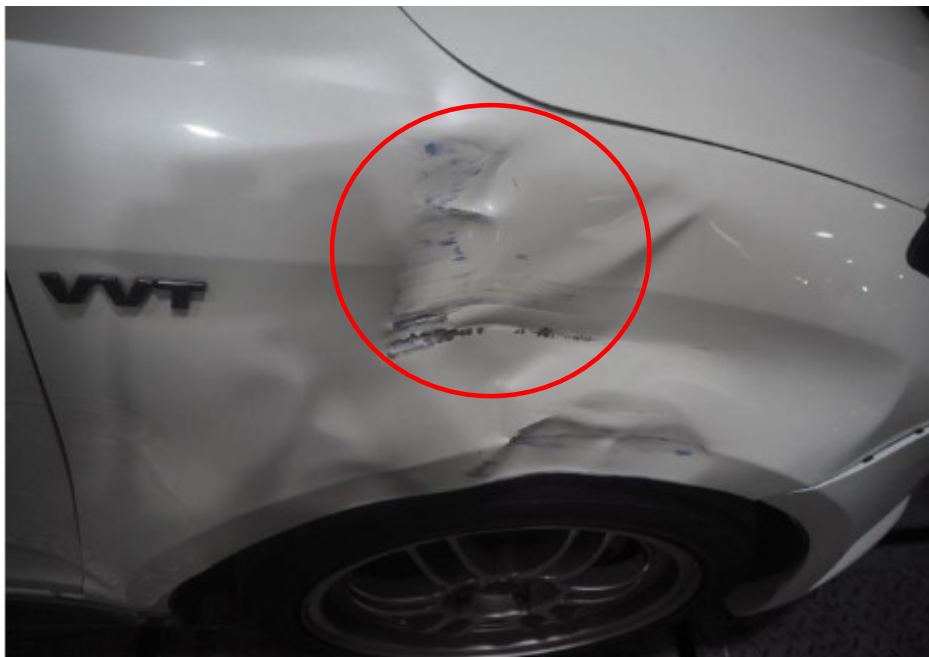
Photo 3 shows a closer view of the dents (circled) found on the right front fender of the Suzuki.
