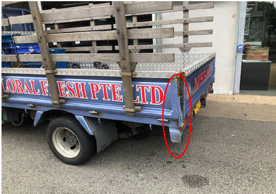
Photo 7 shows the white paint transfer marks found on the rear portion of the Nissan's left side gate (circled).
