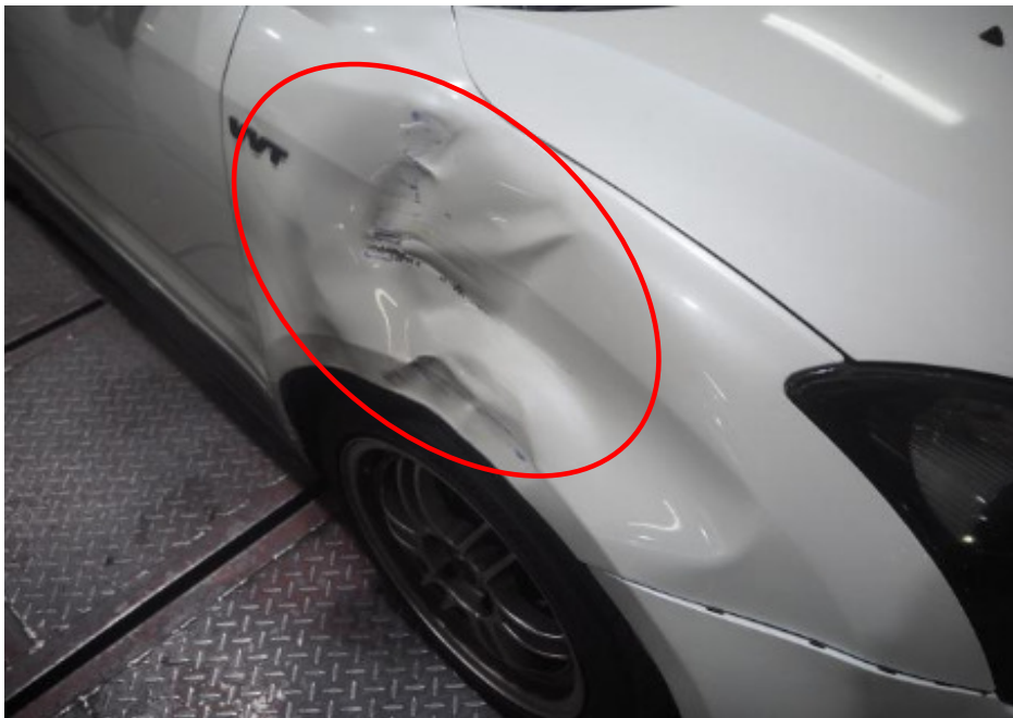
Photo 2 shows the dents (circled) found on the right front fender of the Suzuki.
