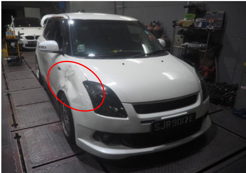
Photo 1 shows the general view of the frontal portion of the Suzuki at the time of the Pre- Repair Survey conducted by LKK Auto Consultants Pte. Ltd. which was taken about 2 weeks after the accident. The damage to the Suzuki was observed to be confined to the right front fender and front bumper (circled).
