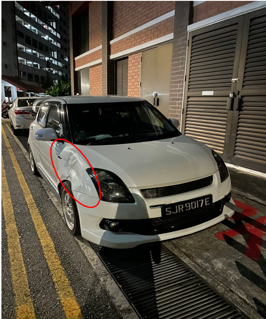
Photo 8 shows the position of the Suzuki at the accident location provided by Mr Tan. The Suzuki had sustained damages at the right front fender as a result of the accident (circled).
