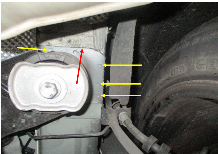
Photo 26 shows the chassis/structural body at the underside rear right of the Motor Car. I did not find any weld marks other than original spot weld marks (yellow arrow) on the chassis/structural body of the Motor Car. The original factory sealant (red arrow) at the joints along the chassis/structural body was untouched, indicating no work was done on the chassis/structural body of the Motor Car and that the chassis/structural body was originally fitted.
