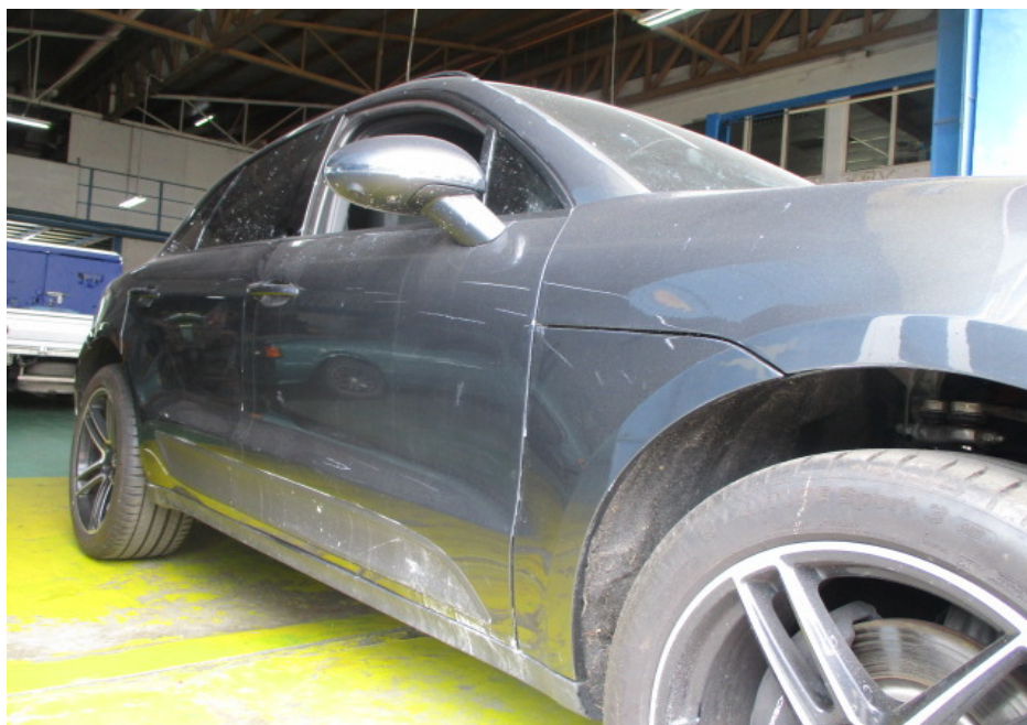
Photo 9 shows a closer view of the Motor Car's front bonnet, front right fender, front right door and right side rocker panel garnish at the time of my inspection. The body parts at the front right portion of the Motor Car were visually examined and it was observed that the repair/restoration works carried out to the damaged area of the Motor Car (refer to photograph 1 above) were reasonably adequate and in order.
