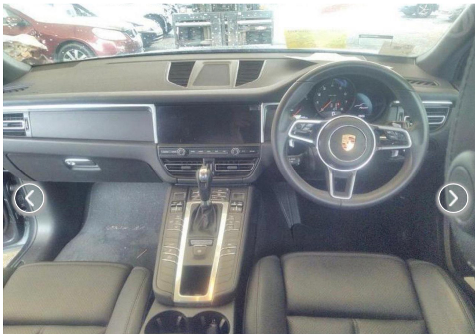
Photo 5 shows the front dashboard of the Motor Car (photograph provided to me). Parts and components within the interior compartment were observed to be intact and unaffected. The airbags of the Motor Car were also not deployed as seen from the photographs that were provided to me.
