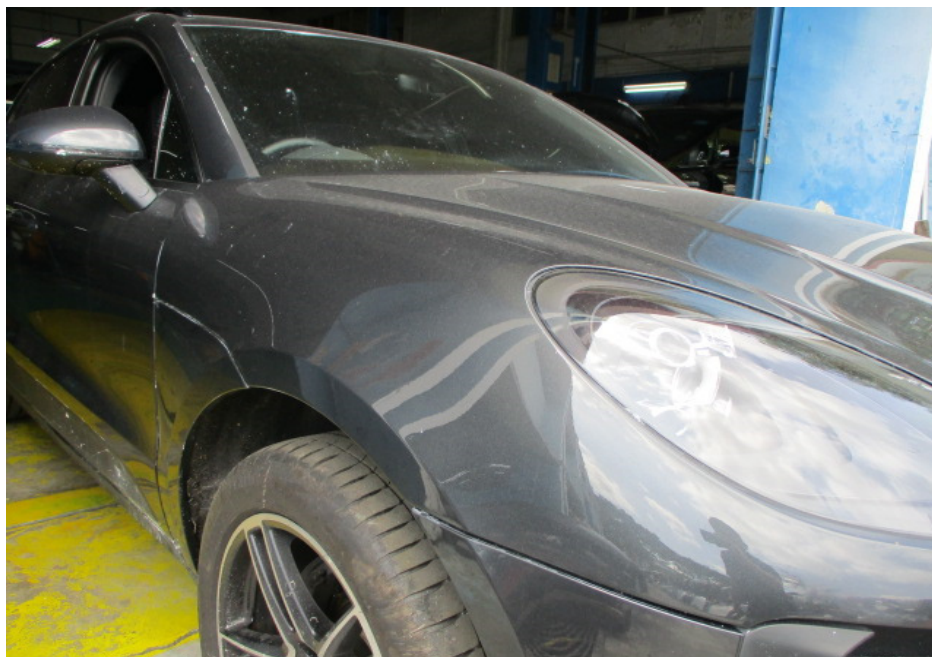
Photo 8 shows a closer view of the Motor Car's front right headlamp, front right fender and front bonnet at the time of my inspection. The body parts at the front right portion of the Motor Car were visually examined and it was observed that the repair/restoration works carried out to the damaged area of the Motor Car (refer to photograph 1 above) were reasonably adequate and in order.
