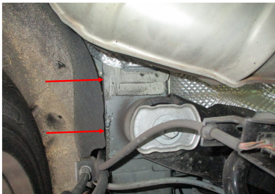
Photo 27 shows the chassis/structural body at the underside rear left of the Motor Car. The original factory sealant (arrowed) at the joints along the chassis/structural body was observed to be untouched. In general, I had found no work was carried out on the chassis/structural body of the Motor Car. The chassis/structural body of the Motor Car was originally fitted.
