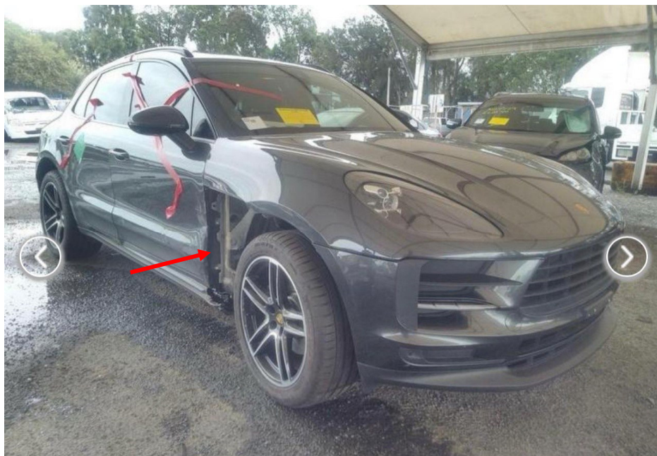
Photo 1 shows the front right body of the Motor Car (photograph provided to me). The photographs provided to me had showed the front right fender of the Motor Car dislodged/missing/damaged (arrowed). Apart for this, there was no physical damage observed to other areas of the Motor Car.
