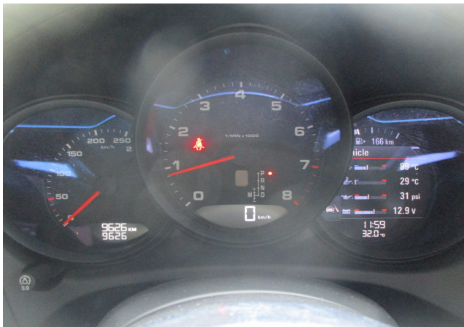
Photo 18 shows the respective warning lights no longer illuminated, indicating that there is no fault detected to the ABS, SRS, TPM and TCS systems of the Motor Car during the self-test. These electronic systems were hence in working condition at the time of my inspection.
