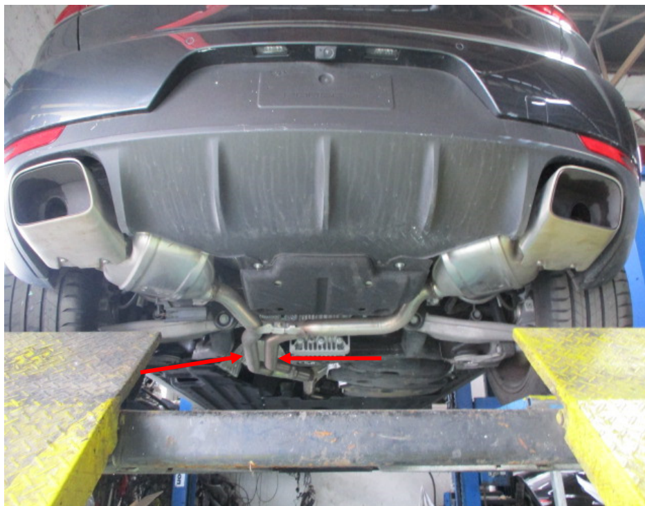
Photo 24 shows the rear section of the Motor Car's exhaust system. My examination of the Motor Car's exhaust system revealed no sign(s) or indication(s) of any cut or weld marks along its exhaust pipes (arrowed), on its rear mufflers and on its catalytic converter.
