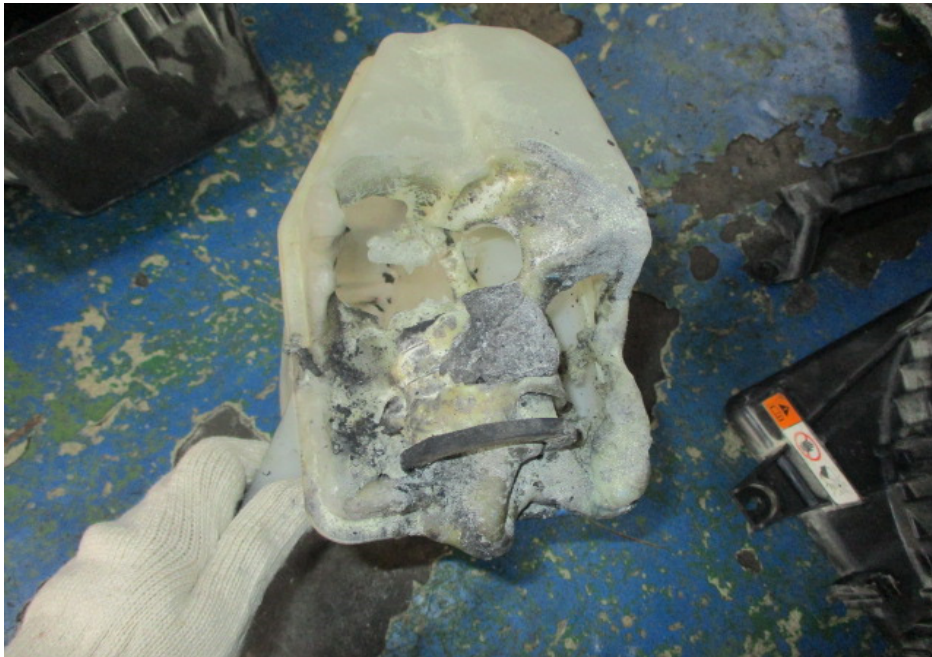
Photo 6 shows the partially melted wiper washer tank of the vehicle.
