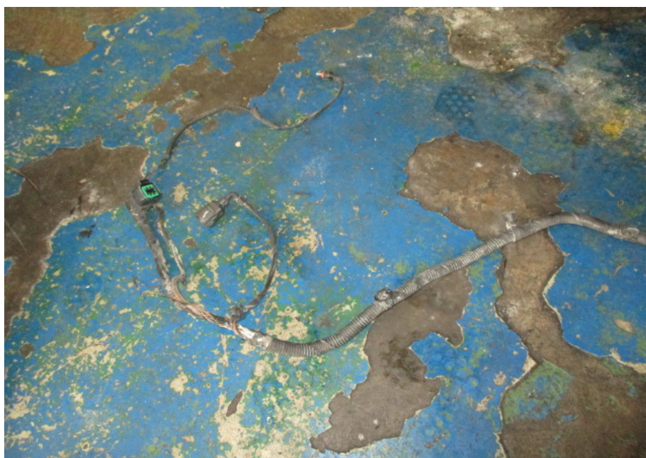
Photo 9 shows a general of the vehicle's front wire harness, which was found to be burnt.
