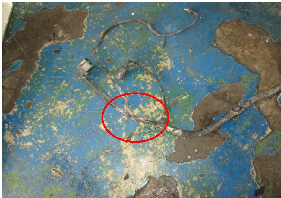
Photo 18 shows a general view of the burnt wirings (circled) from the front wire harness of the vehicle. Upon closer examination, I had found greenish residue on a stretch of burnt wirings. The presence of greenish residue indicates internal heating of copper wires, a sign of an electrical abnormality occurring. Such greenish residue is normally left behind from oxidation as result of chemical reaction involving copper wires, heat and oxygen.
