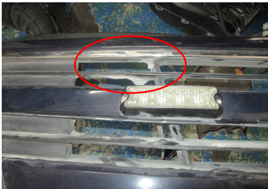
Photo 3 shows a closer view of the minor melting (circled) of the vehicle's radiator grille. Apart for this minor melting of the radiator grille, I did not observe any damage of fire nature to the exterior body of the vehicle.
