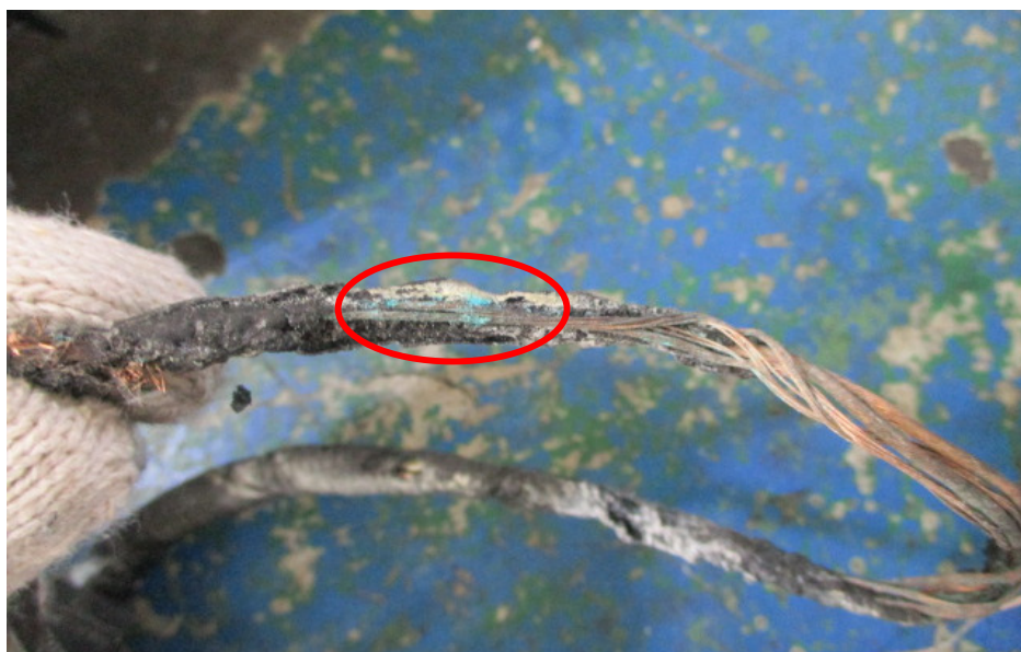
Photo 19 shows a closer view of the greenish residue (circled) that was found on a stretch of burnt wirings from the front wire harness of the vehicle. The presence of greenish residue indicates internal heating of copper wires, a sign of an electrical abnormality occurring. Such greenish residue is normally left behind from oxidation as result of chemical reaction involving copper wires, heat and oxygen. This stretch of burnt wirings is located at the middle section area of the vehicle's front support panel (refer to photograph 22 & 23 below).
