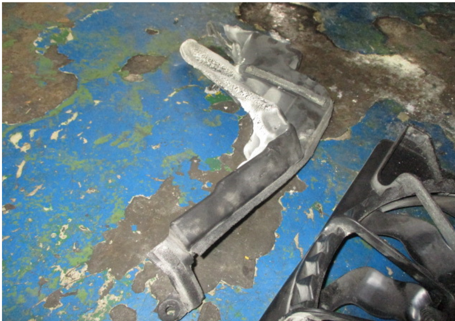
Photo 7 shows the partially melted air intake shield of the vehicle.
