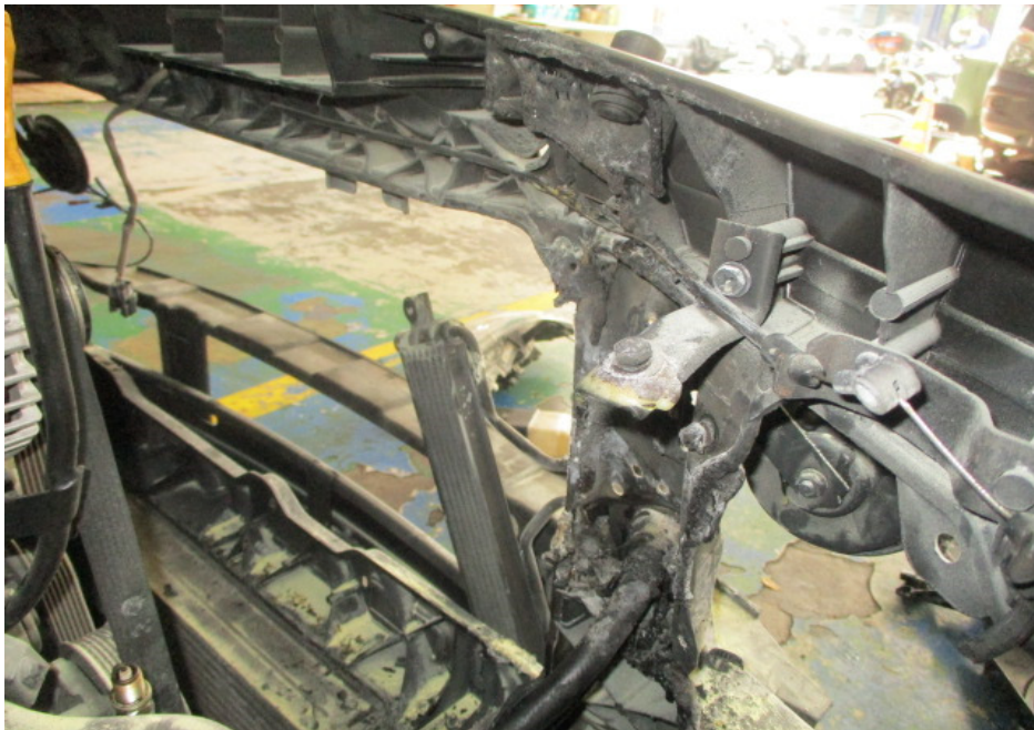
Photo 13 shows the area behind the burnt front support panel, at the right side of the vehicle. Parts surrounding this area were removed prior to my inspection. Some of these parts like the air duct, aircon condenser and radiator were burnt and/or had sustained heat/smoke damage. Refer to photograph 5 & 8 above.
