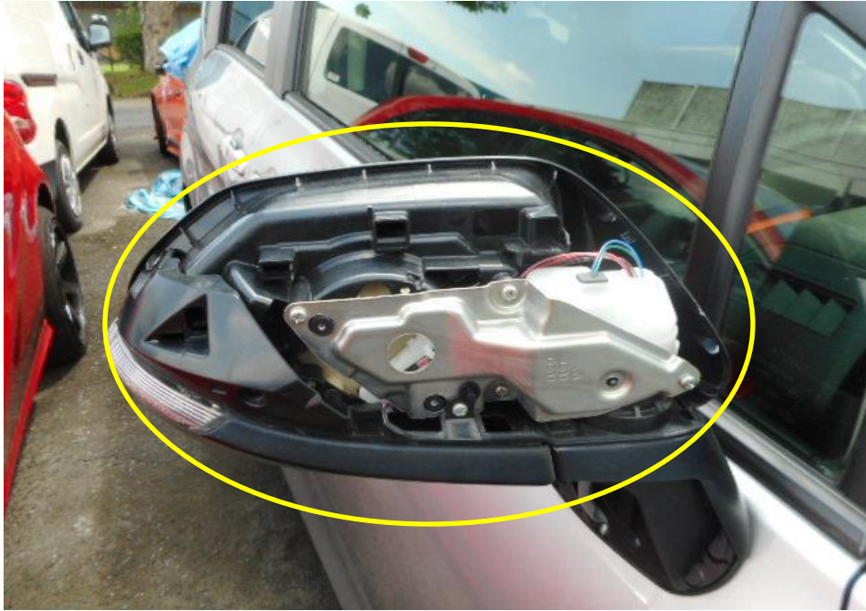
Photo 6 shows a close up view of the Motor Car's front body at the time of my inspection. The front portion of the Motor Car was observed to have sustained damage. Its front right side view mirror (circled) was the body parts that were damaged as a result of the accident.
