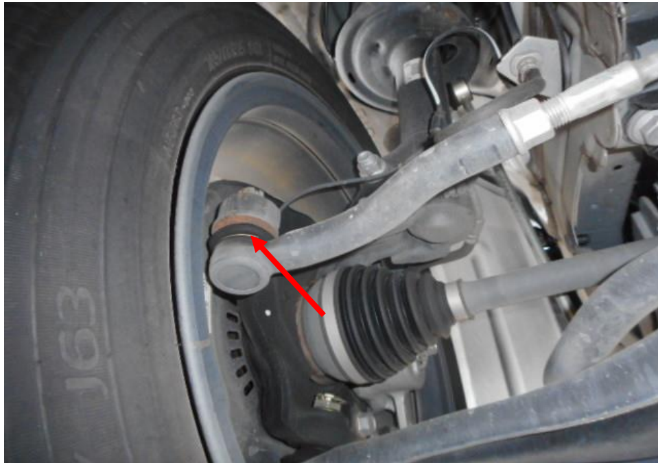
Photo 24 shows the various undercarriage components at the front left wheel of the Motor Car, which had included the steering tie rod (red arrow). The various undercarriage components of the Motor Car were all found to be intact without any visible damage.
