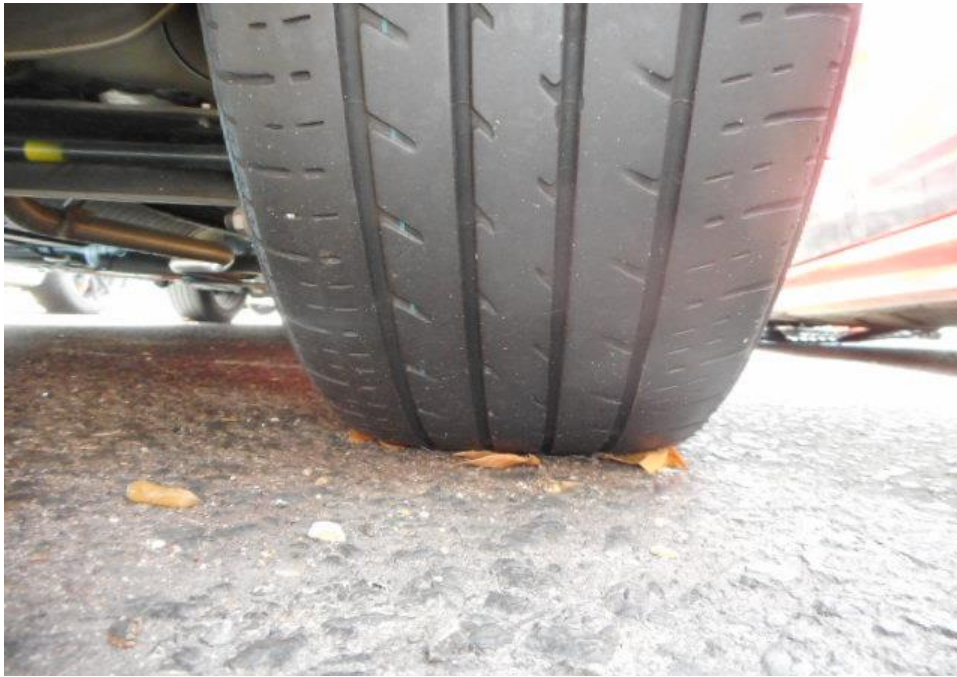
Photo 10 shows the condition of the rear right tyre of the Motor Car, which was observed to be in serviceable condition with remaining tread depth of approximately 3.8mm. The tyre was also observed to be sufficiently inflated for vehicular operation with no tear, cut or burst mark(s).
