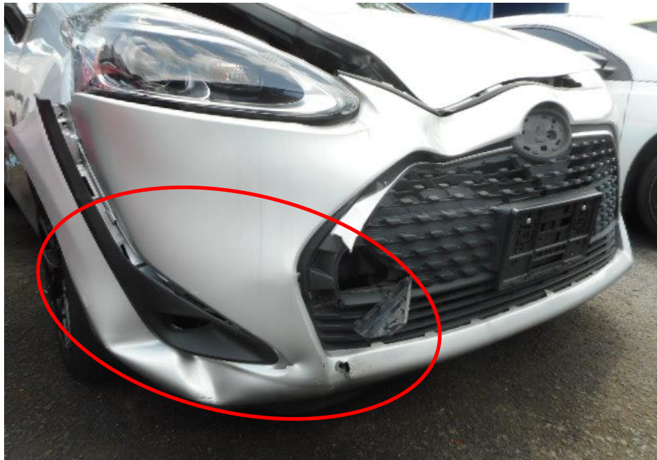
Photo 5 shows a close up view of the Motor Car's front body at the time of my inspection. The front portion of the Motor Car was observed to have sustained damage. Its front bumper (circled) was the body parts that were damaged as a result of the accident.
