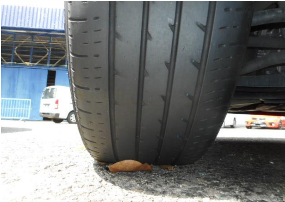
Photo 12 shows the condition of the front left tyre of the Motor Car, which was observed to be in serviceable condition with remaining tread depth of approximately 3.2mm. There was also no tear, cut or burst mark(s) on the outer and the inner sidewalls as well as across the tread of the Motor Car's 4 tyres.
