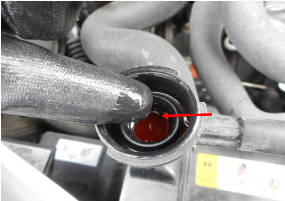
Photo 15 shows checks being carried out to the engine coolant of the Motor Car at the time of my inspection. The engine coolant was observed to be of sufficient level (arrowed) and without any visible contamination.
