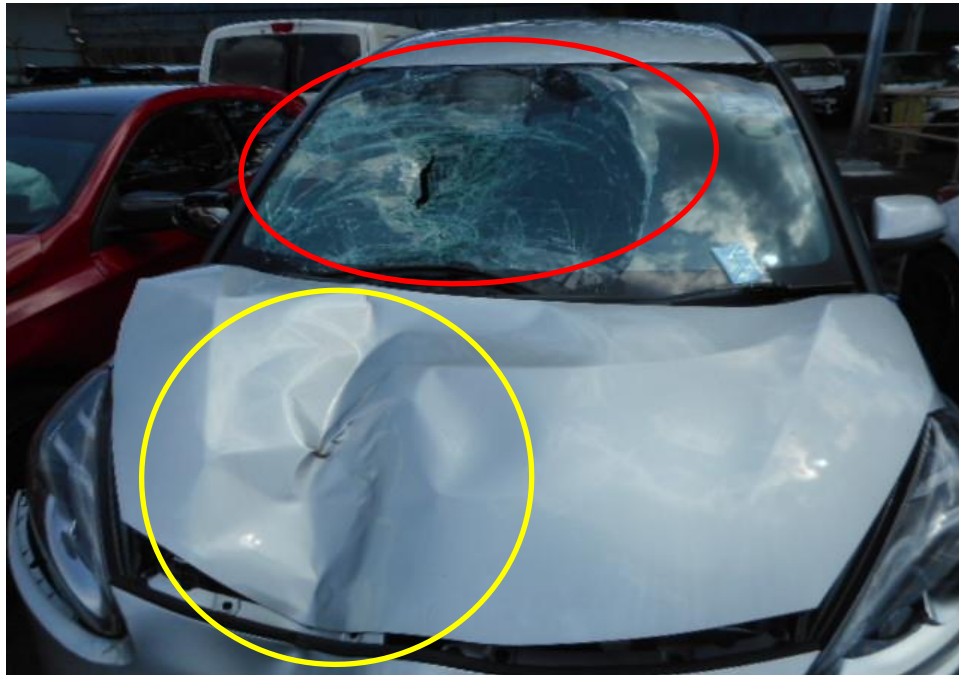
Photo 4 shows a close up view of the Motor Car's front body at the time of my inspection. The front portion of the Motor Car was observed to have sustained damage. Its front windscreen (red circle) and front bumper (yellow circle) was the body parts that were damaged as a result of the accident.
