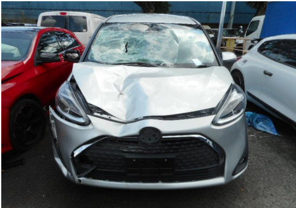
Photo 3 shows a general view of the Motor Car's front body at the time of my inspection. The front portion of the Motor Car was observed to have sustained damage. Its front windscreen, front bonnet, front bumper and front right side view mirror was amongst the body parts that were damaged as a result of the accident.
