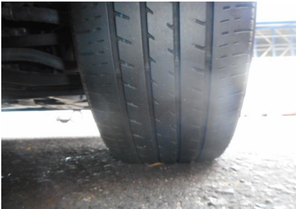
Photo 9 shows the condition of the front right tyre of the Motor Car, which was observed to be in serviceable condition with remaining tread depth of approximately 4mm. The tyre was sufficiently inflated for vehicular operation with no tear, cut or burst mark(s) on the outer and the inner sidewalls as well as across the tread. The 4 tyres of the Motor Car were wrapped around standard steel wheel rims without any damage.
