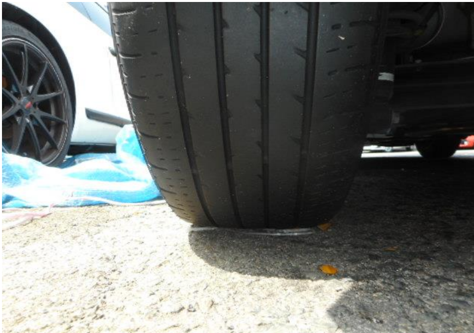
Photo 11 shows the condition of the rear left tyre of the Motor Car, which was observed to be in serviceable condition with remaining tread depth of approximately 3.2mm. The tyre, which was wrapped around steel wheel rim, was also observed to be sufficiently inflated for vehicular operation. The 4 tyres of the Motor Car were wrapped around standard steel wheel rims.
