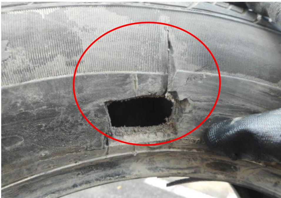
Photo 13 shows close up view and the condition of the rear left tyre of the Motor Car, which was observed to be in unserviceable condition with remaining tread depth of approximately 6mm. The tyre was cut and deflated (circled) as a result of the accident.
