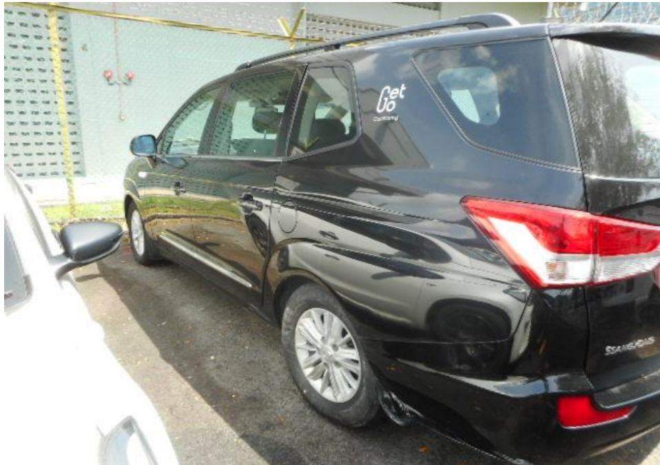
Photo 2 shows a general view of the Motor Car's left body at the time of my inspection. The Motor Car was observed to have sustained damage at its left and rear portion. Its left side skirt and its rear bumper were amongst the body parts that were damaged as a result of the accident.
