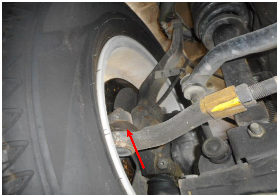
Photo 27 shows the various undercarriage components at the front left wheel of the Motor Car, which had included the steering tie rod (arrowed). The various undercarriage components of the Motor Car were all found to be intact without any visible damage.
