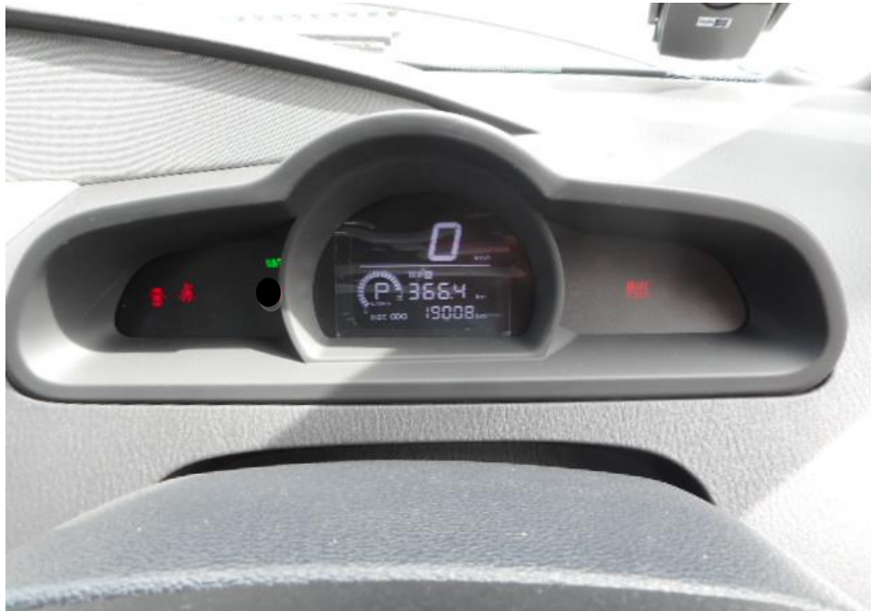
Photo 30 shows no warning lights illuminated on the instrument panel of the Motor Car after the engine was cranked. This would suggest that there was no abnormality to the electronic operating system of the Motor Car, like the ABS and SRS etc.
