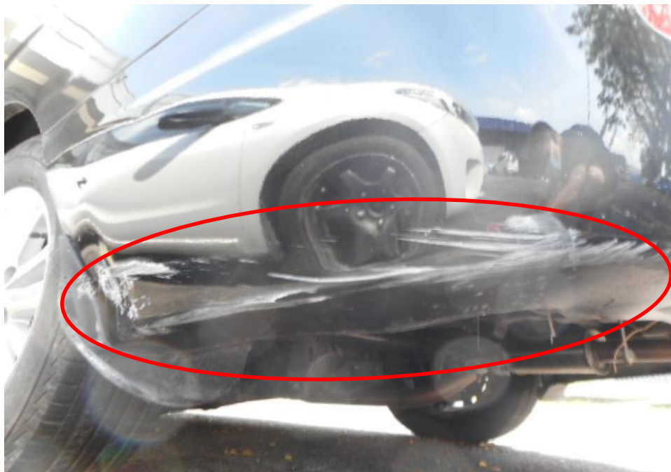
Photo 5 shows a close up view of the Motor Car's rear body at the time of my inspection. The Motor Car was observed to have sustained damage at its left and rear portion. Its rear bumper (circled) were amongst the body parts that were damaged as a result of the accident.
