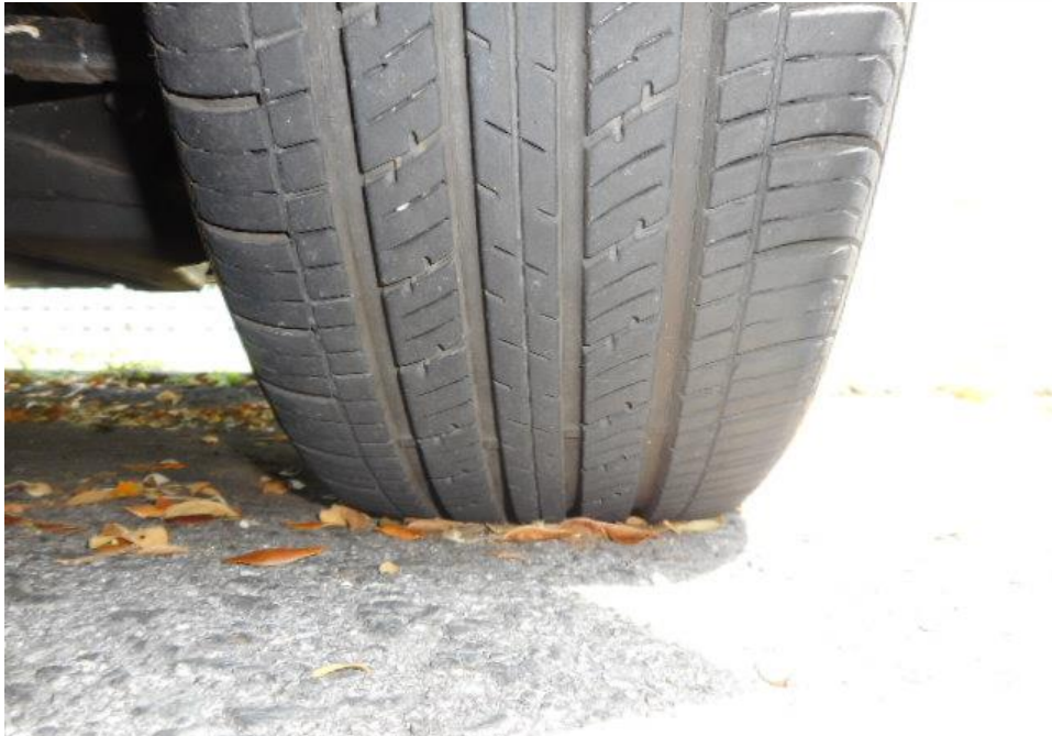
Photo 8 shows the condition of the front right tyre of the Motor Car, which was observed to be in serviceable condition with remaining tread depth of approximately 6.7mm. The tyre was sufficiently inflated for vehicular operation with no tear, cut or burst mark(s) on the outer and the inner sidewalls as well as across the tread. The 2 tyres of the Motor Car were wrapped around standard steel wheel rims without any damage.
