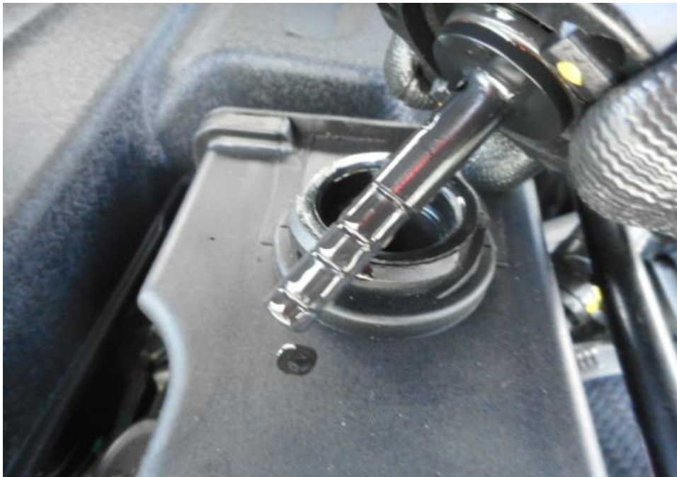
Photo 18 shows the power steering fluid dipstick of the Motor Car at the time of my inspection. The steering fluid was observed to be of sufficient level and without any visible contamination.
