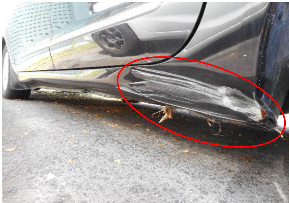
Photo 3 shows a close up view of the Motor Car's left body at the time of my inspection. The Motor Car was observed to have sustained damage at its left and rear portion. Its left side skirt (circled) were amongst the body parts that were damaged as a result of the accident.
