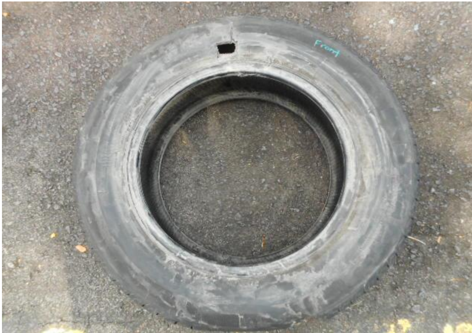
Photo 12 shows the general view and the condition of the front left tyre of the Motor Car, which was observed to be in serviceable condition with remaining tread depth of approximately 6mm. There was also no tear, cut or burst mark(s) on the outer and the inner sidewalls as well as across the tread of the Motor Car's 4 tyres.
