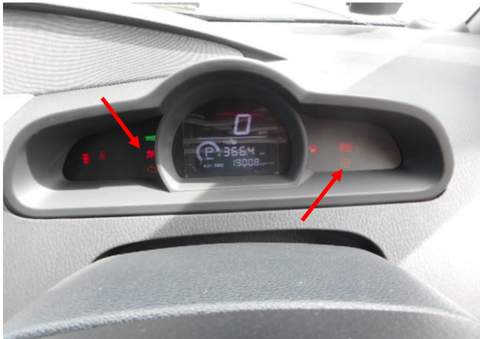
Photo 29 shows the warning light for Anti-Lock Brake System (ABS and Supplemental Restraint System (SRS) (arrowed) appearing on the instrument panel of the Motor Car during the self-test of its various electronic operating systems when its engine was cranked.
