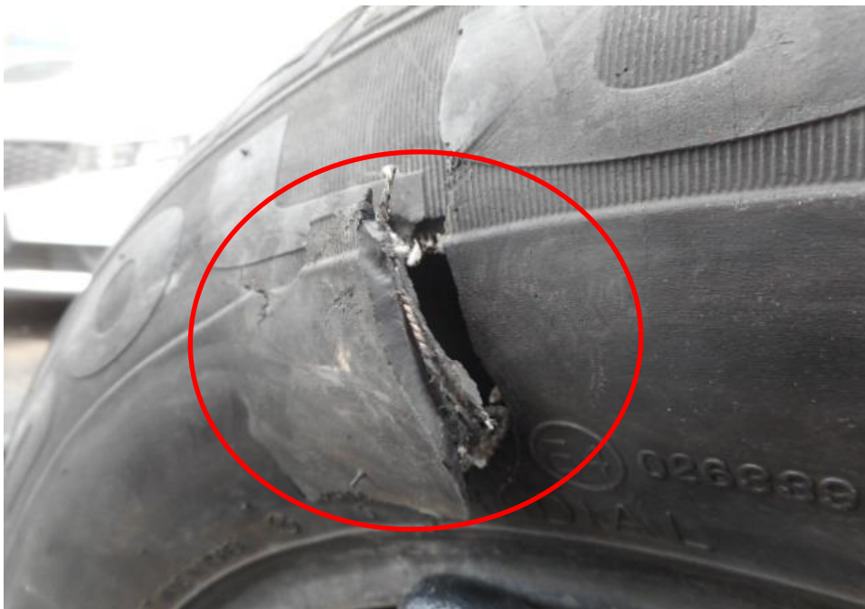
Photo 11 shows close up view and the condition of the rear left tyre of the Motor Car, which was observed to be in unserviceable condition with remaining tread depth of approximately 5.9mm. The tyre was cut and deflated (circled) as a result of the accident.
