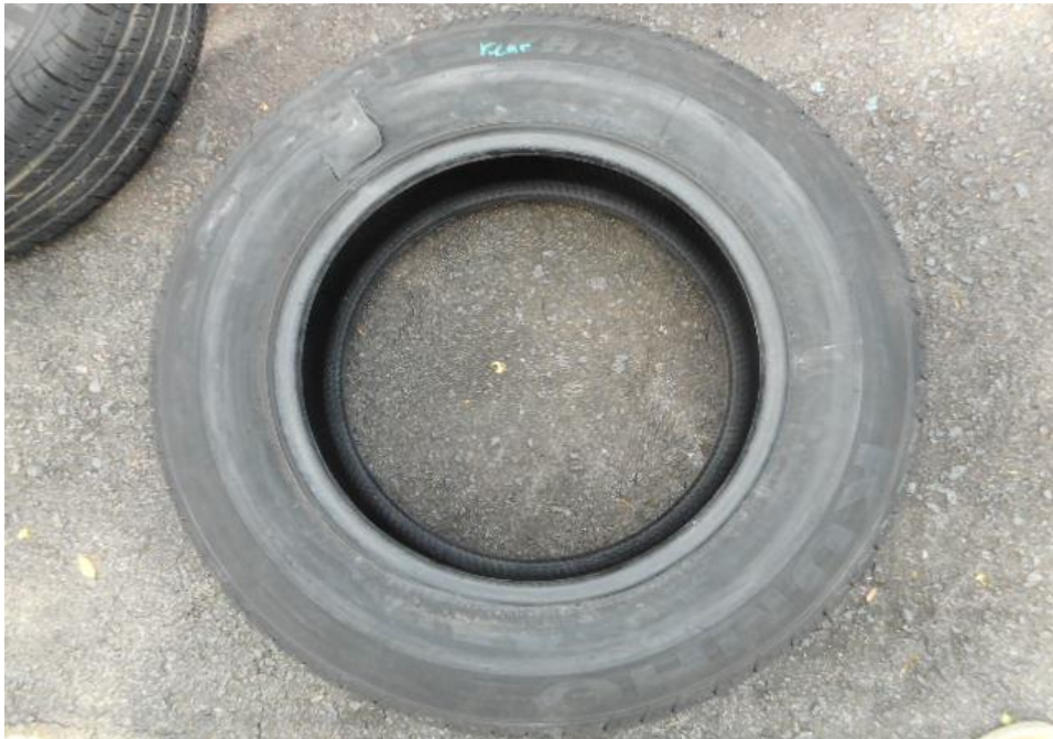
Photo 10 shows the general view and the condition of the rear left tyre of the Motor Car, which was observed to be in unserviceable condition with remaining tread depth of approximately 5.9mm. The tyre, was cut and deflated as a result of the accident.
