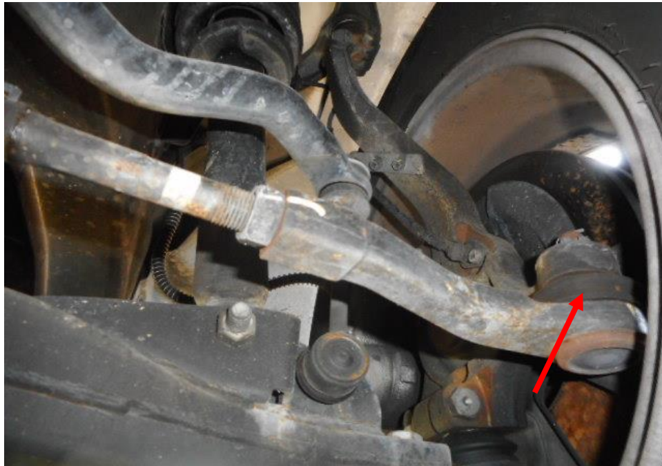
Photo 26 shows the various undercarriage components at the front right wheel of the Motor Car, in particular the steering tie rod (arrowed). The various steering components were all found to be intact, suggesting that the steering system of the Motor Car was likely to be in serviceable condition at the material time of accident. There was also no sign of fluid stain observed on the various undercarriage components at the front right wheel of the Motor Car.
