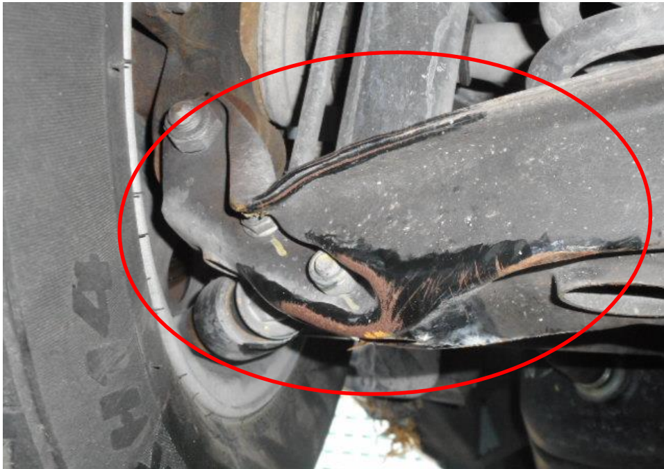
Photo 22 shows the lower arm (circled) at the rear left wheel of the Motor Car. It was observed to sustained damages as a result of the accident at the time of my inspection.
