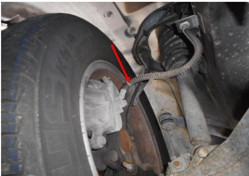
Photo 23 shows the brake hose/pipe (arrowed) at the front right wheel of the Motor Car. I did not observe any leakage of brake fluid at the time of my inspection of the Motor Car. Static tests of the Motor Car's braking system had indicated that there was no internal leakage of pressure/vacuum. The undercarriage components of the Motor Car were also all found to be intact and without any visible damage.
