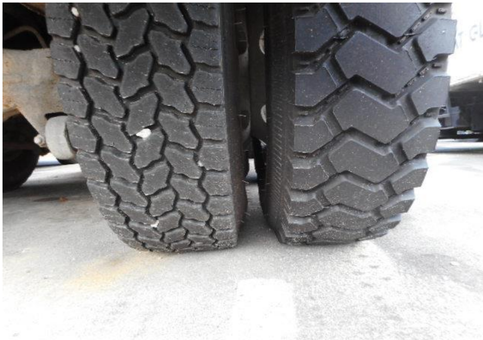
Photo 9 shows the condition of the rear right tyre of the Motor Tipper, which was observed to be in serviceable condition with remaining tread depth of approximately 14.3mm. The tyre, which was wrapped around standard steel wheel rim, was also observed to be sufficiently inflated for vehicular operation.
