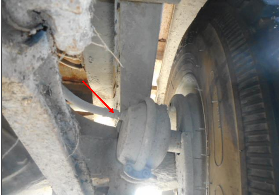
Photo 20 shows the brake pipe (arrowed) at the rear left wheel of the Motor Tipper. I did not observe any leakage of brake fluid at the time of my inspection of the Motor Tipper. My static tests of the Motor Tipper's braking system, along with my visual examination of the various mechanical components in the braking system, had indicated that there was no internal leakage of pressure/vacuum and these components were generally in good condition.
