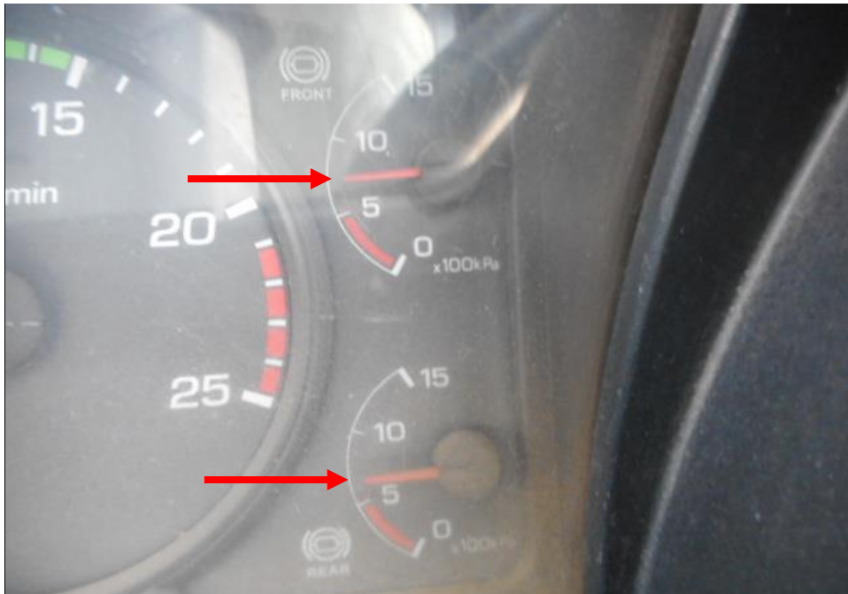
Photo 14 shows the air in the air brake cylinders of the Prime Mover at the time of my inspection. The air in the cylinder was observed to be of sufficient level & serviceable at the time of the accident.
