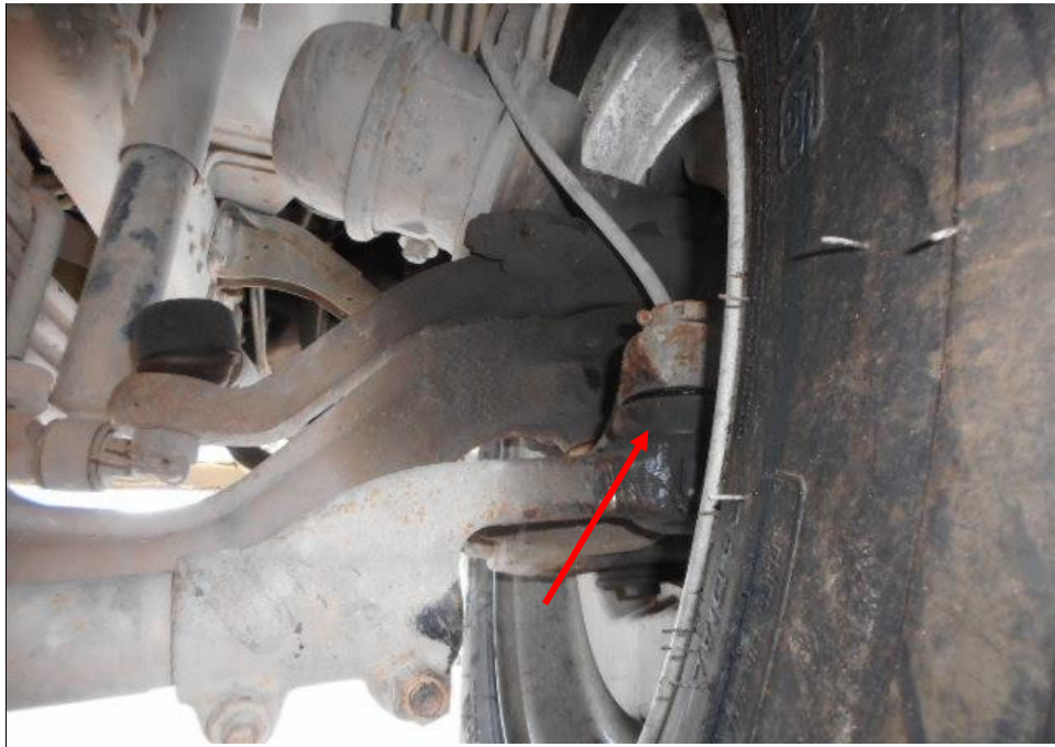
Photo 24 shows the various undercarriage components at the front right wheel of the Motor Tipper, in particular the steering tie rod end (arrowed) were found to be intact, there was also no sign of fluid stain(s) observed on the various undercarriage components.
