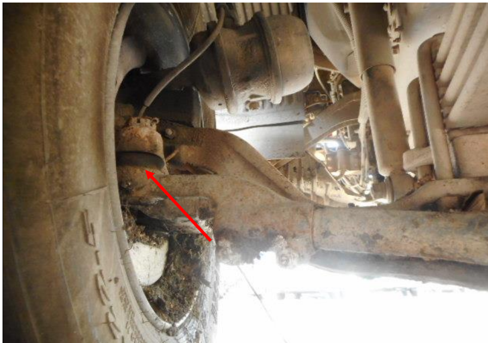
Photo 25 shows the various undercarriage components at the front left wheel of the Motor Tipper, in particular the steering tie rod end (arrowed). were found to be intact, there was also no sign of fluid stain(s) observed on the various undercarriage components.
