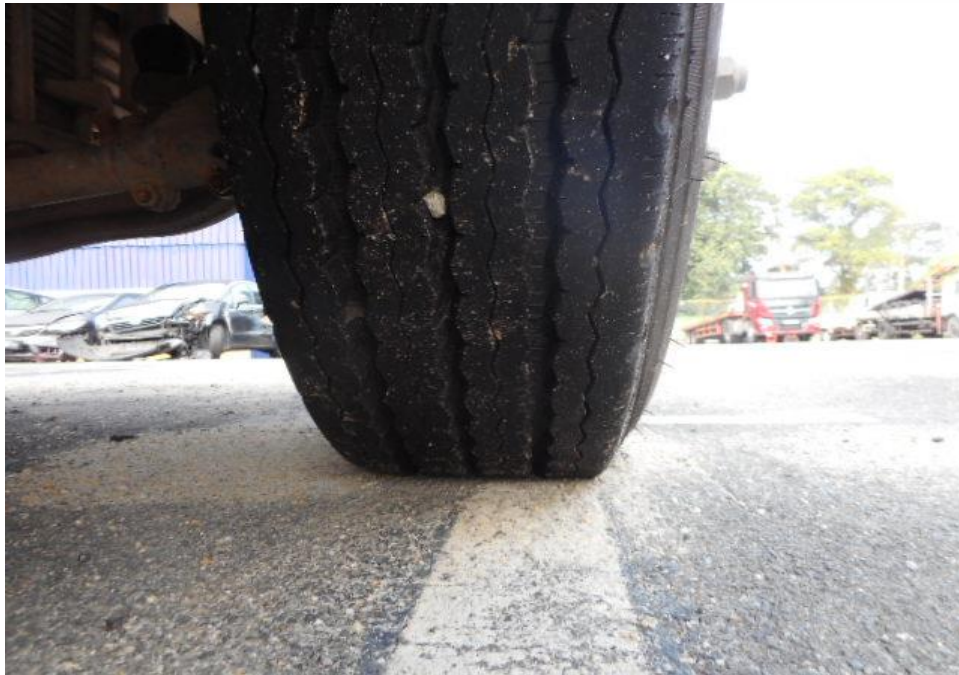
Photo 8 shows the condition of the front right tyre of the Motor Tipper, which was observed to be in serviceable condition with remaining tread depth of approximately 14.5mm. The tyre, which was wrapped around standard steel wheel rim, was also observed to be sufficiently inflated for vehicular operation. There was no tear, cut or burst mark(s) on the outer and the inner sidewalls as well as across the tread of the 10 tyres that were fitted on the Motor Tipper.
