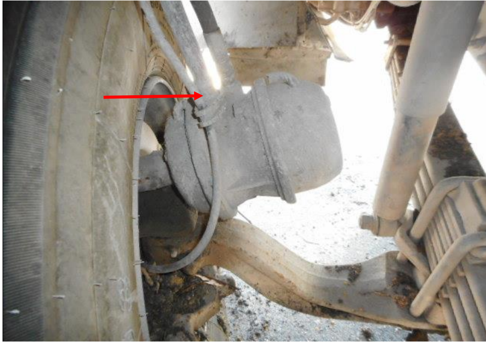
Photo 22 shows the brake pipe (arrowed) at the front left wheel of the Motor Tipper. I did not observe any leakage of brake fluid at the time of my inspection of the Motor Tipper. My visual examination of the various mechanical components in the braking system had indicated that these was no internal leakage of pressure/vacuum and these components were generally in good condition.
