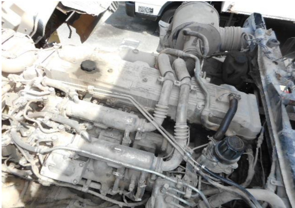
Photo 12 shows a general view of the Motor Tipper's engine compartment, which was accessed by lifting the front cabin of the Motor Tipper. The various parts and components inside the engine compartment were unaffected by the accident. There was also no sign(s) or indication(s) of fresh fluid leakage and/or fluid stain within the engine compartment
