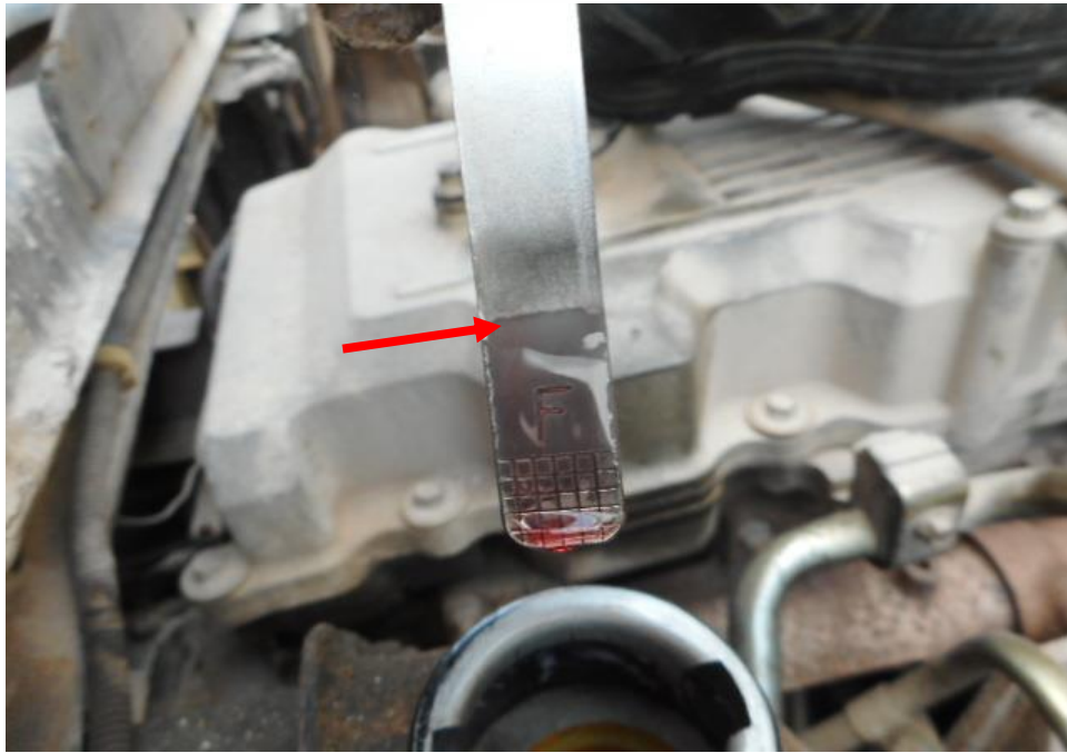
Photo 17 shows the power steering fluid reservoir of the Motor Tipper at the time of my inspection. The power steering fluid was observed to be of sufficient level (arrowed) and without any visible contamination.
