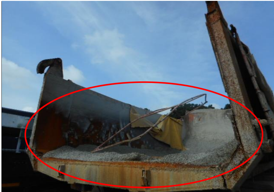
Photo 5 shows a close up view of the Motor Tipper's rear body at the time of my inspection. The Motor Tipper was observed to sustained damage at its rear portion. Its rear tipper body panel (circled) were damage at the time of my inspection as a result of the accident.
