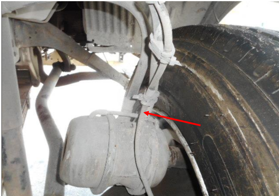
Photo 21 shows the brake pipe (arrowed) at the front right wheel of the Motor Tipper. I did not observe any leakage of brake fluid at the time of my inspection of the Motor Tipper. My static tests of the Motor Tipper's braking system, along with my visual examination of the various mechanical components in the braking system, had indicated that there was no internal leakage of pressure/vacuum and these components were generally in good condition.
