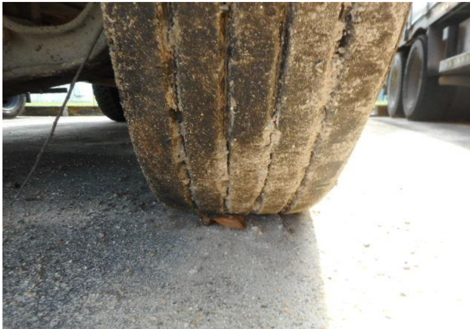
Photo 11 condition of the front left tyre of the Motor Tipper, which was observed to be in serviceable condition with remaining tread depth of approximately 10.6mm. The tyre, which was wrapped around standard steel wheel rim, was also observed to be sufficiently inflated for vehicular operation.
