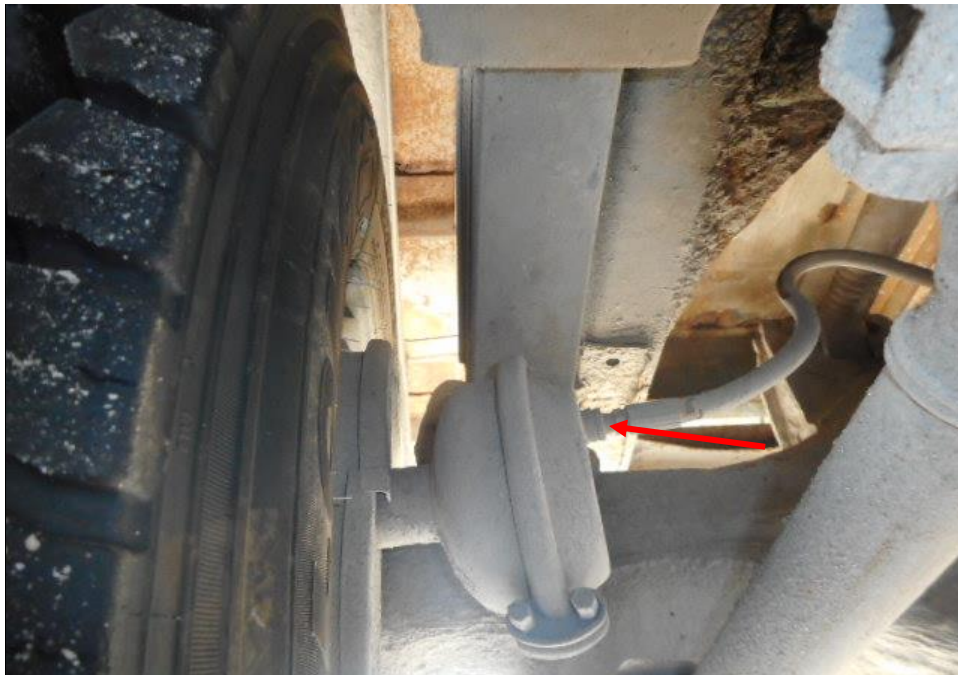
Photo 19 shows the brake pipe (arrowed) at the rear right wheel of the Motor Tipper. I did not observe any leakage of brake fluid at the time of my inspection of the Motor Tipper. My visual examination of the various mechanical components in the braking system, had indicated that there was no internal leakage of pressure/vacuum and these components were generally in good condition.
