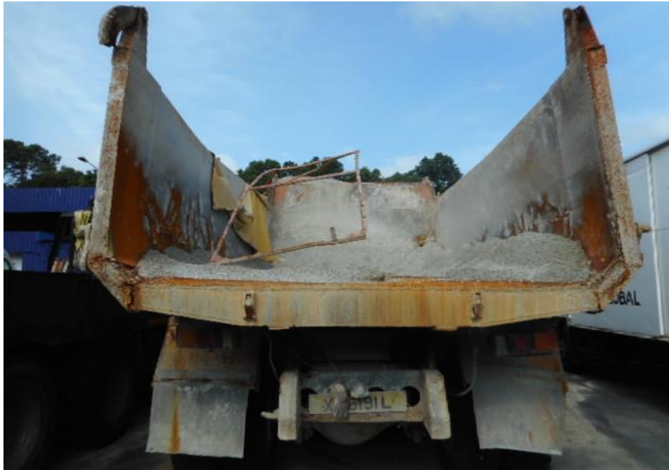
Photo 4 shows a general view of the Motor Tipper's rear body at the time of my inspection. The Motor Tipper was observed to sustained damage at its rear portion. Its rear tipper body panel were damage at the time of my inspection as a result of the accident.
