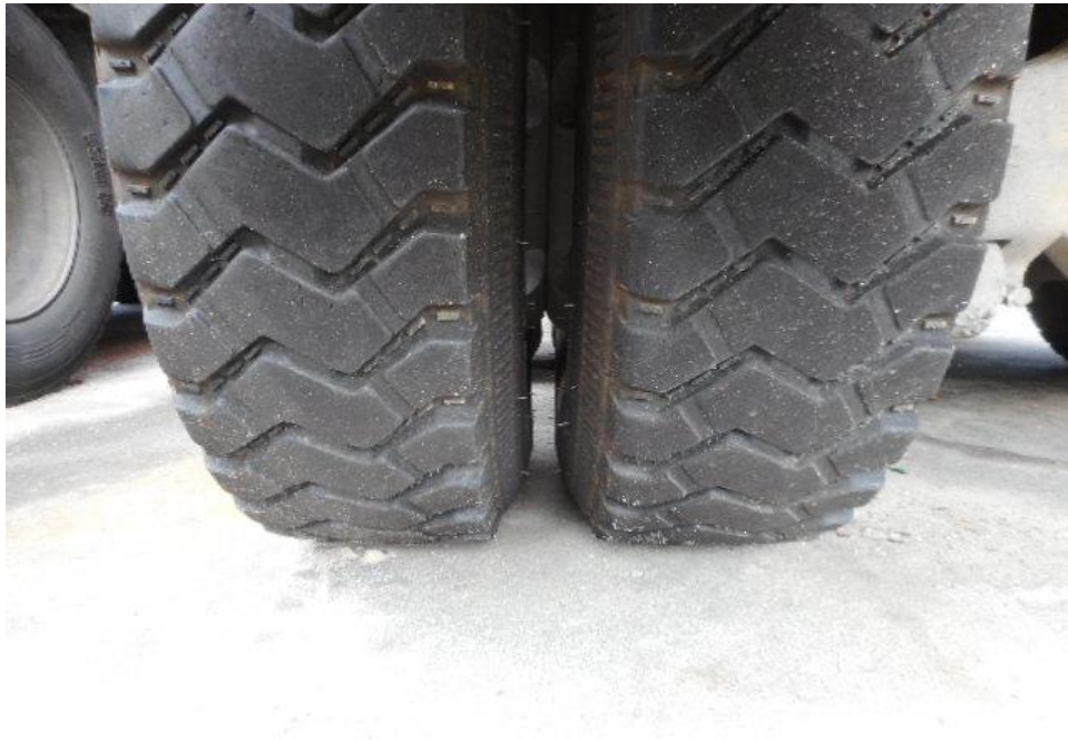
Photo 10 shows the condition of the rear left tyre of the Motor Tipper, which was observed to be in serviceable condition with remaining tread depth of approximately 12.6mm. The tyre, which was wrapped around standard steel wheel rim, was also observed to be sufficiently inflated for vehicular operation.
