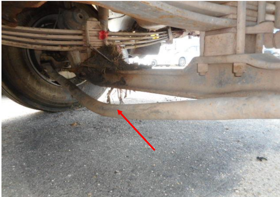
Photo 26 shows the steering tie rod end (arrowed) of the Motor Tipper. The steering tie rod was observed to sustained damage as a result of the accident.
