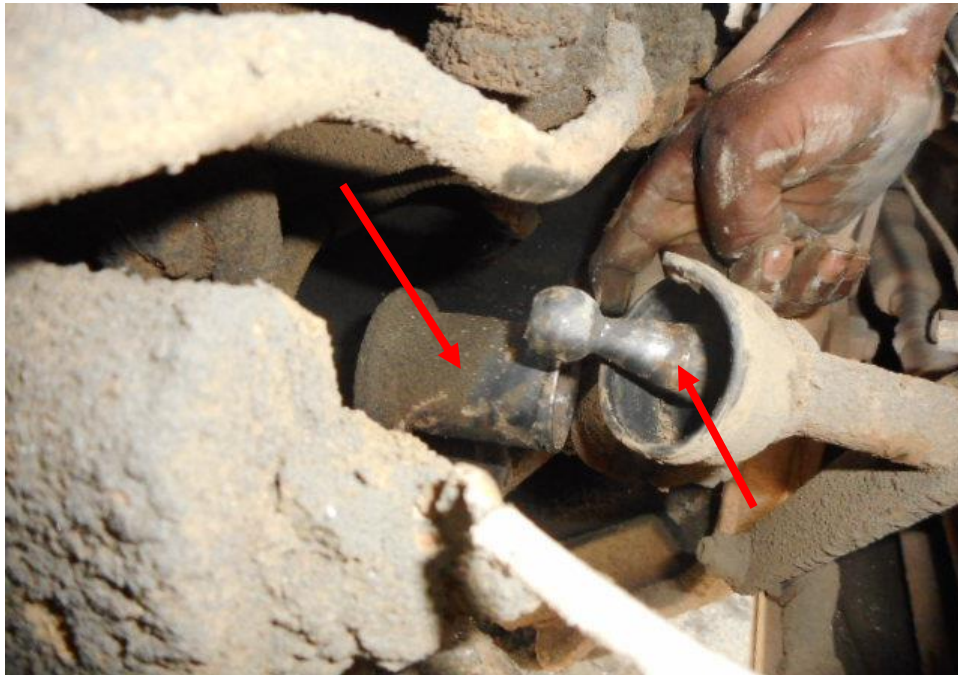
Photo 13 shows a close up view of the Motor Tipper's engine compartment, which was accessed by lifting the front cabin of the Motor Tipper. The gearbox shifter cable linkage (arrowed) was observed to be damaged and detached as a result of the accident.
