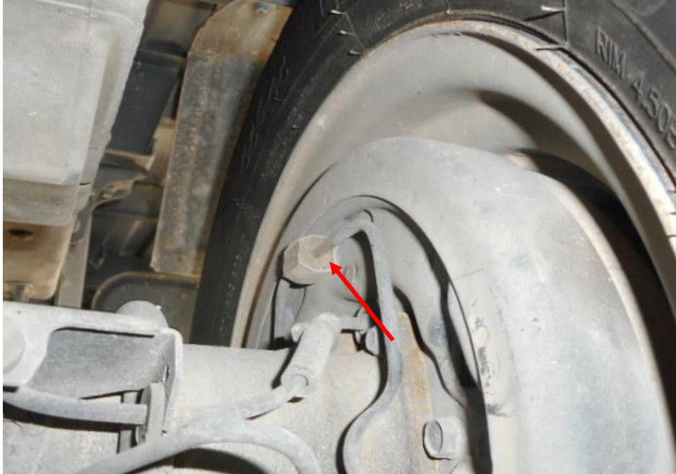
Photo 15 shows the brake pipe (arrowed) at the rear right wheel of the Motor Lorry. I did not observe any leakage of brake fluid at the time of my inspection of the Motor Lorry. My static tests of the Motor Lorry's braking system, along with my visual examination of the various mechanical components in the braking system, had indicated that there was no internal leakage of pressure/vacuum.
