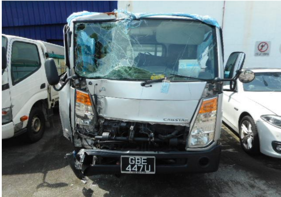
Photo 1 shows a general view of the front portion of the Motor Lorry at the time of our inspection. The Motor Lorry was observed sustained major damages to its front cabin, front windscreen, front bumper and front body panel as well as its right door due to the accident.
