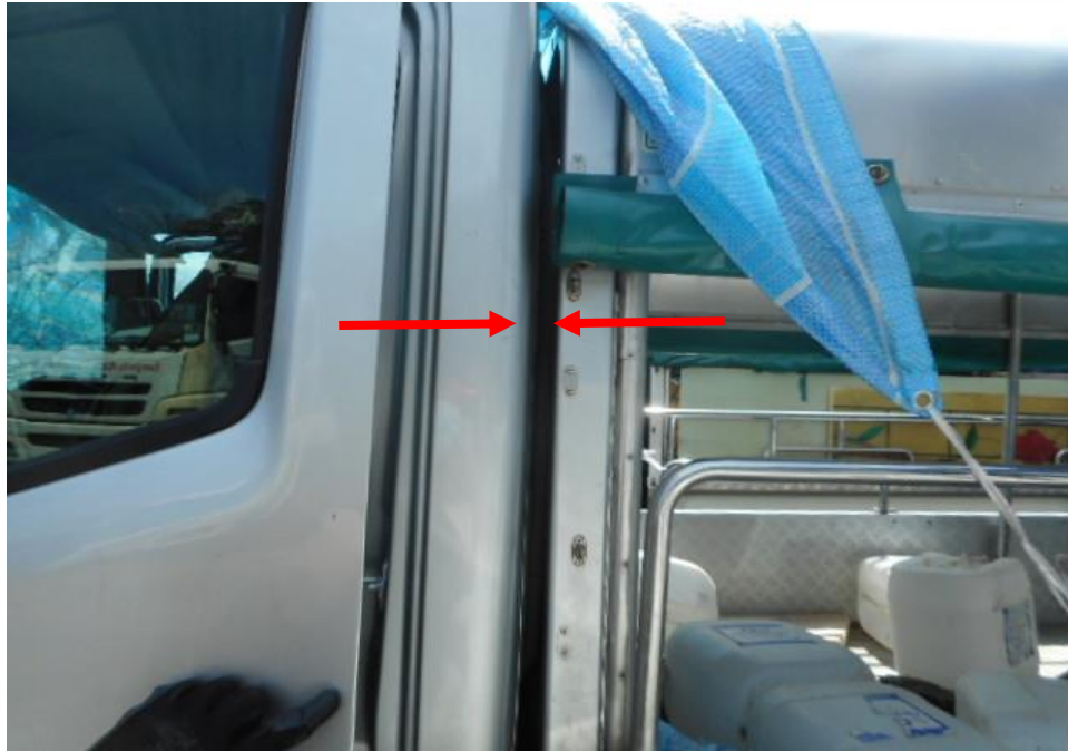
Photo 12 shows the induced damage to the lifter of the front cabin (arrowed) of the Motor Lorry's which had immobilised the opening and viewing of the various parts and components inside the engine compartment a result of the accident.
