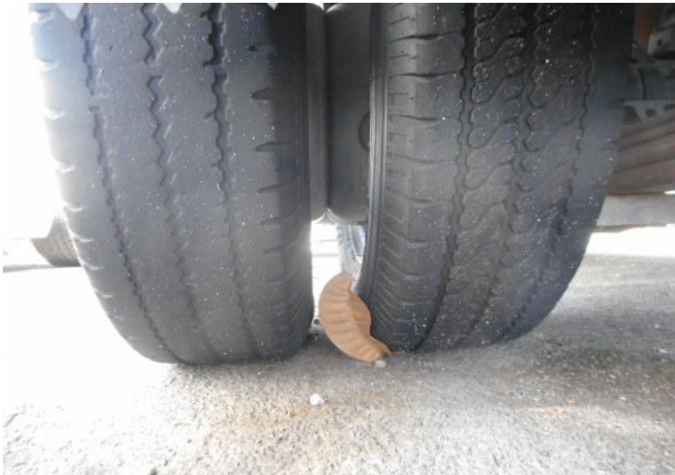
Photo 10 shows the condition of the rear left tyres of the Motor Lorry, which were observed to be in serviceable condition with remaining, tread depth of approximately 1.9mm.
