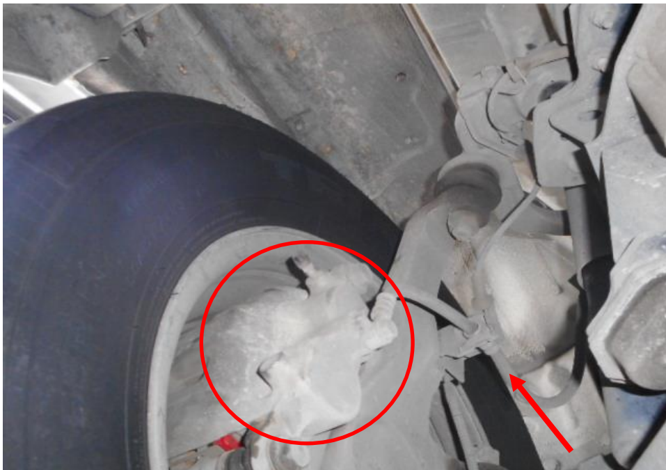
Photo 18 shows the brake hose/pipe (arrowed) at the front left wheel of the Motor Lorry. No leakage of brake fluid was observed. Visual examination of the various components of the braking system like the brake caliper (circled), brake booster, brake pedal etc had revealed all to be intact and without visible damage at the time of accident. There was also no sign of fluid stain(s) observed on the various undercarriage components.
