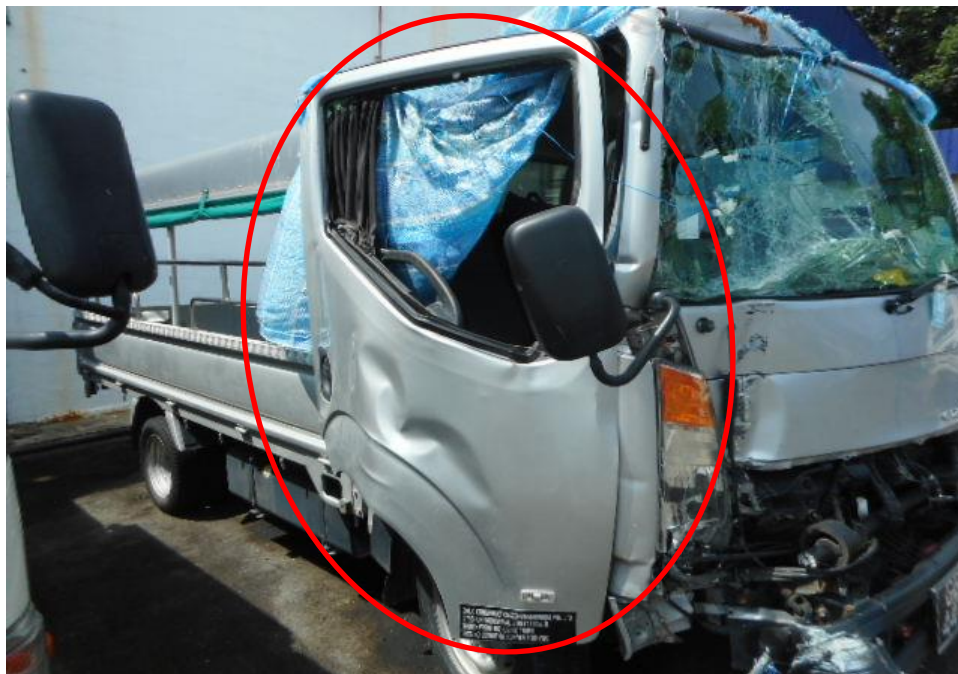
Photo 4 shows the close up view of the right door of the Motor Lorry at the time of our inspection. The Motor Lorry was observed to have sustained damages to its right door (circled) as a result of the accident.
