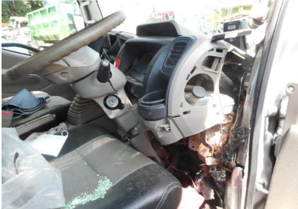
Photo 19 shows instrument cluster and dashboard of the Motor Lorry at the time of our inspection. The instrument cluster was observed to be damaged as a result of the accident.
