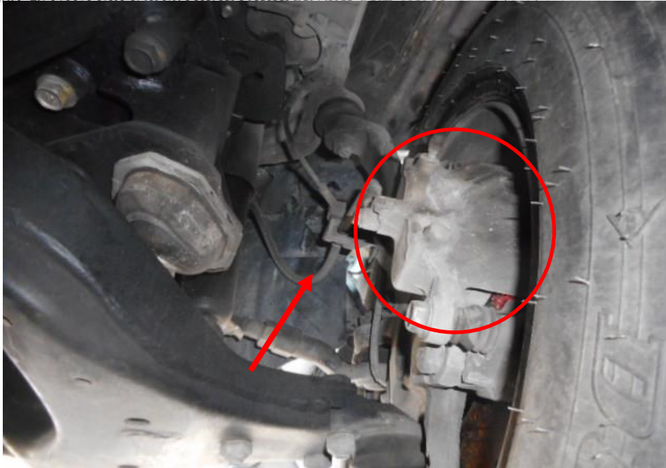
Photo 17 shows the brake hose/pipe (arrowed) at the front right wheel of the Motor Lorry. No leakage of brake fluid was observed. Visual examination of the various components of the braking system like the brake caliper (circled), brake booster, brake pedal etc had revealed all to be intact and without visible damage at the time of accident. There was also no sign of fluid stain(s) observed on the various undercarriage components.
