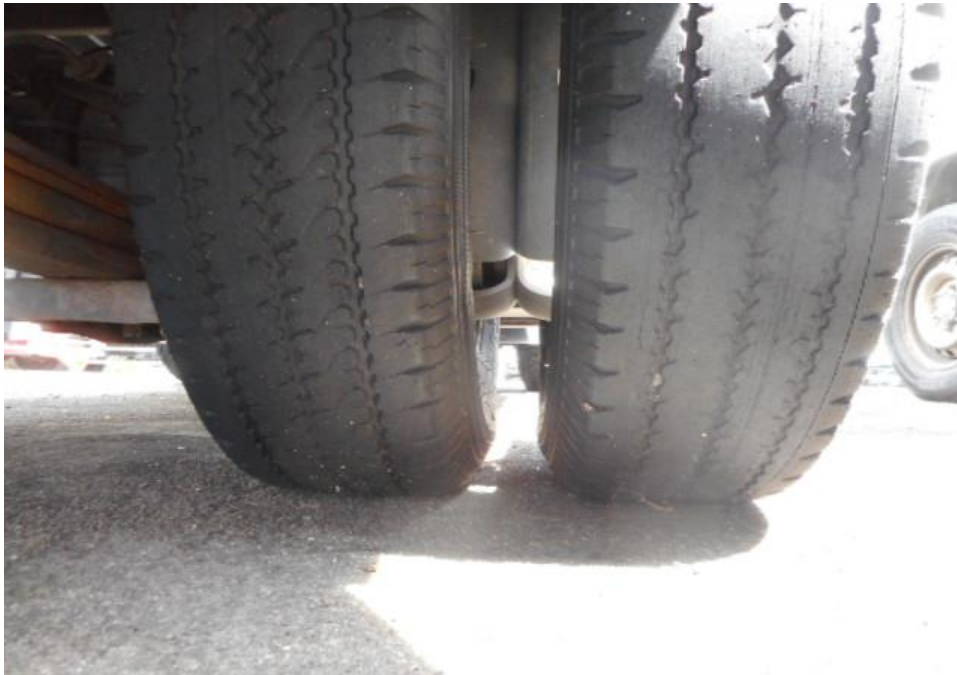
Photo 9 shows the condition of the rear right tyres of the Motor Lorry, which were observed to be in serviceable condition with remaining, tread depth of approximately 1.6mm. The tyre, which was wrapped around standard steel wheel rim, it was observed to be sufficiently inflated for vehicular operation.
