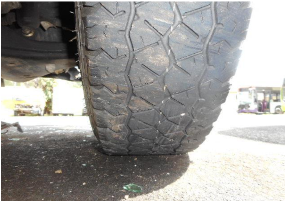
Photo 8 shows the condition of the front right tyre of the Motor Lorry, which were observed to be in serviceable condition with remaining, tread depth of approximately 5.1mm. The tyre, which was wrapped around standard steel wheel rim, it was observed to be sufficiently inflated for vehicular operation.
