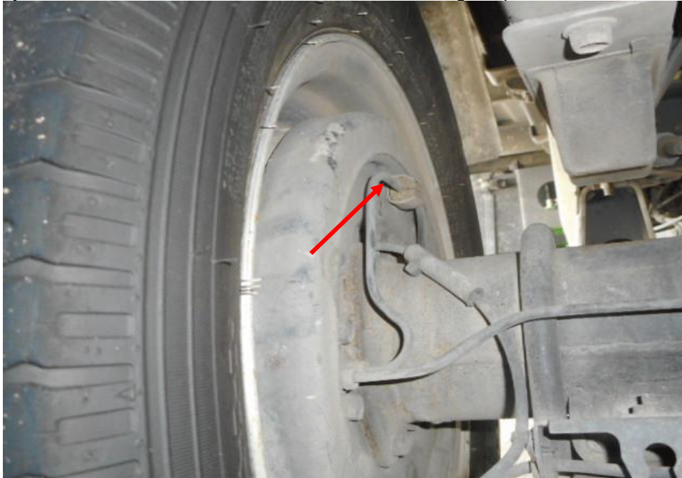
Photo 16 shows the brake pipe (arrowed) at the rear left wheel of the Motor Lorry. I did not observe any leakage of brake fluid at the time of my inspection of the Motor Lorry. My static tests of the Motor Lorry's braking system, along with my visual examination of the various mechanical components in the braking system had indicated that there was no internal leakage of pressure/vacuum. Hence the braking system of the Motor Lorry was likely to be in serviceable condition at the material time of accident.
