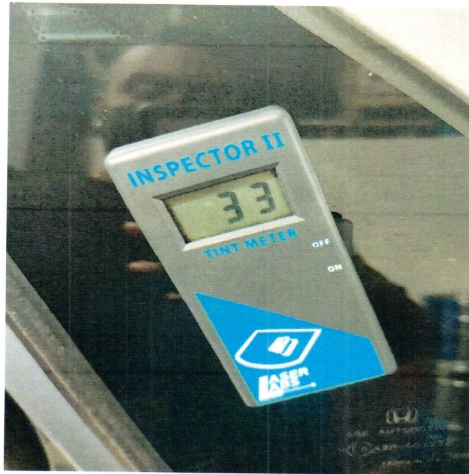
Rear Quarter Glass VLT Reading: 32% (Right)
