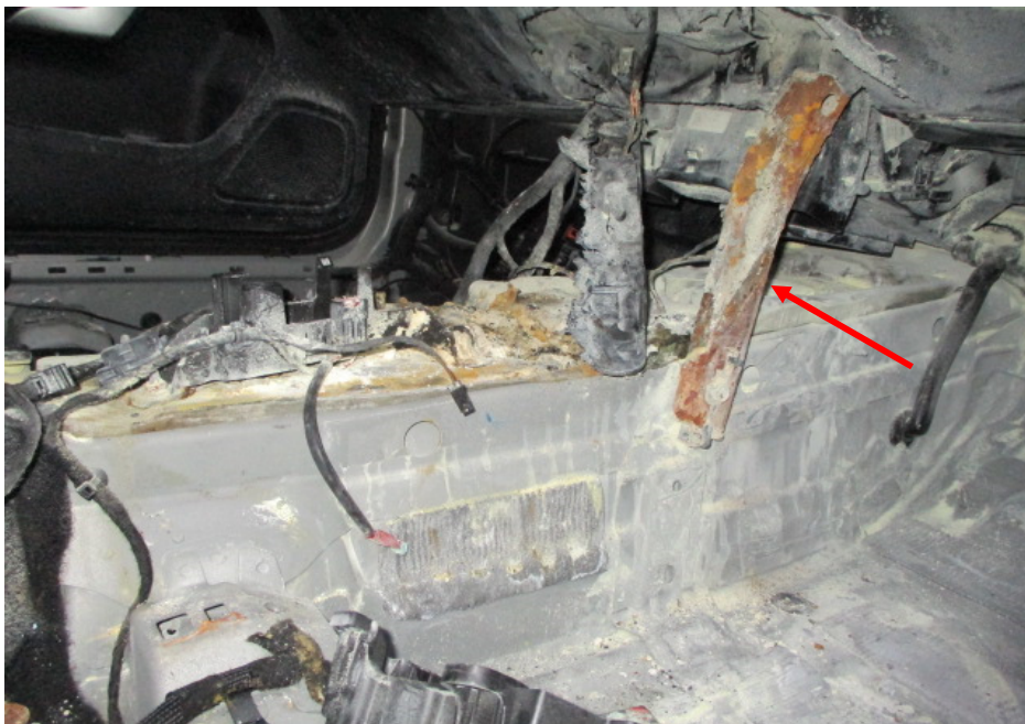
Photo 14 shows a closer view of the rust that had developed on the front dashboard reinforcement, at the right side (arrowed). This is the same side and in close proximity to where the auxiliary power outlet is located.
