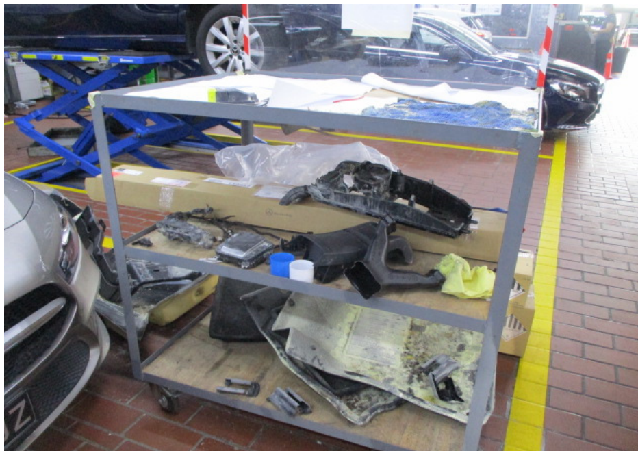
Photo 6 shows a general view of some of the burnt/damaged parts that were removed from the interior compartment of the Insured Vehicle prior to my inspection. These parts had included carpet, control panels, air ducts and trims amongst others.
