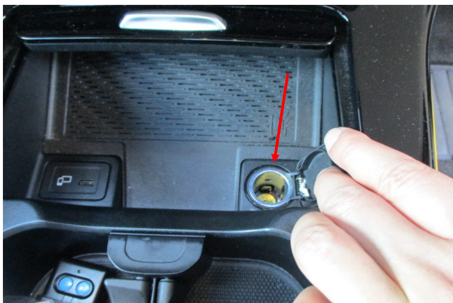
Photo 10 shows the auxiliary power outlet (arrowed) or more commonly referred to as cigarette lighter socket of a similar make and model vehicle as the Insured Vehicle. The auxiliary power outlet of the Insured Vehicle was found to be rusted (refer to photograph 11 & 12 below), which is a sign of prolonged exposure to high heat intensity. The auxiliary power outlet is also located towards the right of the centre console where the front dashboard reinforcement was correspondingly found to be rusted (refer to photograph 13 & 14 below).
