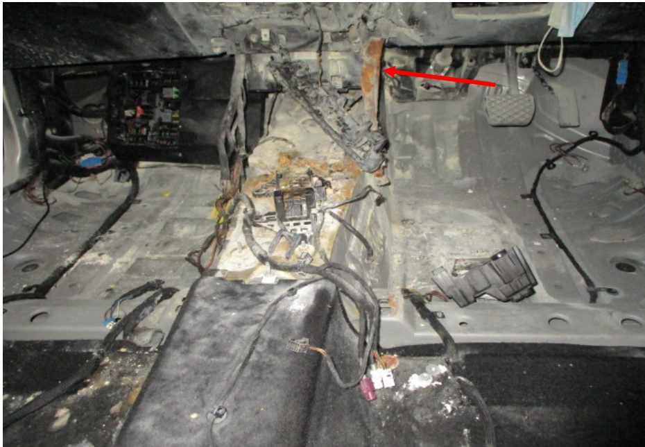
Photo 13 shows a general view of the centre console area of the Insured Vehicle, after the burnt/damaged parts surrounding the centre console were dismantled and removed. Rust was observed on the front dashboard reinforcement, at the right side (arrowed). This is the same side and in close proximity to where the auxiliary power outlet is located. The presence of rust seen on the front dashboard reinforcement is again an indication of prolonged exposure to high heat intensity and hence supports the fire occurring at the auxiliary power outlet of the Insured Vehicle.
