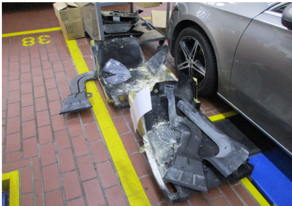
Photo 5 shows a general view of some of the burnt/damaged carpet, trims and aircon ducts that were removed from the interior compartment of the Insured Vehicle prior to my inspection.
