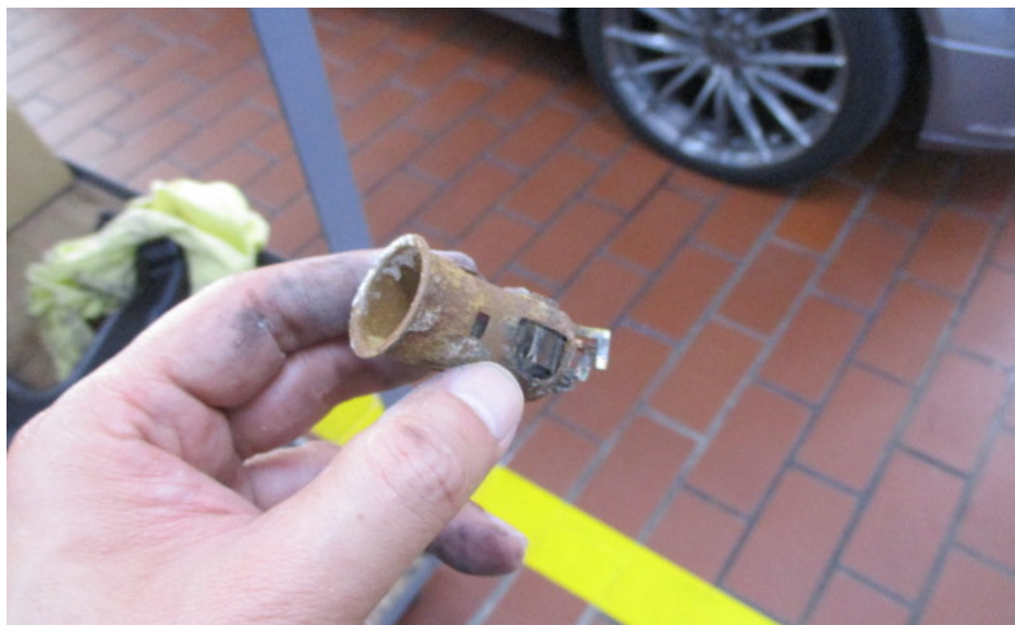
Photo 11 shows the auxiliary power outlet of the Insured Vehicle, which was found to be rusted. The presence of rust on a steel/metal material body part of a vehicle that was involved in a fire incident is a consequence of that body part being exposed to natural environmental condition after layers of paint and its related compounds were melted due to prolonged exposure of that particular body part to high heat intensity. Following the aforesaid, it would be reasonable to determine that the auxiliary power outlet of the Insured Vehicle was exposed to prolonged high heat intensity.
