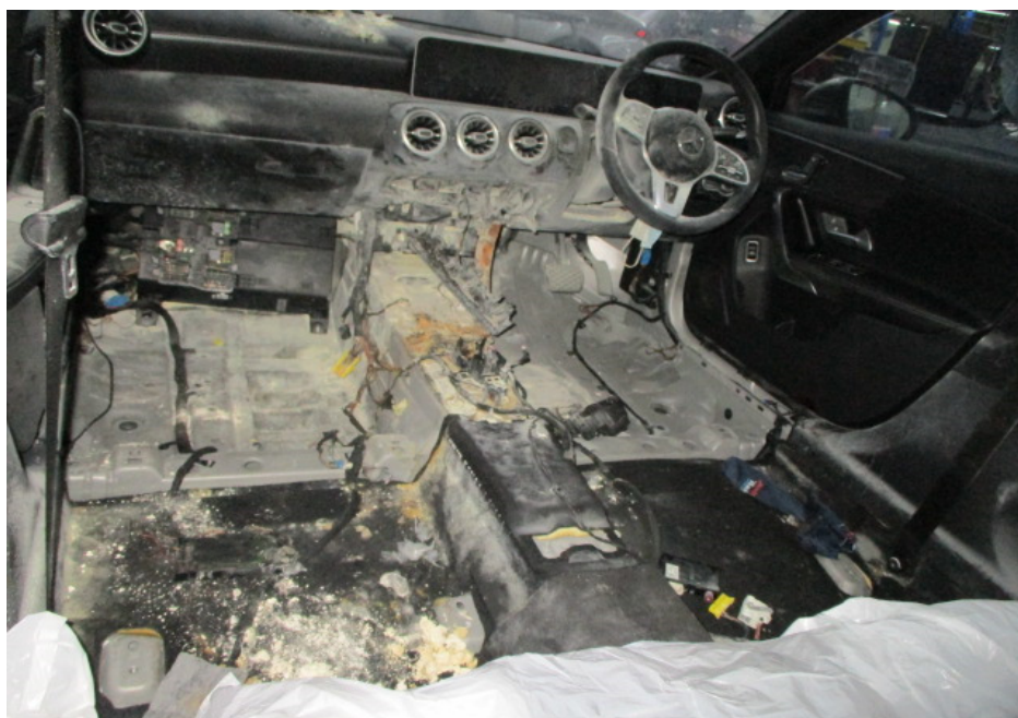
Photo 4 shows the interior compartment of the Insured Vehicle. Fire damage that was confined to the centre console area of the interior compartment was observed. The front dashboard, centre console, arm rest console, carpet, trims, upholstery, wirings and steering wheel were amongst the parts that were observed to be burnt and/or had sustained heat/smoke damage.
