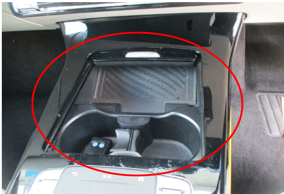
Photo 9 shows the centre console of a similar make and model vehicle as the Insured Vehicle. The fire to the Insured Vehicle had occurred at the area highlighted by the red circle. This takes into consideration that there was no fire damage observed at other areas of the Insured Vehicle apart for the fire damage seen at this same area of the Insured Vehicle immediately after the fire was extinguished, which is shown in photograph 8 above.
