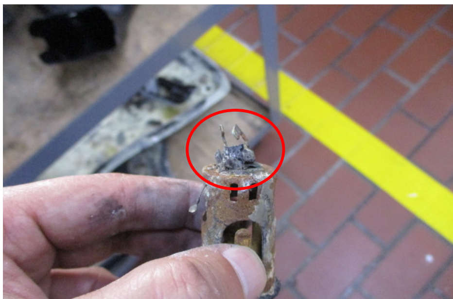
Photo 12 shows the auxiliary power outlet of the Insured Vehicle, which was found to be rusted. The auxiliary power outlet is also a connector supplying electrical power (direct current) from the vehicle's electrical system. The connecting pins are highlighted by the red circle. The fire to the Insured Vehicle had likely arisen due to abnormality of the electrical current at the auxiliary power outlet of the Insured Vehicle. In other words, the fire to the Insured Vehicle was of electrical nature to the wirings connecting to the pins of the auxiliary power outlet.
