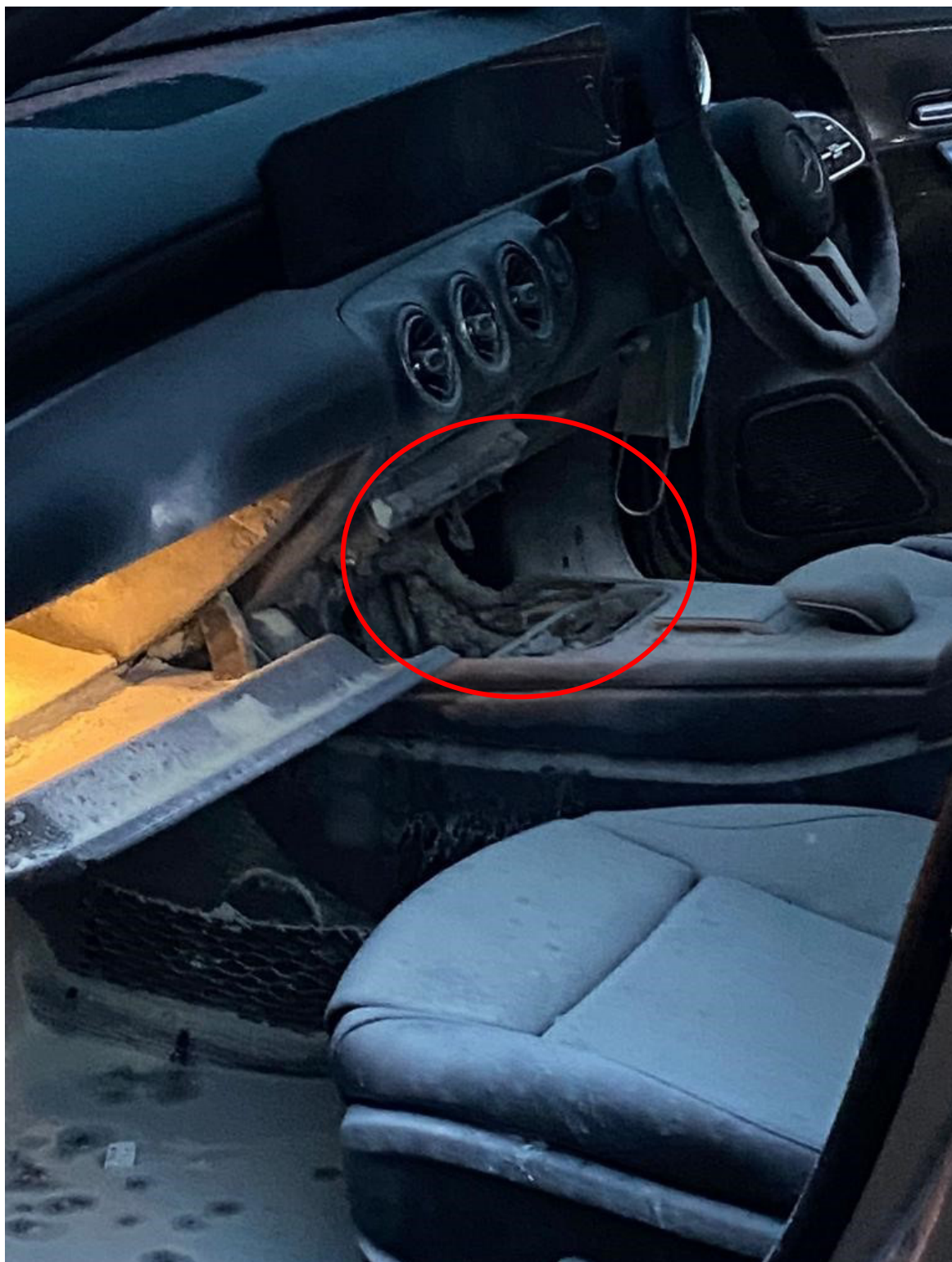
Photo 8 shows the interior compartment of the Insured Vehicle at the incident scene, after the fire was extinguished (photograph provided to me by Mr Tan). A section of the Insured Vehicle's centre console (circled), within the interior compartment, was seen to be melted/burnt. Notable, I did not observe any electronic device(s) placed near the melted/burnt area.
