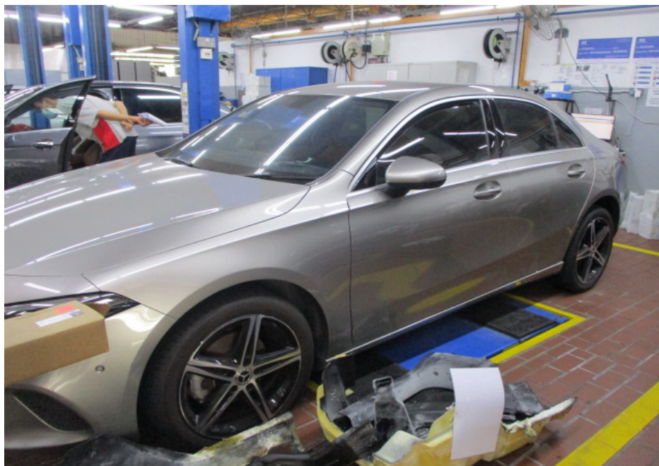
Photo 2 shows a general view of the left body of the Insured Vehicle at the time of my inspection. I did not observe any damage of fire nature to the exterior body of the Insured Vehicle. Its rear boot compartment and engine compartment were also found to be without any damage of fire nature.
