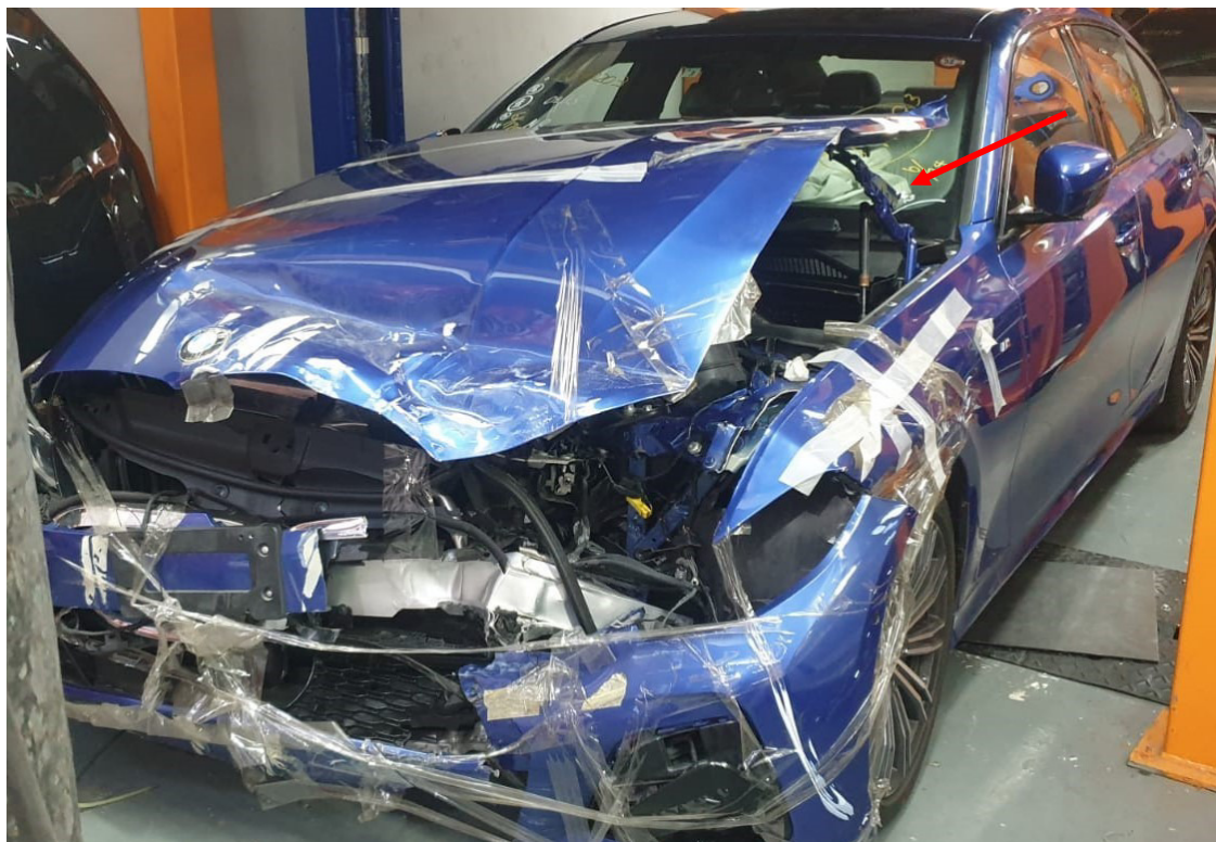
Photo 1 shows the front left body of the Motor Car (photograph provided to me). The Motor Car was observed to have sustained damage at its frontal portion. The front bumper, front bumper reinforcement, front bumper sponge, front bumper centre lower grille, front bumper left lower grille, radar unit, front bonnet, front bonnet left lock, front bonnet left hinge, front left day light, front left headlamp, front left fender, front support panel, front left headlamp top panel, aircon condenser and radiator were amongst the body parts that were observed to have been damaged. The front left passenger airbag was deployed (arrowed).
