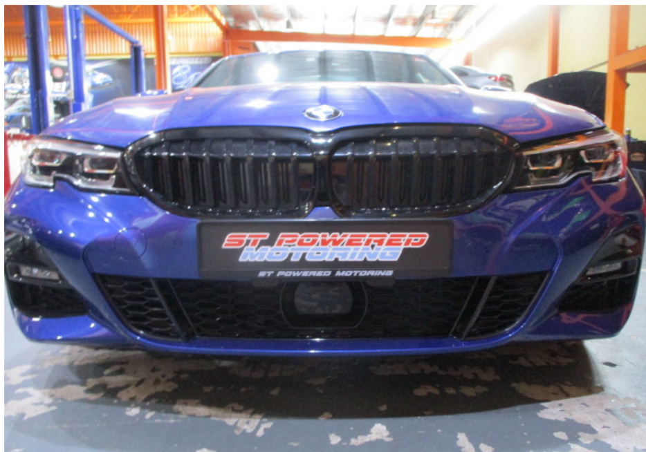
Photo 10 shows a closer view of the Motor Car's front bumper, front bumper centre lower grille, front bonnet, front day lights, front headlamps, radar unit and radiator grilles. The body parts at the frontal portion of the Motor Car were visually examined, and it was observed that the repair/restoration works carried out to the damaged area of the Motor Car (refer to photograph 1 & 2 above) were reasonably adequate and in order.
