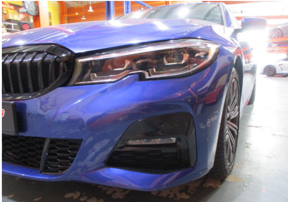
Photo 9 shows a closer view of the Motor Car's front bumper, front bumper left lower grille, front bumper left day light and front left headlamp. The body parts at the frontal portion of the Motor Car were visually examined and it was observed that the repair/restoration works carried out to the damaged area of the Motor Car (refer to photograph 1 & 2 above) were reasonably adequate and in order.
