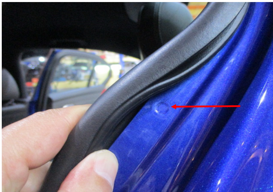
Photo 33 shows the left side "C" pillar of the Motor Car. I did not find any weld marks other than original spot weld marks (arrowed) on the left side "C" pillar of the Motor Car which, indicates that there was no re-welding works carried out. In general, I had found all the non-detachable body panels of the Motor Car to be originally fitted at the time of my inspection.
