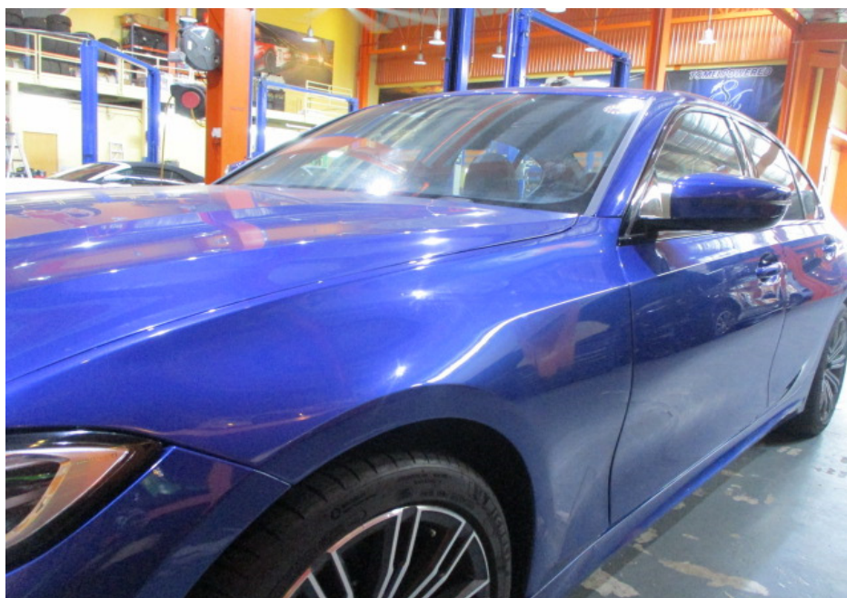
Photo 8 shows a closer view of the Motor Car's front left fender, front left door and front bonnet. The body parts at the frontal portion of the Motor Car were visually examined and it was observed that the repair/restoration works carried out to the damaged area of the Motor Car (refer to photograph 1 & 2 above) were reasonably adequate and in order.
