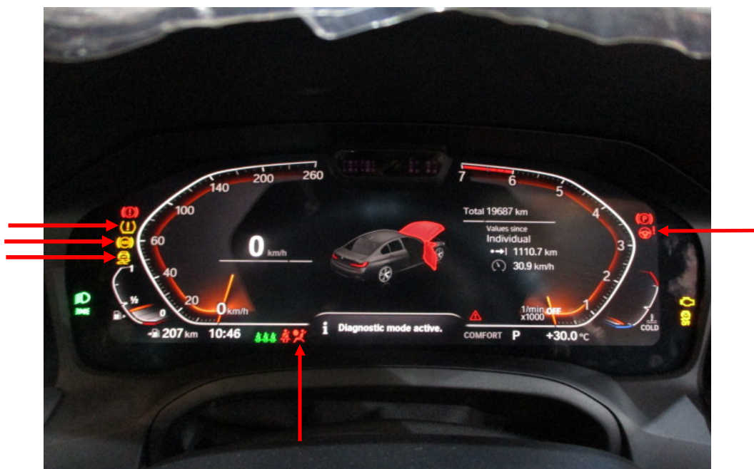
Photo 17 shows the warning lights for the various electronic safety features appearing on the instrument panel of the Motor Car during its self-test when the engine is cranked, in particular the ABS, SRS, IAS, TPM and DSC lights (arrowed).
