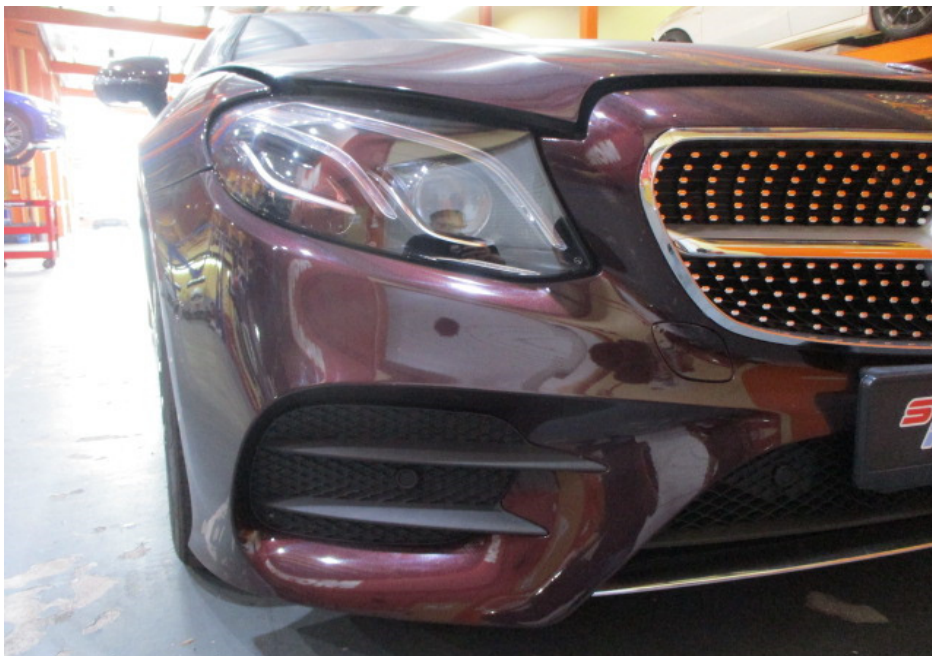
Photo 7 shows a closer view of the Motor Car's front bumper, front bumper right lower grille, front bumper centre lower grille, front bumper lower chrome moulding and front right headlamp. The body parts at the frontal portion of the Motor Car were visually examined and it was observed that the repair/restoration works carried out to the damaged area of the Motor Car (refer to photograph 1 & 2 above) were reasonably adequate and in order.
