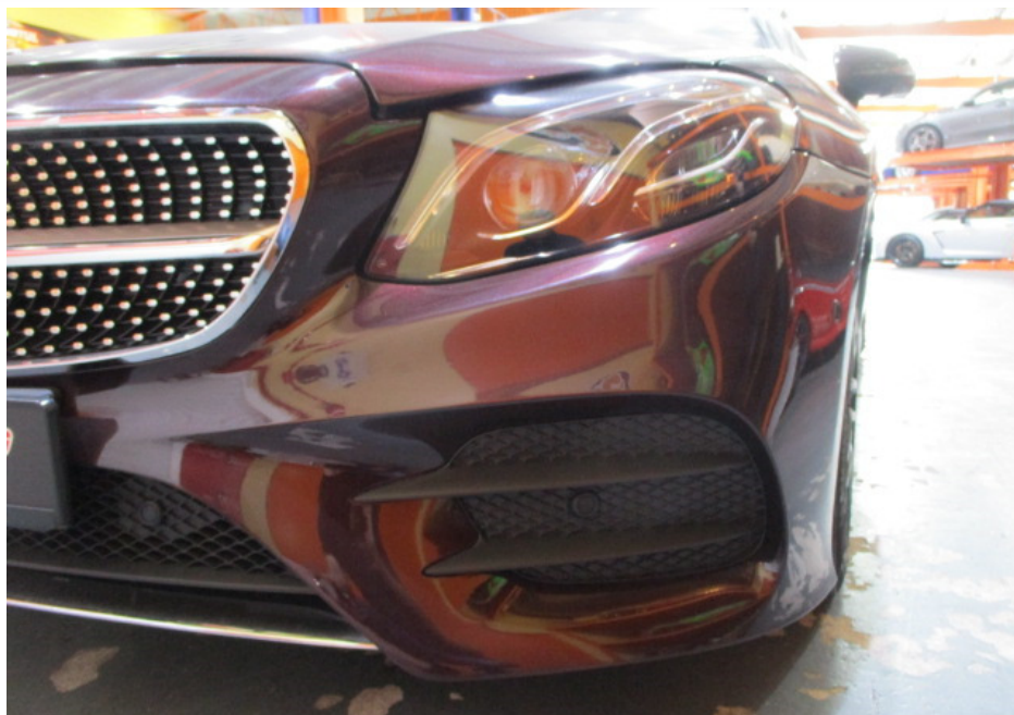
Photo 10 shows a closer view of the Motor Car's front bumper, front bumper left lower grille and front left headlamp. The body parts at the frontal portion of the Motor Car were visually examined and it was observed that the repair/restoration works carried out to the damaged area of the Motor Car (refer to photograph 1 & 2 above) were reasonably adequate and in order.
