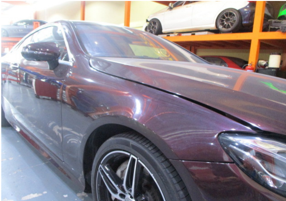
Photo 6 shows a closer view of the Motor Car's front right headlamp, front right fender and front bonnet. The body parts at the frontal portion of the Motor Car were visually examined and it was observed that the repair/restoration works carried out to the damaged area of the Motor Car (refer to photograph 1 & 2 above) were reasonably adequate and in order.
