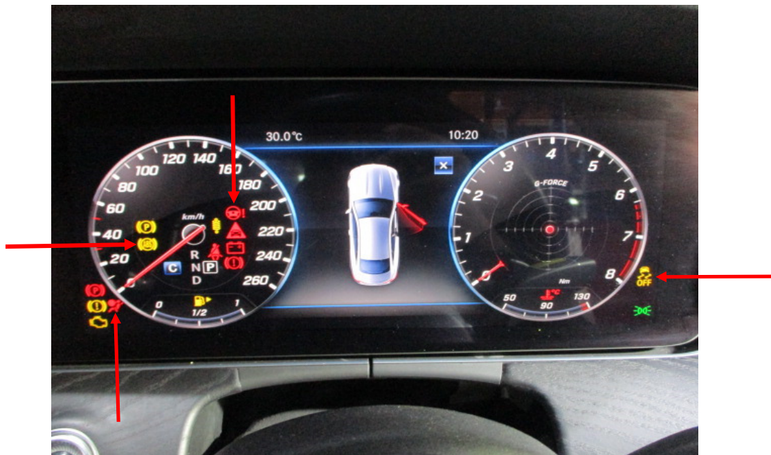
Photo 18 shows the warning lights for the various electronic safety features appearing on the instrument panel of the Motor Car during its self-test when the engine is cranked, in particular the ABS, SRS, EPS and TCS lights (arrowed).
