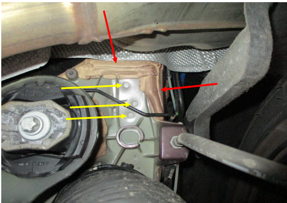
Photo 27 shows the chassis/structural body at the underside rear right of the Motor Car. I did not find any weld marks other than original spot weld marks (yellow arrow) on the chassis/structural body of the Motor Car. The original factory sealant (red arrow) at the joints along the chassis/structural body was also untouched, indicating no work was done on the chassis/structural body of the Motor Car and that the chassis/structural body was originally fitted.
