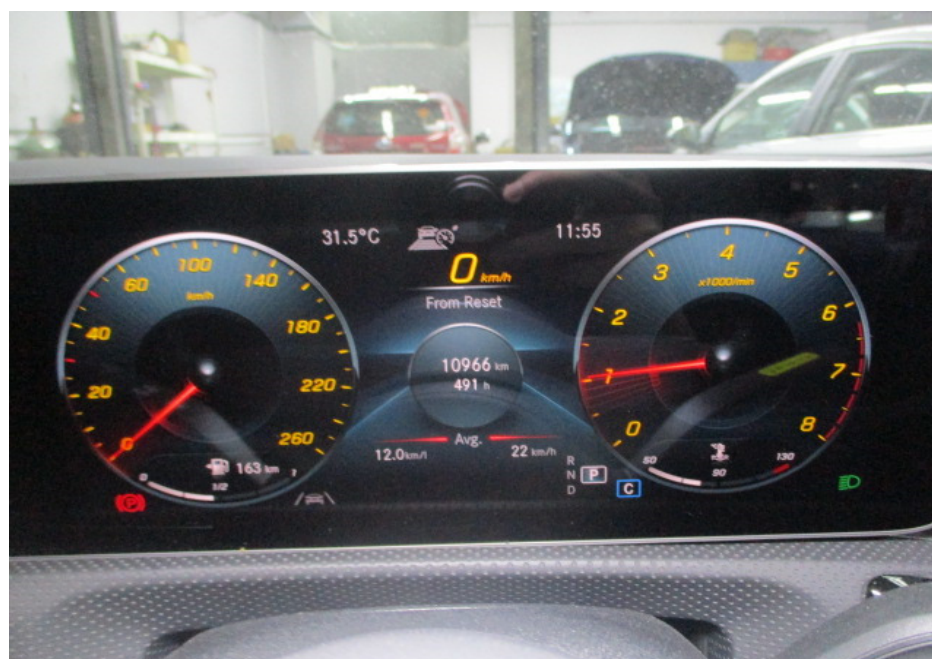
Photo 17 shows the respective warning lights no longer illuminated, indicating that there is no fault detected to the ABS, SRS, EPS and TCS systems of the Motor Car during the self-test. These electronic systems were hence in working condition at the time of my inspection.
