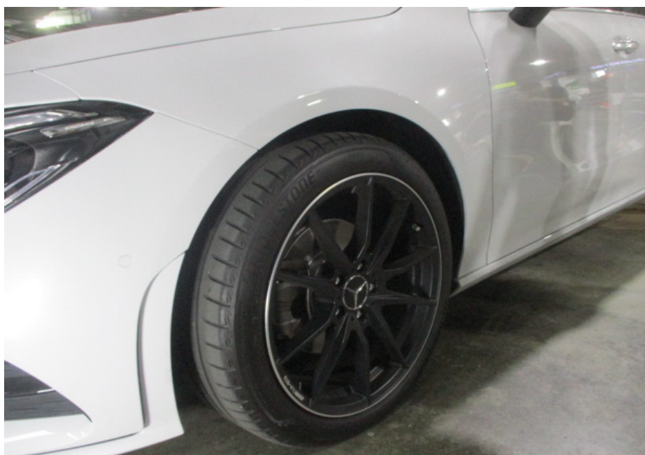
Photo 7 shows a closer view of the Motor Car's front left fender, front left wheel rim, front left tyre and left side rocker panel garnish. The body parts at the front left portion of the Motor Car were visually examined and it was observed that the repair/restoration works carried out to the damaged area of the Motor Car (refer to photograph 1 & 2 above) were reasonably adequate and in order.
