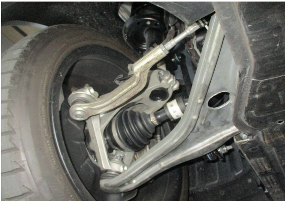
Photo 21 shows a general view of the control arms and linkages at the front left wheel of the Motor Car. I did not observe any fluid leak and/or fluid stain on the underside of the Motor Car. All of the Motor Car's undercarriage components were observed to be intact and secured in an appropriate manner.
