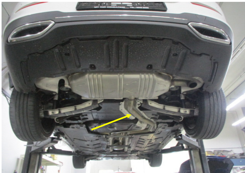
Photo 23 shows the rear section of the Motor Car's exhaust system. My examination of the Motor Car's exhaust system revealed no sign(s) or indication(s) of any cut or weld marks along its exhaust pipes (arrowed), on its rear muffler, on its centre resonator box and on its catalytic converter.
