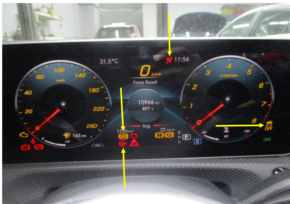
Photo 16 shows the warning lights for the various electronic safety features appearing on the instrument panel of the Motor Car during its self-test when the engine is cranked, in particular the ABS, SRS, EPS and TCS lights (arrowed).
