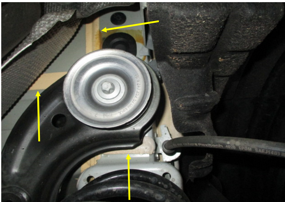
Photo 25 shows the chassis/structural body at the underside rear right of the Motor Car. I did not find any weld marks other than original spot weld marks on the chassis/structural body of the Motor Car. The original factory sealant (arrowed) at the joints along the chassis/structural body was also untouched, indicating no work was done on the chassis/structural body of the Motor Car and that the chassis/structural body was originally fitted.
