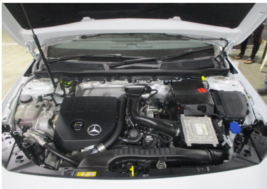
Photo 13 shows a general view of the engine compartment of the Motor Car at the time of my inspection. The various parts and components inside the engine compartment were all observed to be intact and properly fitted. There was also no sign(s) or indication(s) of fluid leak and/or fluid stain found inside the engine compartment. The repair/restoration works carried out to the various parts within the engine compartment like the front support panel and front windscreen washer tank amongst others, were reasonably adequate and in order.
