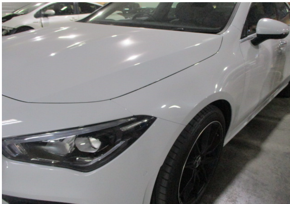
Photo 6 shows a closer view of the Motor Car's front bumper, front bonnet, front left headlamp and front left fender. The body parts at the front left portion of the Motor Car were visually examined and it was observed that the repair/restoration works carried out to the damaged area of the Motor Car (refer to photograph 1 & 2 above) were reasonably adequate and in order.
