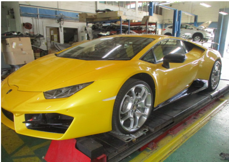
Photo 7 shows a general view of the front left body of the Motor Car at the time of my inspection. The Motor Car was observed to be in a relatively good general condition with no loose exterior fittings observed. The body parts at the left side portion of the Motor Car were visually examined and it was observed that the repair/restoration works carried out to the damaged area of the Motor Car (refer to photograph 1 – 4 above) were reasonably adequate and in order.
