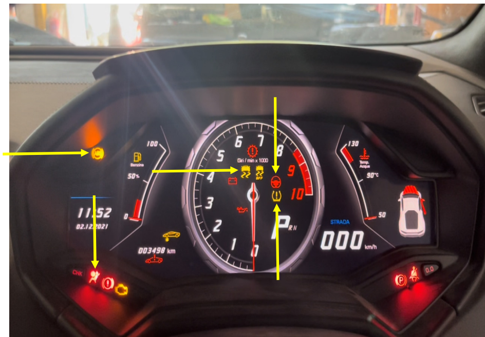
Photo 20 shows the warning lights for the various electronic safety features appearing on the instrument panel of the Motor Car during its self-test when the engine is cranked, in particular the ABS, SRS, EPAS, TPM and TCS lights (arrowed).
