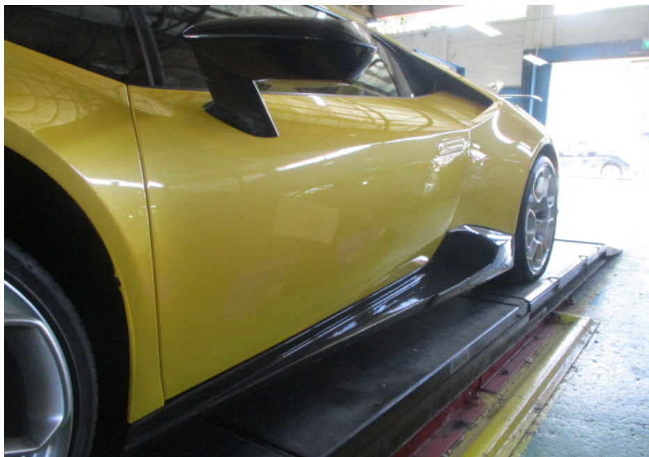
Photo 8 shows a closer view of the Motor Car's front left door, left wing mirror and left side lower skirting at the time of my inspection. The body parts at the left side portion of the Motor Car were visually examined and it was observed that the repair/restoration works carried out to the damaged area of the Motor Car (refer to photograph 1 – 4 above) were reasonably adequate and in order.
