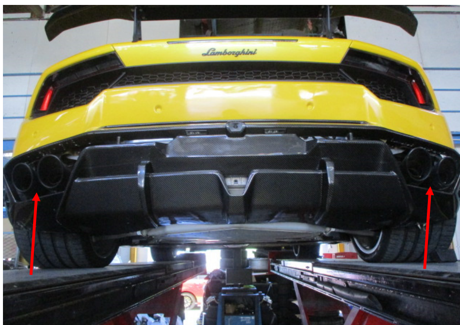
Photo 27 shows the rear exhaust tips (arrowed) of the Motor Car. The Motor Car's exhaust system could not be examined as the exhaust pipes, rear mufflers and catalytic converters were all hidden from view.
