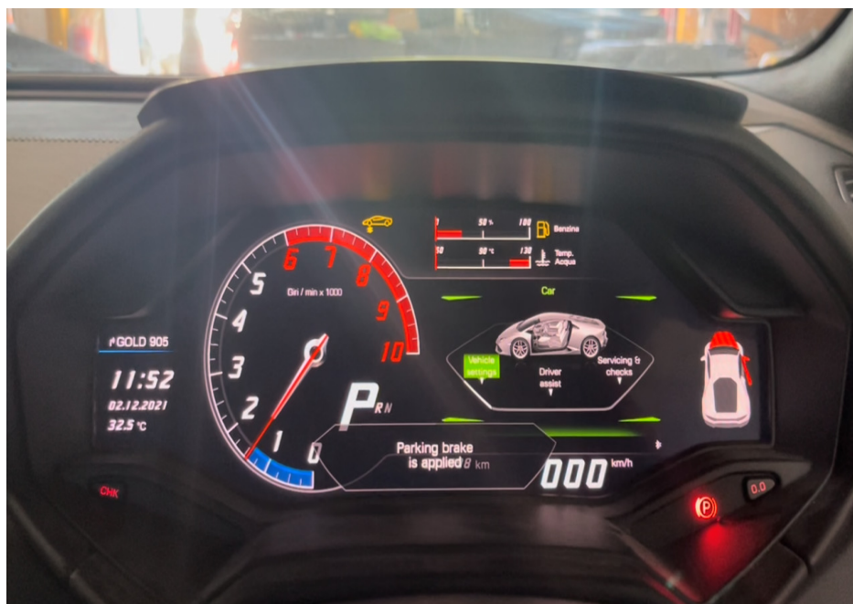
Photo 21 shows the respective warning lights no longer illuminated, indicating that there is no fault detected to the ABS, SRS, EPAS, TPM and TCS systems of the Motor Car during the self-test. These electronic systems were hence in working condition at the time of my inspection.
