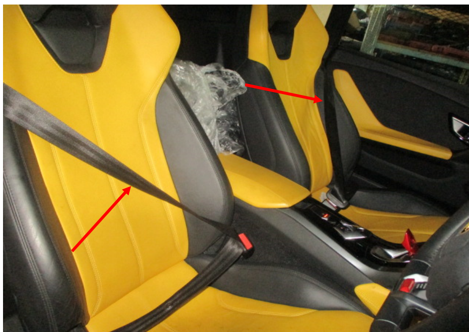
Photo 19 shows the seats of the Motor Car. All the seats of the Motor Car were secured via seat rails to the floorboard. They were also fitted with a retractable seat belt reel and a pre-tensioner. The seat belts (arrowed) were tested and were able to be fastened into the respective pre-tensions that were fitted on the side of each individual seat.
