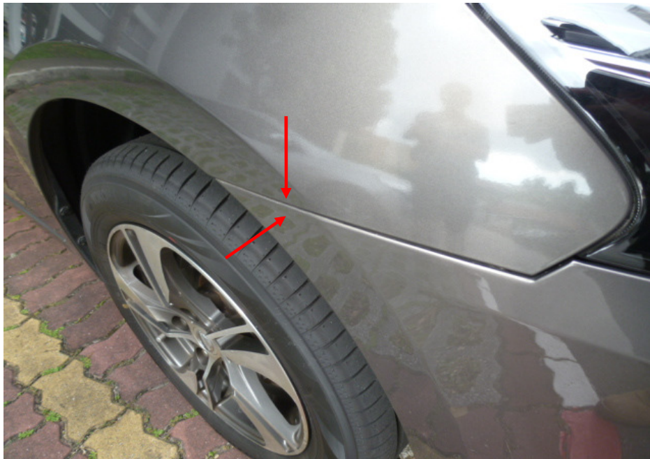
Photo 11 shows a closer view of the right corner edge of the front bumper of the Nissan. We observed no misalignment at the corner edges (red arrows).
