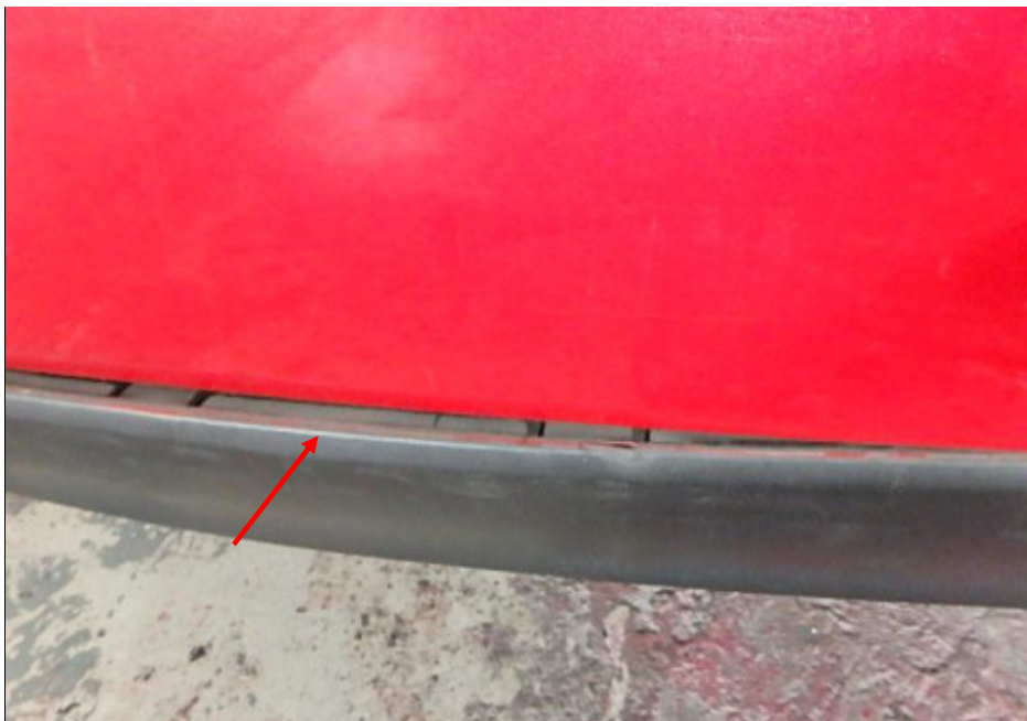
Photo 3 shows a close up view of the slight dislodgement of the lower rear bumper cover (arrowed) of the Taxi.
