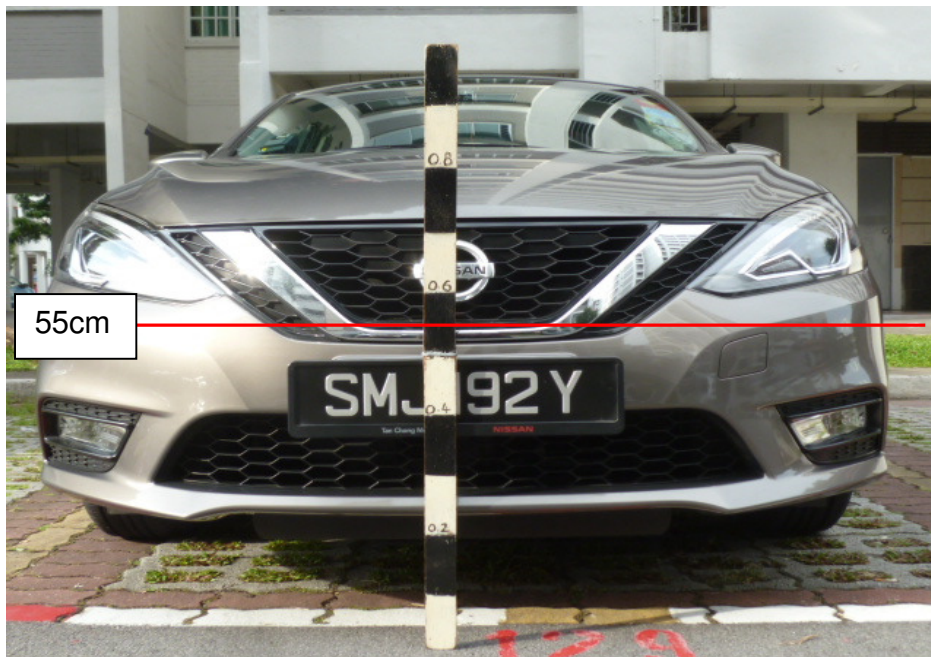
Photo 16 shows the height measurement being conducted on the frontal portion of the Nissan. The height above ground level of the Nissan's front bumper where the paint graze marks were found was measured to be approximately 55cm.
