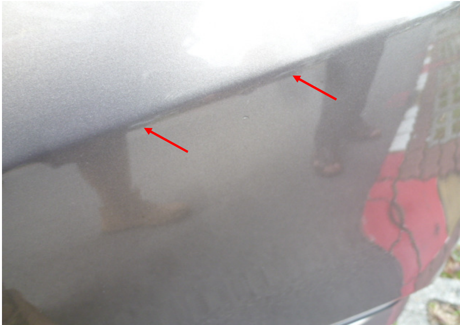
Photo 9 shows a close up view of the paint graze marks on the left portion of the Nissan's front bumper (arrowed). Mr Wong informed us that the paint graze marks were pre- existing damages.
