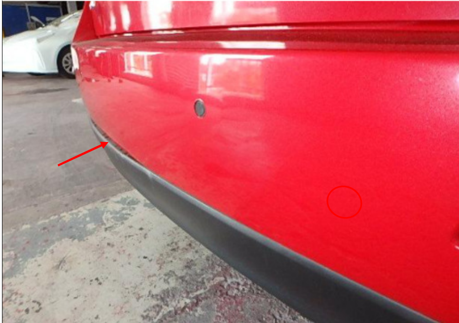
Photo 2 shows upon closer examination of the lower portion of the rear bumper, we observed a slight dislodgement of the lower rear bumper cover (arrowed) of the Taxi.
