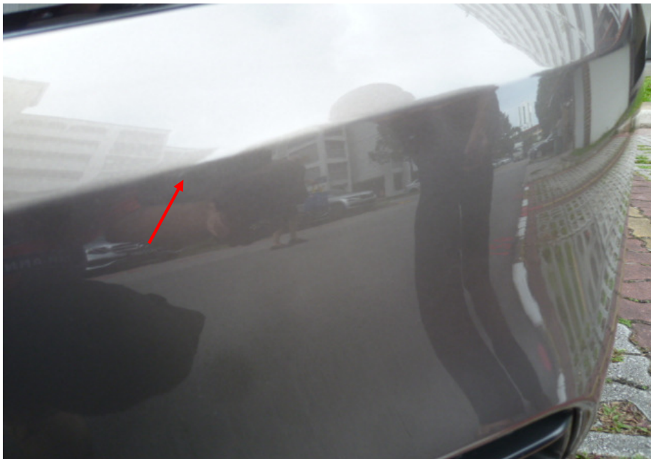
Photo 8 shows a closer view of the paint graze marks on the left portion of the Nissan's front bumper (arrowed).
