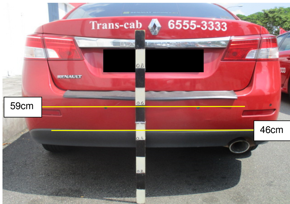
Photo 15 shows the height measurement being conducted on the rear portion of the Taxi (using a similar make and model). The height above ground level of the Taxi's lower rear bumper cover where the dislodgement was found was measured to be approximately 46cm. The height above ground level of the Taxi's rear bumper where the paint graze marks were found was measured to be approximately 59cm.
