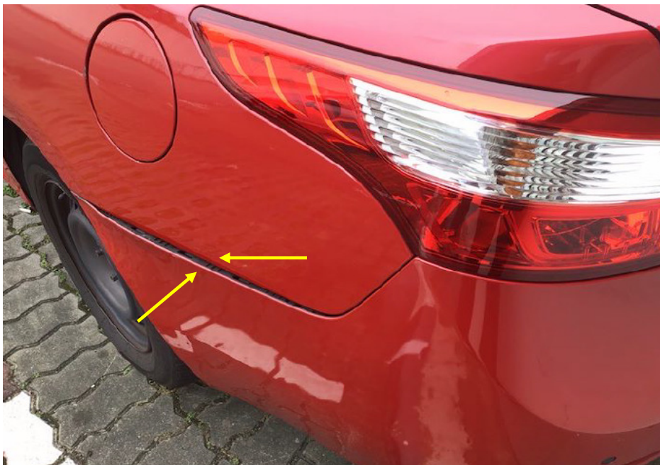
Photo 5 shows the left corner edge of the rear bumper of the Taxi which was taken at the time of reporting. We observed that the rear bumper was slightly dislodged at the left corner edge (arrowed).
