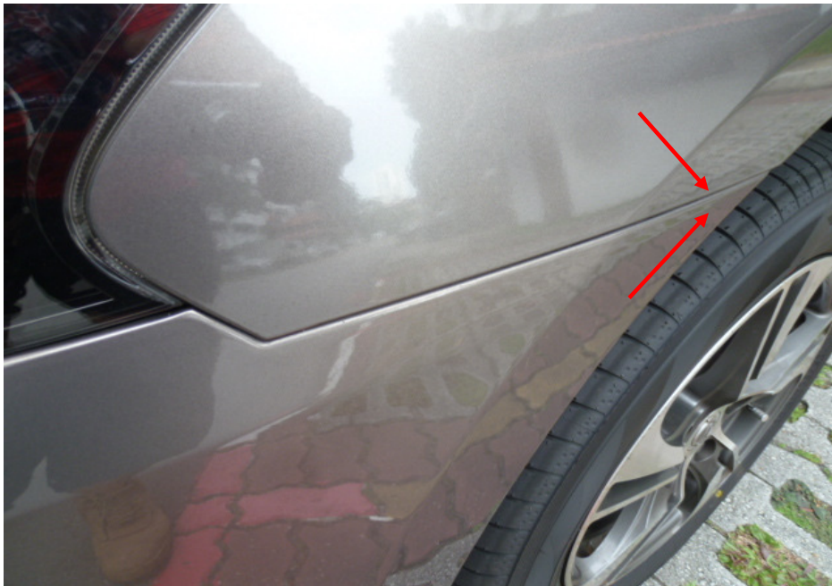
Photo 10 shows a closer view of the left corner edge of the front bumper of the Nissan. We observed no misalignment at the corner edges (red arrows).
