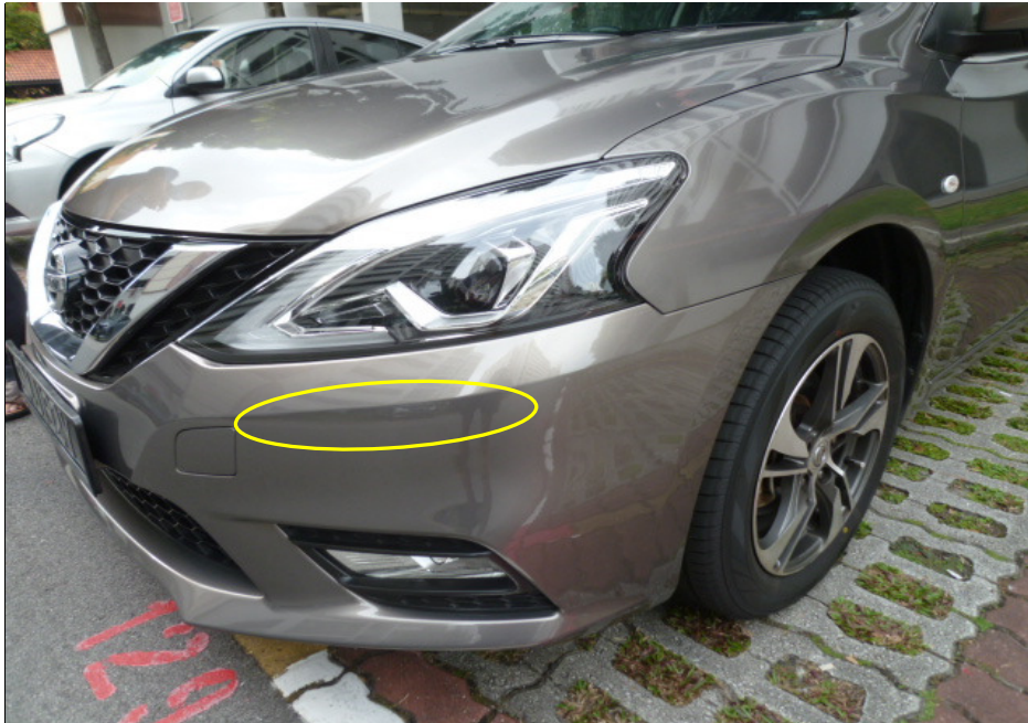
Photo 7 shows upon closer visual examination, we observed paint graze marks on the left portion of the Nissan's front bumper (circled).
