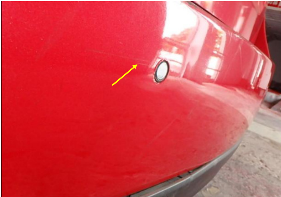
Photo 4 shows a close up view of the paint graze marks (arrowed) at the left portion of the Taxi's rear bumper.
