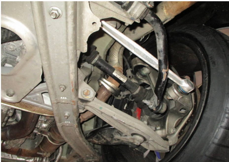
Photo 31 shows a general view of the control arms and linkages at the rear right wheel of the Motor Car. I did not observe any fluid leak and/or fluid stain on the underside of the Motor Car. All of the Motor Car's undercarriage components were observed to be intact and secured in an appropriate manner.
