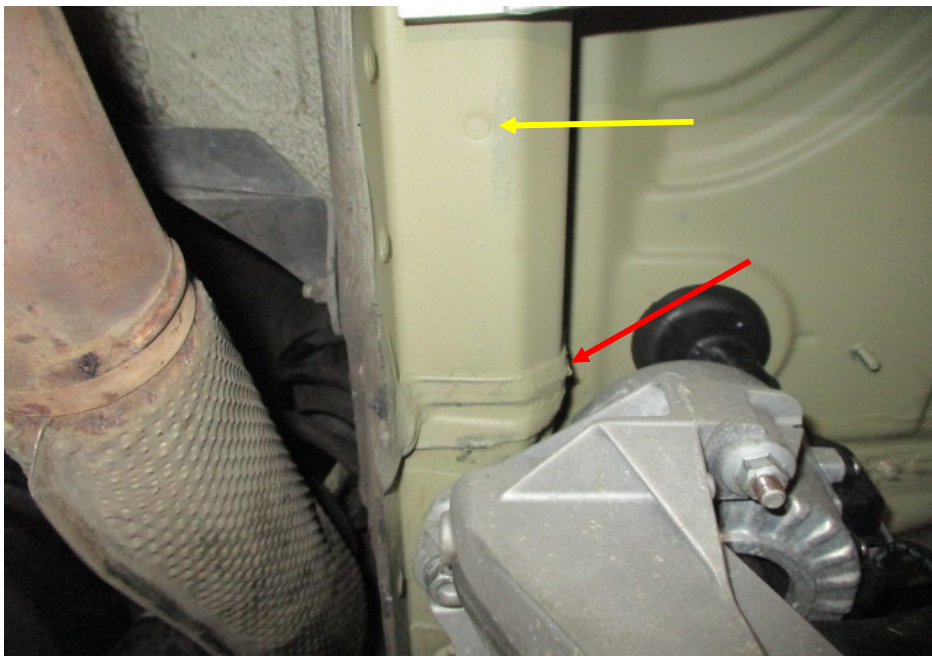
Photo 39 shows the chassis/structural body at the underside rear left of the Motor Car. I did not find any weld marks other than original spot weld marks (yellow arrow) on the chassis/structural body of the Motor Car. The original factory sealant (red arrow) at the joints along the chassis/structural body was also untouched. In general, the Motor Car's chassis/structural body was found to be originally fitted.
