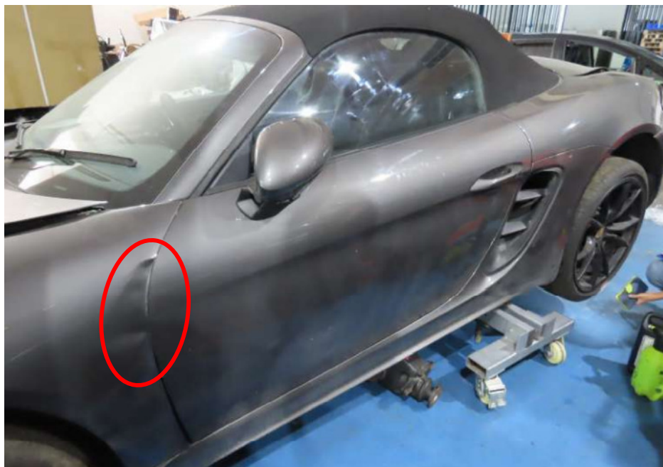
Photo 4 shows the left side body of the Motor Car (photograph provided to me). The Motor Car's front left fender was observed to be damaged (circled).
