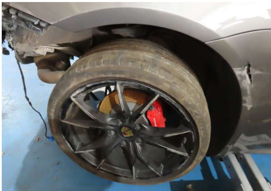
Photo 6 shows the damage to the rear right wheel rim and right side rocker panel garnish of the Motor Car (photograph provided to me). The orientation of the Motor Car's rear right wheel indicates damage to its rear right undercarriage parts. Undercarriage parts that may possibly be damaged include the rear right lower arm, rear right upper arm, rear right shock absorber and rear right knuckle arm amongst others.
