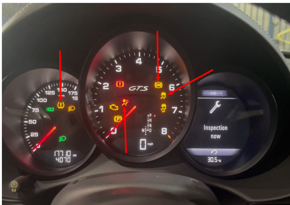
Photo 28 shows the warning lights for the various electronic safety features appearing on the instrument panel of the Motor Car during its self-test when the engine is cranked, in particular the ABS, SRS, TPM and TCS lights (arrowed).
