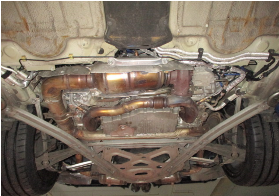
Photo 36 shows the Motor Car's catalytic converters. My examination of the Motor Car's exhaust system revealed no sign(s) or indication(s) of any cut or weld marks along its exhaust pipes, on its catalytic converters and on its rear mufflers.
