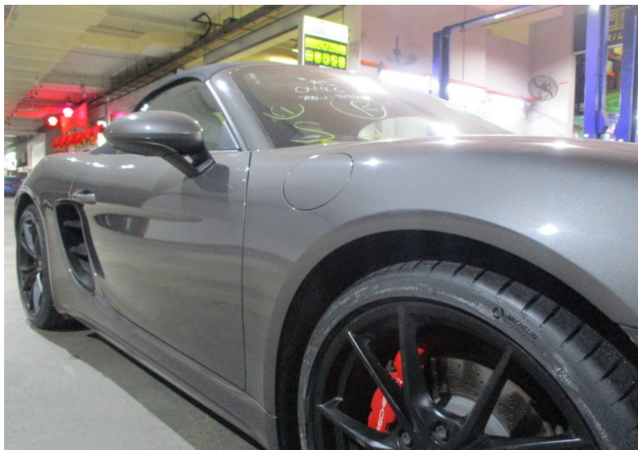
Photo 12 shows a closer view of the Motor Car's front right fender, petrol filler outer cover and front right door. The body parts at the front right portion of the Motor Car were visually examined and it was observed that the repair/restoration works carried out to the damaged area of the Motor Car (refer to photograph 1 & 2 above) were reasonably adequate and in order.
