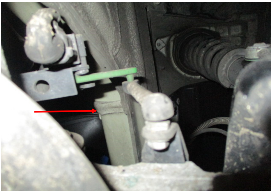
Photo 41 shows the chassis/structural body at the underside front right of the Motor Car. The original factory sealant (arrowed) at the joints along the chassis/structural body was observed to be untouched. In general, I had found the chassis/structural body of the Motor Car to be originally fitted.
