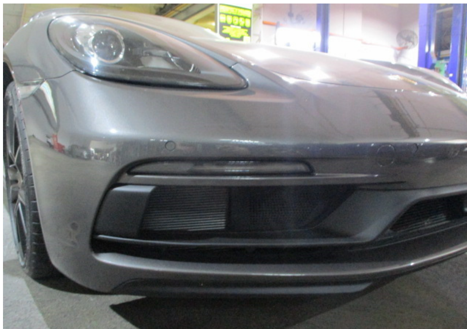
Photo 10 shows a closer view of the Motor Car's front bumper, front bumper lower grille, front right day light, front right headlamp and front right aircon condenser. The body parts at the front right portion of the Motor Car were visually examined and it was observed that the repair/restoration works carried out to the damaged area of the Motor Car (refer to photograph 1 & 2 above) were reasonably adequate and in order.
