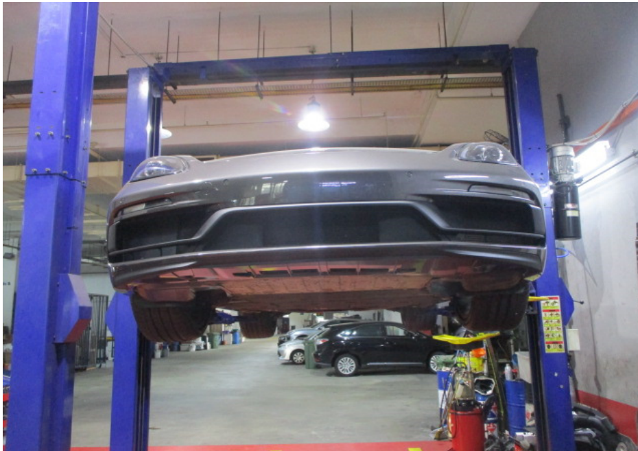
Photo 30 shows the Motor Car hoisted up for checks on its undercarriage. There was no sign(s) or indication(s) of fluid leakage and/or fluid stain(s) on the underside of the Motor Car. The undercarriage components of the Motor Car were also all observed to be intact and secured in an appropriate manner.
