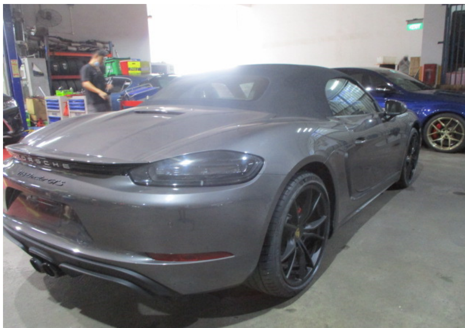
Photo 17 shows a general view of the rear right body of the Motor Car at the time of my inspection. The Motor Car was observed to be in a relatively good general condition with no loose exterior fittings observed. The body parts at the rear right portion of the Motor Car were visually examined and it was observed that the repair/restoration works carried out to the damaged area of the Motor Car (refer to photograph 5 & 6 above) were reasonably adequate and in order.
