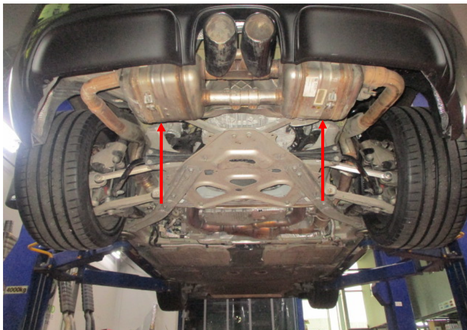
Photo 35 shows the Motor Car's rear mufflers (arrowed). My examination of the Motor Car's exhaust system revealed no sign(s) or indication(s) of any cut or weld marks along its exhaust pipes, on its catalytic converters and on its rear mufflers.
