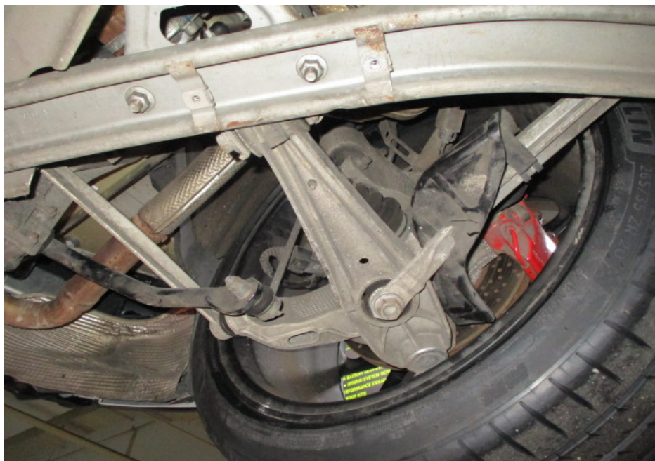
Photo 32 shows a general view of the control arms and linkages at the rear left wheel of the Motor Car. I did not observe any fluid leak and/or fluid stain on the underside of the Motor Car. All of the Motor Car's undercarriage components were observed to be intact and secured in an appropriate manner.
