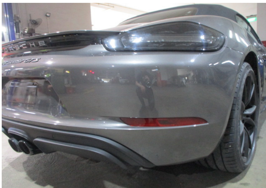
Photo 19 shows a closer view of the Motor Car's rear bumper, rear bumper right reflector, rear bumper lower cover and rear right taillamp. The body parts at the rear right portion of the Motor Car were visually examined and it was observed that the repair/restoration works carried out to the damaged area of the Motor Car (refer to photograph 5 above) were reasonably adequate and in order.
