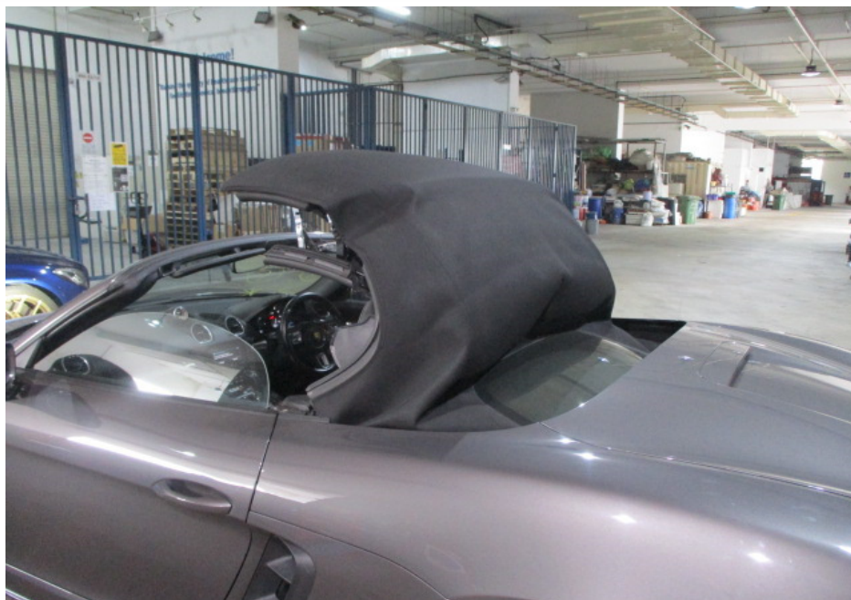
Photo 26 shows the Motor Car's soft top roof being tested. It was observed that as a safety feature, the soft top roof could only open and close when the Motor Car was in a stationary position. When in an open position, the soft top roof is completely folded into its rear compartment with no parts protruding out of the Motor Car's body. The soft top roof was also found adequately secured to the "A" pillar after closing.
