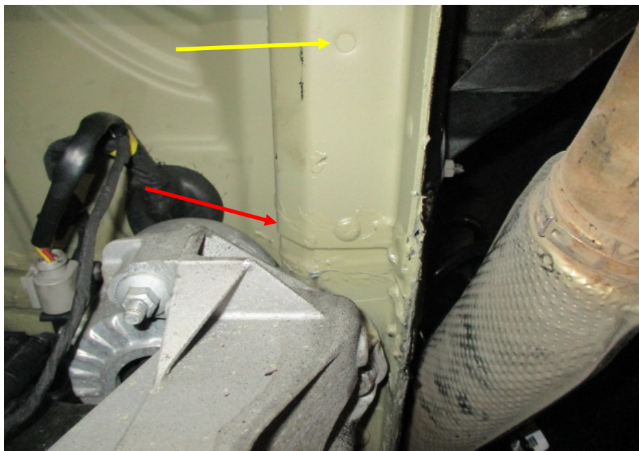
Photo 40 shows the chassis/structural body at the underside rear right of the Motor Car. The end section of the chassis/structural body at the underside rear right was found with signs of repair. However, the rear right chassis of the Motor Car was still observed to be an originally fitted part given that original factory sealant (red arrow) and original spot weld mark (yellow arrow) were seen on the rear right chassis.
