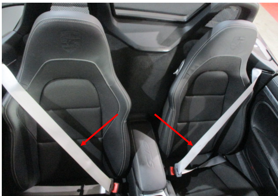
Photo 25 shows the seats of the Motor Car. All the seats of the Motor Car were secured via seat rails to the floorboard. They were also fitted with a retractable seat belt reel and a pre-tensioner. The seat belts (arrowed) were tested and were able to be fastened into the respective pre-tensions that were fitted on the side of each individual seat.
