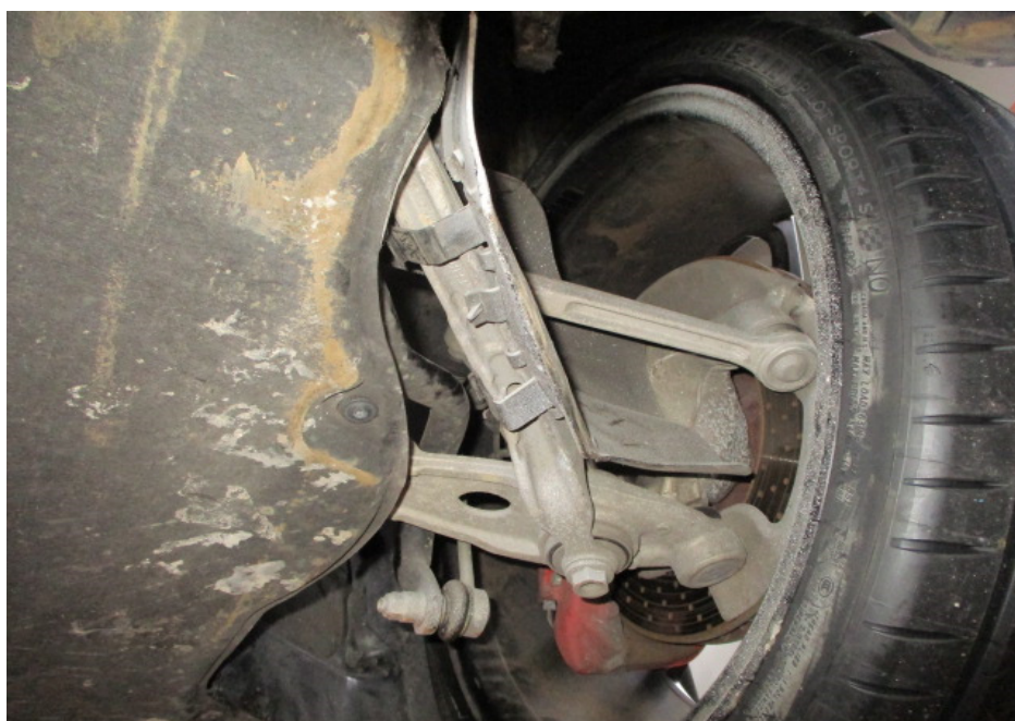
Photo 33 shows the various undercarriage components at the front left wheel of the Motor Car. The mechanical components, control arms and linkages were all found to be intact and secured in an appropriate manner.
