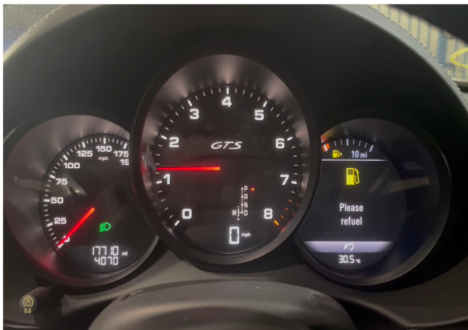
Photo 29 shows the respective warning lights no longer illuminated, indicating that there is no fault detected to the ABS, SRS, TPM and TCS systems of the Motor Car during the self-test. These electronic systems were hence in working condition at the time of my inspection.
