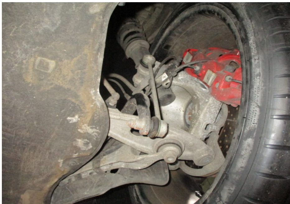
Photo 34 shows the various undercarriage components at the front right wheel of the Motor Car. The mechanical components, control arms and linkages were all found to be intact and secured in an appropriate manner. I also did not observe any fluid leak and/or fluid stain on the underside of the Motor Car.
