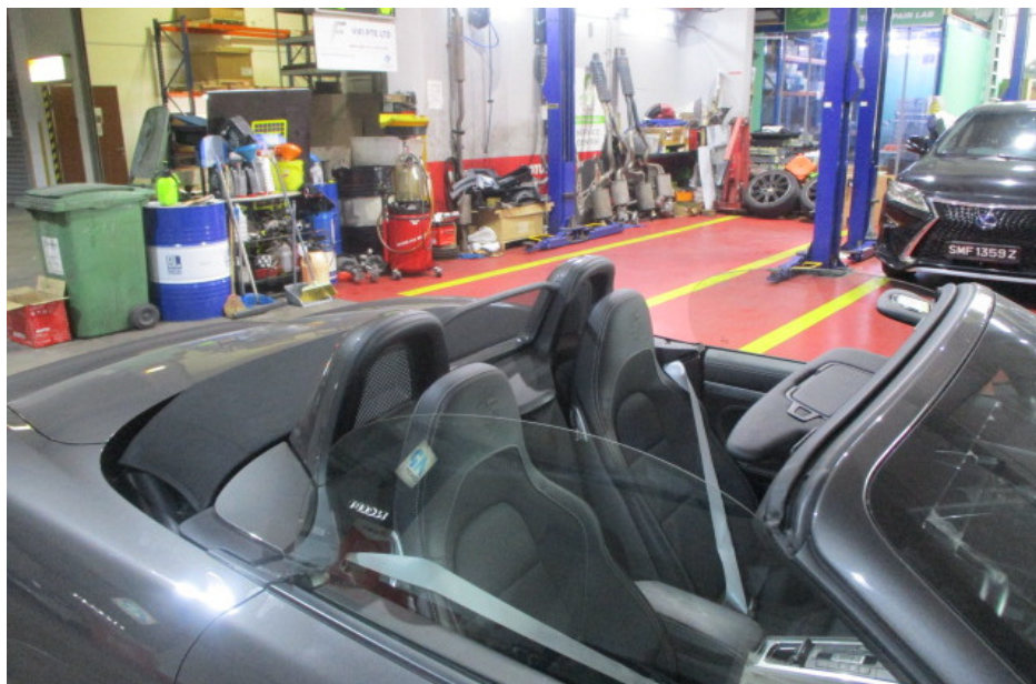
Photo 27 shows the Motor Car with its soft top roof in an open position. It was observed that as a safety feature, the soft top roof could only open and close when the Motor Car was in a stationary position. When in an open position, the soft top roof is completely folded into its rear compartment with no parts protruding out of the Motor Car's body. The soft top roof was also found adequately secured to the "A" pillar after closing.
