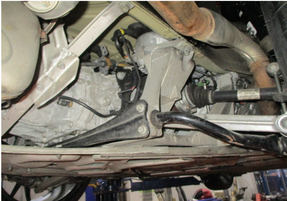
Photo 38 shows another view of the Motor Car's engine compartment. The engine compartment was at the rear underside of the Motor Car. The various parts and components inside the engine compartment were all observed to be intact and properly fitted. There was also no sign(s) or indication(s) of fluid leak and/or fluid stain found inside the engine compartment.
