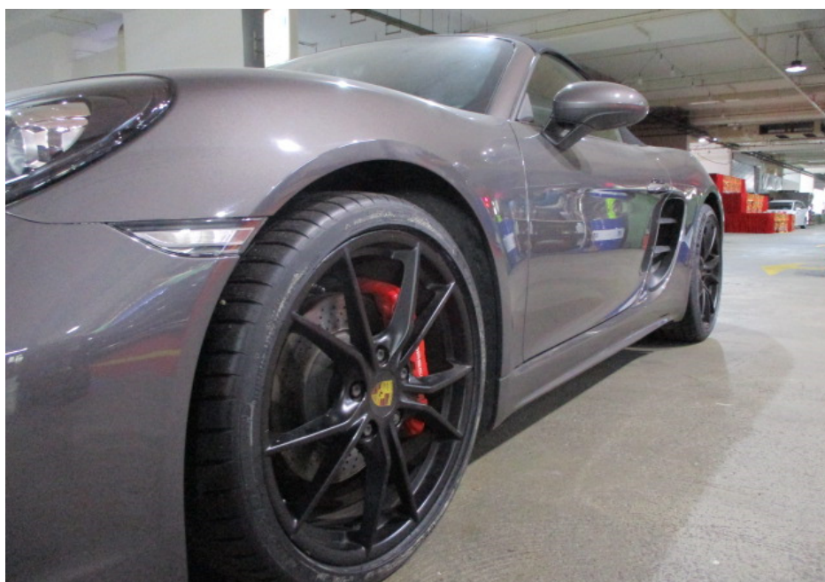
Photo 15 shows a closer view of the Motor Car's front bumper, front left signal lamp, front left fender and front left wheel rim. The body parts at the front left portion of the Motor Car were visually examined and it was observed that the repair/restoration works carried out to the damaged area of the Motor Car (refer to photograph 3 & 4 above) were reasonably adequate and in order.
