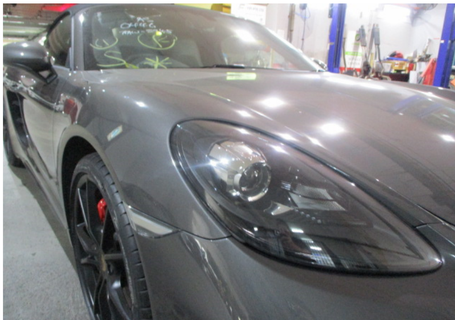
Photo 11 shows a closer view of the Motor Car's front bonnet, front right headlamp, front right fender and front right signal lamp. The body parts at the front right portion of the Motor Car were visually examined and it was observed that the repair/restoration works carried out to the damaged area of the Motor Car (refer to photograph 1 & 2 above) were reasonably adequate and in order.
