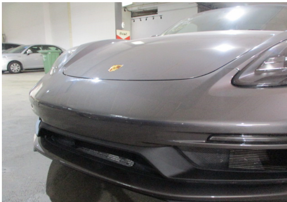
Photo 14 shows a closer view of the Motor Car's front bumper, front bumper lower grille, front left day light and front bonnet. The body parts at the front left portion of the Motor Car were visually examined and it was observed that the repair/restoration works carried out to the damaged area of the Motor Car (refer to photograph 3 above) were reasonably adequate and in order.
