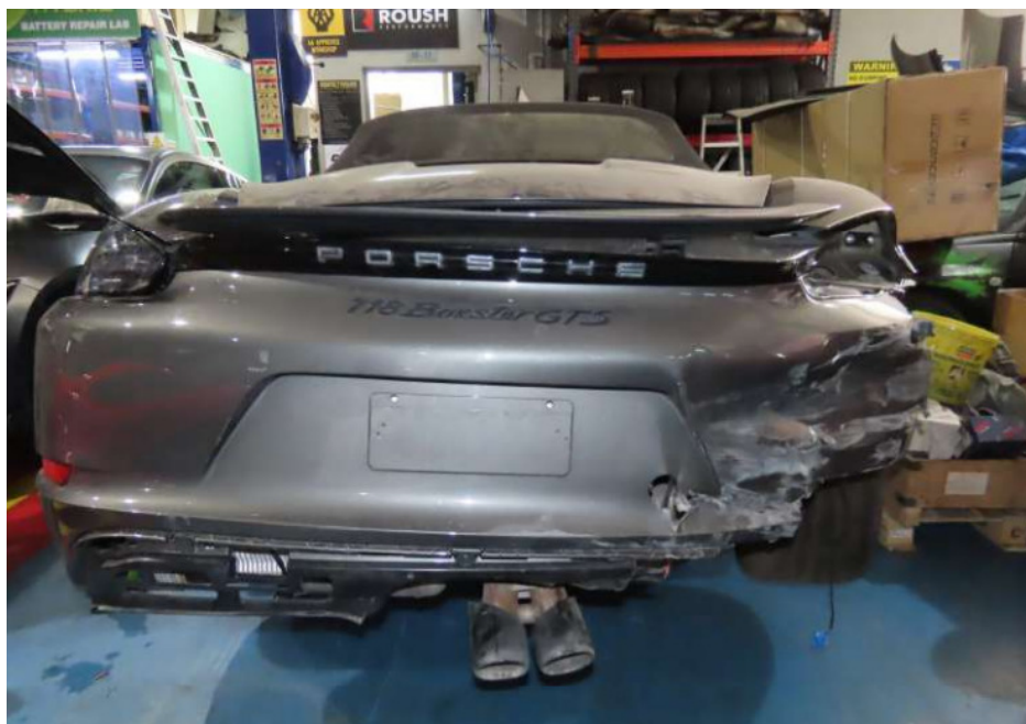
Photo 5 shows the rear body of the Motor Car (photograph provided to me). Apart for the front right portion and left front portion, the Motor Car had also sustained damages at its rear right portion. Body parts damaged include the rear bumper, rear bumper lower cover, rear bumper tow hook cover, rear bumper right reflector, rear exhaust, rear bootlid and rear right taillamp amongst others.
