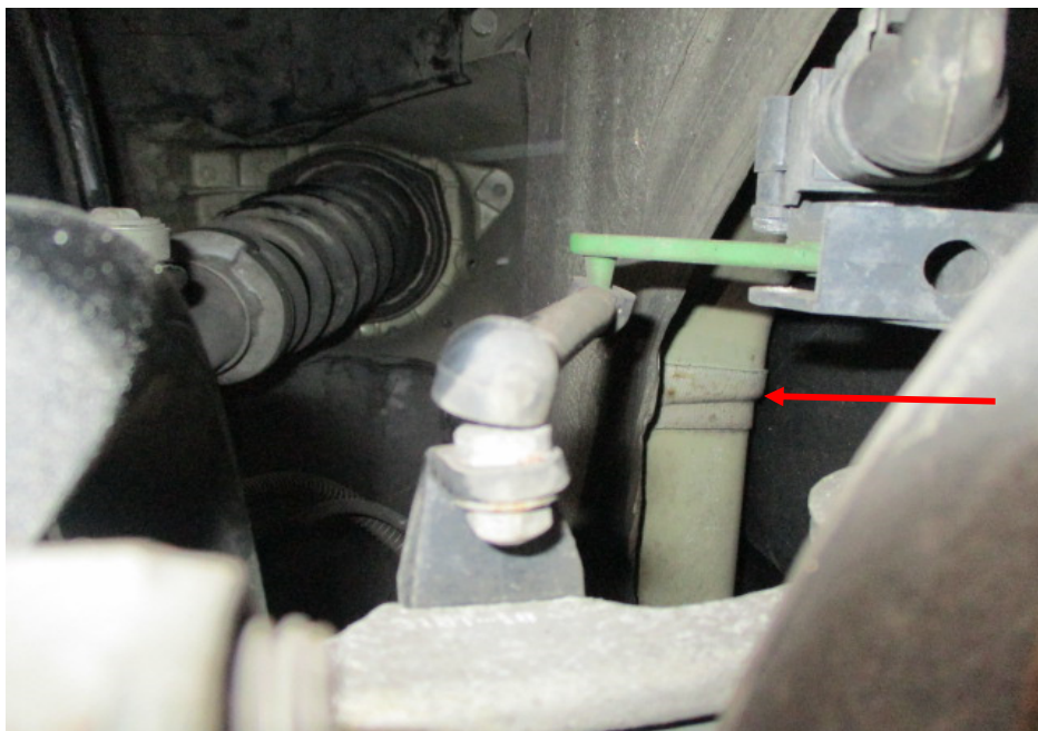
Photo 42 shows the chassis/structural body at the underside front left of the Motor Car. The original factory sealant (arrowed) at the joints along the chassis/structural body was observed to be untouched. In general, I had found the chassis/structural body of the Motor Car to be originally fitted.
