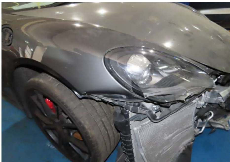
Photo 2 shows a closer view of the damaged front right fender, front right headlamp, front right aircon condenser and front right radiator of the Motor Car (photograph provided to me).
