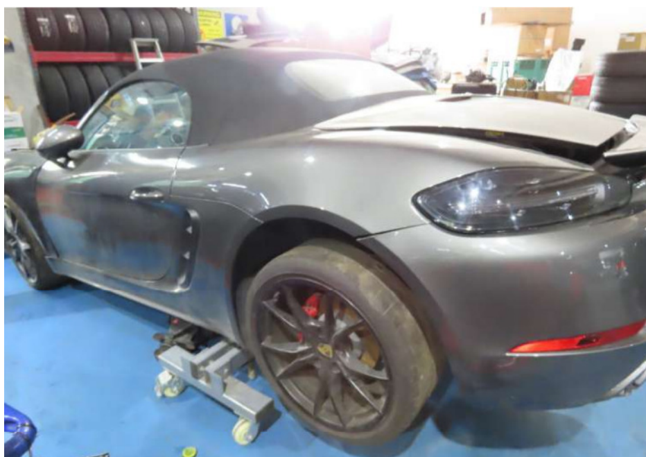
Photo 7 shows the rear left body of the Motor Car (photograph provided to me). No physical damage was observed to the rear left portion of the Motor Car.
