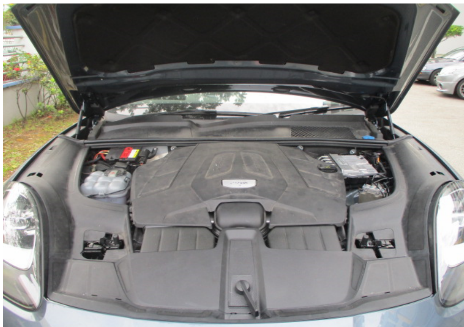
Photo 15 shows a general view of the engine compartment of the Motor Car at the time of my inspection. The various parts and components inside the engine compartment were all observed to be intact and properly fitted. There was also no sign(s) or indication(s) of fluid leak and/or fluid stain found inside the engine compartment.
