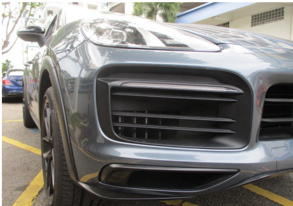
Photo 7 shows a closer view of the Motor Car's front bumper, front bumper right grille, front bumper right lower grille, front right day light and front right headlamp at the time of my inspection. The body parts at the frontal portion of the Motor Car were visually examined and it was observed that the repair/restoration works carried out to the damaged area of the Motor Car (refer to photograph 1 - 3 above) were reasonably adequate and in order.
