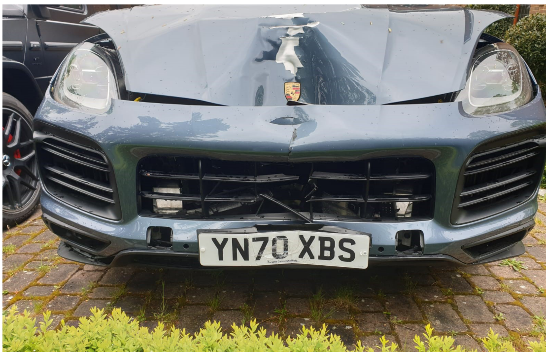
Photo 3 shows the frontal body of the Motor Car (photograph provided to me). The photographs provided to me had showed damage to the frontal portion of the Motor Car. Body parts damaged include the front bumper, front bumper reinforcement, front bumper centre lower grille, front bumper tow hook covers, front sensor, radiator grille, front bonnet and front bonnet lock amongst others.
