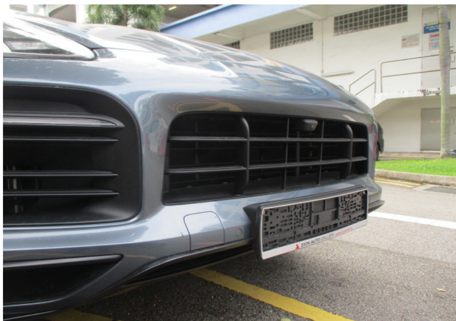
Photo 8 shows a closer view of the Motor Car's front bumper, front bumper tow hook cover, front bumper centre lower grille and radiator grille. The body parts at the frontal portion of the Motor Car were visually examined and it was observed that the repair/restoration works carried out to the damaged area of the Motor Car (refer to photograph 1 - 3 above) were reasonably adequate and in order.
