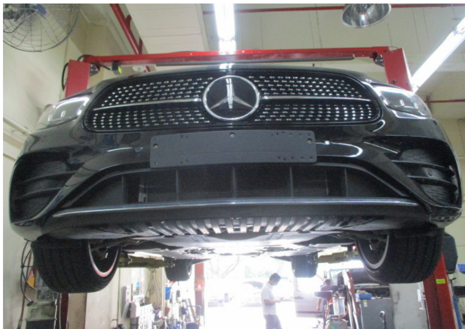
Photo 21 shows the Motor Car hoisted up for checks on its undercarriage. There was no sign(s) or indication(s) of fluid leakage and/or fluid stain(s) on the underside of the Motor Car. The undercarriage components of the Motor Car were also all observed to be intact and secured in an appropriate manner.
