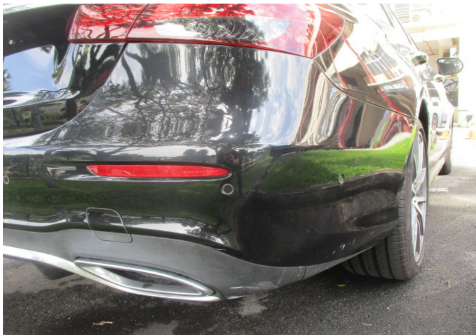
Photo 8 shows a closer view of the Motor Car's rear bumper, rear bumper lower cover, rear bumper right reflector and rear bumper sensors at the time of my inspection. The body parts at the right rear portion of the Motor Car were visually examined and it was observed that the repair/restoration works carried out to the damaged area of the Motor Car (refer to photograph 1 above) were reasonably adequate and in order.
