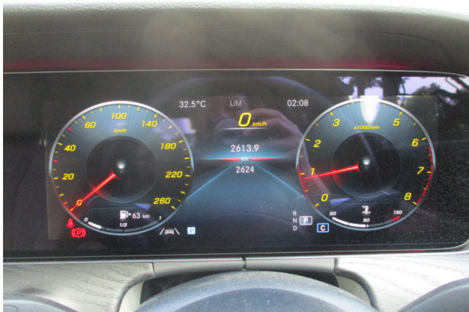
Photo 20 shows the respective warning lights no longer illuminated, indicating that there is no fault detected to the ABS, SRS, EPS and TCS systems of the Motor Car during the self-test. These electronic systems were hence in working condition at the time of my inspection.
