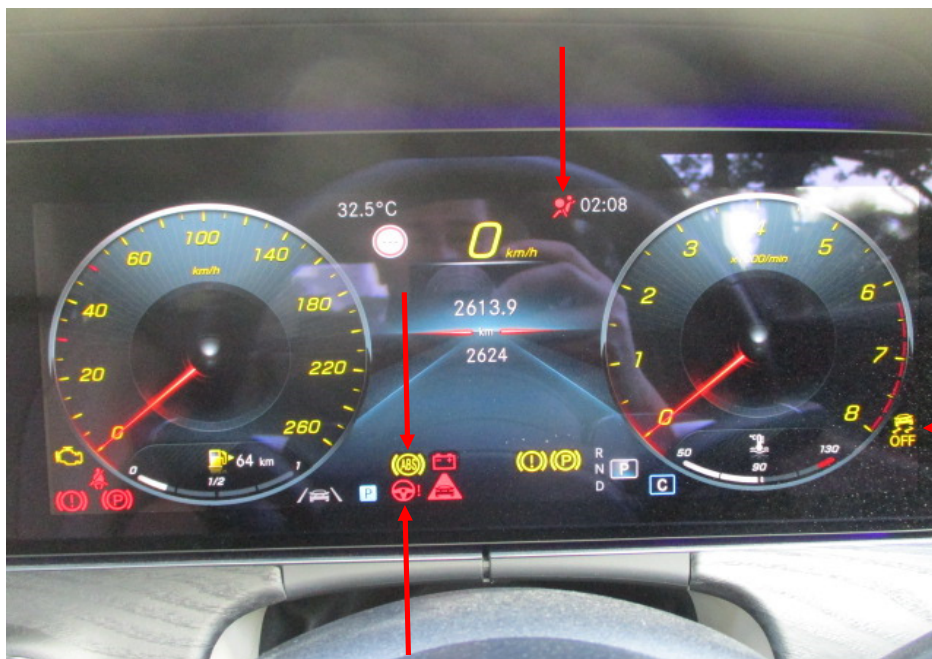
Photo 19 shows the warning lights for the various electronic safety features appearing on the instrument panel of the Motor Car during its self-test when the engine is cranked, in particular the ABS, SRS, EPS and TCS lights (arrowed).
