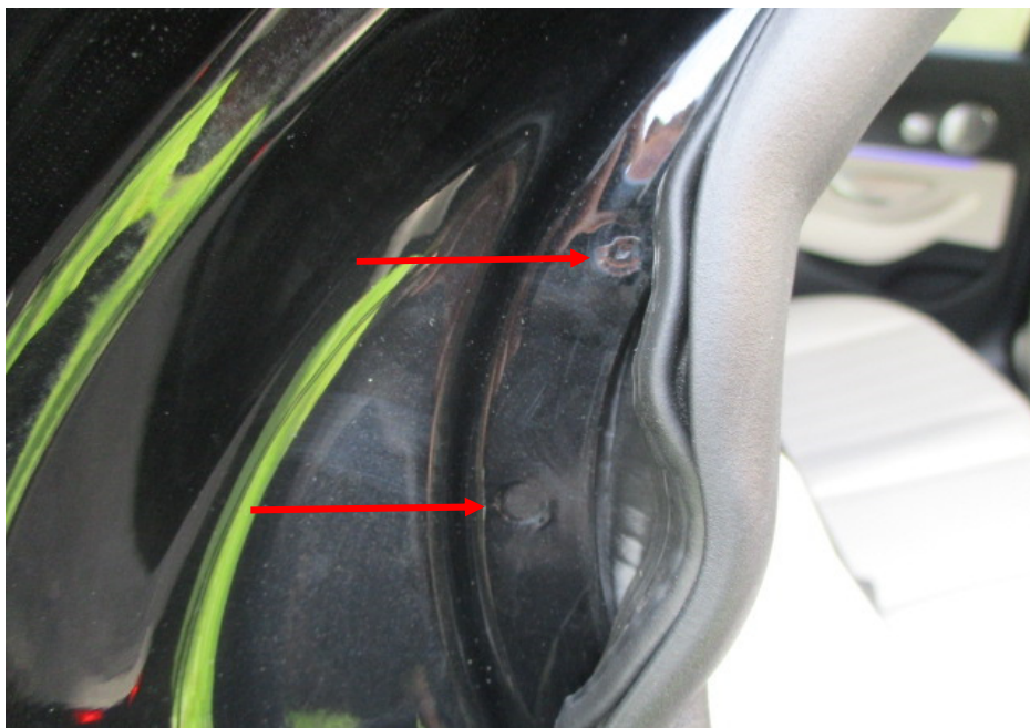
Photo 34 shows the right side “C” pillar of the Motor Car. I did not find any weld marks other than original spot weld marks (arrowed) on the right side “C” pillar of the Motor Car which, indicates that there was no re-welding works carried out. In general, I had found all the non-detachable body panels of the Motor Car to be originally fitted at the time of my inspection.
