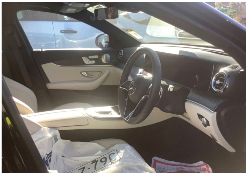
Photo 5 shows the front interior compartment of the Motor Car (photograph provided to me). Parts and components within the interior compartment were observed to be unaffected. The airbags of the Motor Car were also not deployed as seen from the photographs that were provided to me.
