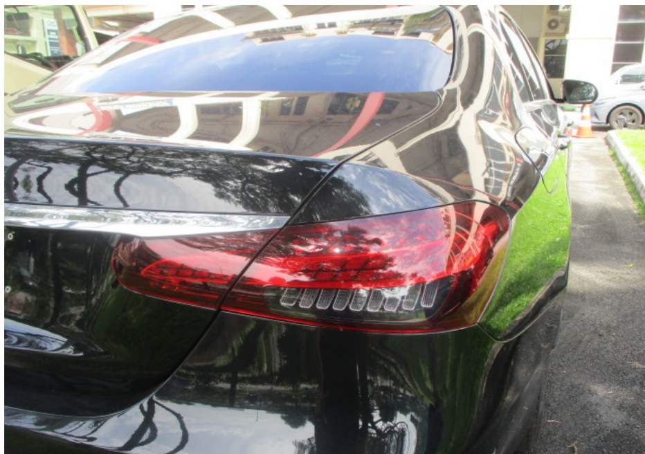
Photo 9 shows a closer view of the Motor Car's rear bootlid, rear right bootlid lamp and rear right taillamp at the time of my inspection. The body parts at the right rear portion of the Motor Car were visually examined and it was observed that the repair/restoration works carried out to the damaged area of the Motor Car (refer to photograph 1 above) were reasonably adequate and in order.
