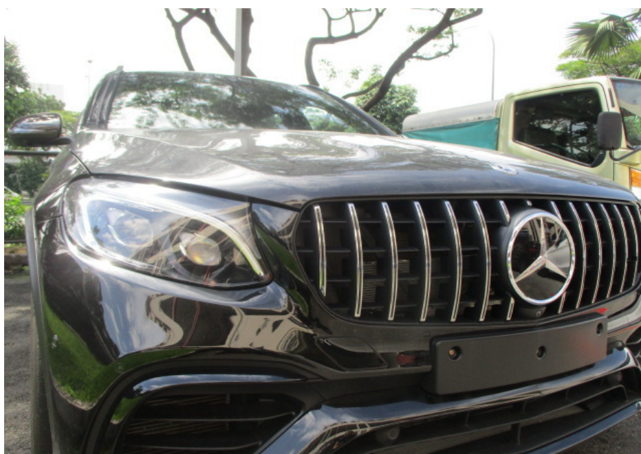
Photo 12 shows a closer view of the Motor Car's front bumper, front bumper right lower grille, front right headlamp and radiator grille. The body parts at the frontal portion of the Motor Car were visually examined and it was observed that the repair/restoration works carried out to the damaged area of the Motor Car (refer to photograph 2 above) were reasonably adequate and in order.
