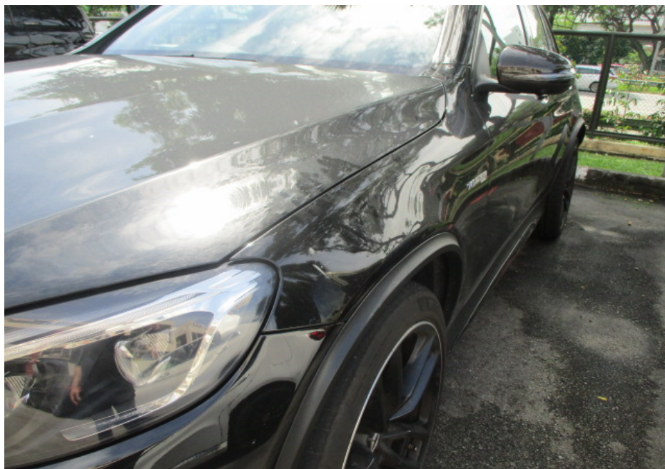
Photo 9 shows a closer view of the Motor Car's front bonnet, front left headlamp, front left fender and front left fender wheel arc garnish. The body parts at the front left portion of the Motor Car were visually examined and it was observed that the repair/restoration works carried out to the damaged area of the Motor Car (refer to photograph 1 above) were reasonably adequate and in order.
