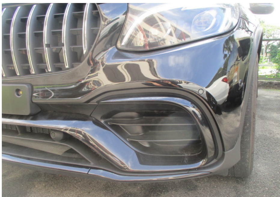
Photo 10 shows a closer view of the Motor Car's front bumper, front bumper left lower grille, front bumper centre lower grille and radiator grille. The body parts at the front left portion of the Motor Car were visually examined and it was observed that the repair/restoration works carried out to the damaged area of the Motor Car (refer to photograph 1 above) were reasonably adequate and in order.
