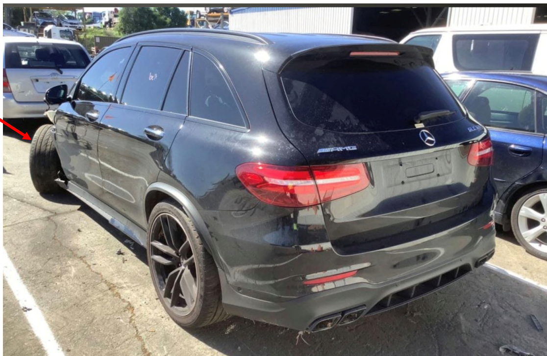
Photo 4 shows the rear left body of the Motor Car (photograph provided to me). No physical damage was observed to the rear left portion of the Motor Car. The orientation of the front left wheel (arrowed) and front right wheel (refer to photograph 3 above) indicates damage to the front left undercarriage parts of the Motor Car.
