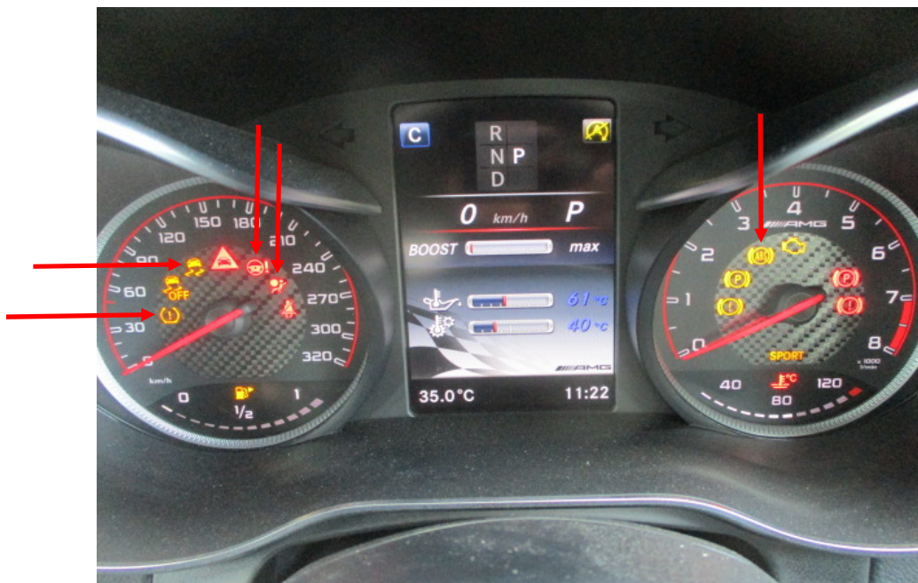
Photo 20 shows the warning lights for the various electronic safety features appearing on the instrument panel of the Motor Car during its self-test when the engine is cranked, in particular the ABS, SRS, EPS, TPM and TCS lights (arrowed).
