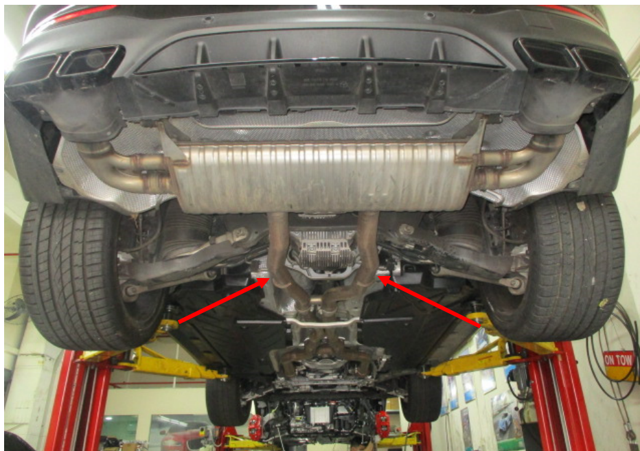
Photo 27 shows the rear section of the Motor Car's exhaust system. My examination of the Motor Car's exhaust system revealed no sign(s) or indication(s) of any cut or weld marks along its exhaust pipes (arrowed), on its rear muffler and on its catalytic converters.
