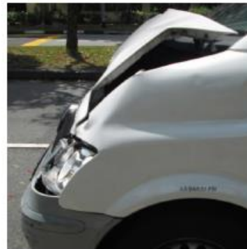
Figure C-5: Close up Damage on the front of MID46356
