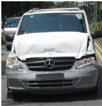
Figure C-5: Close up Damage on the front of MID46356
