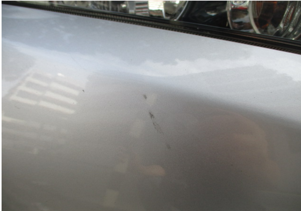
Photo 10 shows a close up view of the relatively faint grazed mark that I had observed on the Insured Vehicle's front bumper, at the area below the front right headlamp.
