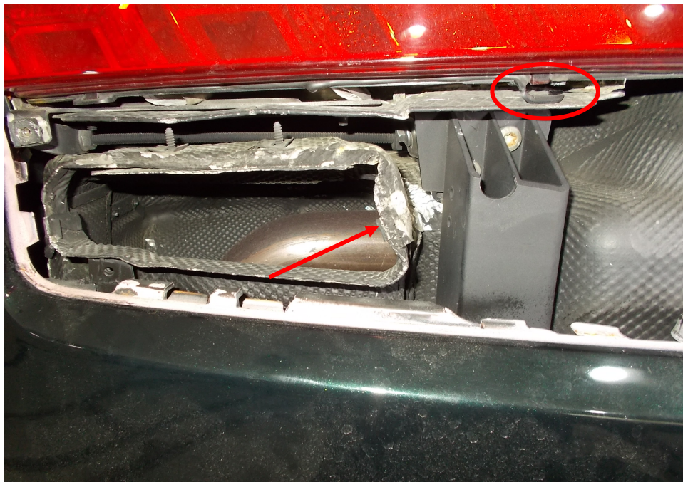
Photo 6 shows the damage to the rear left taillamp of the Third Party Vehicle at the time of physical inspection by LKK Auto Consultants Pte Ltd. This was after the front bumper grille was removed. The mounting loop of the rear left taillamp was observed to be broken (circled). The heat shield for the rear left exhaust was also observed to be bent (arrowed). These damages are induced damages.
