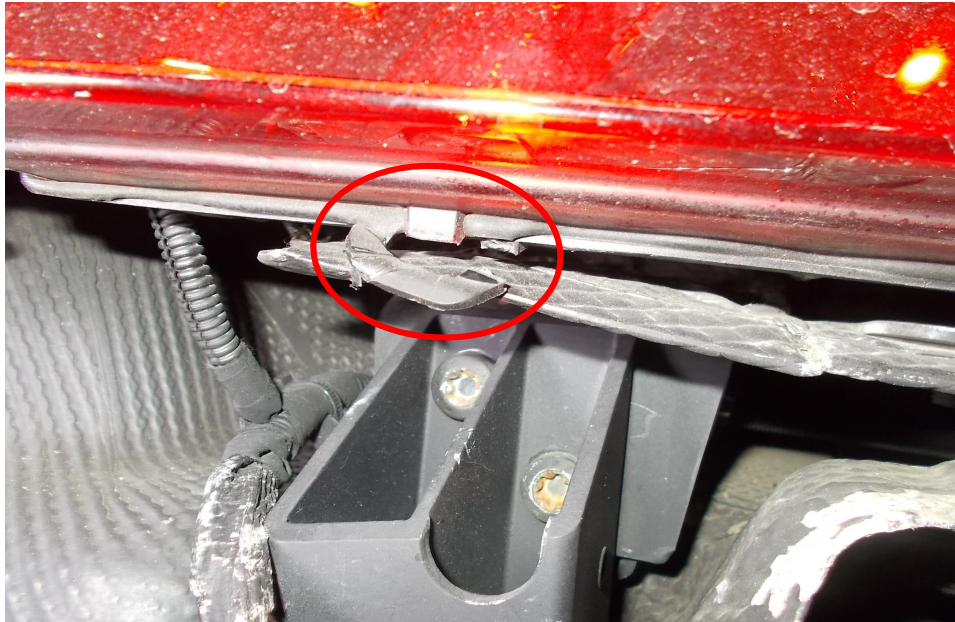
Photo 7 shows the damage to the rear right taillamp of the Third Party Vehicle at the time of physical inspection by LKK Auto Consultants Pte Ltd. This was after the front bumper grille was removed. The mounting loop of the rear right taillamp was observed to be broken (circled). This damage is an induced damage.
