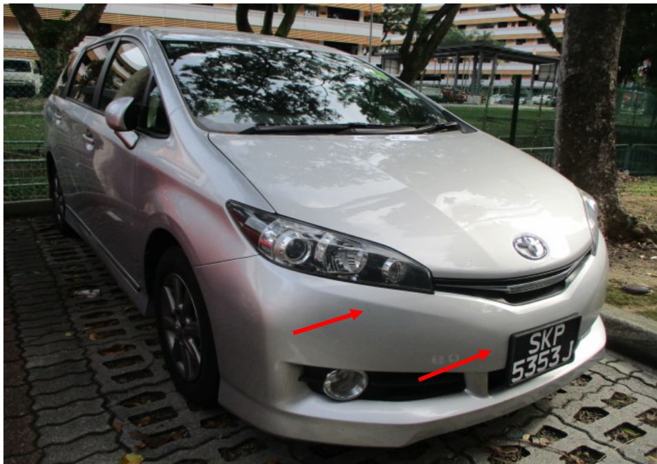
Photo 9 shows a general view of the front right body of the Insured Vehicle at the time of my physical inspection on 17 December 2021. My inspection of the Insured Vehicle had primarily focused on its front right portion. This was because the contact, if any, would have occurred at the front right portion of the Insured Vehicle. Upon close examination, I had found a relatively faint grazed mark and a semi-circular imprint mark on the right side of the Insured Vehicle's front bumper, which are highlighted by the red arrows with close up shown in the below photographs.
