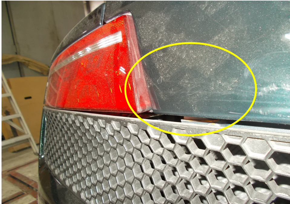
Photo 5 shows the misalignment between the rear centre top panel and the rear left taillamp of the Third Party Vehicle at the time of physical inspection by LKK Auto Consultants Pte Ltd. The rear centre top panel appears to be bent inwards at the area (circled) adjacent to the rear left taillamp.
