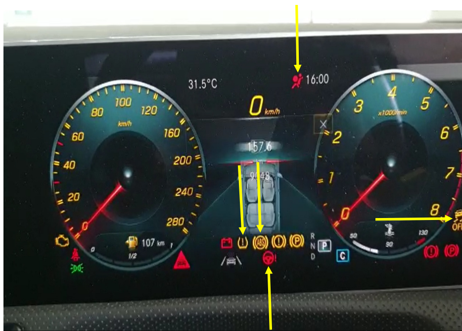
Photo 17 shows the warning lights for the various electronic safety features appearing on the instrument panel of the Motor Car during its self-test when the engine is cranked, in particular the ABS, SRS, EPS, TPM and TCS lights (arrowed).
