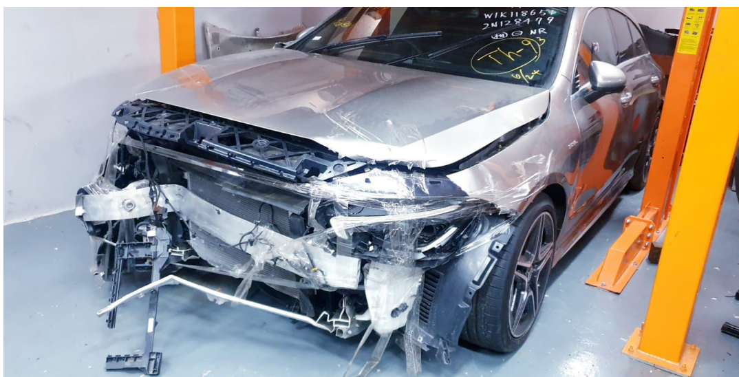
Photo 2 shows the front left body of the Motor Car (photograph provided to me). The Motor Car was observed to have sustained damage at its frontal portion. The front bumper, front bumper reinforcement, front bumper sponge, front bumper lower reinforcement, front bumper left lower grille, front bonnet, front left headlamp, front left fender, front left fender inner shield, front support panel, aircon condenser and radiator were amongst the body parts that were observed to have been damaged. The extent of damage to the frontal portion of the Motor Car would suggest to me that either the driver airbag and/or the front left passenger airbag was possibly deployed.
