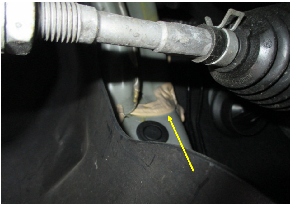
Photo 29 shows the chassis/structural body at the underside front right of the Motor Car. I did not find any weld marks other than original spot weld marks on the chassis/structural body of the Motor Car. The original factory sealant (arrowed) at the joints along the chassis/structural body was also untouched, indicating no work was done on the chassis/structural body of the Motor Car and that the chassis/structural body was originally fitted.
