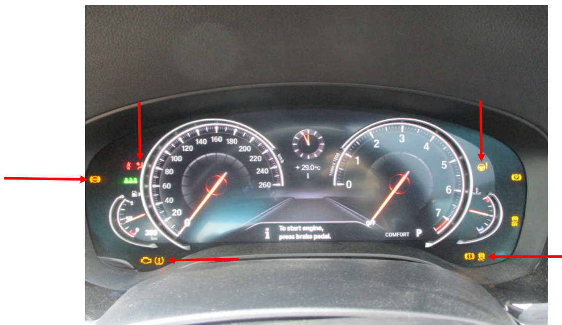
Photo 15 shows the warning lights for the various electronic safety features appearing on the instrument panel of the Motor Car during its self-test when the engine is cranked, in particular the ABS, SRS, IAS, TPM and DSC lights (arrowed).
