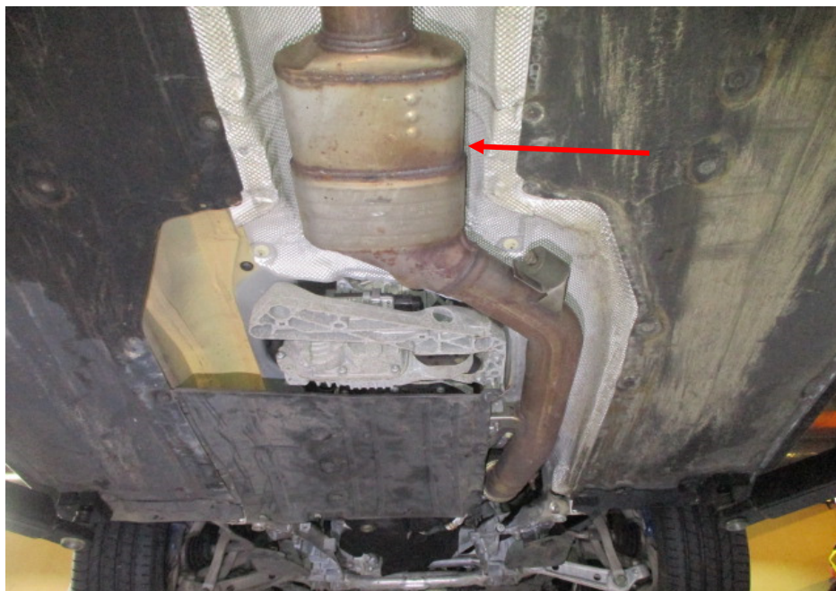
Photo 23 shows the front section of the Motor Car's exhaust system. My examination of the Motor Car's exhaust system revealed no sign(s) or indication(s) of any cut or weld marks along its exhaust pipes, on its rear muffler, on its centre resonator box (arrowed) and on its catalytic converter.
