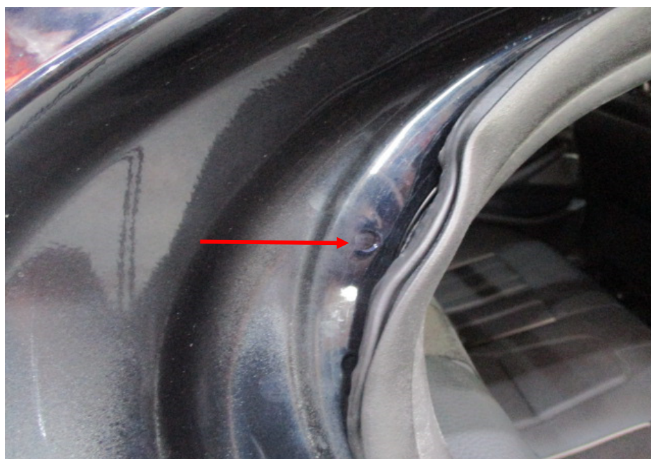
Photo 29 shows the right side "C" pillar of the Motor Car. I did not find any weld marks other than original spot weld marks (arrowed) on the right side "C" pillar of the Motor Car which, indicates that there was no re-welding works carried out. In general, I had found all the non-detachable body panels of the Motor Car to be originally fitted at the time of my inspection.
