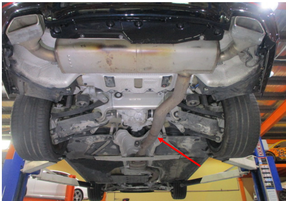
Photo 22 shows the rear section of the Motor Car's exhaust system. My examination of the Motor Car's exhaust system revealed no sign(s) or indication(s) of any cut or weld marks along its exhaust pipes (arrowed), on its rear muffler, on its centre resonator box and on its catalytic converter.
