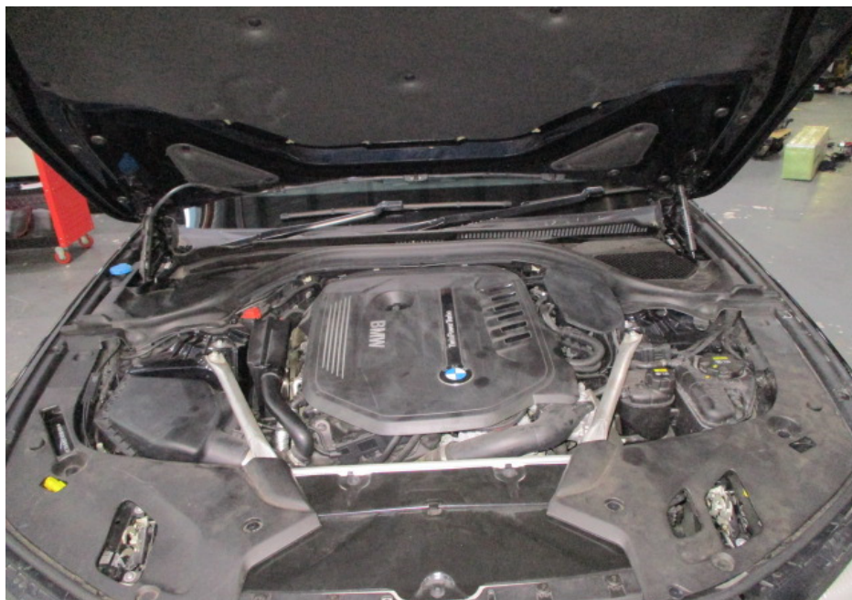
Photo 12 shows a general view of the engine compartment of the Motor Car at the time of my inspection. The various parts and components inside the engine compartment were all observed to be intact and properly fitted. There was also no sign(s) or indication(s) of fluid leak and/or fluid stain found inside the engine compartment. The repair/restoration works carried out to the various parts within the engine compartment like the front bonnet right side lock, front support panel, front support panel top centre garnish and front right headlamp top garnish amongst others, were reasonably adequate and in order.
