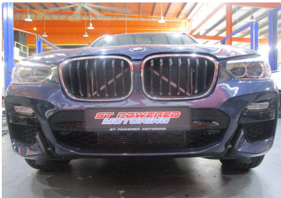
Photo 7 shows a closer view of the Motor Car's front bumper, front bumper centre lower grille, front bonnet, radiator grilles, front day lights and front headlamps. The body parts at the frontal portion of the Motor Car were visually examined and it was observed that the repair/restoration works carried out to the damaged area of the Motor Car (refer to photograph 1 – 3 above) were reasonably adequate and in order.
