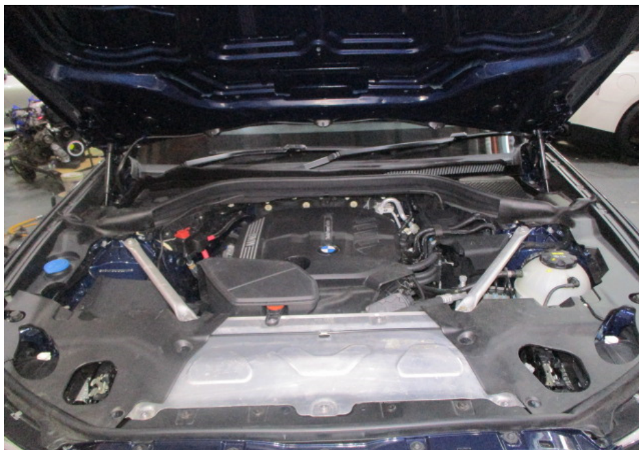
Photo 14 shows a general view of the engine compartment of the Motor Car at the time of my inspection. The various parts and components inside the engine compartment were all observed to be intact and properly fitted. There was also no sign(s) or indication(s) of fluid leak and/or fluid stain found inside the engine compartment. The repair/restoration works carried out to the various parts within the engine compartment like the front bonnet locks, front support panel, front support panel top centre garnish, aircon condenser, radiator and oil cooler amongst others, were reasonably adequate and in order.
