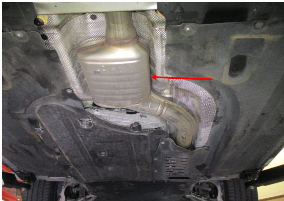
Photo 25 shows the front section of the Motor Car's exhaust system. My examination of the Motor Car's exhaust system revealed no sign(s) or indication(s) of any cut or weld marks along its exhaust pipes, on its rear muffler, on its centre resonator box (arrowed) and on its catalytic converter.
