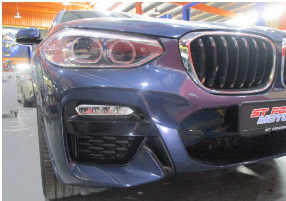
Photo 6 shows a closer view of the Motor Car's front bumper, front bumper right lower grille, front right headlamp and front right day light. The body parts at the frontal portion of the Motor Car were visually examined and it was observed that the repair/restoration works carried out to the damaged area of the Motor Car (refer to photograph 1 – 3 above) were reasonably adequate and in order.
