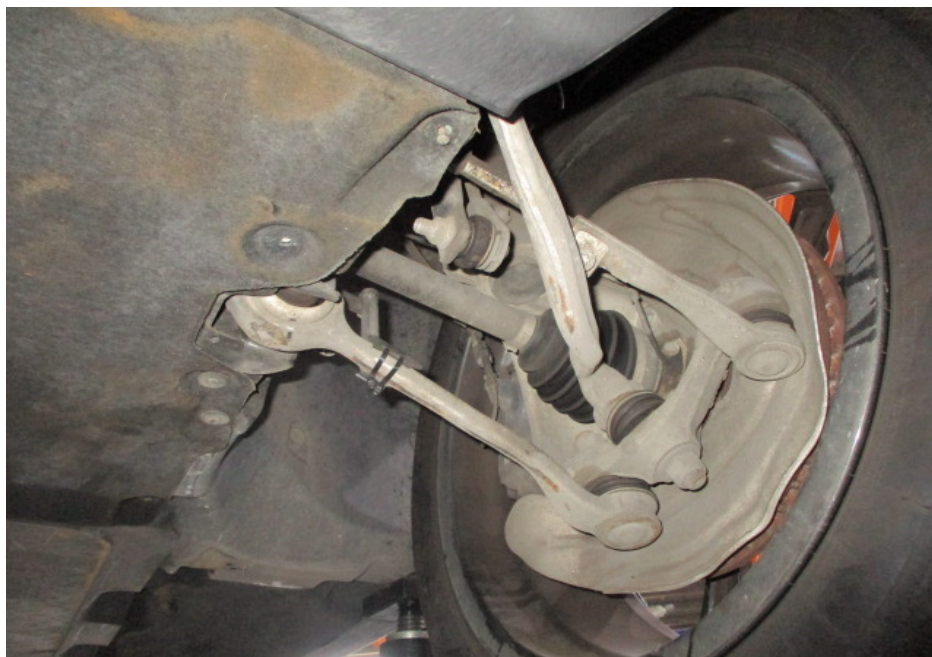
Photo 22 shows the various undercarriage components at the front left wheel of the Motor Car. The mechanical components, control arms and linkages were all found to be intact and secured in an appropriate manner.
