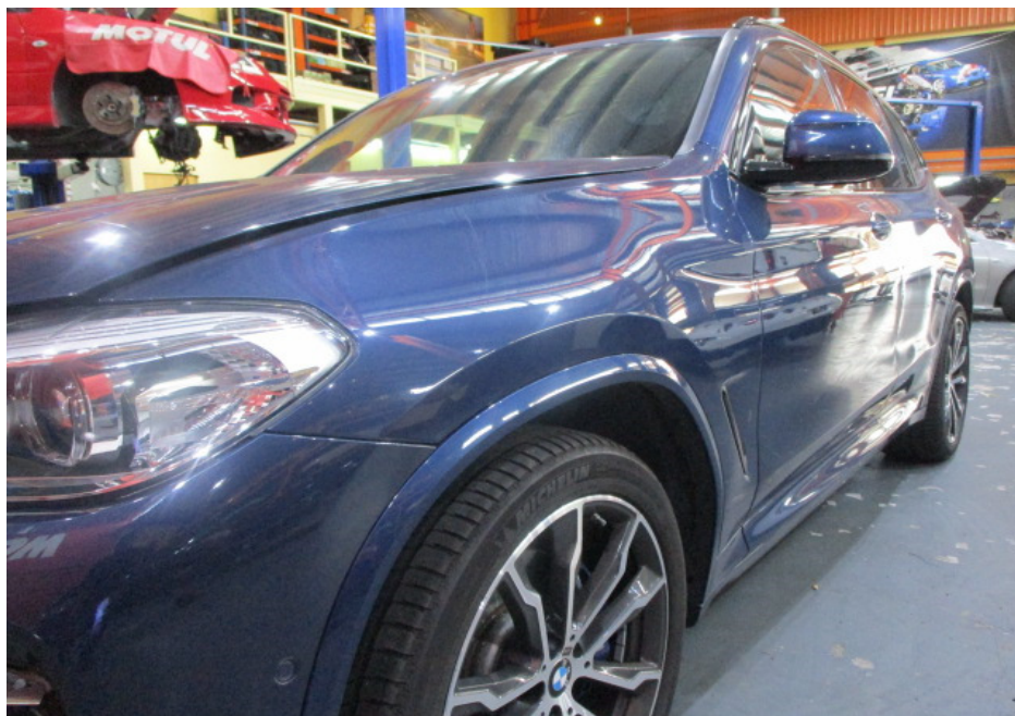
Photo 9 shows a closer view of the Motor Car's front left fender, front left fender wheel arc garnish and front left headlamp. The body parts at the frontal portion of the Motor Car were visually examined and it was observed that the repair/restoration works carried out to the damaged area of the Motor Car (refer to photograph 1 – 3 above) were reasonably adequate and in order.
