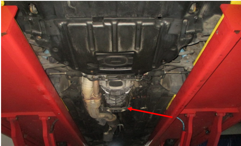
Photo 2 shows a general view of the transmission (arrowed) that was fitted on the Motor Car. The front (input) side of the transmission is bolted to the crankshaft side of the engine block. The gear set in the input side of the transmission connects to the transfer case, which is the output (rear) side of the Motor Car's transmission. The transfer case connects to the propeller shaft, which leads to the rear differential of the Motor Car.
