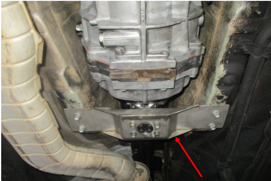
Photo 4 shows a closer view of the bracket (arrowed) mounted to the underside of the Motor Car's floorboard via bolts and nuts. The bracket supports the rear (output) side of the transmission. Rubber bushing absorbs any vibrations arising from the rotation of the transmission gears, minimising any stress to the bracket and correspondingly also minimise any stress at the mounting points of this bracket.
