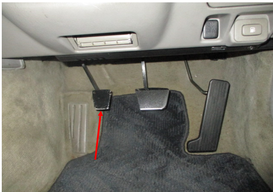
Photo 9 shows the clutch pedal (arrowed) of the Motor Car, for engaging and disengaging the transmission gears.
