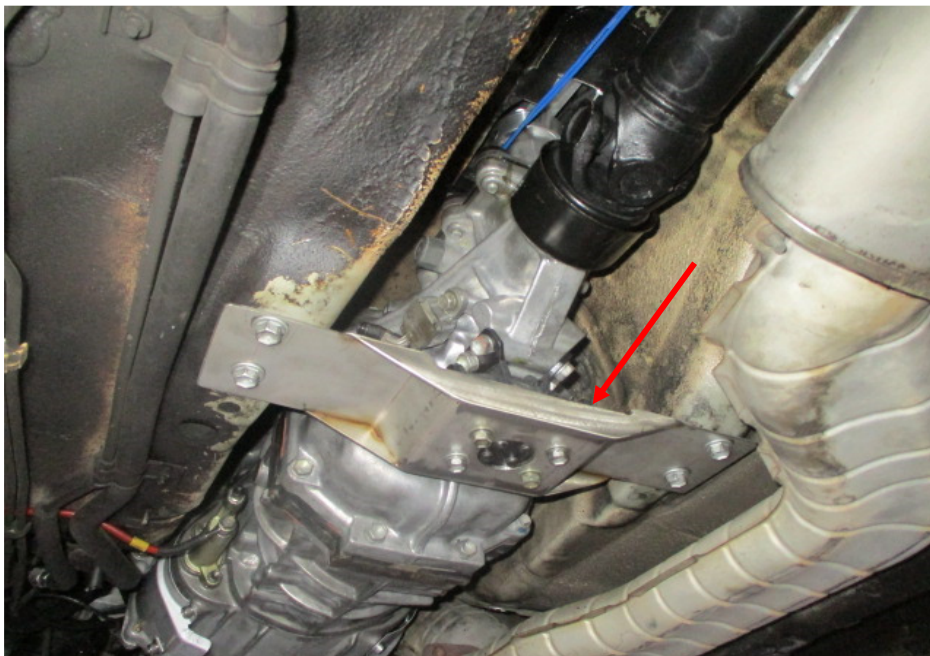
Photo 5 shows another view of the bracket (arrowed) that supports the transmission of the Motor Car, as viewed from the rear to front. This bracket at the rear of the transmission was with rubber bushing, which absorbs any vibrations arising from the rotation of the transmission gears, minimising any stress to the bracket and correspondingly also minimise any stress at the mounting points of this bracket.
