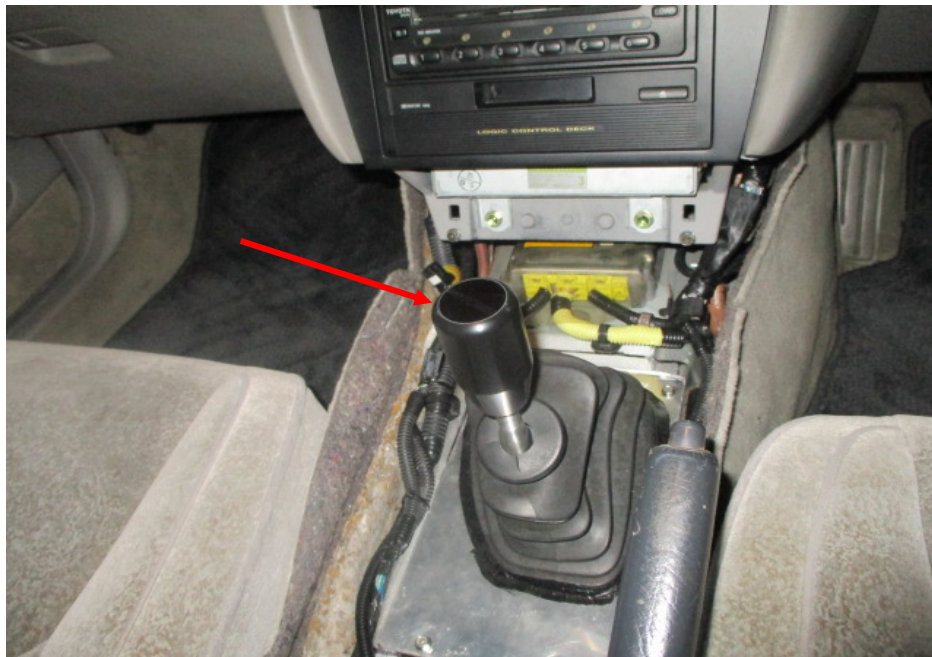
Photo 8 shows the manual gear shifter (arrowed) that was fitted on the Motor Car, for manually selecting the transmission gear to be engaged.
