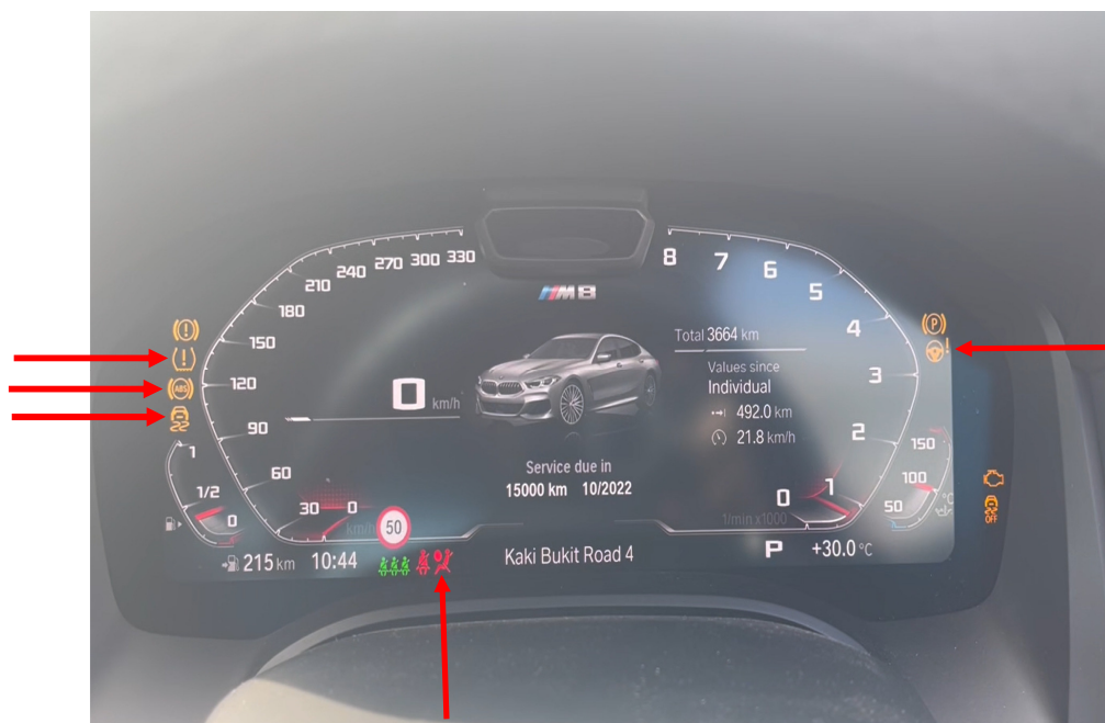
Photo 15 shows the warning lights for the various electronic safety features appearing on the instrument panel of the Motor Car during its self-test when the engine is cranked, in particular the ABS, SRS, IAS, TPM and DSC lights (arrowed).
