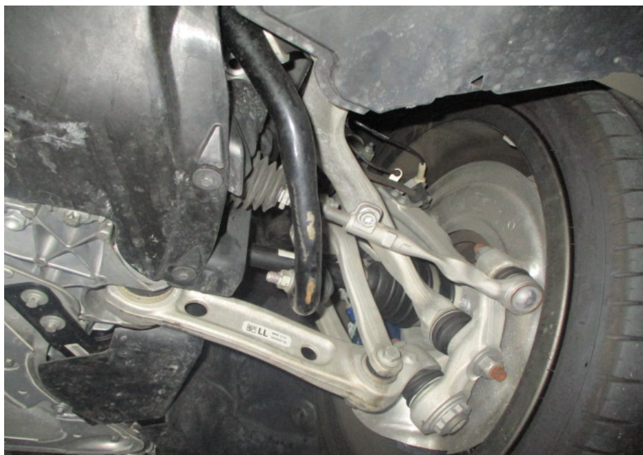
Photo 21 shows the various undercarriage components at the front left wheel of the Motor Car. The mechanical components, control arms and linkages were all found to be intact and secured in an appropriate manner. I also did not observe any fluid leak and/or fluid stain on the underside of the Motor Car.
