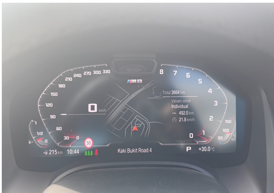
Photo 16 shows the respective warning lights no longer illuminated, indicating that there is no fault detected to the ABS, SRS, IAS, TPM and DSC systems of the Motor Car during the self-test. These electronic systems were hence in working condition at the time of my inspection.
