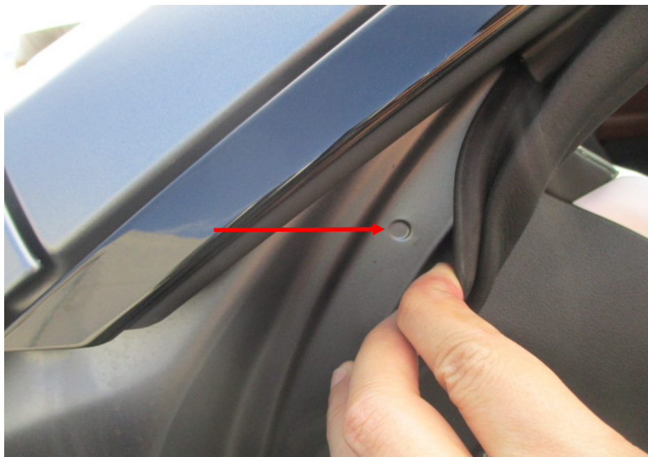
Photo 28 shows the left side "A" pillar of the Motor Car. I did not find any weld marks other than original spot weld marks (arrowed) on the left side "A" pillar of the Motor Car which, indicates that there was no re-welding works carried out. In general, I had found all the non-detachable body panels of the Motor Car to be originally fitted at the time of my inspection.
