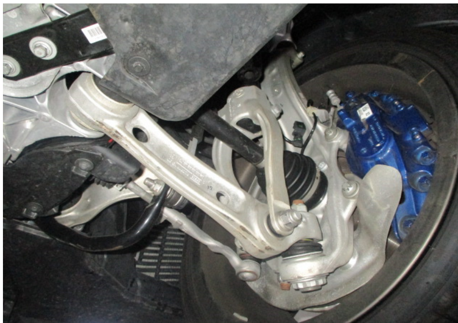
Photo 20 shows the various undercarriage components at the front right wheel of the Motor Car. I did not observe any fluid leak and/or fluid stain on the underside of the Motor Car. All of the Motor Car's undercarriage components were observed to be intact and secured in an appropriate manner.
