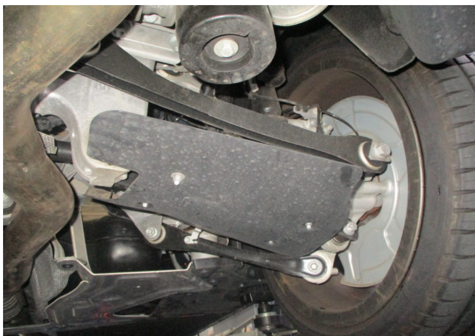
Photo 19 shows the various undercarriage components at the rear right wheel of the Motor Car. The mechanical components, control arms and linkages were all found to be intact and secured in an appropriate manner.
