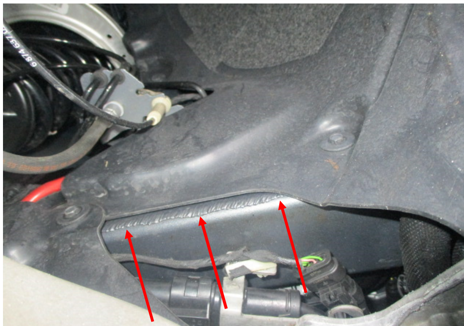
Photo 26 shows the chassis/structural body at the underside front right of the Motor Car. I did not find any weld marks other than original spot weld marks on the chassis/structural body of the Motor Car. The original factory sealant (arrowed) at the joints along the chassis/structural body was untouched, indicating no work was done on the chassis/structural body of the Motor Car and that the chassis/structural body was originally fitted.
