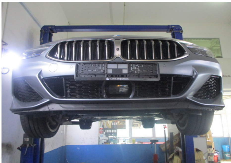
Photo 17 shows the Motor Car hoisted up for checks on its undercarriage. There was no sign(s) or indication(s) of fluid leakage and/or fluid stain(s) on the underside of the Motor Car. The undercarriage components of the Motor Car were also all observed to be intact and secured in an appropriate manner.
