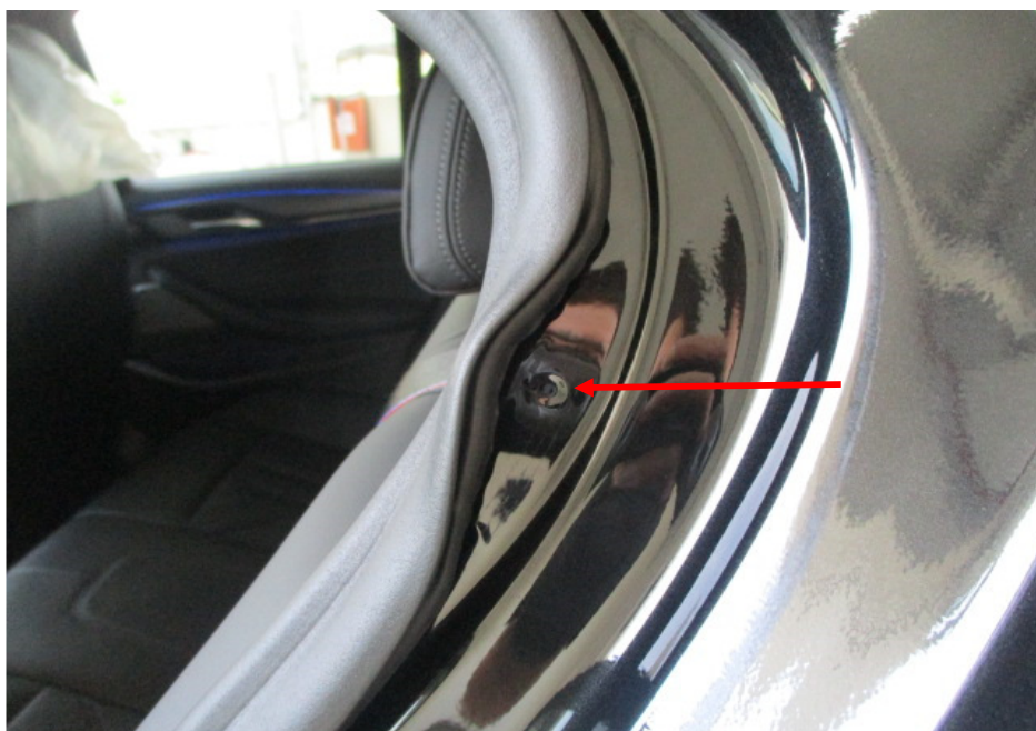
Photo 29 shows the left side "C" pillar of the Motor Car. I did not find any weld marks other than original spot weld marks (arrowed) on the left side "C" pillar of the Motor Car which, indicates that there was no re-welding works carried out. In general, I had found all the non-detachable body panels of the Motor Car to be originally fitted at the time of my inspection.
