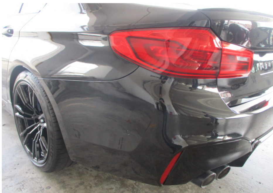
Photo 7 shows a closer view of the Motor Car's rear bumper, rear bumper lower diffuser, rear bumper left reflector, rear left taillamp, rear left fender and rear left wheel rim at the time of my inspection. The body parts at the rear left portion of the Motor Car were visually examined, and it was observed that the repair/restoration works carried out to the damaged area of the Motor Car (refer to photograph 1 – 3) were reasonably adequate and in order.
