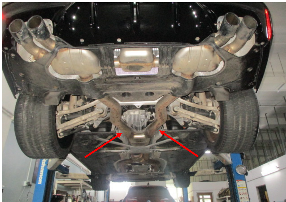
Photo 22 shows a general view of the rear section of the Motor Car's exhaust system. My examination of the Motor Car's exhaust system revealed no sign(s) or indication(s) of any cut or weld marks along its exhaust pipes (arrowed), on its centre resonators boxes, on its catalytic converters and on its rear mufflers.
