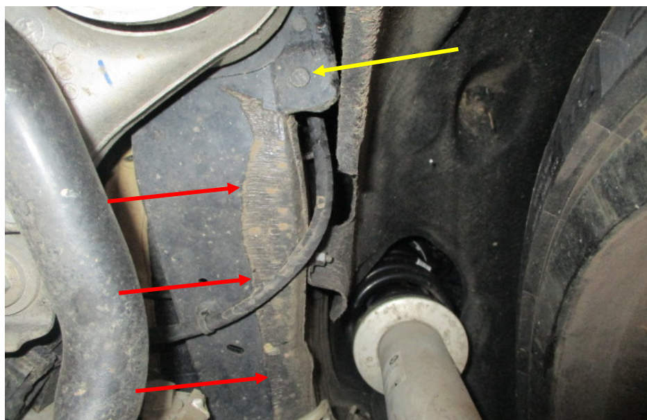
Photo 27 shows the chassis/structural body at the underside rear right of the Motor Car. I did not find any weld marks other than original spot weld marks (yellow arrow) on the chassis/structural body of the Motor Car. The original factory sealant (red arrow) at the joints along the chassis/structural body was untouched, indicating no work was done on the chassis/structural body of the Motor Car and that the chassis/structural body was originally fitted.
