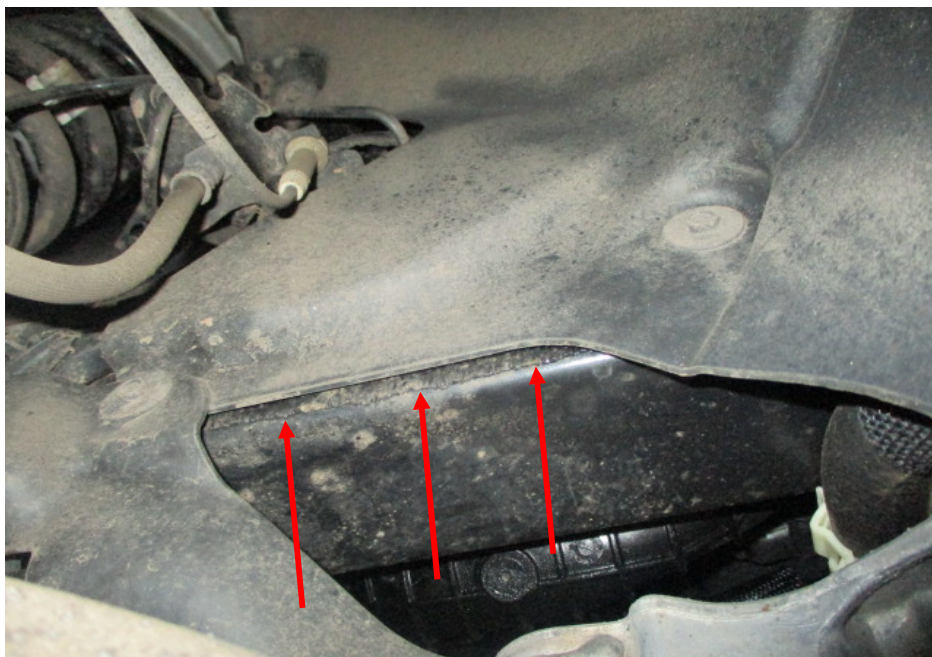
Photo 24 shows the chassis/structural body at the underside front right of the Motor Car. I did not find any weld marks other than original spot weld marks on the chassis/structural body of the Motor Car. The original factory sealant (arrowed) at the joints along the chassis/structural body was untouched, indicating no work was done on the chassis/structural body of the Motor Car and that the chassis/structural body was originally fitted.
