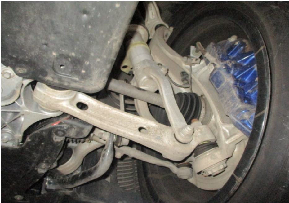
Photo 21 shows the various undercarriage components at the front right wheel of the Motor Car. The mechanical components, control arms and linkages were all found to be intact and secured in an appropriate manner. I also did not observe any fluid leak and/or fluid stain on the underside of the Motor Car.
