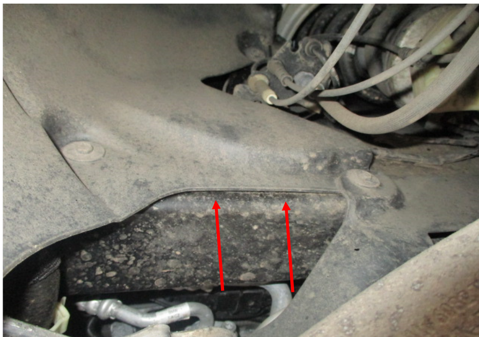
Photo 25 shows the chassis/structural body at the underside front left of the Motor Car. The original factory sealant (arrowed) at the joints along the chassis/structural body was observed to be untouched. In general, I had found no work was carried out on the chassis/structural body of the Motor Car. The chassis/structural body of the Motor Car was originally fitted.
