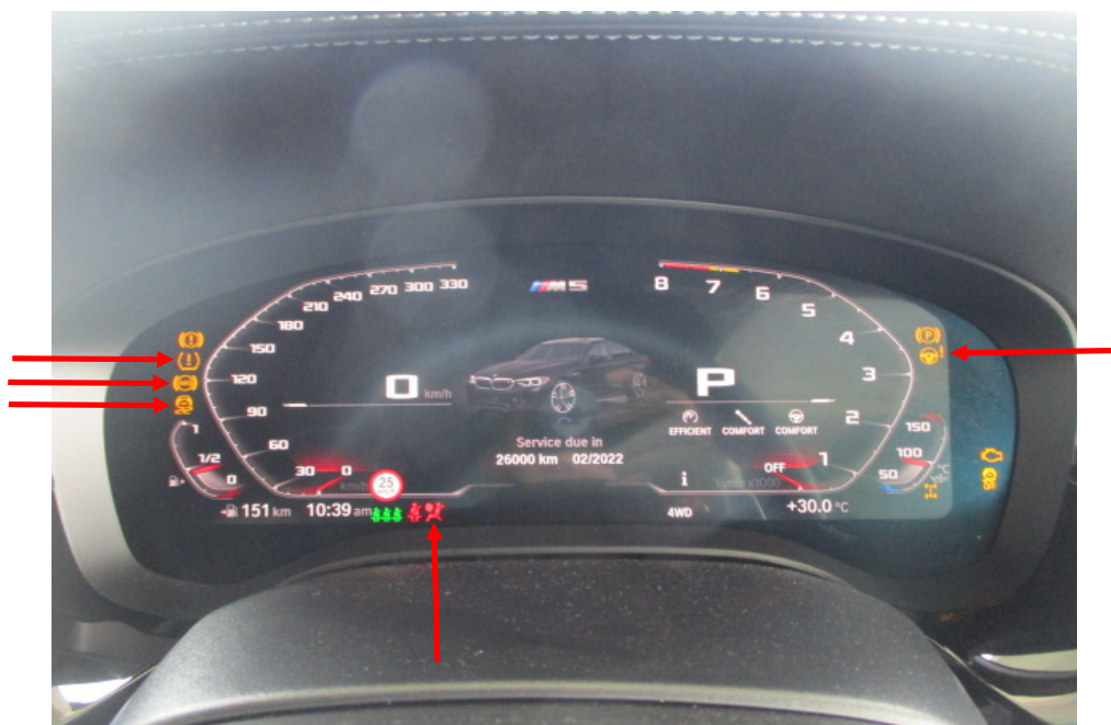
Photo 15 shows the warning lights for the various electronic safety features appearing on the instrument panel of the Motor Car during its self-test when the engine is cranked, in particular the ABS, SRS, IAS, TPM and DSC lights (arrowed).
