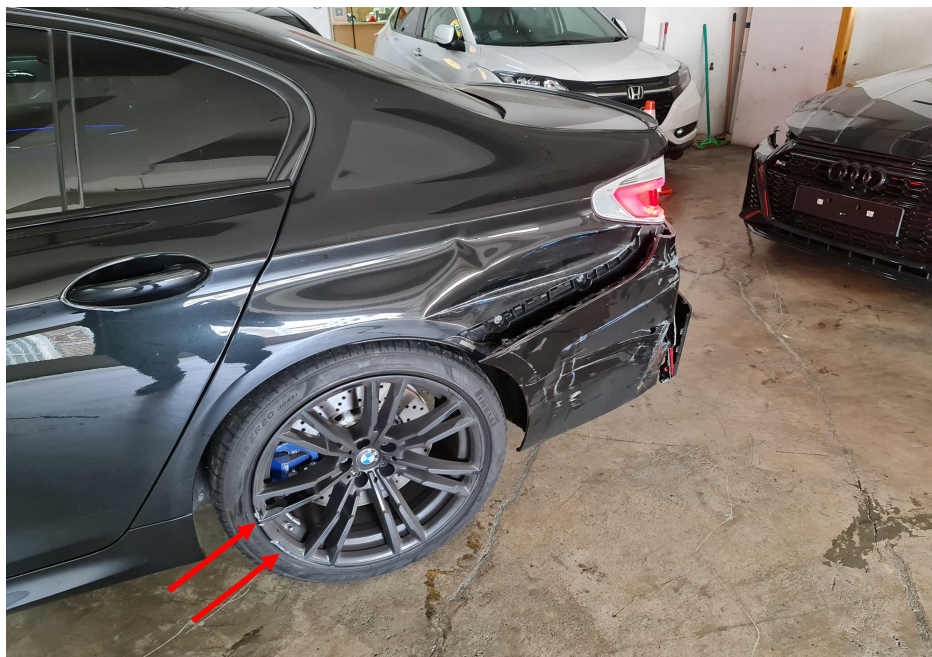
Photo 3 shows another view of the rear left body of the Motor Car (photograph provided to me). The Motor Car was observed to have sustained damage at its rear left portion. The rear bumper, rear bumper lower diffuser, rear bumper left reflector, rear left taillamp, rear left fender and rear left wheel rim (arrowed) were amongst the body parts that were observed to be damaged.
