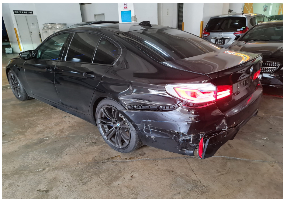
Photo 2 shows the rear left body of the Motor Car (photograph provided to me). The Motor Car was observed to have sustained damage at its rear left portion. The rear bumper, rear bumper lower diffuser, rear bumper left reflector, rear bumper sensor, rear left taillamp and rear left fender were amongst the body parts that were observed to be damaged.
