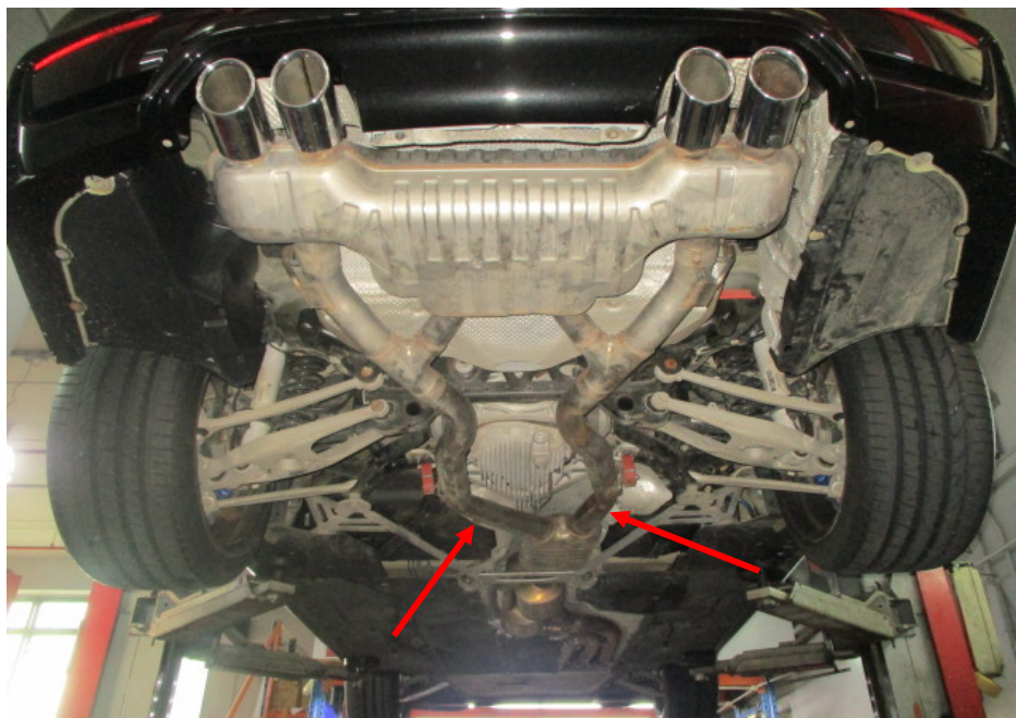
Photo 23 shows a general view of the rear section of the Motor Car's exhaust system. My examination of the Motor Car's exhaust system revealed no sign(s) or indication(s) of any cut or weld marks along its exhaust pipes (arrowed), on its centre resonator boxes, on its catalytic converters and on its rear muffler.
