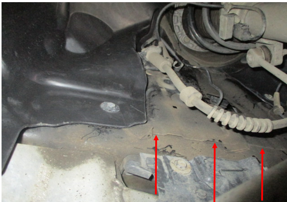
Photo 26 shows the chassis/structural body at the underside front left of the Motor Car. The original factory sealant (arrowed) at the joints along the chassis/structural body was observed to be untouched. In general, I had found no work was carried out on the chassis/structural body of the Motor Car. The chassis/structural body of the Motor Car was originally fitted.
