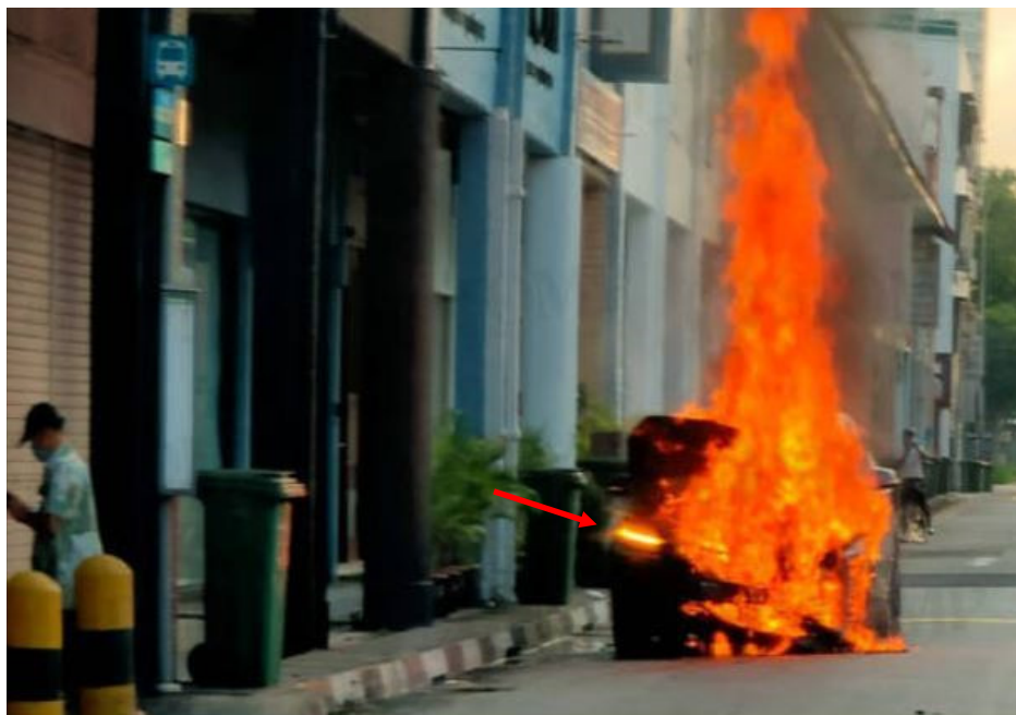
Photo 10 shows the Insured Vehicle on fire before the arrival of the SCDF. In general, the information that could be gathered from this photograph had corresponded to the events that were related to us by Ms Goh and Mr Lee which is the fire had started from the engine compartment of the Insured Vehicle (arrowed).
