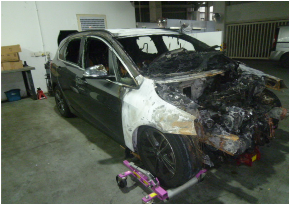
Photo 3 shows the closer view of the right front body of the Insured Vehicle at the time of our inspection. The fire damage to the Insured Vehicle was confined to its frontal portion. Its front bumper, front bonnet, front support panel, front grille, front headlamps, front windscreen, front wheel rims, front fenders and front tyres, amongst others were amongst the body parts that were found to have been affected by the fire.
