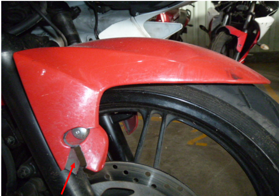
Photo 6 shows a close up view of the front mudguard which was amongst the body parts of the Motorcycle that had sustained damage as a result of the accident (arrowed).
