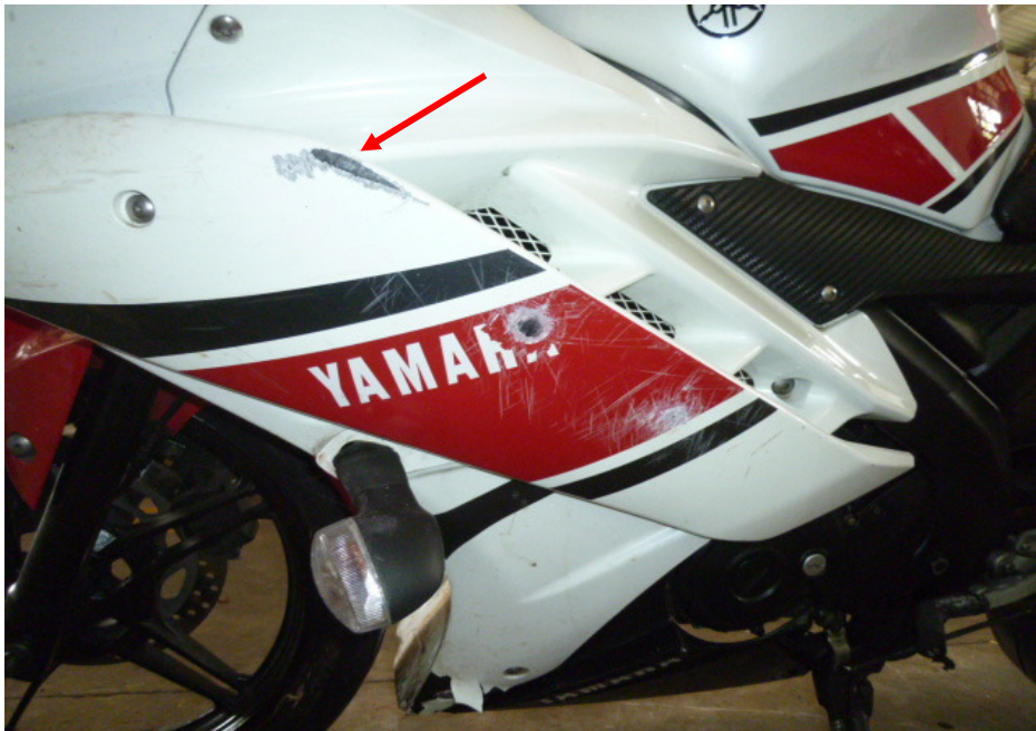
Photo 8 shows a closer view of the grazed left cowling of the Motorcycle as a result of the accident (arrowed).
