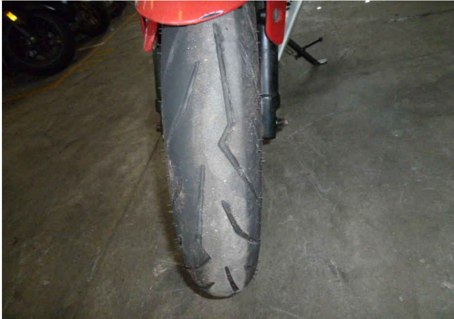
Photo 15 shows the condition of the Motorcycle's front tyre. The front tyre was observed to be in serviceable condition with remaining tread depth of approximately 5mm. There was no tear, burst mark(s) and/or punctured hole(s) on the sidewalls as well as across the tread of the front tyre.
