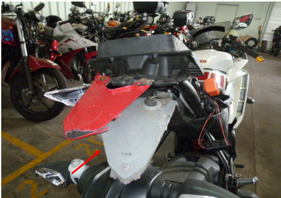
Photo 12 shows a closer view of the broken tail light assembly which was amongst the body parts of the Motorcycle that had sustained damage as a result of the accident (arrowed).
