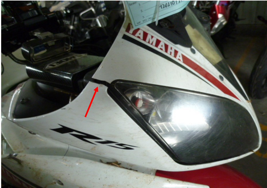
Photo 5 shows a closer view of the cracked head cowl which was amongst the body parts at the front body of the Motorcycle that had sustained damage as a result of the accident (arrowed).
