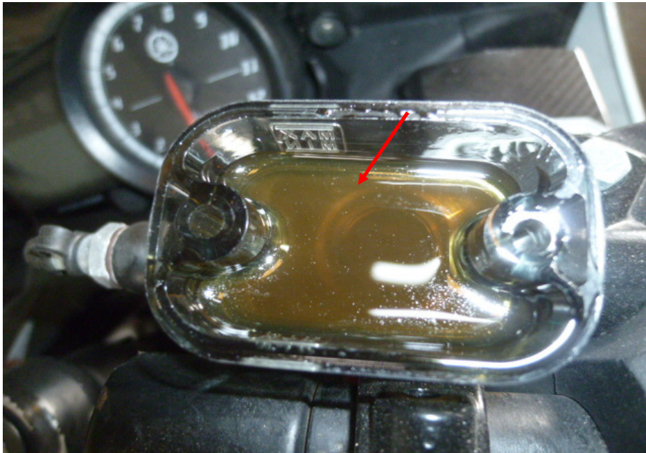
Photo 23 shows the brake fluid reservoir for the front brake of the Motorcycle. The brake fluid was observed to be of sufficient level for operational purposes and without contamination. However the brake fluid was found to be slightly contaminated (arrowed).
