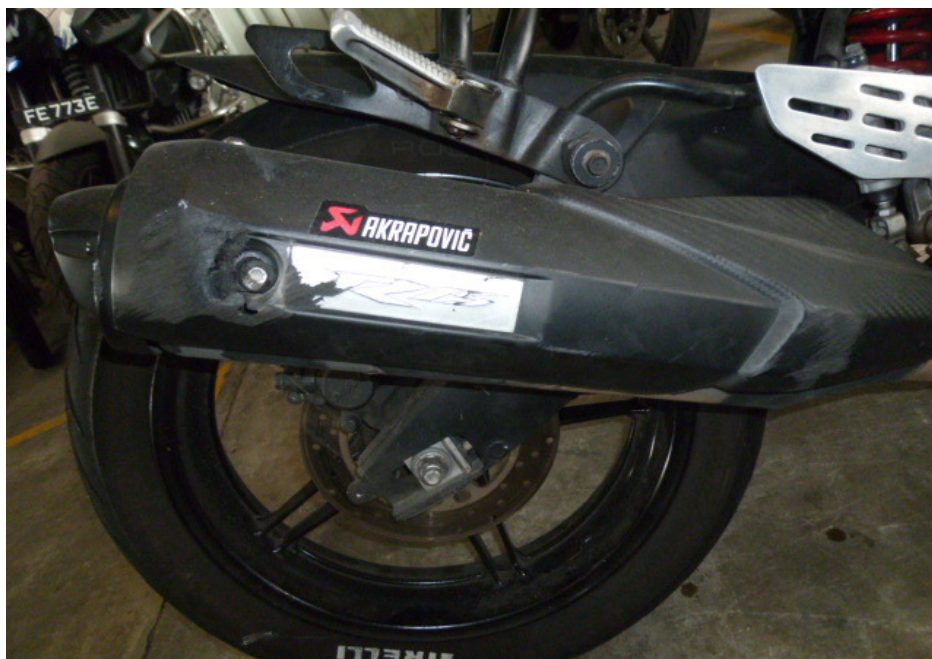
Photo 14 shows a closer view of the exhaust muffler heat shield of the Motorcycle that had sustained damages of grazing nature as a result of the accident.
