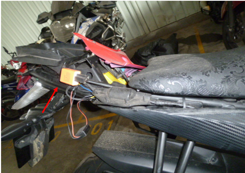
Photo 11 shows the missing right rear side cover of the Motorcycle which was amongst the body parts of the Motorcycle as a result of the accident (arrowed).
