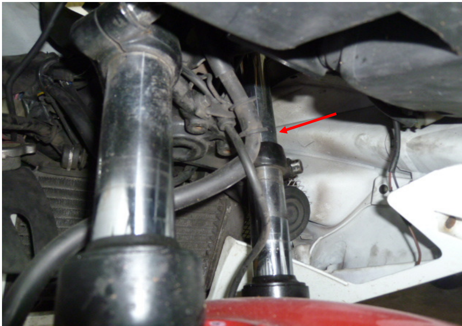
Photo 21 shows the front fork assembly of the Motorcycle. The front left fork was observed to be slightly bent (arrowed) as a result of the accident. We were hence not able to conduct any tests on the steering system of the Motorcycle.
