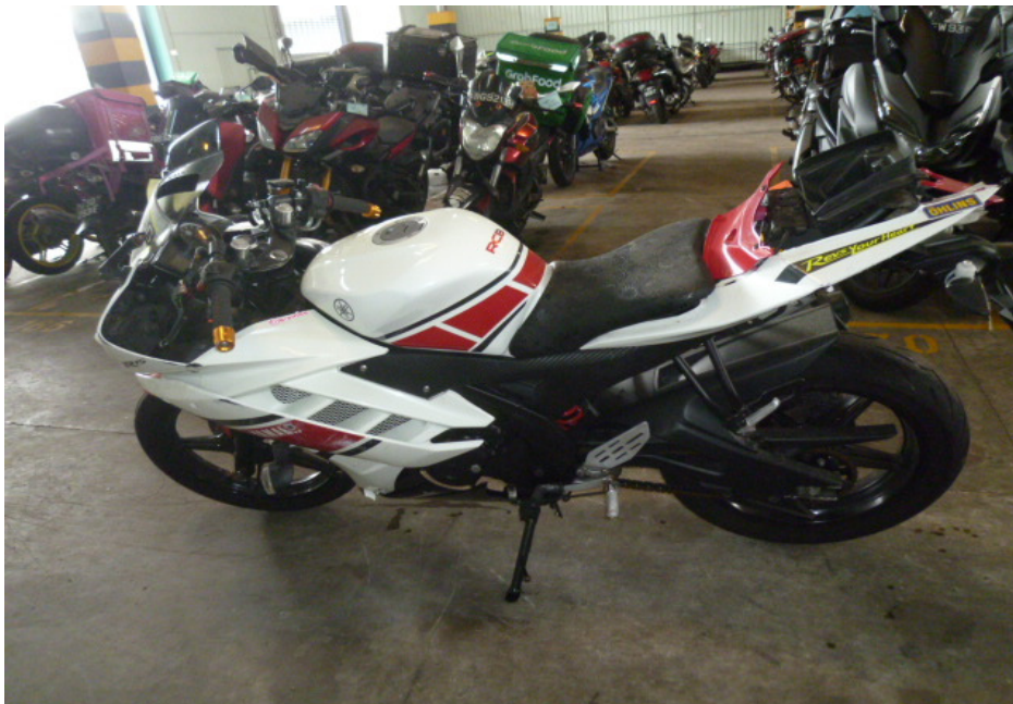
Photo 4 shows a general view of the left body of the Motorcycle at the time of our inspection. The Motorcycle was observed to have sustained damages all around. Amongst the body parts that were found to have been damaged include its head cowlings, front mudguard, side cowlings, right handlebar end, front brake lever, rear brake pedal, right front footrest, rear side covers, tail light assembly, left front footrest, gear shift pedal and exhaust muffler heat shield, amongst others.
