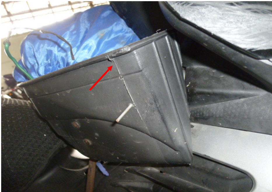
Photo 8 shows a closer view of the grazed front basket of the Motorcycle as a result of the accident (arrowed).
