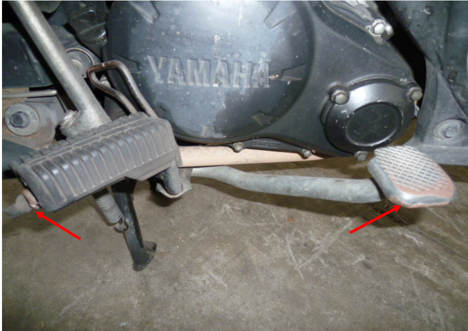
Photo 10 shows a closer view of the right front footrest and rear brake pedal which were amongst the body parts of the Motorcycle that had sustained damages as a result of the accident (arrowed).
