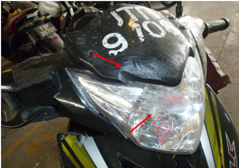
Photo 5 shows a close up view of the grazed head cowl and headlight of the Motorcycle as a result of the accident (arrowed).
