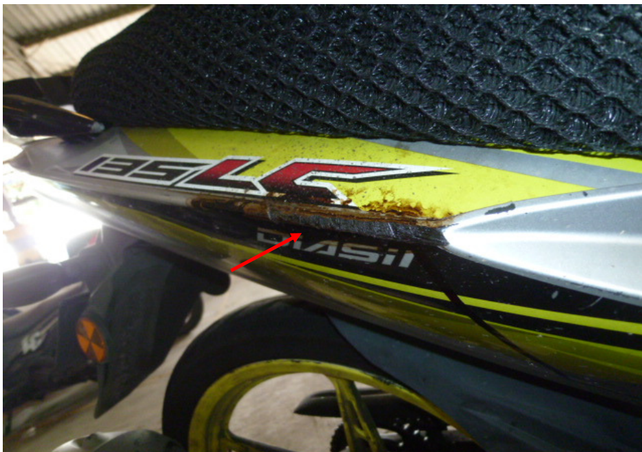
Photo 9 shows a closer view of the grazed right rear side cover of the Motorcycle as a result of the accident (arrowed).
