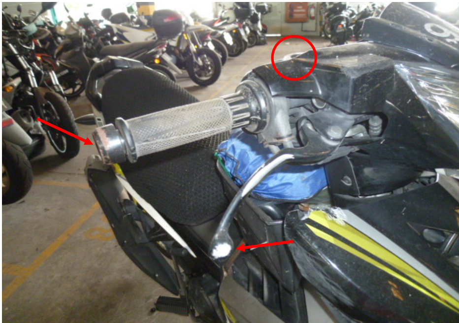
Photo 7 shows the right handlebar end and front brake lever (arrowed) as well as the missing right side mirror (circled), which were amongst the body parts of the Motorcycle that had sustained damage as a result of the accident.
