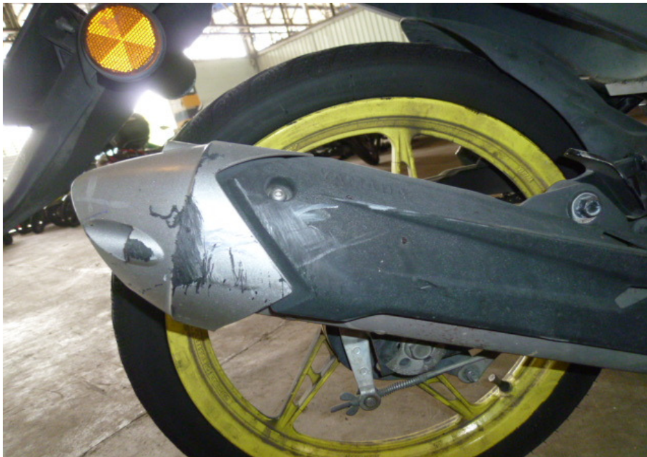
Photo 11 shows the exhaust muffler heat shield of the Motorcycle that had sustained damages of grazing nature as a result of the accident.
