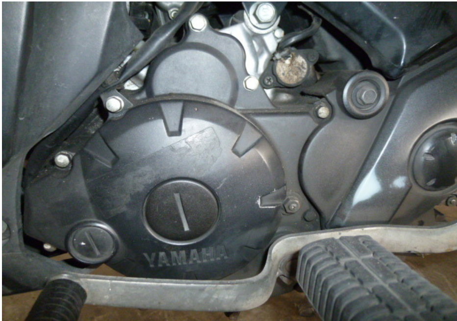
Photo 15 shows the left side of the engine of the Motorcycle at the time of our inspection. The various engine related parts and components were found to be intact with no visible damage. There was also no sign(s) or indication(s) of fluid leak observed around the left engine area of the Motorcycle.
