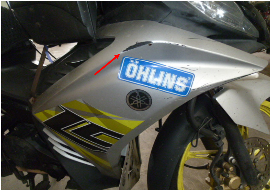
Photo 6 shows a closer view of the grazed right cowling which was amongst the body parts of the Motorcycle that had sustained damage as a result of the accident (arrowed).
