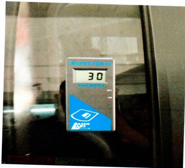
Rear Windows VLT Reading: 30% (right)
