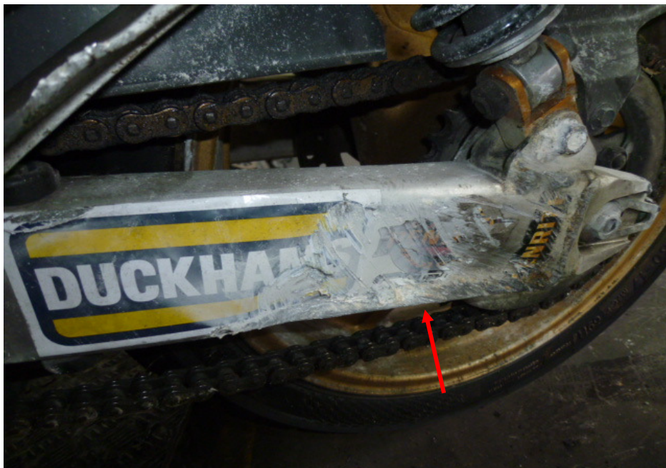
Photo 10 shows a closer view of the deformed rear swingarm (arrowed) of the Motorcycle as a result of the accident.
