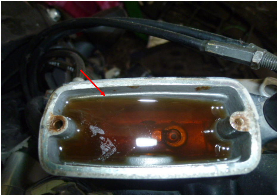
Photo 24 shows the brake fluid reservoir for the front brake of the Motorcycle. The brake fluid was observed to be of sufficient level for operational purposes. However it was found to be slightly contaminated (arrowed).
