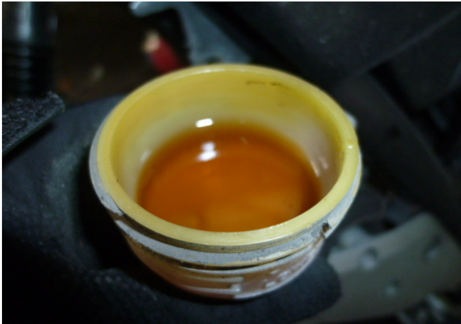
Photo 27 shows the brake fluid reservoir for the rear brake of the Motorcycle. The brake fluid was observed to be of sufficient level for operational purposes and without contamination.
