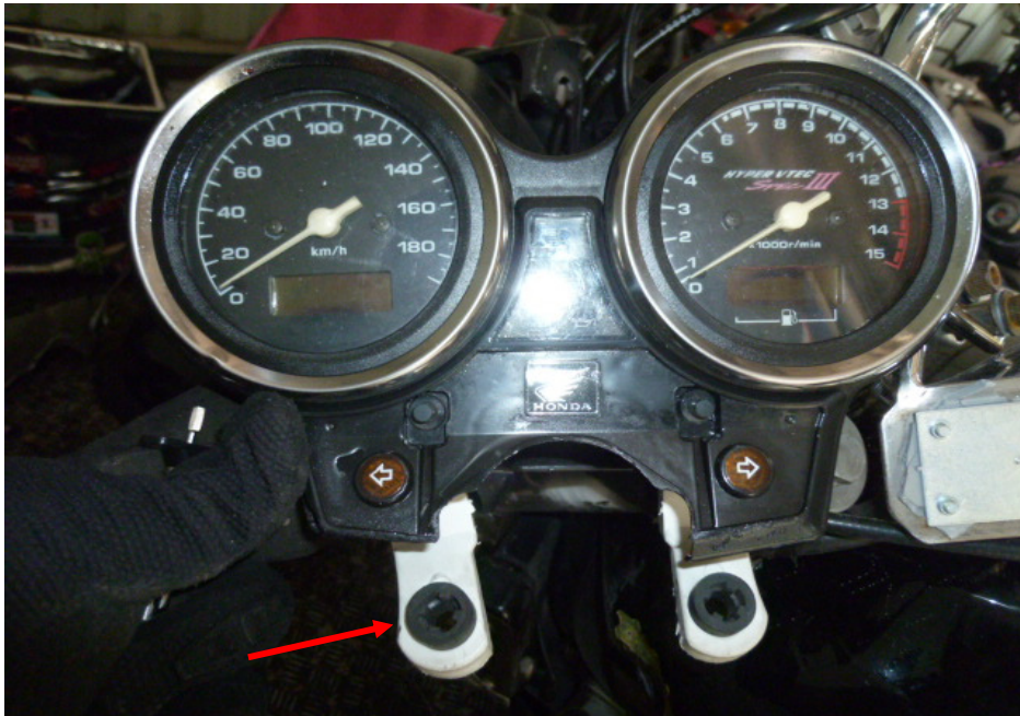
Photo 7 shows the broken speedometer of the Motorcycle as a result of the accident (arrowed).
