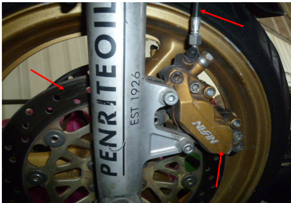
Photo 23 shows a close up view of the front brake caliper, front brake disc and front brake hose (arrowed) at the left side of the Motorcycle's front wheel, which are all part of the components in the hydraulic front brake system of the Motorcycle. Our visual checks of these various components had revealed all to be intact with no visible damage. No leakage of brake fluid was also observed.
