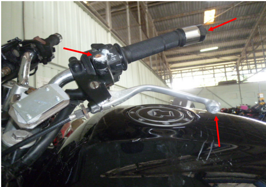
Photo 6 shows a closer view of the clutch lever, left side mirror and left handlebar end (arrowed) which were amongst the body parts at the front body of the Motorcycle that had sustained damage as a result of the accident.
