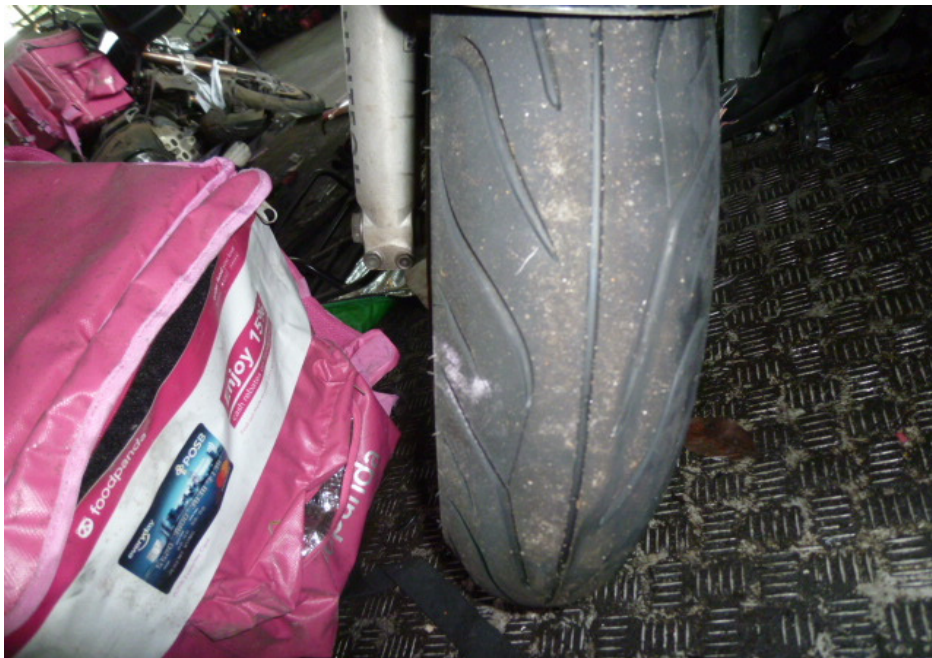
Photo 14 shows the front tyre of the Motorcycle at the time of our inspection. The front tyre was observed to be in serviceable condition with remaining tread depth of approximately 5mm. The pattern of the tread was also clearly visible. There was no tear, burst mark(s) and/or punctured hole(s) on the sidewalls as well as across the tread of the front tyre.
