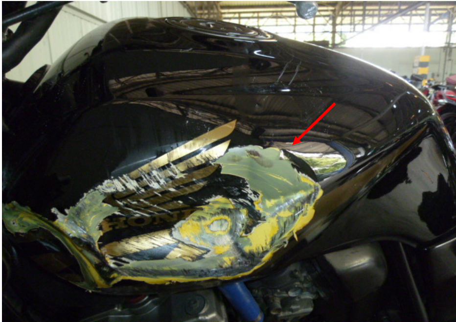
Photo 9 shows a closer view of the dented petrol tank of the Motorcycle as a result of the accident (circled).
