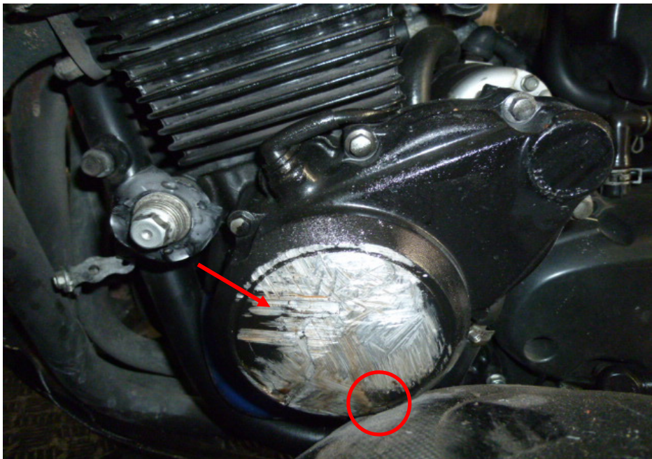
Photo 17 shows the left side of the engine of the Motorcycle at the time of our inspection. The various left engine components had sustained damage of grazing nature as a result of the accident (arrowed). Wet fluid stains were observed on the underside of the damaged left engine cover of the Motorcycle (circled).
