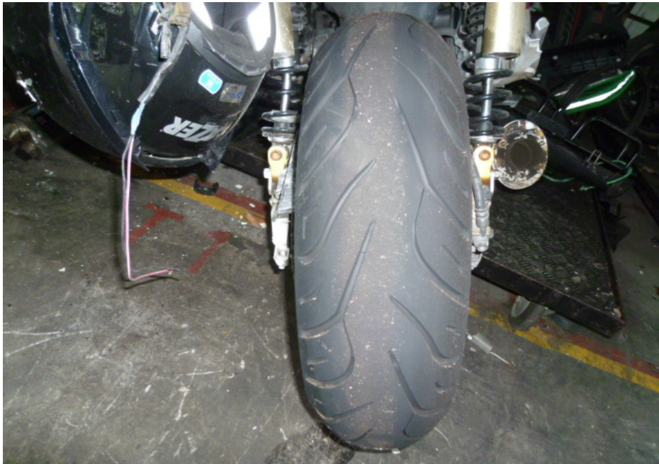
Photo 15 shows the condition of the Motorcycle's rear tyre. The rear tyre was observed to be in serviceable condition with remaining tread depth of approximately 7mm. The tyre was also observed to be sufficiently inflated for vehicular operation. We did not observe any tear, burst mark(s) and/or punctured hole(s) on the sidewalls as well as across the tread of the rear tyre.
