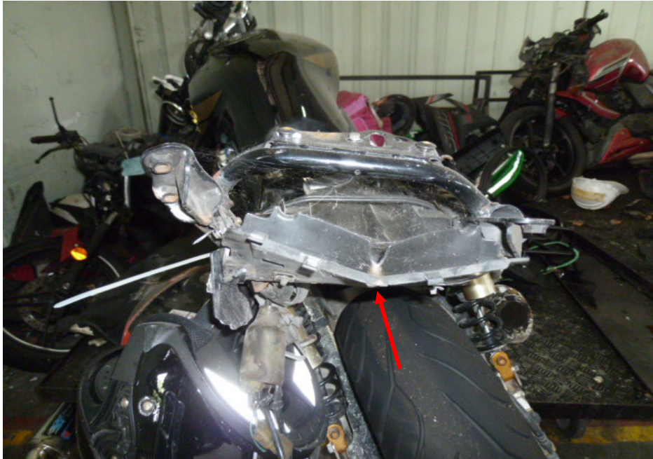
Photo 13 shows the missing tail light assembly (arrowed) of the Motorcycle as a result of the accident.
