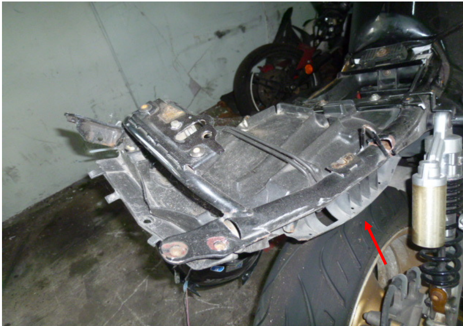
Photo 11 shows a closer view of the missing right rear side cover (arrowed) which were amongst the body parts at the rear body of the Motorcycle that had sustained damage as a result of the accident.
