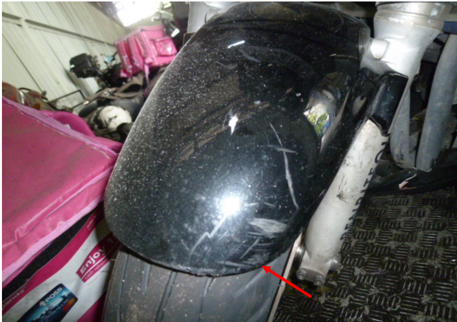
Photo 5 shows a closer view of the front mudguard which was amongst the body parts at the front body of the Motorcycle that had sustained damage as a result of the accident (arrowed).
