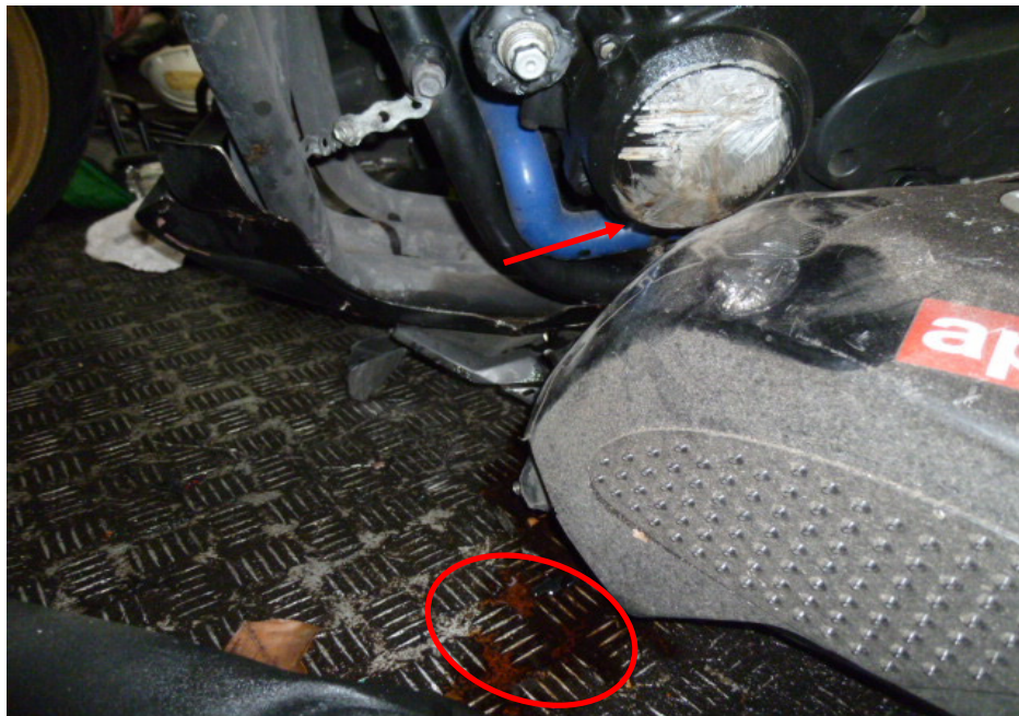
Photo 18 shows wet fluid stains observed on the ground (circled) directly below the damaged left engine cover of the Motorcycle (arrowed), indicating that a fluid leak had occurred as a result of the accident.
