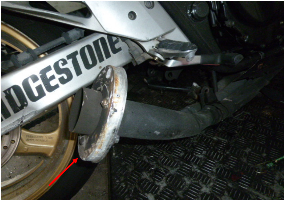
Photo 12 shows a closer view of the broken exhaust muffler (arrowed) of the Motorcycle as a result of the accident.
