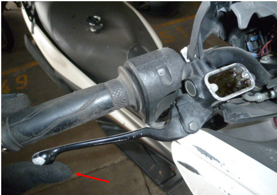
Photo 25 shows the front brake lever being depressed. There was some resistance felt (spongy like feel) upon pressing the front brake lever (arrowed). This would indicate that there is no leakage of pressure/vacuum in the front brake system.
