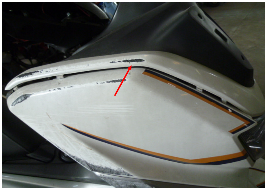
Photo 8 shows a close-up view of the grazed front cowling of the Motorcycle at the time of our inspection (arrowed).
