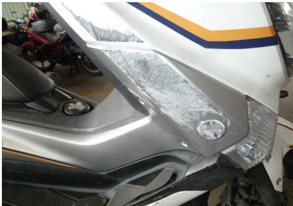
Photo 9 shows the damaged right side cowling of the Motorcycle as a result of the accident.
