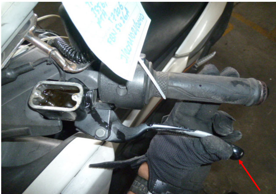
Photo 27 shows the rear brake lever being depressed. There was some resistance felt (spongy like feel) upon pressing the rear brake lever (arrowed). This would indicate that there is no leakage of pressure/vacuum in the rear brake system.
