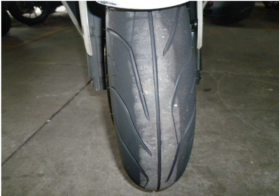
Photo 14 shows the condition of the Motorcycle's front tyre. The front tyre was observed to be in serviceable condition with remaining tread depth of approximately 6mm. There was no tear, burst mark(s) and/or punctured hole(s) on the sidewalls as well as across the tread of the front tyre.
