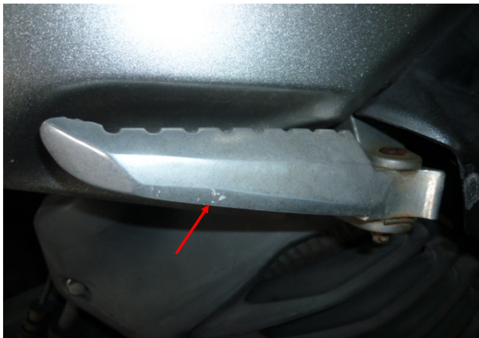
Photo 11 shows a closer view of the grazed right pillion foot peg (arrowed) of the Motorcycle as a result of the accident.
