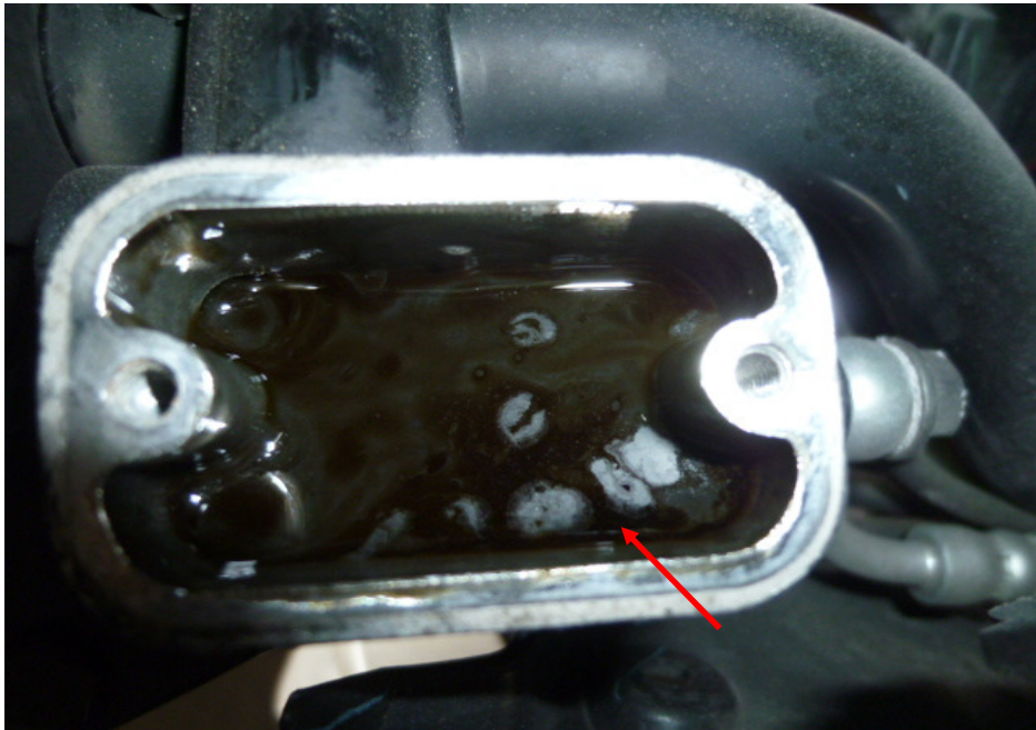
Photo 24 shows the brake fluid reservoir for the front brake of the Motorcycle. The brake fluid was observed to be of sufficient level for operational purposes. However it was found to be contaminated (arrowed).
