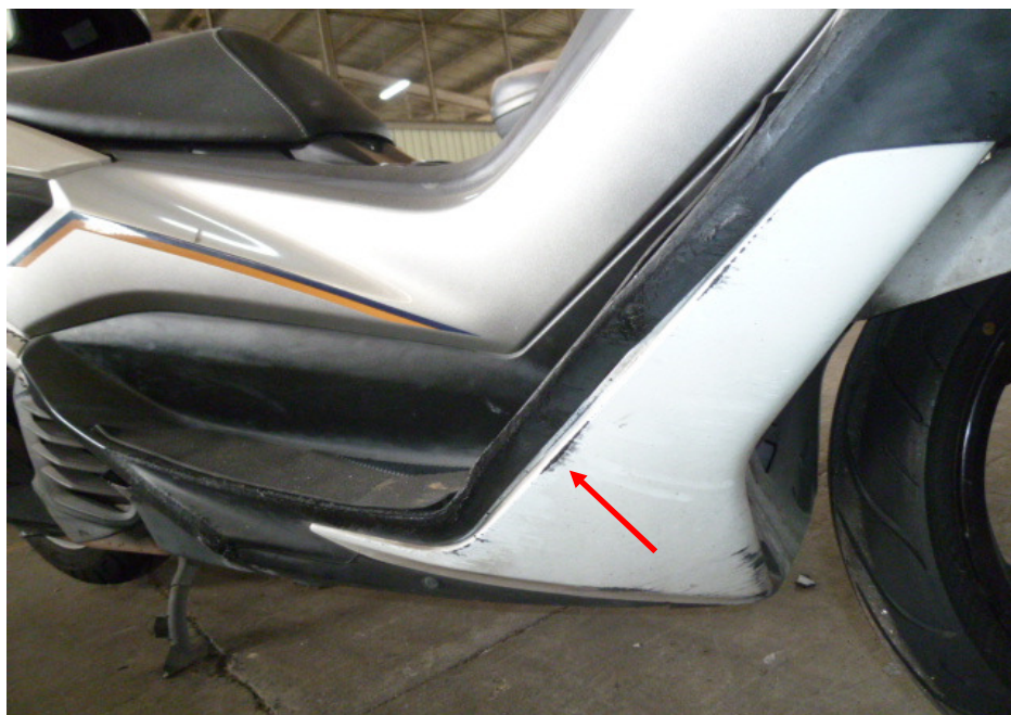
Photo 10 shows a closer view of the grazed right lower side cowling of the Motorcycle as a result of the accident (arrowed).
