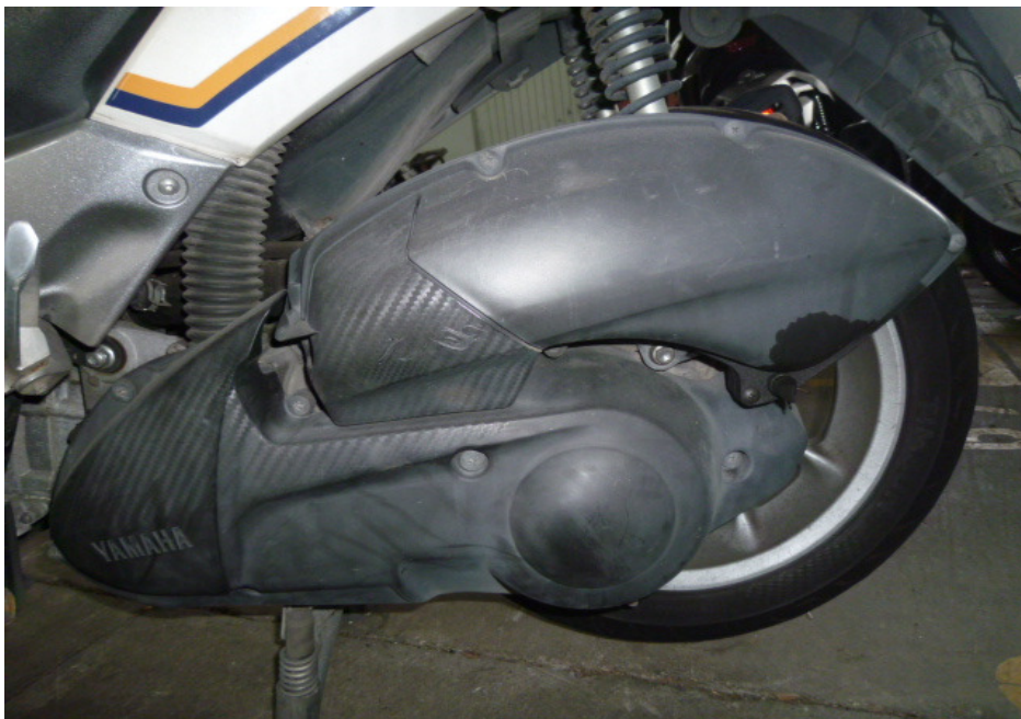
Photo 17 shows the drive train cover of the Motorcycle which was found to be intact without any misalignment. Upon examination of the Motorcycle's engine area, we had observed that the various engine related parts and components were intact with no visible damage. There was also no sign(s) or indication(s) of fluid leak observed around the engine area of the Motorcycle.
