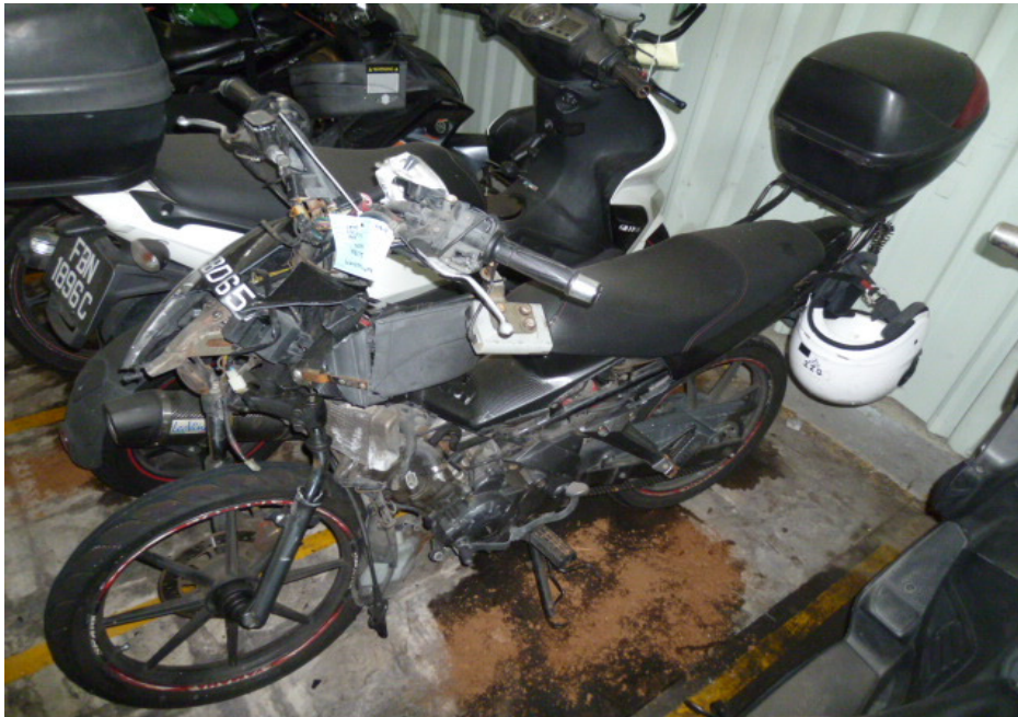
Photo 3 shows a general view of the left body of the Motorcycle at the time of our inspection. The Motorcycle had sustained damages all around. Body parts that were found to have been damaged include its headlight assembly, front cowling, front fork assembly, front mudguard, side cowlings, right side mirror, front brake lever, right handlebar end, radiator, left rear side cover and top box, amongst others.
