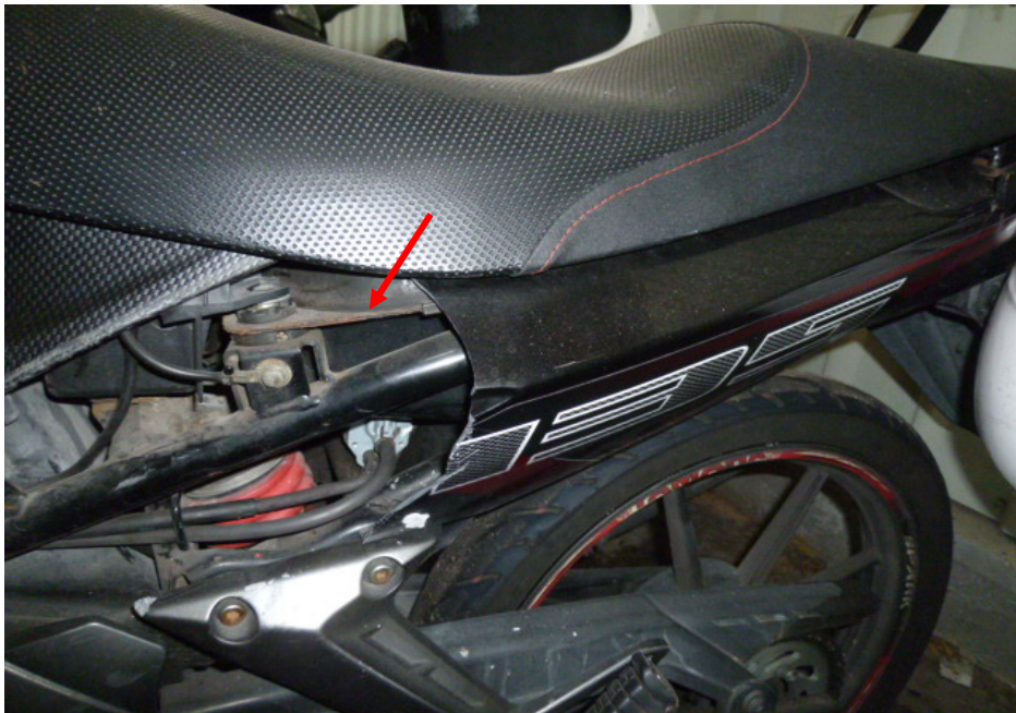
Photo 10 shows a closer view of the cracked left rear side cover (arrowed), which were amongst the body parts of the Motorcycle that had sustained damage as a result of the accident.
