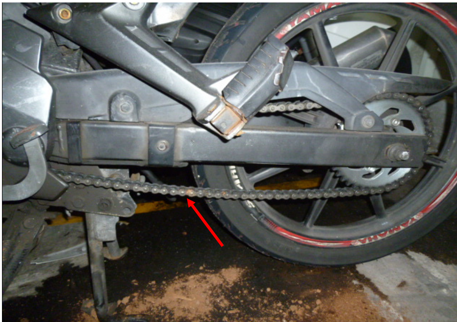
Photo 17 shows the gear train (arrowed) of the Motorcycle, which was observed to be intact with no misalignment. It was also adequately lubricated for operating purposes. The gear train rotates the rear wheel of the Motorcycle.
