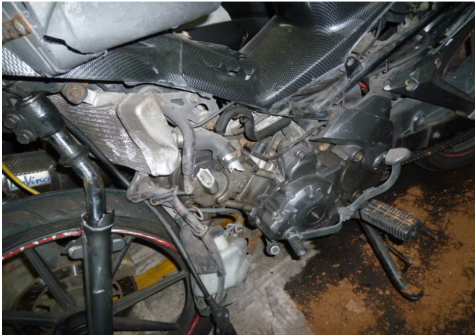
Photo 9 shows a closer view of the missing left cowling which was amongst the body parts at the front of the Motorcycle that had sustained damages as a result of the accident.
