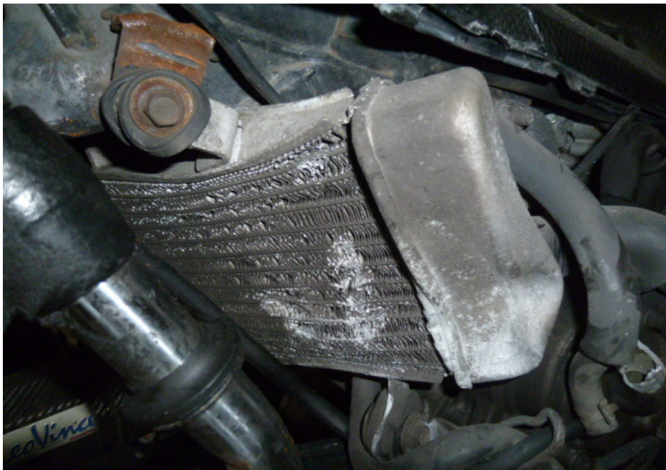
Photo 12 shows the deformed radiator of the Motorcycle as a result of the accident at the time of our inspection.
