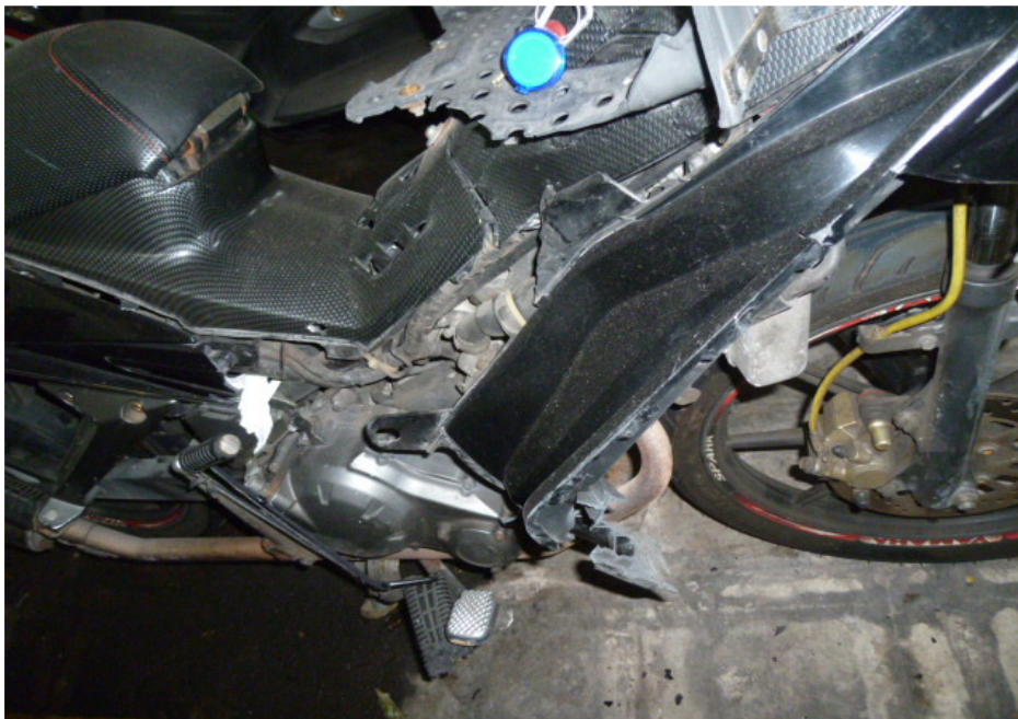
Photo 8 shows a closer view of the right cowling which was amongst the body parts at the front body of the Motorcycle that had sustained damages as a result of the accident.
