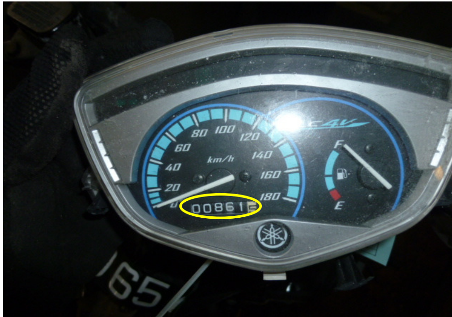
Photo 1 shows the speedometer gauge of the Motorcycle where the mileage recorded at the time of our inspection was 861km (circled).
