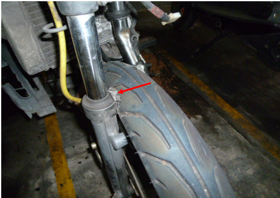
Photo 6 shows a closer view of the cracked front mudguard of the Motorcycle as a result of the accident (arrowed).
