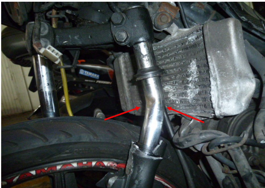
Photo 19 shows the front fork assembly of the Motorcycle. The front left fork (arrowed) was observed to be bent as a result of the accident. We were hence not able to conduct any tests on the steering system of the Motorcycle.
