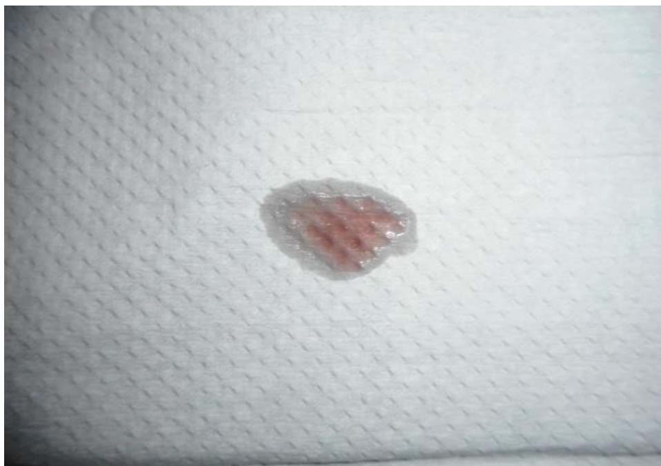
Photo 8 shows the close up view of the CVT transmission fluid of the Insured Vehicle at the time of our inspection. We observed that CVT transmission fluid was observed to be without any visible contamination.
