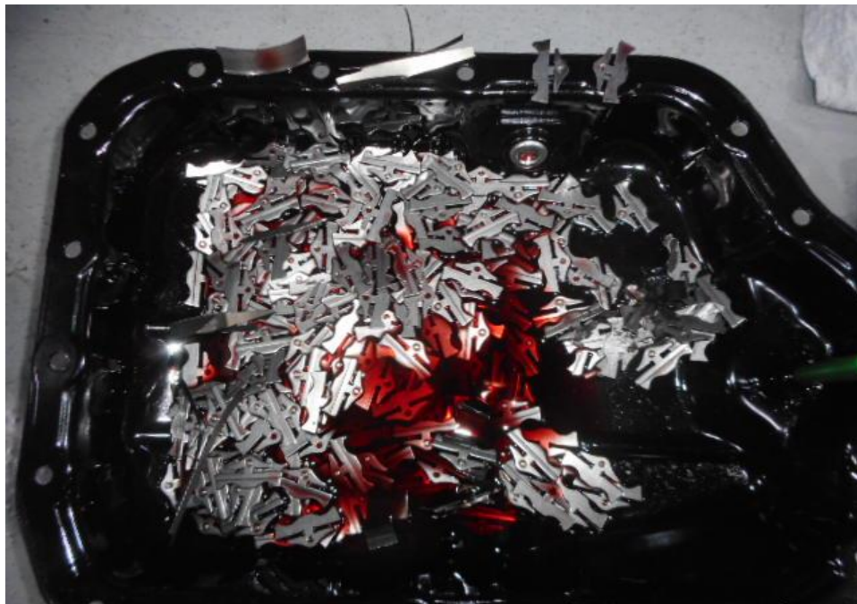
Photo 7 shows the close up view of the CVT transmission unit underside portion of the Insured Vehicle at the time of our inspection. We observed broken CVT transmission drive belt and transmission components that had fallen down to the oil sump.
