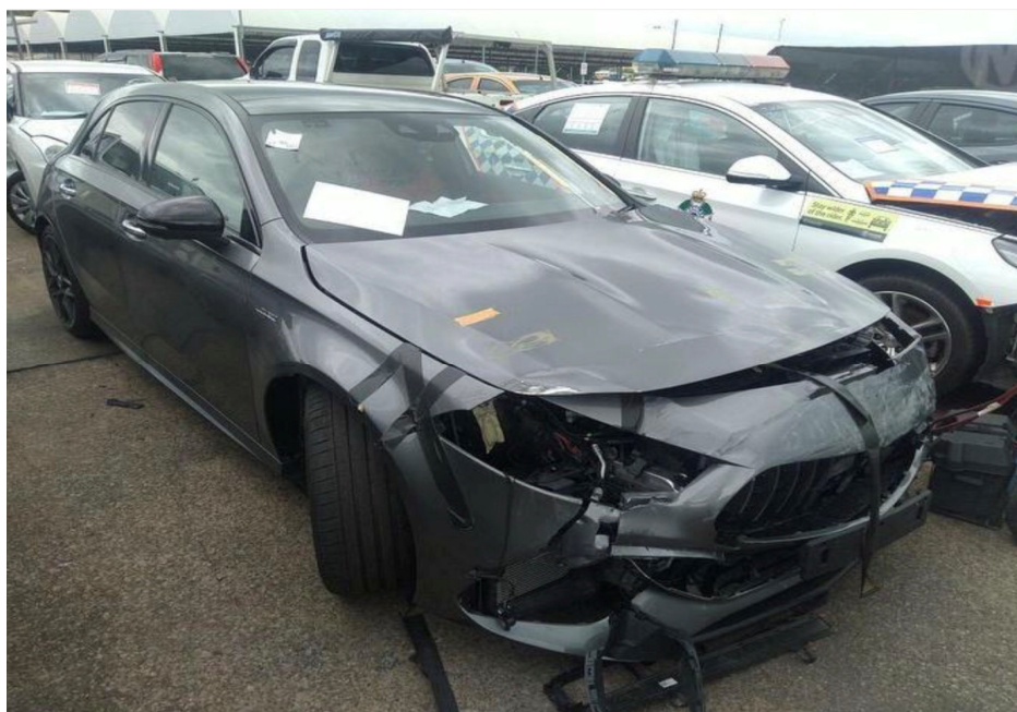
Photo 2 shows the front right body of the Motor Car (photograph provided to me). The Motor Car was observed to have sustained damage at its frontal portion. Body parts damaged include the front bumper, front bumper sponge, front bumper reinforcement, front bumper centre lower grille, front bumper right lower grille, front bonnet and radiator grille amongst others. The front right headlamp was also observed to be missing/dislodged/damaged.
