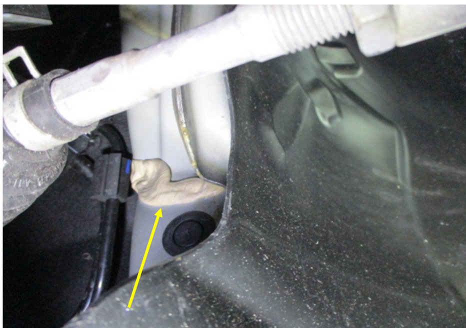
Photo 27 shows the chassis/structural body at the underside front left of the Motor Car. The original factory sealant (arrowed) at the joints along the chassis/structural body was observed to be untouched. In general, I had found no work was carried out on the chassis/structural body of the Motor Car. The chassis/structural body of the Motor Car was originally fitted.
