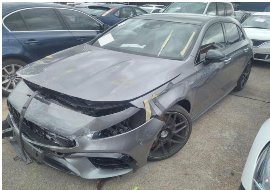
Photo 1 shows the front left body of the Motor Car (photograph provided to me). The Motor Car was observed to have sustained damage at its frontal portion. Body parts damaged include the front bumper, front bumper sponge, front bumper centre garnish, front support panel and radiator grille amongst others. The front left headlamp was also observed to be missing/dislodged/damaged.
