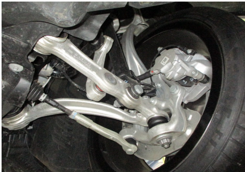
Photo 24 shows the various undercarriage components at the front right wheel of the Motor Car. The mechanical components, control arms and linkages were all found to be intact and secured in an appropriate manner. I also did not observe any fluid leak and/or fluid stain on the underside of the Motor Car.
