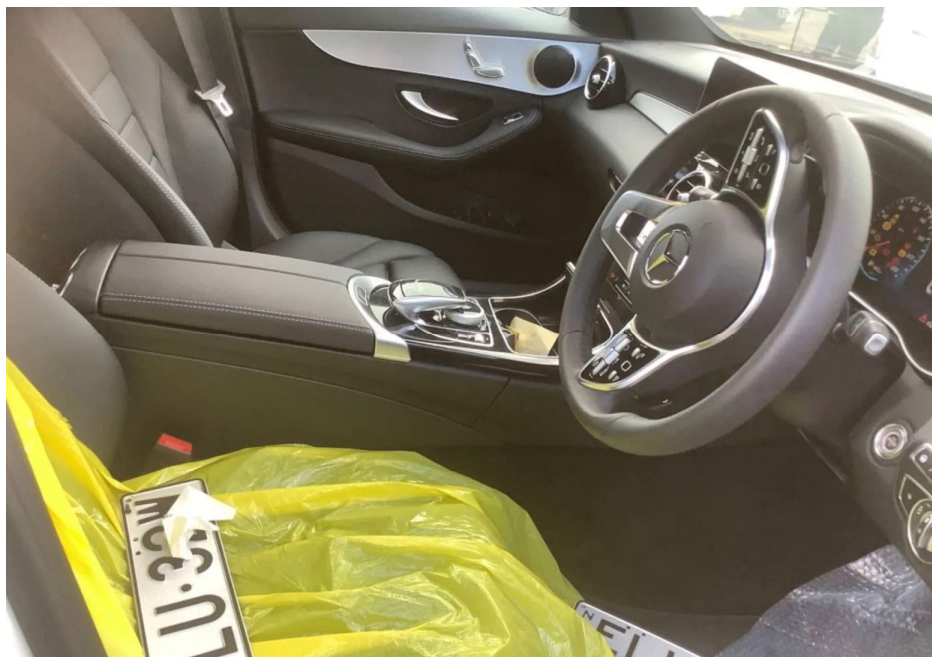
Photo 5 shows the interior compartment of the Motor Car (photograph provided to me). The various parts and components, upholstery, carpet and inner trims were all intact and undamaged. The airbag(s) of the Motor Car was not deployed as seen from the photographs that were provided to me.
