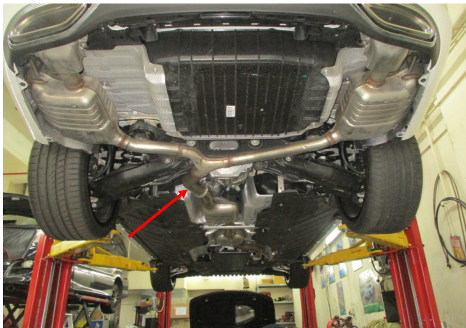
Photo 25 shows the rear section of the Motor Car's exhaust system. My examination of the Motor Car's exhaust system revealed no sign(s) or indication(s) of any cut or weld marks along its exhaust pipes (arrowed), on its centre resonator boxes, on its rear mufflers and on its catalytic converter.
