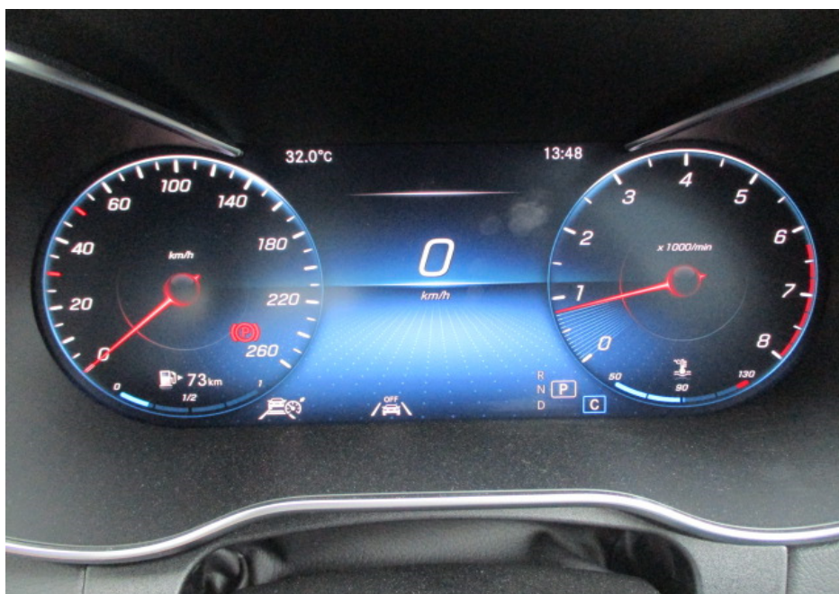
Photo 19 shows the respective warning lights no longer illuminated, indicating that there is no fault detected to the ABS, SRS, EPS and TCS systems of the Motor Car during the self-test. These electronic systems were hence in working condition at the time of my inspection.
