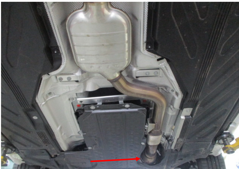
Photo 26 shows the front section of the Motor Car's exhaust system. My examination of the Motor Car's exhaust system revealed no sign(s) or indication(s) of any cut or weld marks along its exhaust pipes, on its centre resonator boxes, on its rear mufflers and on its catalytic converter (arrowed).
