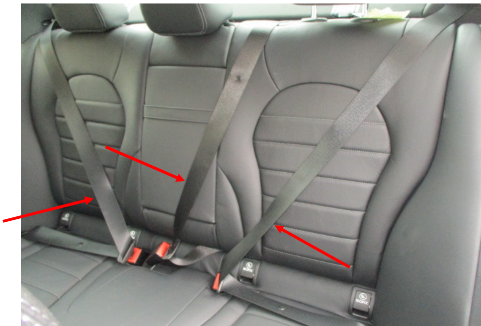
Photo 17 shows the rear seats of the Motor Car. All the seats of the Motor Car were secured via seat rails to the floorboard. They were also fitted with a retractable seat belt reel and a pre-tensioner. The seat belts (arrowed) were tested and were able to be fastened into the respective pre-tensions that were fitted on the side of each individual seat.
