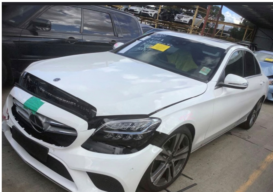
Photo 1 shows the front left body of the Motor Car (photograph provided to me). The Motor Car was observed to have sustained damage at its frontal portion. Body parts damaged include the front bumper and radiator grille amongst others.
