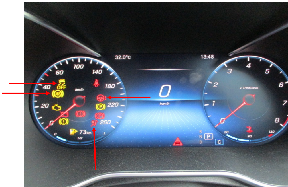
Photo 18 shows the warning lights for the various electronic safety features appearing on the instrument panel of the Motor Car during its self-test when the engine is cranked, in particular the ABS, SRS, EPS and TCS lights (arrowed).
