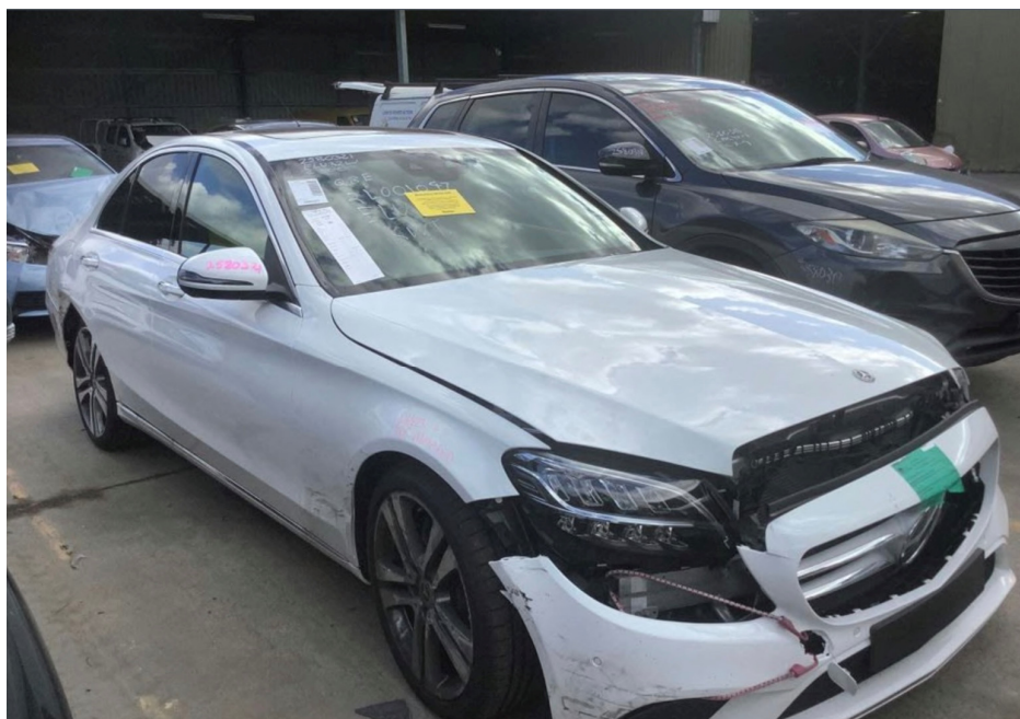
Photo 2 shows the front right body of the Motor Car (photograph provided to me). The Motor Car was observed to have sustained damage at its frontal portion. Body parts damaged include the front bumper and radiator grille amongst others.
