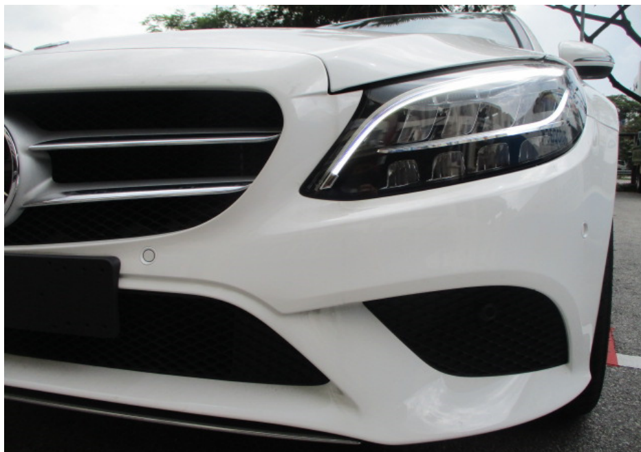
Photo 9 shows a closer view of the Motor Car's front bumper, front bumper left lower grille and front left headlamp. The body parts at the frontal portion of the Motor Car were visually examined and it was observed that the repair/restoration works carried out to the damaged area of the Motor Car (refer to photograph 1 & 2 above) were reasonably adequate and in order.
