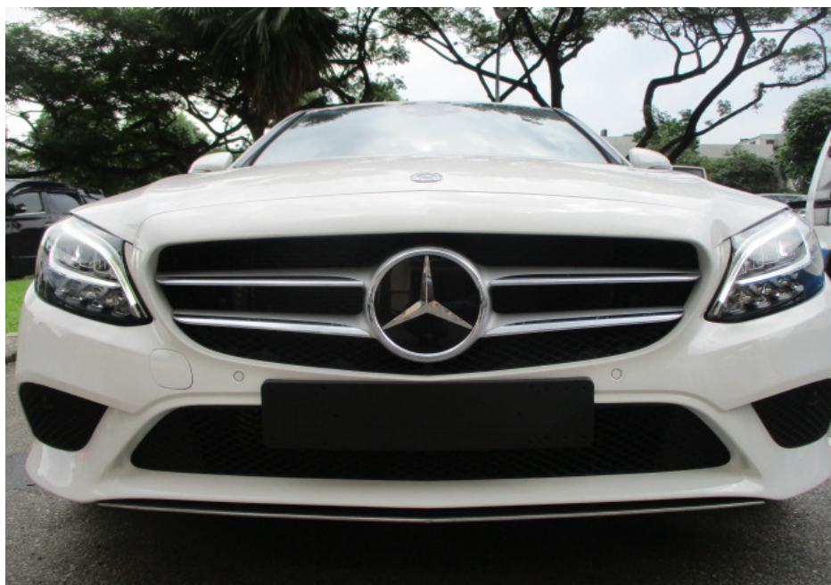
Photo 10 shows a closer view of the Motor Car's front bumper, radiator grille and radiator grille emblem. The body parts at the frontal portion of the Motor Car were visually examined and it was observed that the repair/restoration works carried out to the damaged area of the Motor Car (refer to photograph 1 & 2 above) were reasonably adequate and in order.
