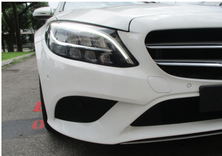
Photo 7 shows a closer view of the Motor Car's front bumper, front bumper right lower grille and front right headlamp. The body parts at the frontal portion of the Motor Car were visually examined and it was observed that the repair/restoration works carried out to the damaged area of the Motor Car (refer to photograph 1 & 2 above) were reasonably adequate and in order.
