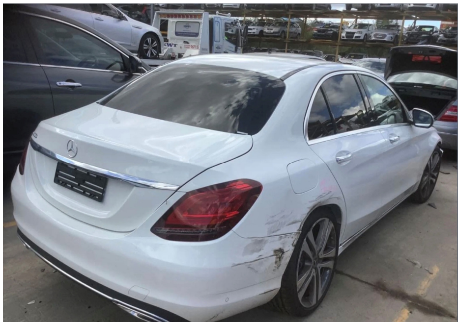
Photo 3 shows the rear right body the Motor Car (photograph provided to me). Apart for the frontal portion, I had also observed damage to the rear right portion of the Motor Car. Body parts damaged include the rear bumper and rear right fender amongst others.
