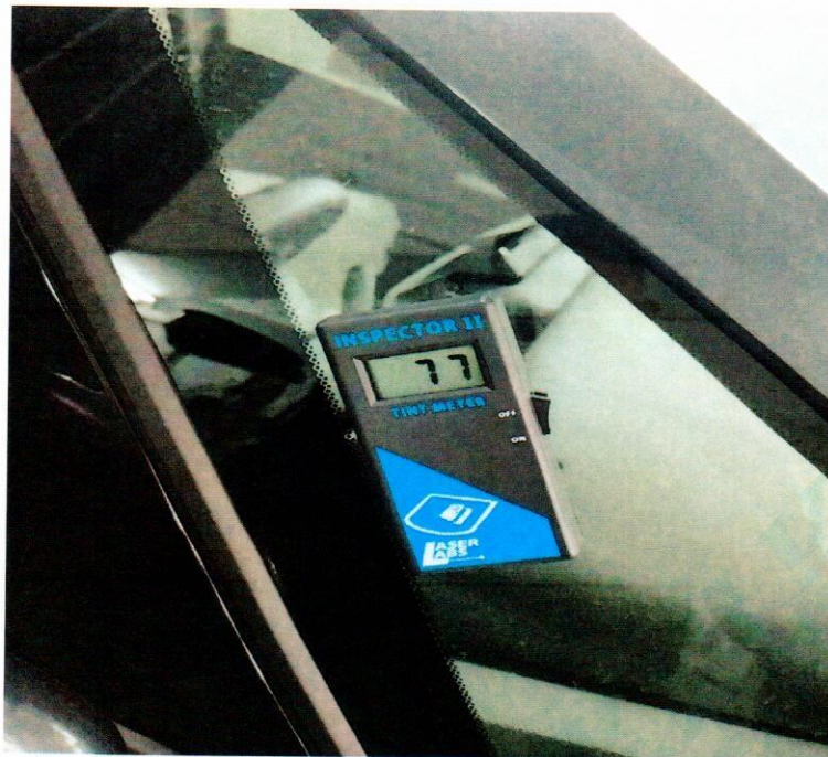
Front Quarter Glass VLT Reading: 77% (Right)
