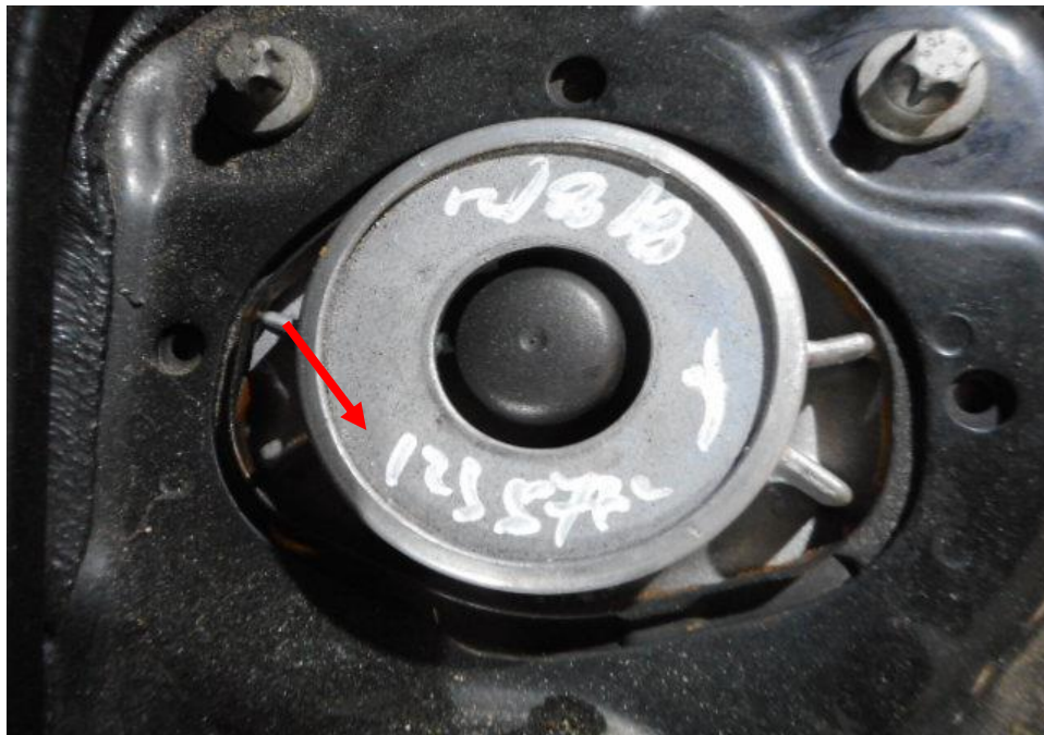
Photo 10 shows the close up view of the front right wheel of the Insured Vehicle at the time of our inspection. The suspension system (arrowed) is observed to be just replaced approximately 6,000km from the material time of inspection and visually unaffected by any signs of accident.
