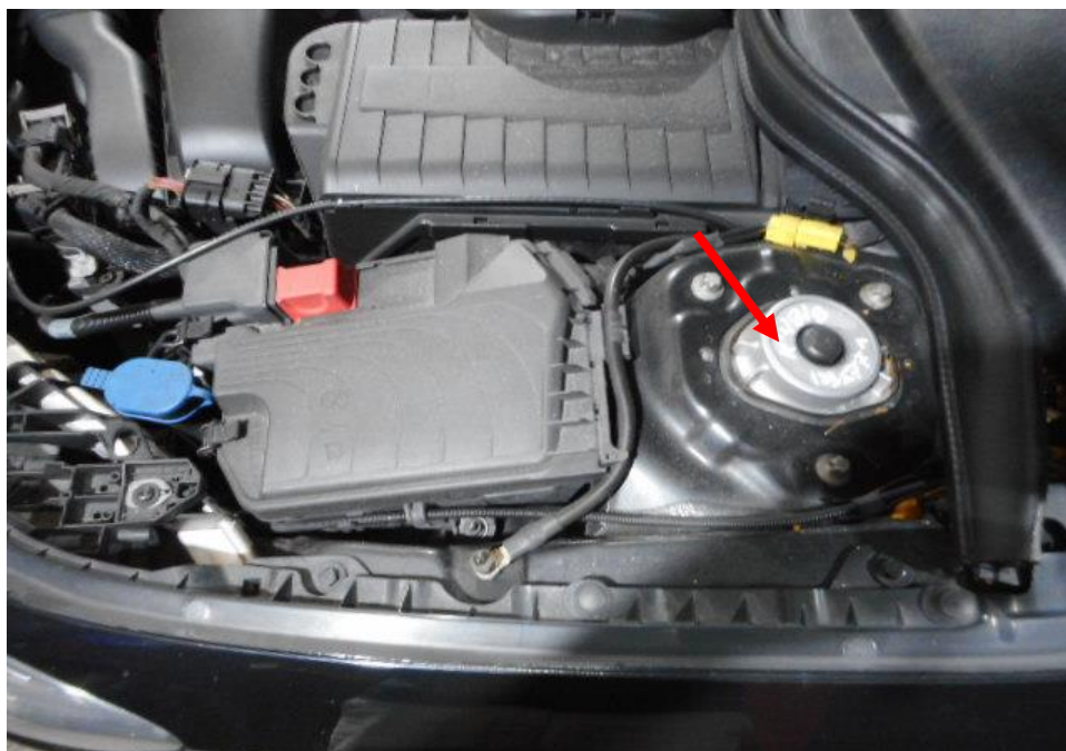
Photo 11 shows the general view of the front left wheel of the Insured Vehicle at the time of our inspection. The suspension system (arrowed) is observed to be just replaced approximately 6,000km from the material time of inspection and visually unaffected by any signs of accident.
