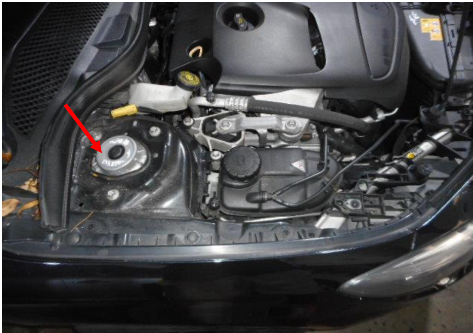
Photo 9 shows the general view of the front right wheel of the Insured Vehicle at the time of our inspection. The suspension system (arrowed) is observed to be just replaced approximately 6,000km from the material time of inspection and visually unaffected by any signs of accident.
