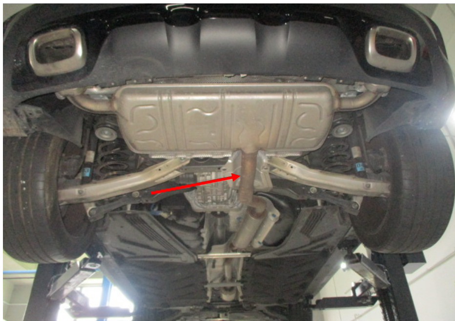
Photo 22 shows the rear section of the Motor Car's exhaust system. My examination of the Motor Car's exhaust system revealed no sign(s) or indication(s) of any cut or weld marks along its exhaust pipes (arrowed), on its centre resonator boxes, on its rear muffler and on its catalytic converter.
