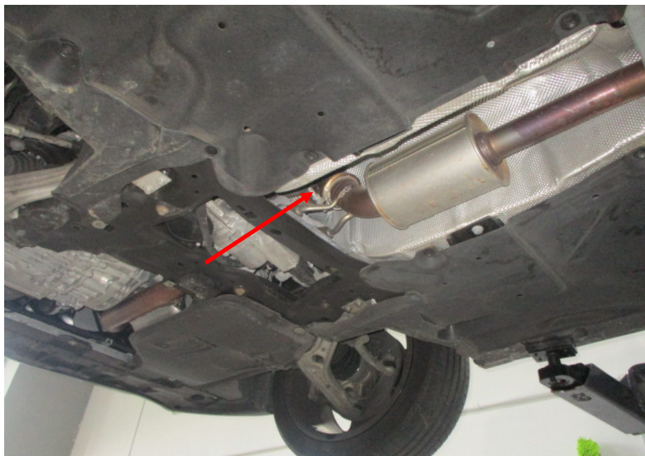
Photo 23 shows the front section of the Motor Car's exhaust system. My examination of the Motor Car's exhaust system revealed no sign(s) or indication(s) of any cut or weld marks along its exhaust pipes, on its centre resonator boxes, on its rear muffler and on its catalytic converter (arrowed).
