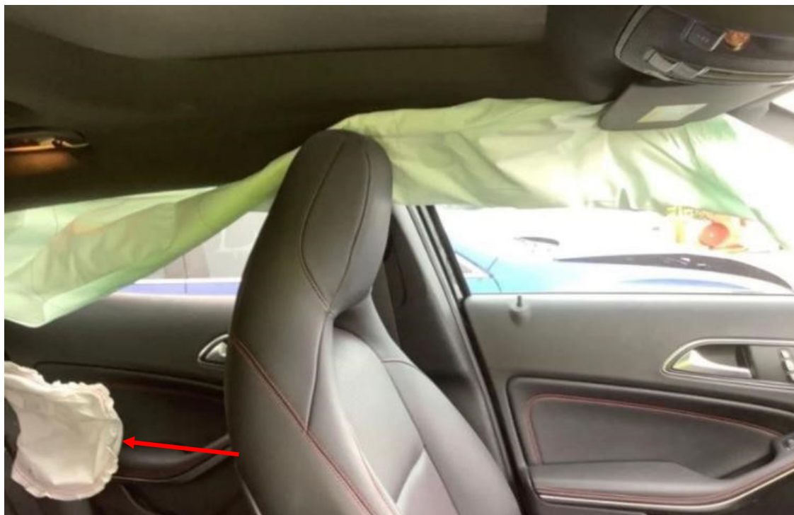
Photo 3 shows the interior compartment of the Motor Car (photograph provided to me). The left side curtain airbag and rear left passenger seat airbag (arrowed) were deployed.
