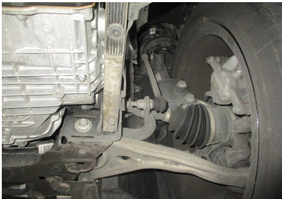
Photo 20 shows the various undercarriage components at the front left wheel of the Motor Car. I did not observe any fluid leak and/or fluid stain on the underside of the Motor Car. All the Motor Car's undercarriage components were observed to be intact and secured in an appropriate manner.
