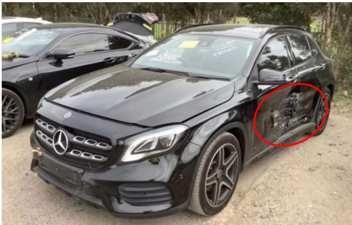
Photo 1 shows the front left body of the Motor Car (photograph provided to me). The Motor Car was observed to have sustained damage at its left side centre portion (circled). Body parts damaged include the left front door, left rear door and left side rocker panel garnish amongst others.
