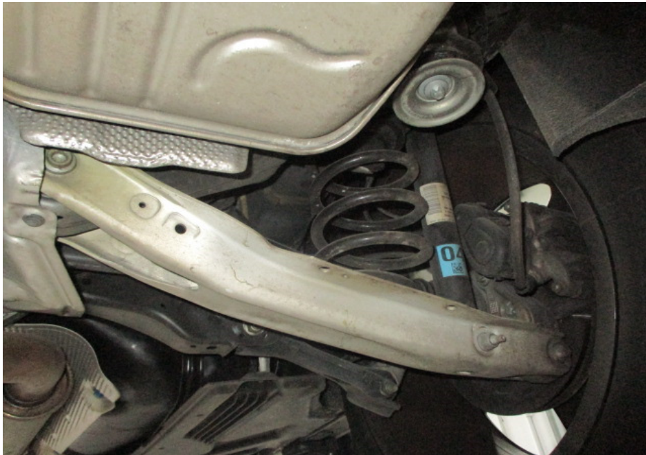
Photo 18 shows a general view of the control arms and linkages at the rear right wheel of the Motor Car. I did not observe any fluid leak and/or fluid stain on the underside of the Motor Car. All the Motor Car's undercarriage components were observed to be intact and secured in an appropriate manner.
