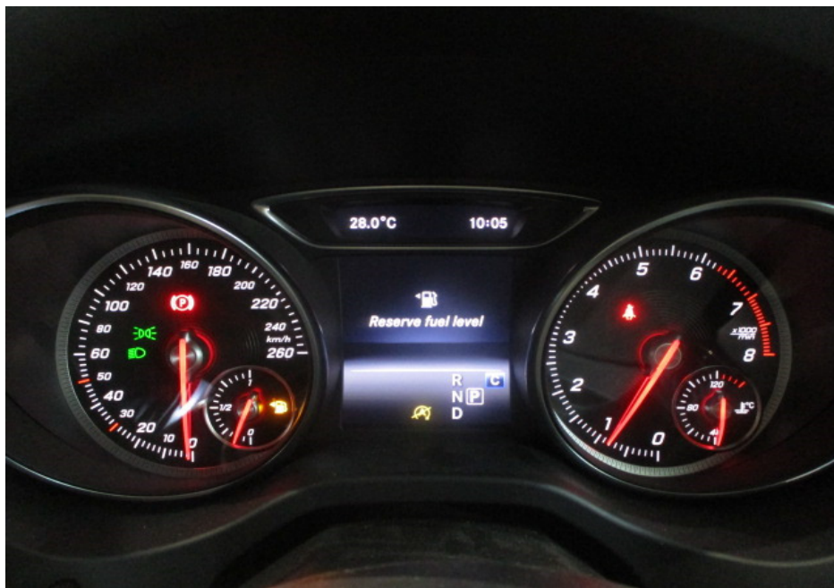
Photo 16 shows the respective warning lights no longer illuminated, indicating that there is no fault detected to the ABS, SRS and TCS systems of the Motor Car during the self-test. These electronic systems were hence in working condition at the time of my inspection.
