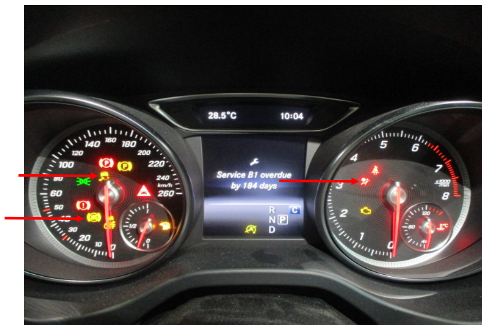
Photo 15 shows the warning lights for the various electronic safety features appearing on the instrument panel of the Motor Car during its self-test when the engine is cranked, in particular the ABS, SRS and TCS lights (arrowed).
