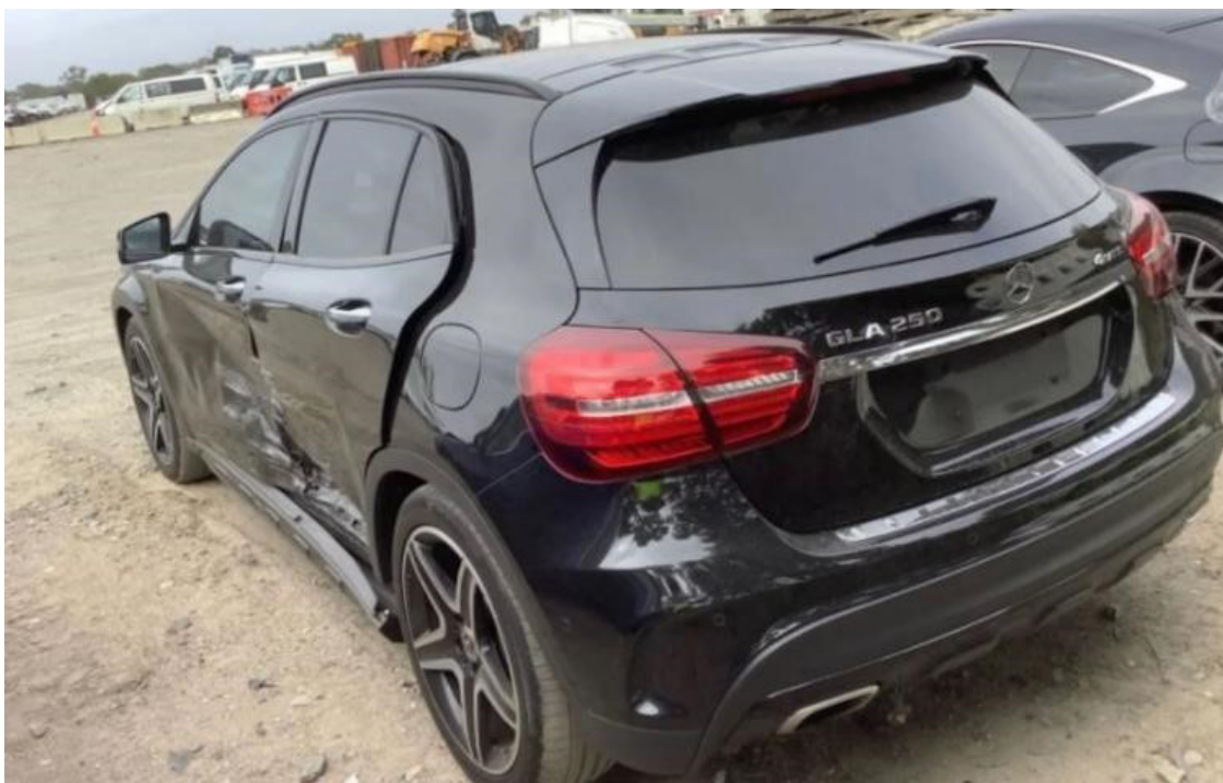
Photo 2 shows the rear left body of the Motor Car (photograph provided to me). The Motor Car was observed to have sustained damage at its left side centre portion. Body parts damaged include the left front door, left rear door and left side rocker panel garnish amongst others.
