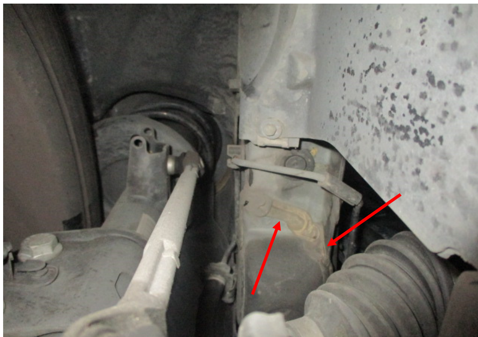
Photo 27 shows the chassis/structural body at the underside front right of the Motor Car. The original factory sealant (arrowed) at the joints along the chassis/structural body was observed to be untouched. In general, I had found no work was carried out on the chassis/structural body of the Motor Car. The chassis/structural body of the Motor Car was originally fitted.
