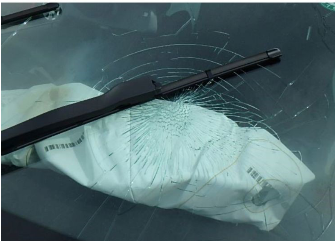
Photo 5 shows a closer view of the cracked front windscreen of the Motor Car (photograph provided to me). The front left passenger airbag was deployed.
