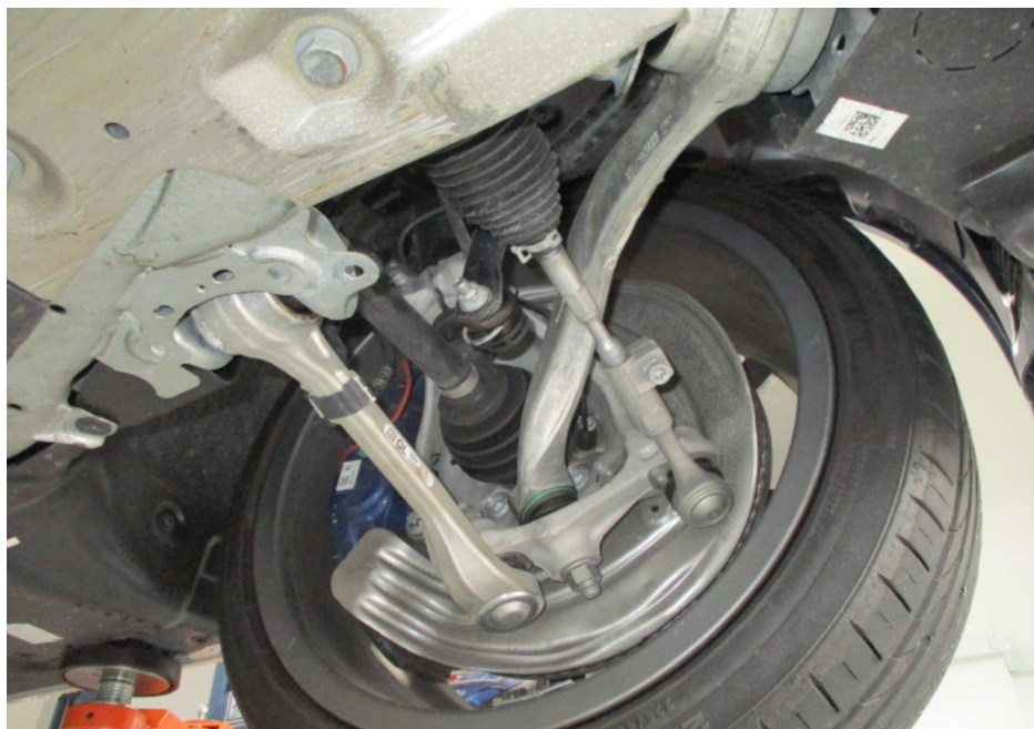
Photo 22 shows the various undercarriage components at the front left wheel of the Motor Car. The mechanical components, control arms and linkages were all found to be intact and secured in an appropriate manner. The undercarriage parts at the front left portion of the Motor Car were visually examined and it was observed that the repair/restoration works carried out to the damaged area of the Motor Car (refer to photograph 1 - 3 above) were reasonably adequate and in order.
