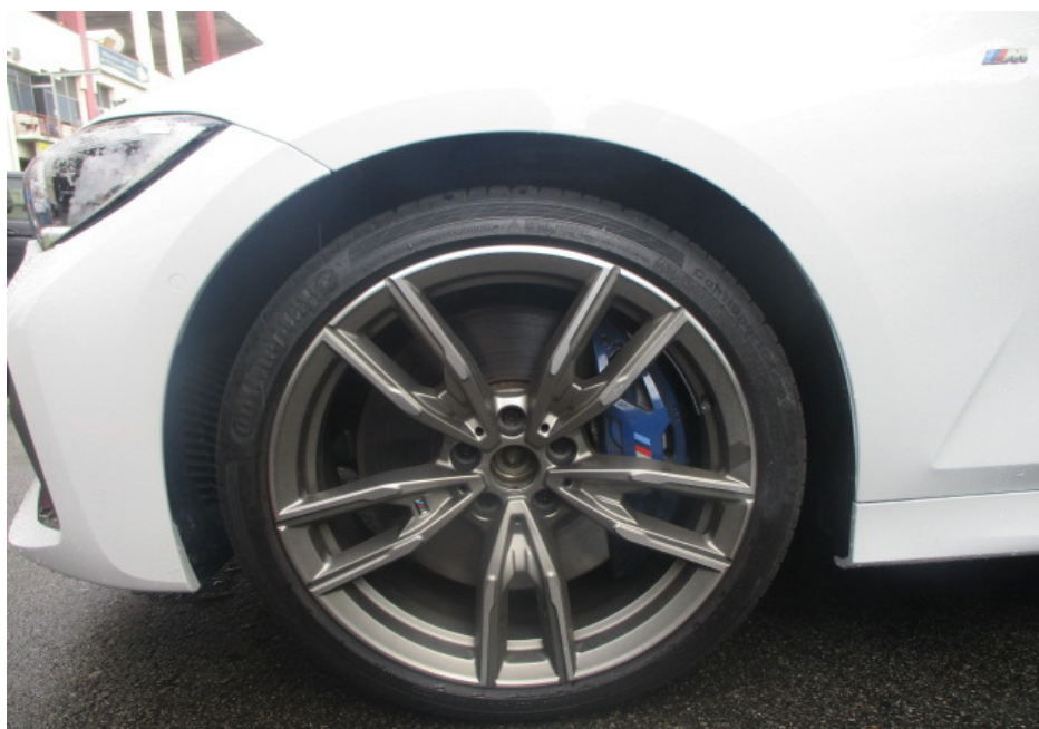
Photo 9 shows a closer view of the Motor Car's front bumper, front left fender, front left tyre and front left wheel rim. The body parts and undercarriage parts at the front left portion of the Motor Car were visually examined and it was observed that the repair/restoration works carried out to the damaged area of the Motor Car (refer to photograph 1, 2, 3 and 5 above) were reasonably adequate and in order.
