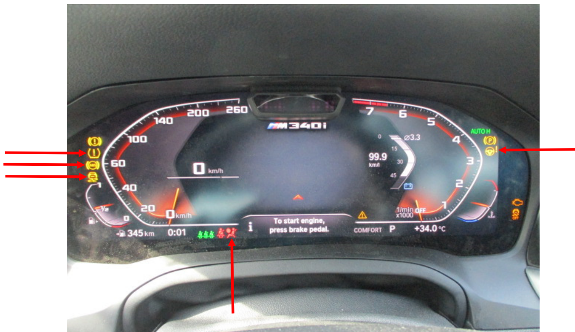
Photo 17 shows the warning lights for the various electronic safety features appearing on the instrument panel of the Motor Car during its self-test when the engine is cranked, in particular the ABS, SRS, IAS, TPM and DSC lights (arrowed).
