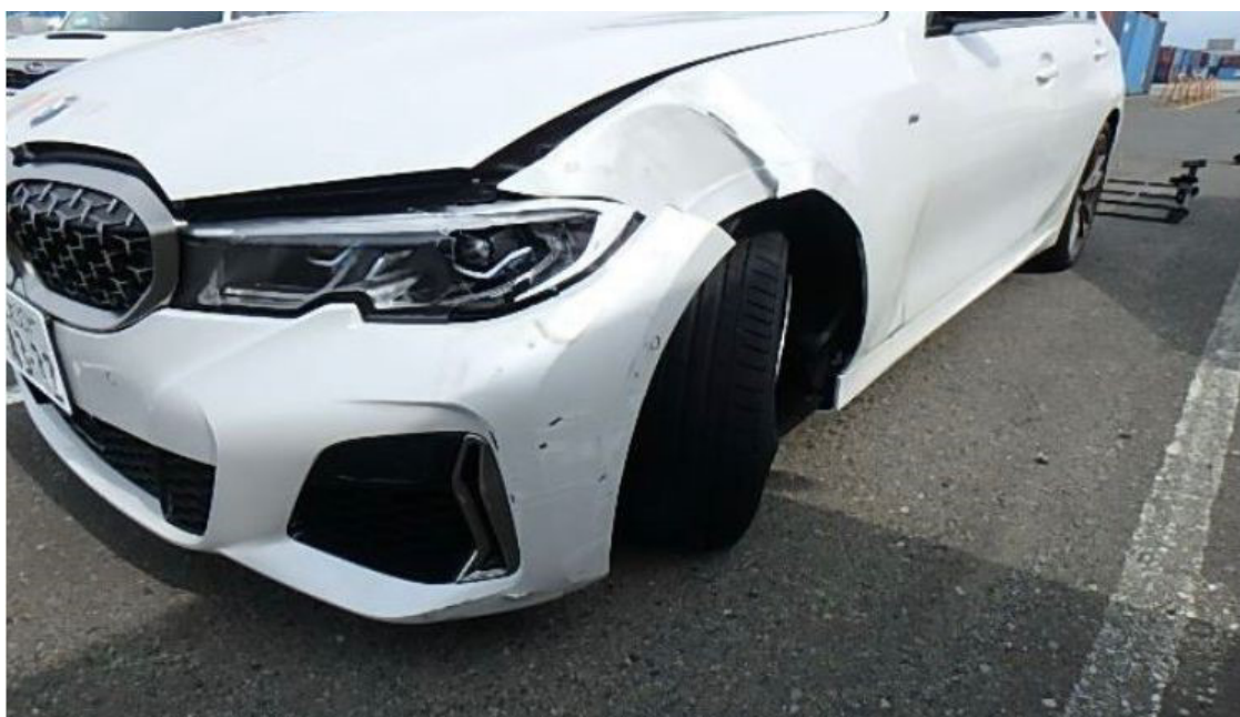
Photo 3 shows a closer view of the front left body of the Motor Car (photograph provided to me). The Motor Car was observed to have sustained damage at its front left portion. Body parts damaged include the front bumper, front bonnet, front left headlamp and front left fender amongst others.
