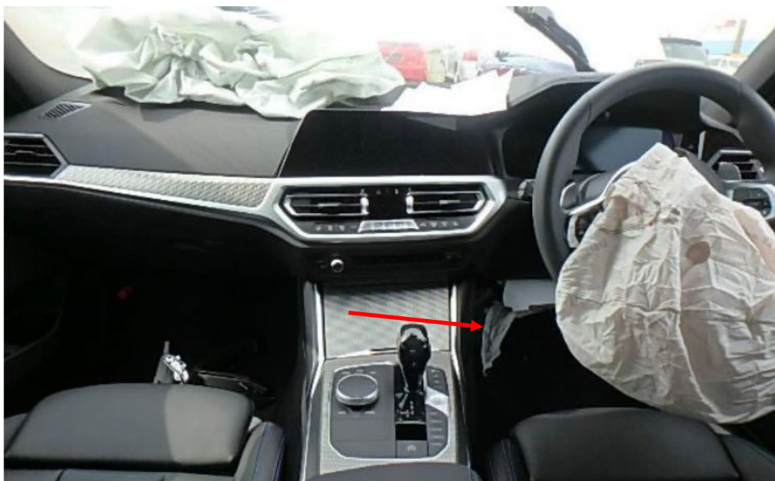
Photo 6 shows the interior compartment of the Motor Car (photograph provided to me). The front left passenger airbag, driver airbag and driver knee airbag (arrowed) were deployed.
