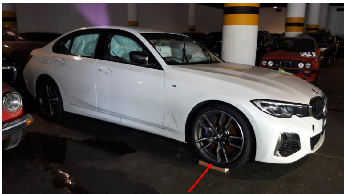
Photo 4 shows the front right body of the Motor Car (photograph provided to me). The front right portion of the Motor Car was observed to be relatively unaffected. The front left wheel (refer to photograph 1 & 2 above) and front right wheel (arrowed) were orientated in different direction, which suggests damage to the Motor Car's front left undercarriage parts. The right side curtain airbag was deployed.
