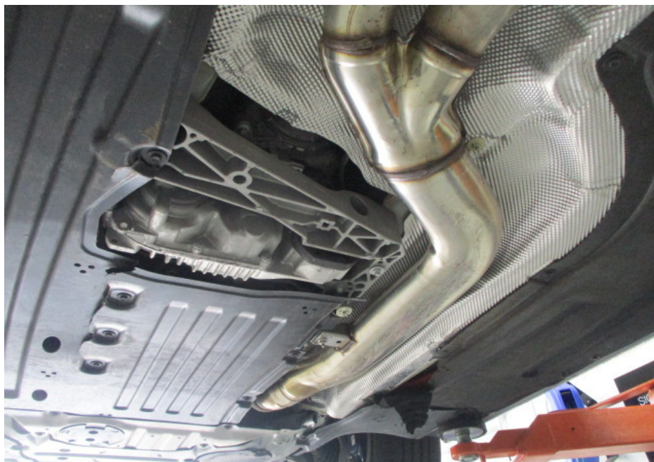
Photo 25 shows the front section of the Motor Car's exhaust system. My examination of the Motor Car's exhaust system revealed no sign(s) or indication(s) of any cut or weld marks along its exhaust pipes, on its rear muffler and on its catalytic converter.
