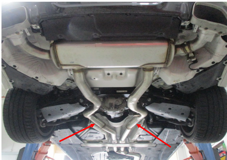
Photo 24 shows the rear section of the Motor Car's exhaust system. My examination of the Motor Car's exhaust system revealed no sign(s) or indication(s) of any cut or weld marks along its exhaust pipes (arrowed), on its rear muffler and on its catalytic converter.
