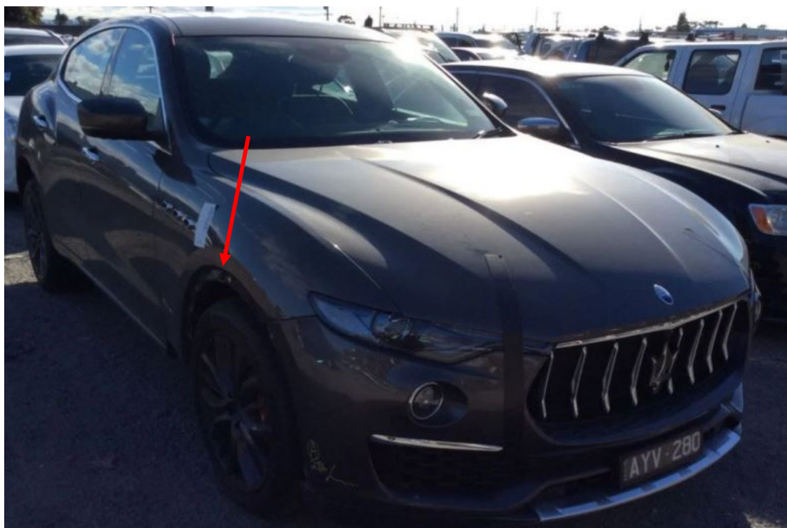
Photo 2 shows the front right body of the Motor Car (photograph provided to me). The front right fender wheel arc garnish (arrowed) was observed to be missing/dislodged/damaged. Apart for this, there was no physical damage observed to the exterior body of the Motor Car.
