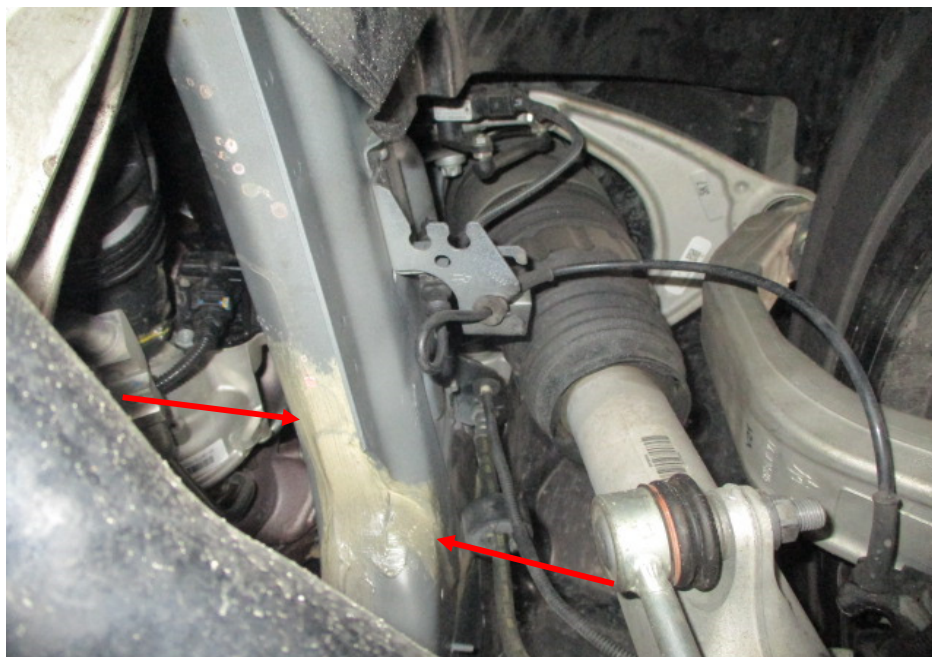
Photo 27 shows the chassis/structural body at the underside front left of the Motor Car. I did not find any weld marks other than original spot weld marks on the chassis/structural body of the Motor Car. The original factory sealant (arrowed) at the joints along the chassis/structural body was untouched, indicating no work was done on the chassis/structural body of the Motor Car and that the chassis/structural body was originally fitted.
