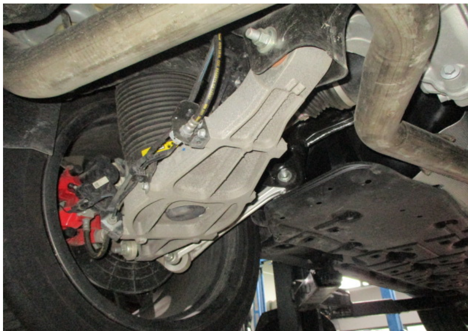
Photo 20 shows a general view of the control arms and linkages at the rear left wheel of the Motor Car. I did not observe any fluid leak and/or fluid stain on the underside of the Motor Car. All the Motor Car's undercarriage components were observed to be intact and secured in an appropriate manner.
