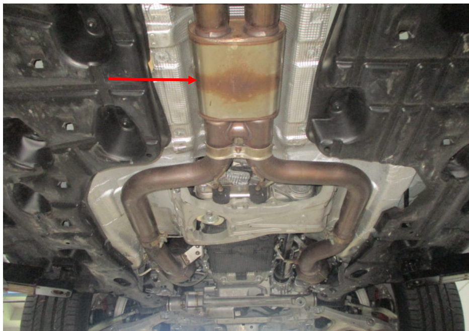
Photo 24 shows the front section of the Motor Car's exhaust system. My examination of the Motor Car's exhaust system revealed no sign(s) or indication(s) of any cut or weld marks along its exhaust pipes, on its centre resonator box (arrowed), on its rear mufflers and on its catalytic converters.
