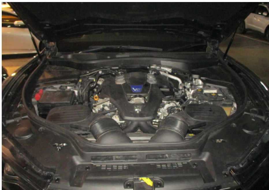
Photo 13 shows a general view of the engine compartment of the Motor Car at the time of my inspection. The various parts and components within the engine compartment were all observed to be intact and properly fitted. There was also no sign(s) or indication(s) of fluid leak and/or fluid stain found inside the engine compartment.
