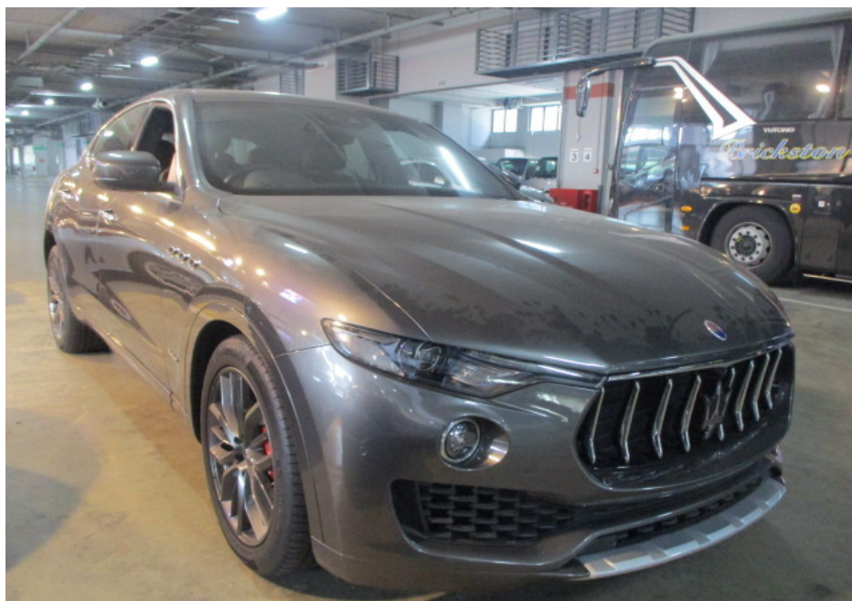
Photo 8 shows a general view of the front right body of the Motor Car at the time of my inspection. The Motor Car was observed to be in a relatively good general condition with no loose exterior fittings observed. The body parts of the Motor Car were visually examined, and it was noted that the repair/restoration works carried out to the damaged area of the Motor Car (refer to photograph 1 - 3 above) were reasonably adequate and in order.
