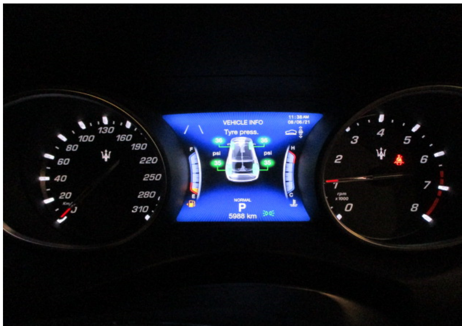
Photo 17 shows the respective warning lights no longer illuminated, indicating that there is no fault detected to the ABS, SRS, TPM and TCS systems of the Motor Car during the self-test. These electronic systems were hence in working condition at the time of my inspection.
