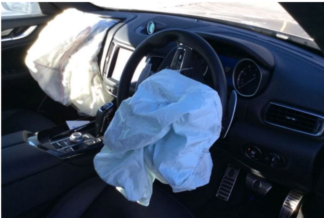
Photo 3 shows the interior compartment of the Motor Car (photograph provided to me). The driver airbag and front left passenger seat airbag were deployed.
