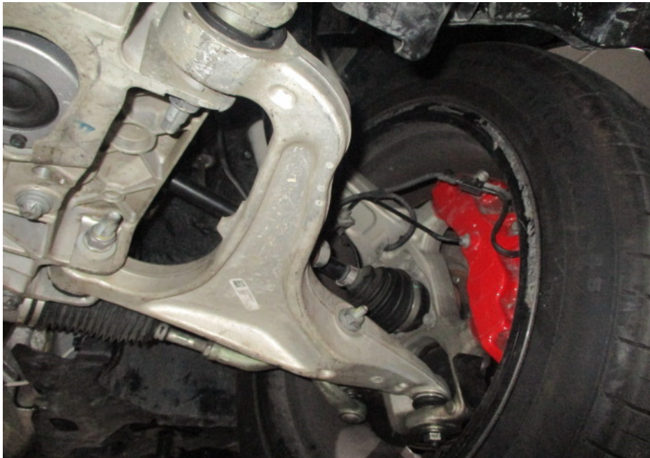
Photo 21 shows the various undercarriage components at the front left wheel of the Motor Car. I did not observe any fluid leak and/or fluid stain on the underside of the Motor Car. All the Motor Car's undercarriage components were observed to be intact and secured in an appropriate manner.
