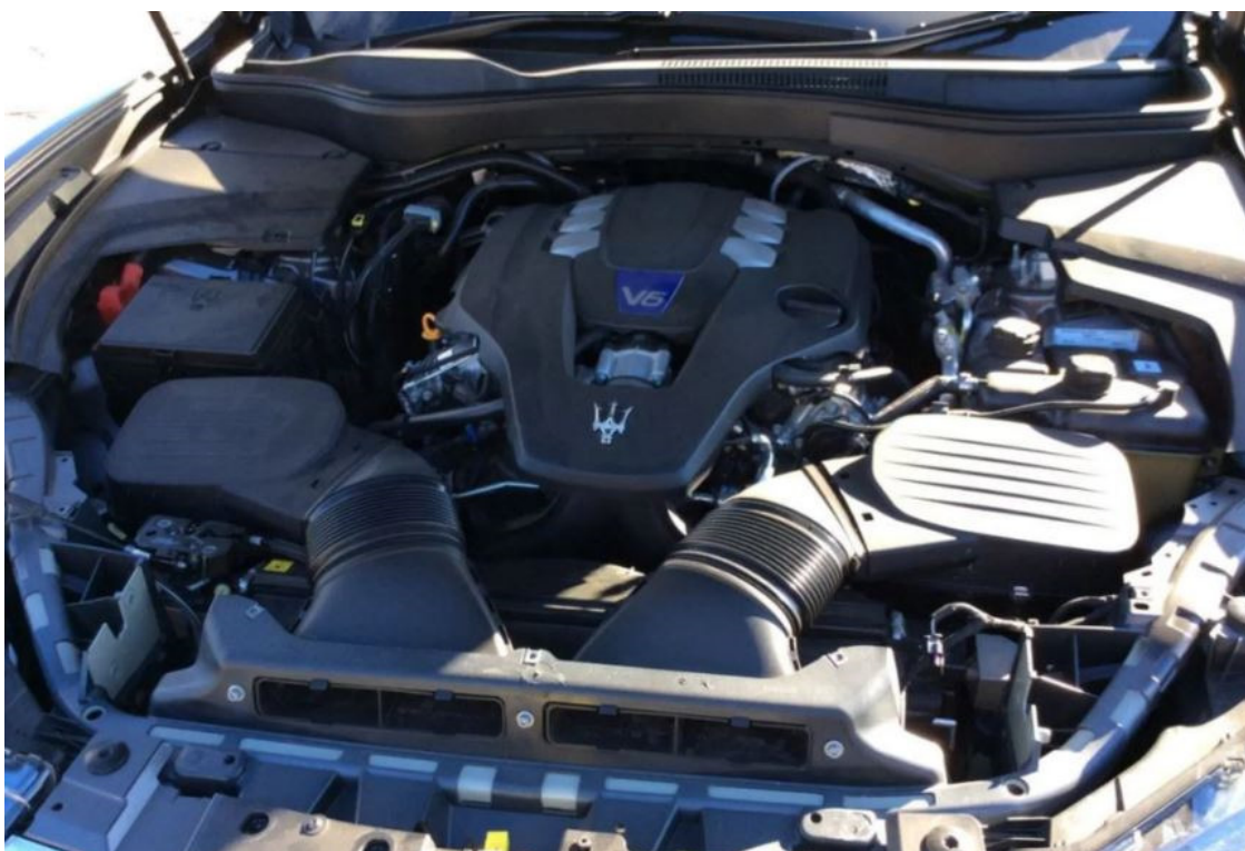
Photo 4 shows the engine compartment of the Motor Car (photograph provided to me). The various parts and components within the engine compartment were intact and unaffected.
