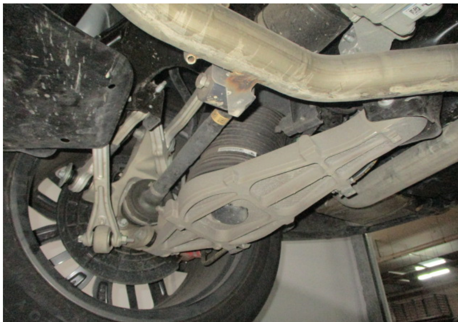
Photo 19 shows a general view of the control arms and linkages at the rear right wheel of the Motor Car. I did not observe any fluid leak and/or fluid stain on the underside of the Motor Car. All the Motor Car's undercarriage components were observed to be intact and secured in an appropriate manner.
