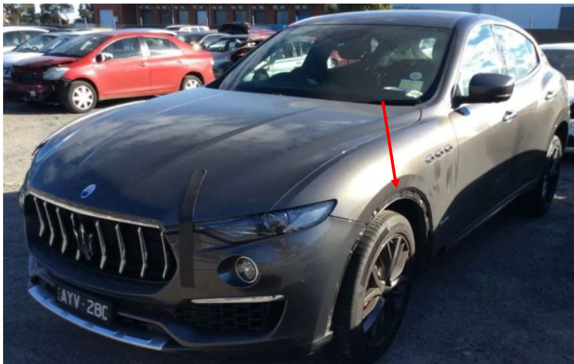
Photo 1 shows the front left body of the Motor Car (photograph provided to me). The front left fender wheel arc garnish (arrowed) was observed to be missing/dislodged/damaged. Apart for this, there was no physical damage observed to the exterior body of the Motor Car.
