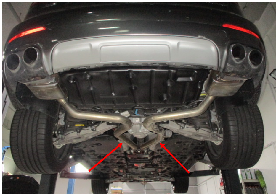
Photo 23 shows the rear section of the Motor Car's exhaust system. My examination of the Motor Car's exhaust system revealed no sign(s) or indication(s) of any cut or weld marks along its exhaust pipes (arrowed), on its centre resonator box, on its rear mufflers and on its catalytic converters.
