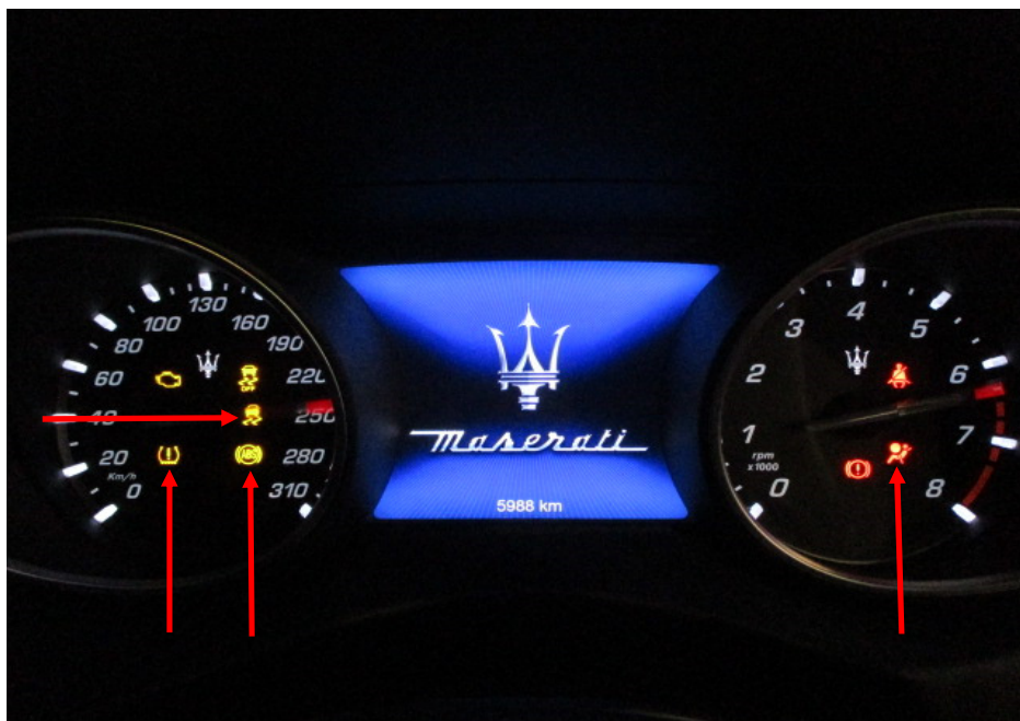
Photo 16 shows the warning lights for the various electronic safety features appearing on the instrument panel of the Motor Car during its self-test when the engine is cranked, in particular the ABS, SRS, TPM and TCS lights (arrowed).
