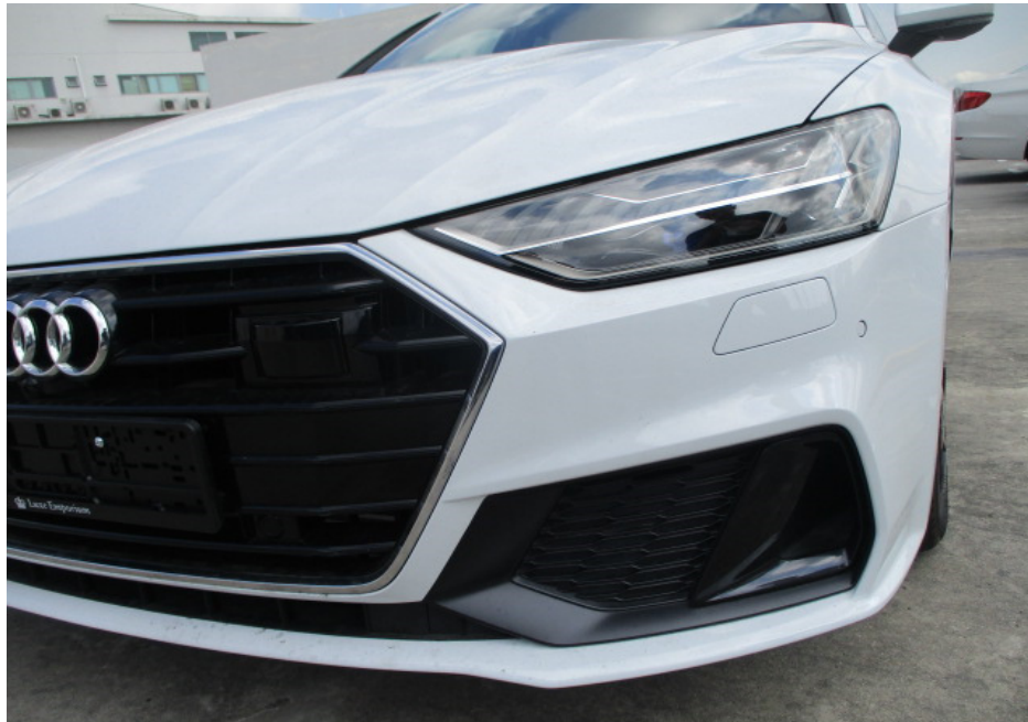
Photo 10 shows a closer view of the Motor Car's front bumper, front bumper left lower grille and garnish. The body parts at the front right portion of the Motor Car were visually examined and it was observed that the repair/restoration works carried out to the damaged area of the Motor Car (refer to photograph 1 - 3 above) were reasonably adequate and in order.
