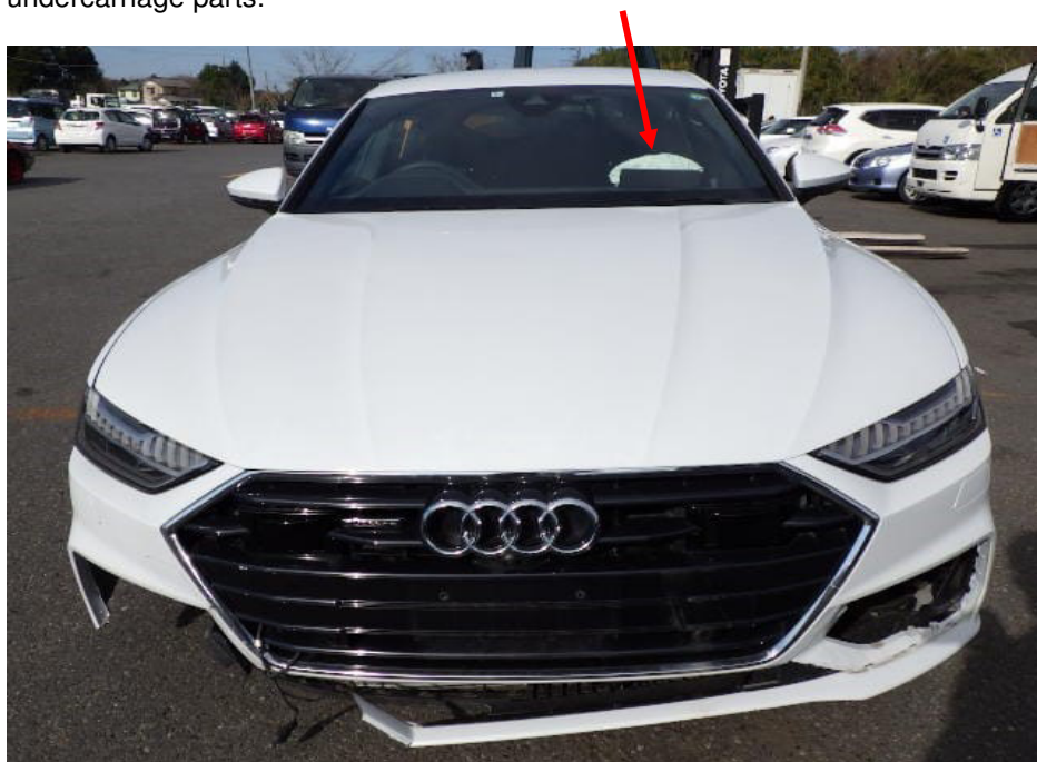
Photo 2 shows the frontal body of the Motor Car (photograph provided to me). The Motor Car was observed to have sustained damage at its front right portion. Body parts damaged include the front bumper, front bumper centre lower grille, front bumper right lower grille and garnish, front bumper left lower grille and garnish. The front left passenger airbag (arrowed) was deployed.
