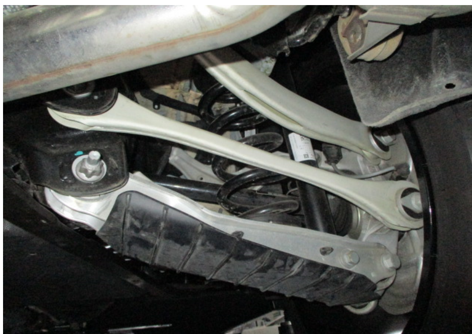
Photo 21 shows the various undercarriage components at the rear right wheel of the Motor Car. The mechanical components, control arms and linkages were all found to be intact and secured in an appropriate manner.
