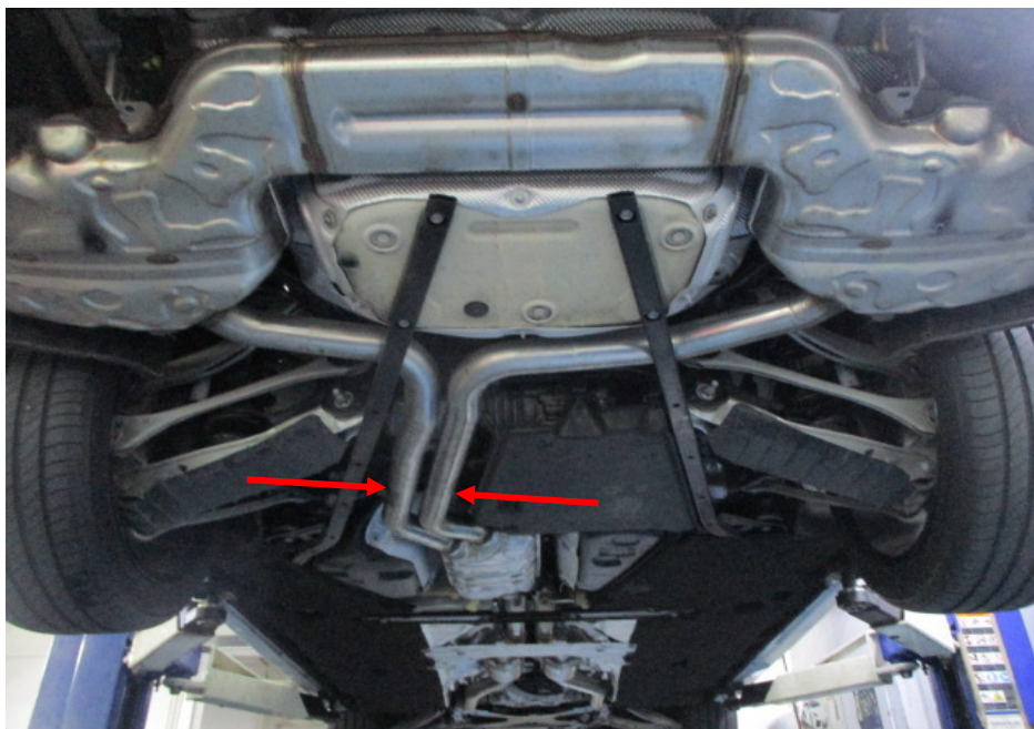
Photo 24 shows the rear section of the Motor Car's exhaust system. My examination of the Motor Car's exhaust system revealed no sign(s) or indication(s) of any cut or weld marks along its exhaust pipes (arrowed), on its centre resonator boxes, on its rear muffler and on its catalytic converters.
