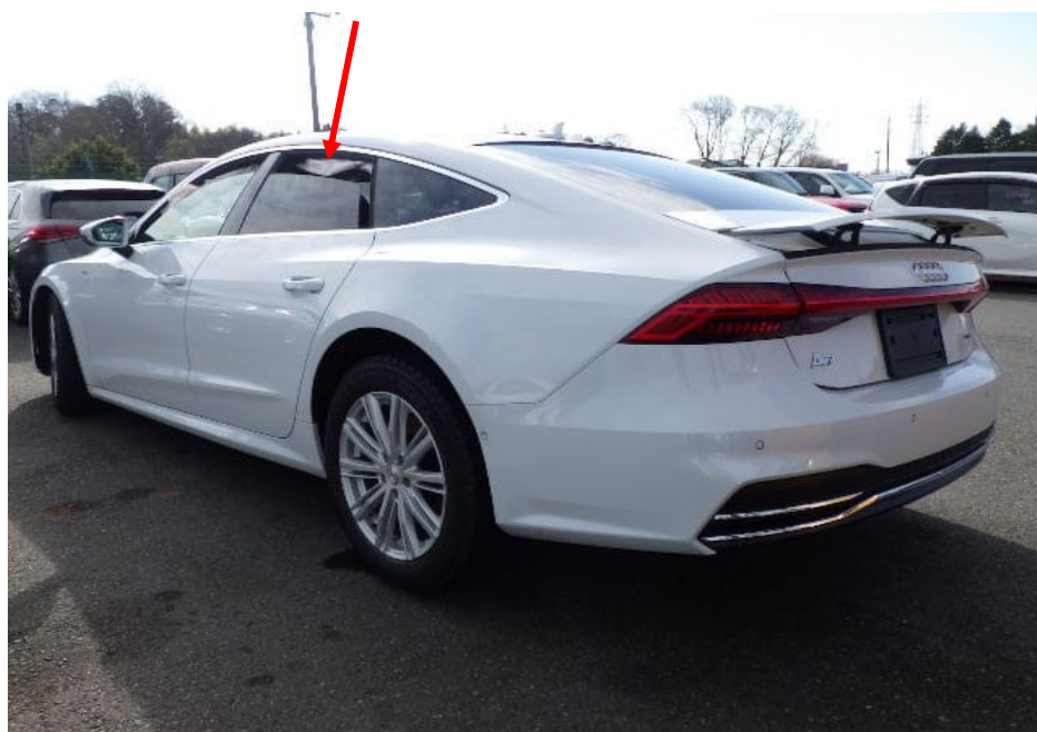
Photo 4 shows the rear left body of the Motor Car (photograph provided to me). Apart for the front right portion, there was no physical damage seen to other areas of the Motor Car. The left side curtain airbag (arrowed) of the Motor Car was deployed.
