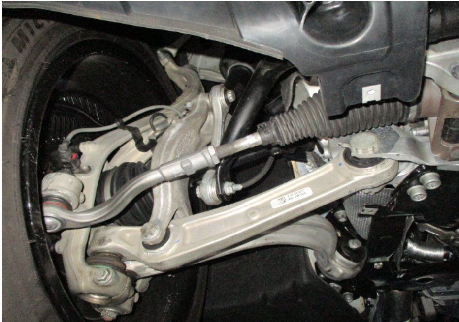
Photo 22 shows the various undercarriage components at the front right wheel of the Motor Car. The mechanical components, control arms and linkages were all found to be intact and secured in an appropriate manner. The undercarriage parts at the front right portion of the Motor Car were visually examined and it was observed that the repair/restoration works carried out to the damaged area of the Motor Car (refer to photograph 1 - 3 above) were reasonably adequate and in order.
