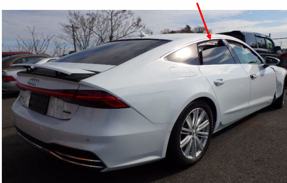
Photo 5 shows the rear right body of the Motor Car (photograph provided to me). Apart for the front right portion, there was no physical damage seen to other areas of the Motor Car. The right side curtain airbag (arrowed) of the Motor Car was deployed.
