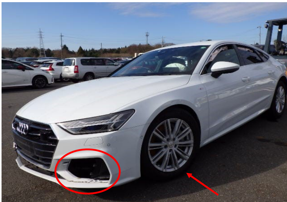
Photo 3 shows the front left body of the Motor Car (photograph provided to me). The front left portion of the Motor Car was relatively unaffected however I had observed that the front bumper left lower grille and garnish (circled) were dislodged/missing/damaged. The front left wheel (arrowed) and front right wheel (refer to photograph 1 above) were both orientated in an inward direction, which suggests damage to the Motor Car's front right undercarriage parts.
