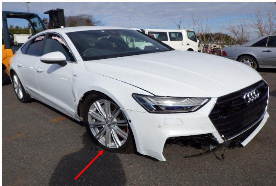
Photo 1 shows the front right body of the Motor Car (photograph provided to me). The Motor Car was observed to have sustained damage at its front right portion. Body parts damaged include the front bumper, front bumper right lower grille and garnish and front right fender amongst others. The front right wheel (arrowed) and front left wheel (refer to photograph 3 below) were both orientated in an inward direction, which suggests damage to the Motor Car's front right undercarriage parts.
