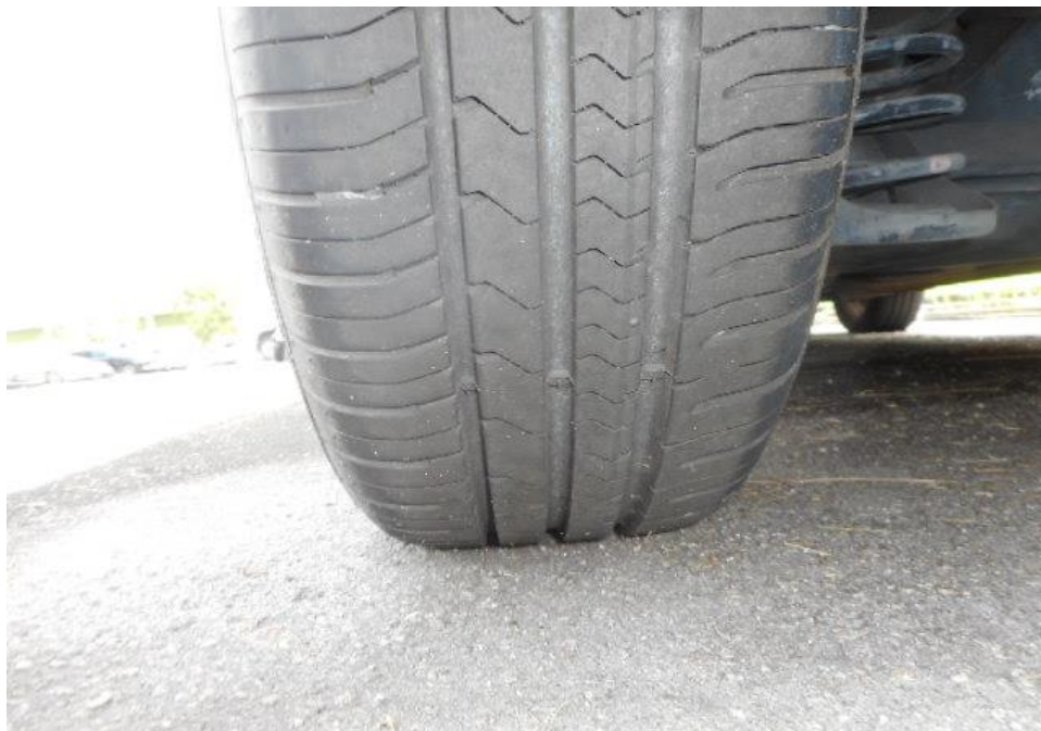
Photo 9 shows the condition of the rear left tyre of the Motor Car, which was observed to be in serviceable condition with remaining tread depth of approximately 6.7mm. The tyre, which was wrapped around steel wheel rim, was also observed to be sufficiently inflated for vehicular operation. The 4 tyres of the Motor Car were wrapped around standard steel wheel rims.
