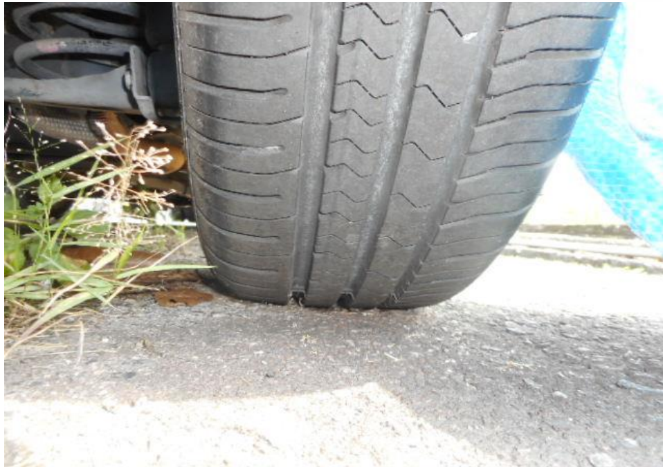
Photo 8 shows the condition of the rear right tyre of the Motor Car, which was observed to be in serviceable condition with remaining tread depth of approximately 6.7mm. The tyre was also observed to be sufficiently inflated for vehicular operation with no tear, cut or burst mark(s).
