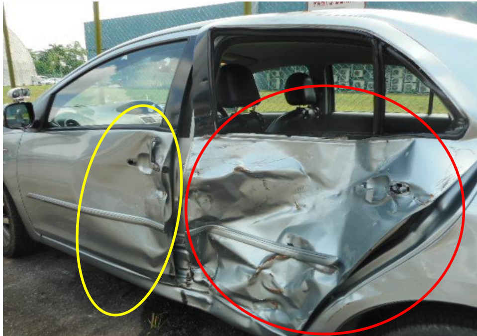
Photo 4 shows a close up view of the Motor Car's left body at the time of my inspection. The Motor Car was observed to have sustained damage at its left portion. Its left front (yellow circle) and rear door panel (red circle) were amongst the body parts that were damaged as a result of the accident.
