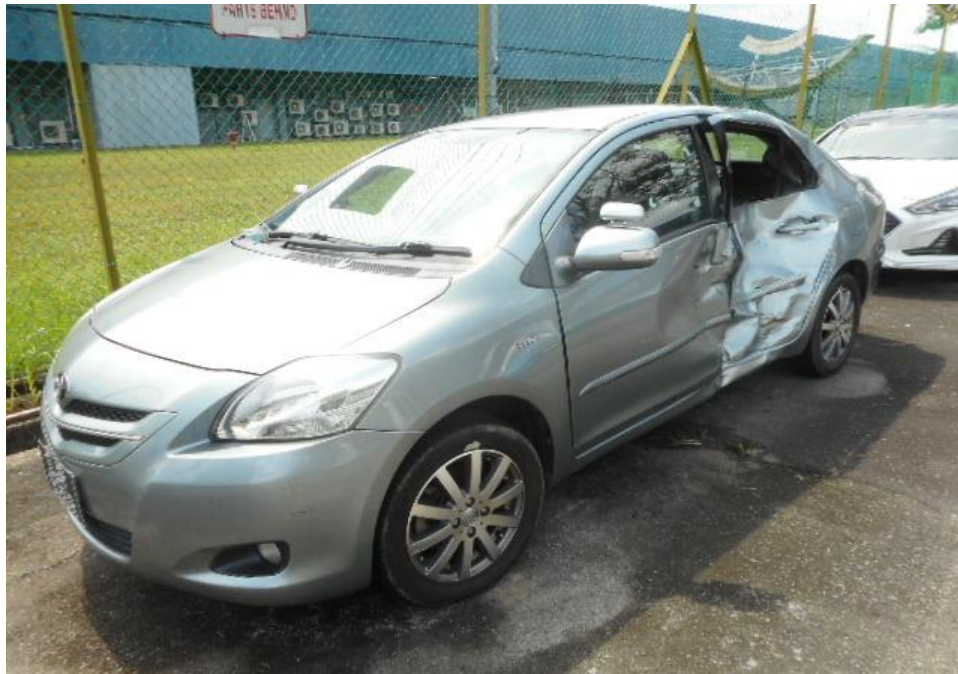
Photo 3 shows a general view of the Motor Car's left body at the time of my inspection. The Motor Car was observed to have sustained damage at its left portion. Its left front and rear door panel were amongst the body parts that were damaged as a result of the accident.
