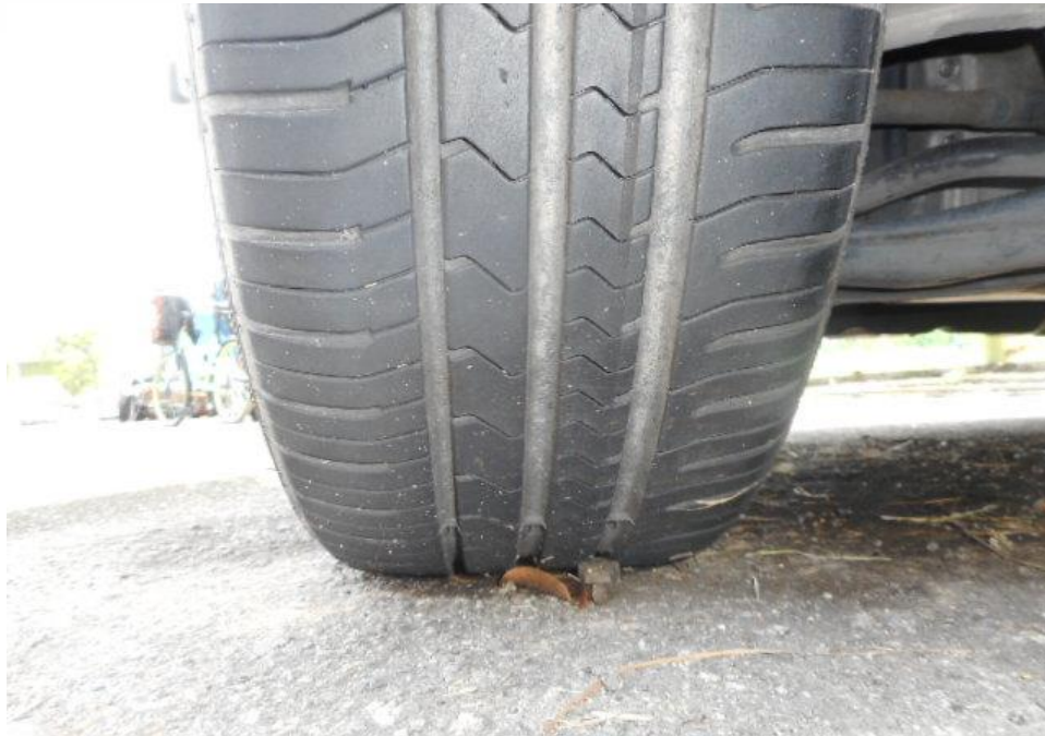
Photo 10 shows the condition of the front left tyre of the Motor Car, which was observed to be in serviceable condition with remaining tread depth of approximately 5.8mm. There was also no tear, cut or burst mark(s) on the outer and the inner sidewalls as well as across the tread of the Motor Car's 4 tyres.
