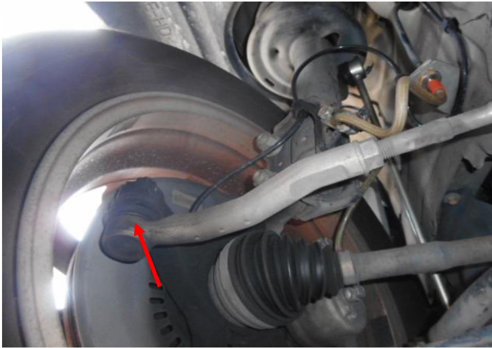
Photo 22 shows the various undercarriage components at the front left wheel of the Motor Car, which had included the steering tie rod (red arrow). The various undercarriage components of the Motor Car were all found to be intact without any visible damage.
