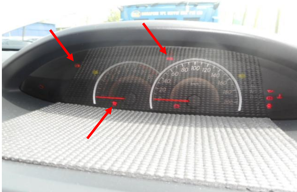
Photo 23 shows the warning light for Anti-Lock Brake System (ABS), Electric Power Steering System (EPS), and Supplemental Restraint System (SRS) (arrowed) appearing on the instrument panel of the Motor Car during the self-test of its various electronic operating systems when its engine was cranked.
