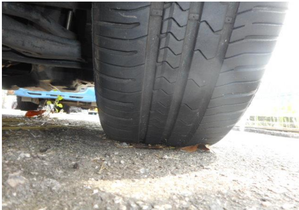
Photo 7 shows the condition of the front right tyre of the Motor Car, which was observed to be in serviceable condition with remaining tread depth of approximately 6mm. The tyre was sufficiently inflated for vehicular operation with no tear, cut or burst mark(s) on the outer and the inner sidewalls as well as across the tread. The 4 tyres of the Motor Car were wrapped around standard steel wheel rims without any damage.
